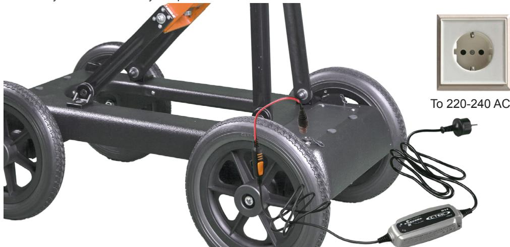
Charging battery with antenna outside of Handcart.
