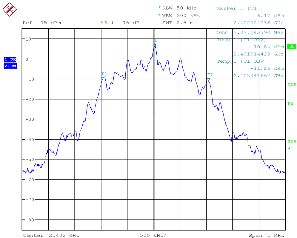
Figure 29: Chart of occupied bandwidth test on lowest channel, 2 Mbps
