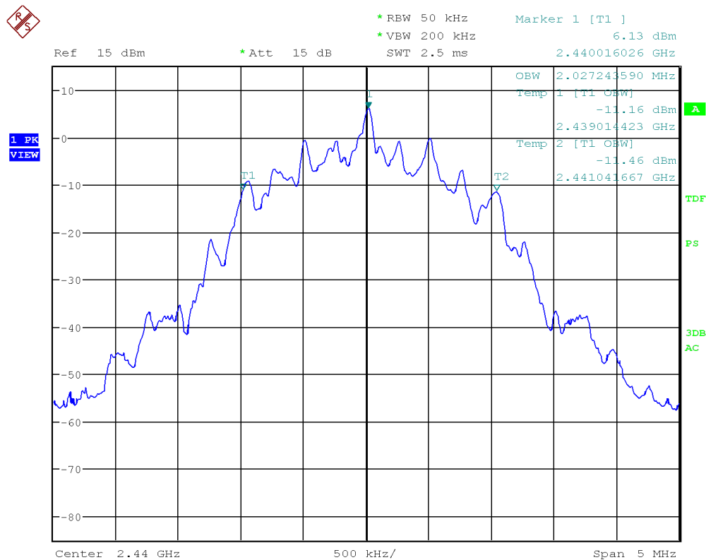
Figure 30: Chart of occupied bandwidth test on middle channel, 2 Mbps
