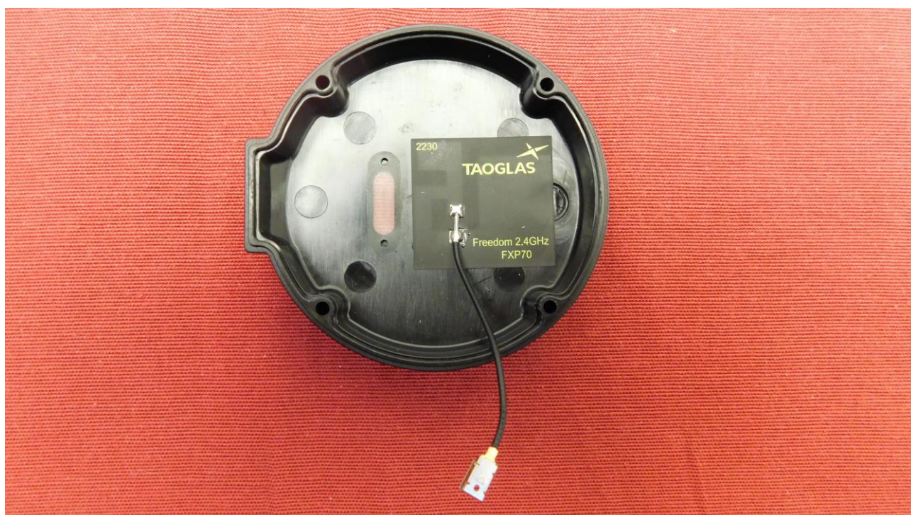
Picture 2: Cover with antenna – top view
