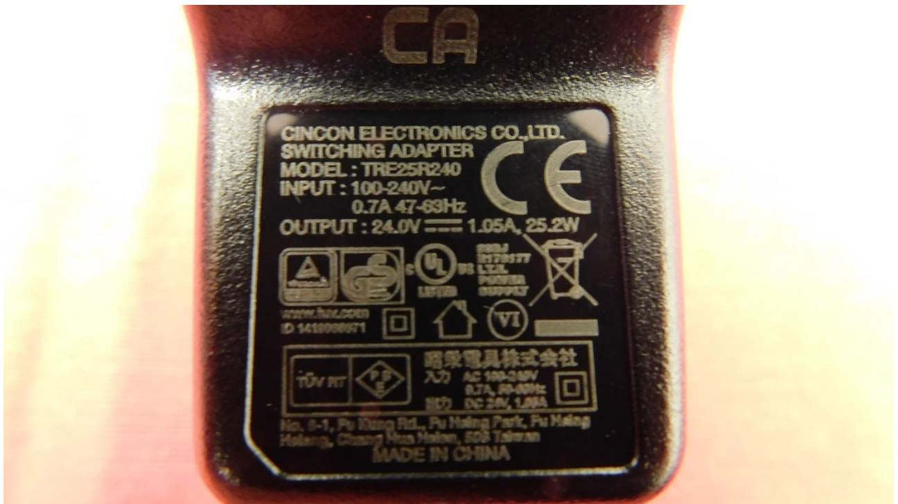
Picture 9: Name plate of power supply
