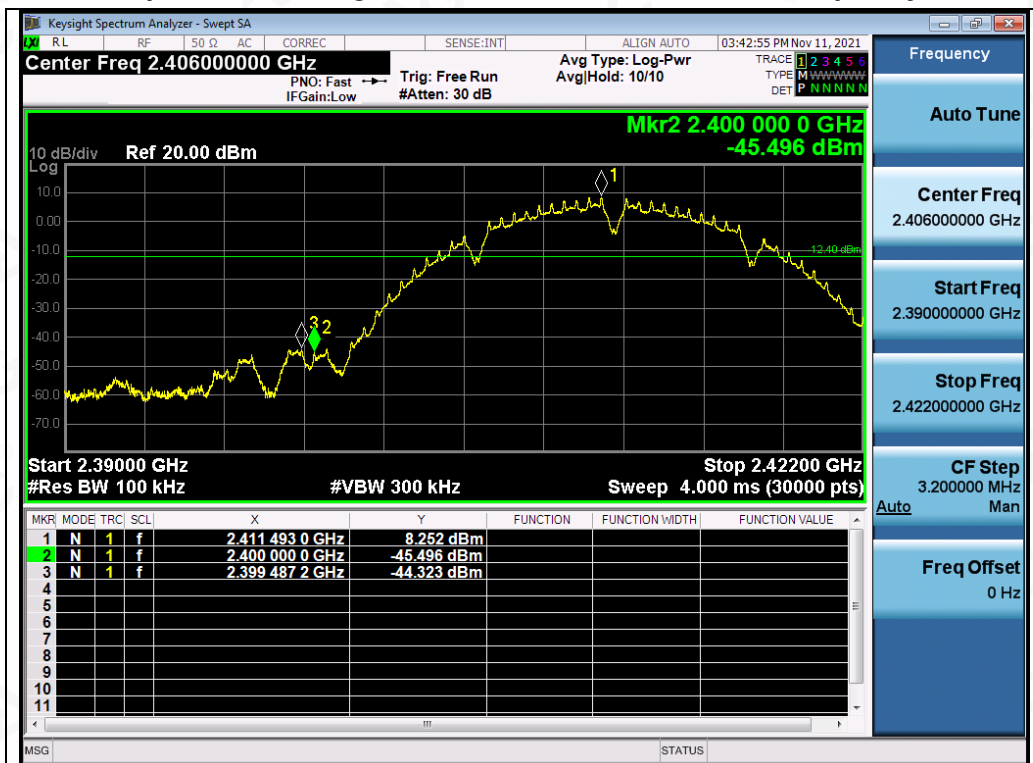
Test_Graph_802.11b_ANT1_2412_1Mbps_Lower Band Edge Emissions
