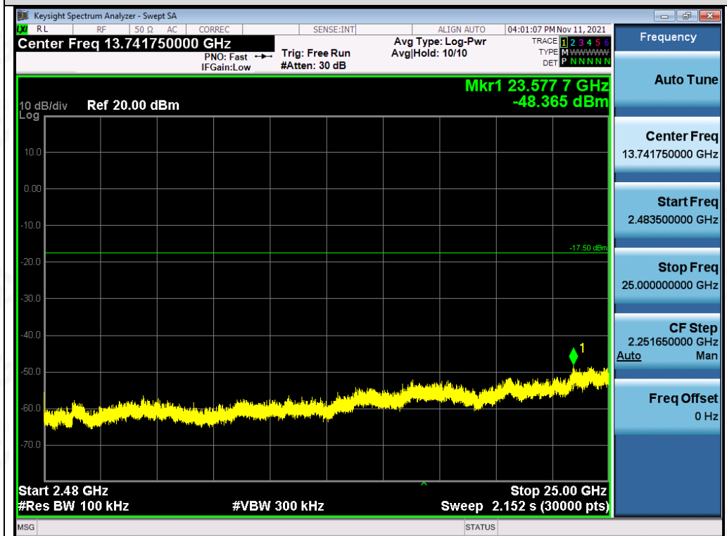
Test_Graph_802.11g_ANT1_2437_6Mbps_Higher Band Emissions
