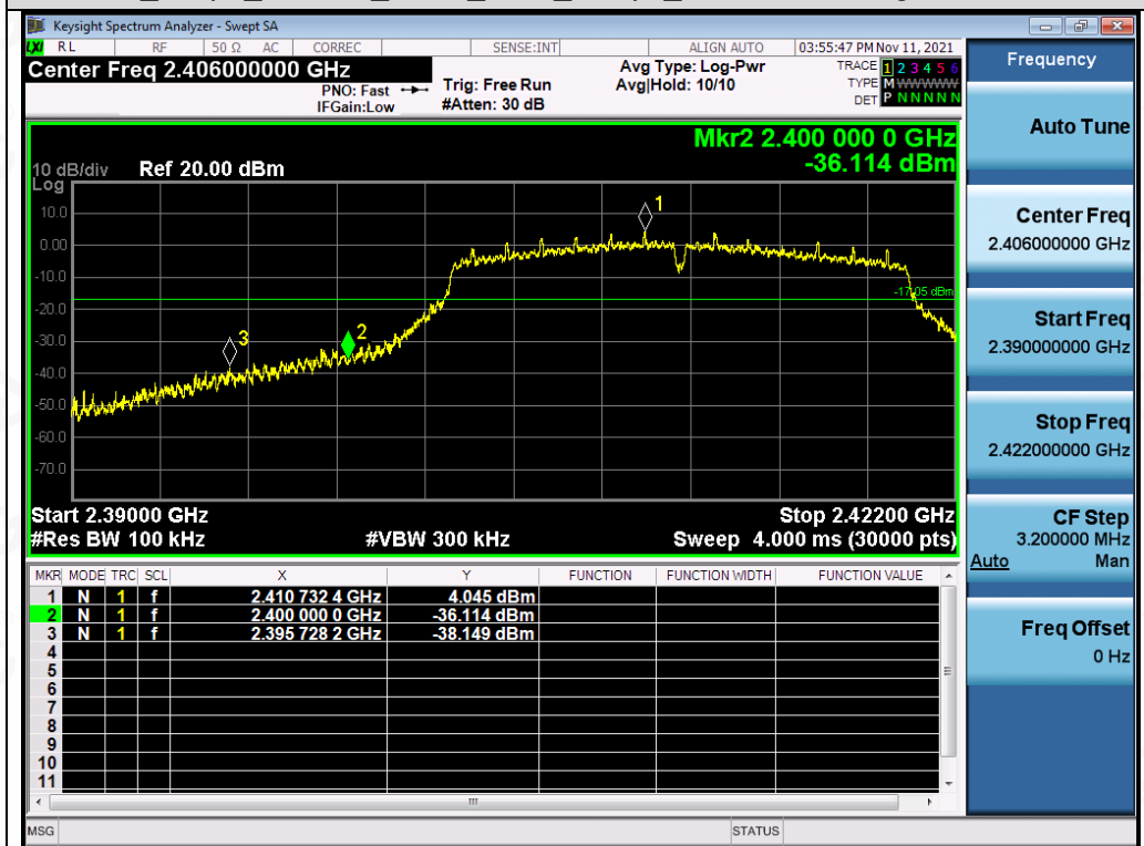
Test_Graph_802.11g_ANT1_2412_6Mbps_Lower Band Edge Emissions
