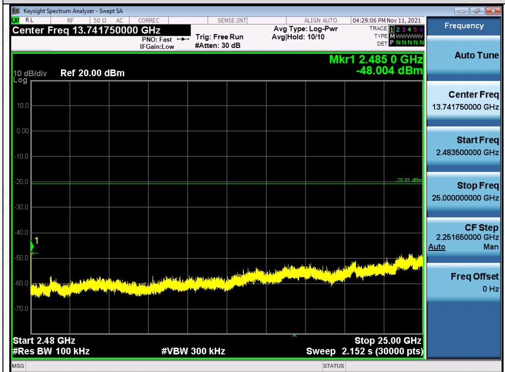
Test_Graph_802.11n40_ANT1_2437_MCS0_Higher Band Emissions
