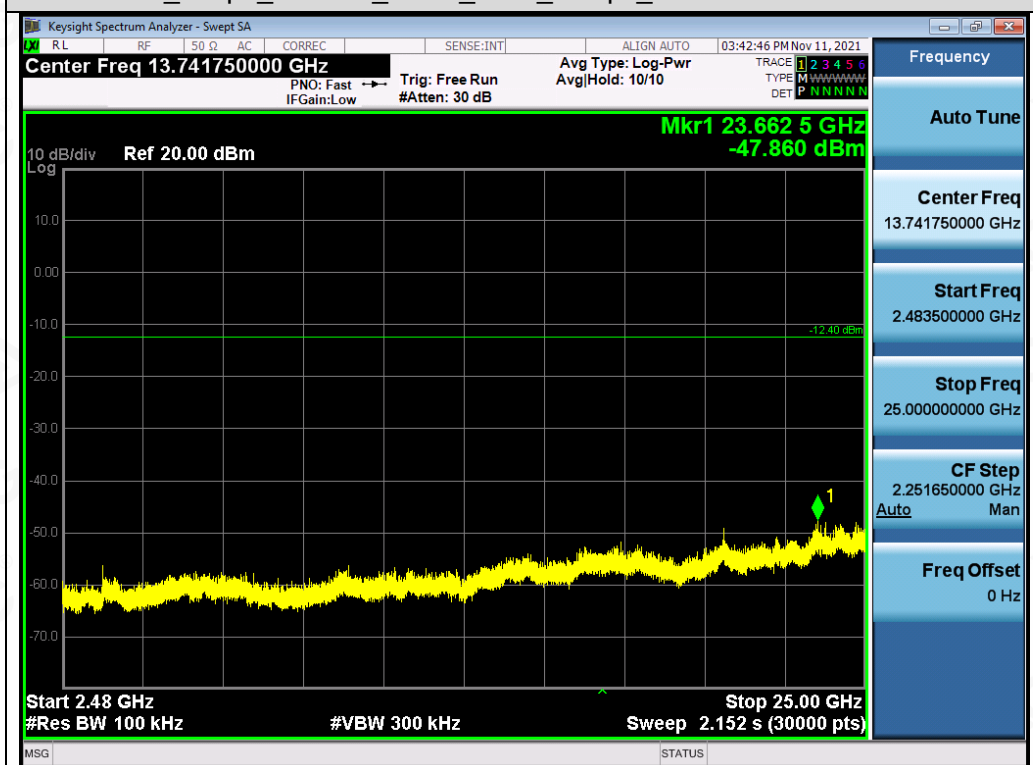
Test_Graph_802.11b_ANT1_2412_1Mbps_Higher Band Emissions
