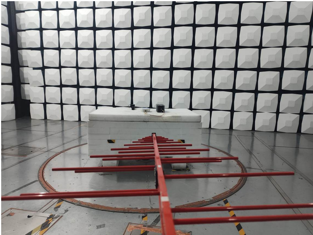
Model: SF006A Radiated Emission Below 1GHz View-Downlink
