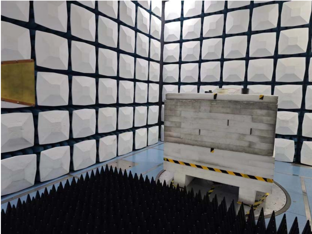
Model: SF006B Radiated Emission Above 1GHz View-Downlink
