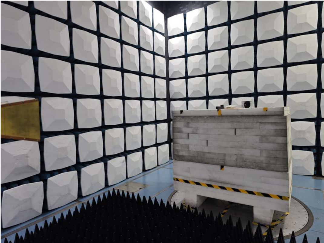
Model: SF006A Radiated Emission Above 1GHz View-Downlink
