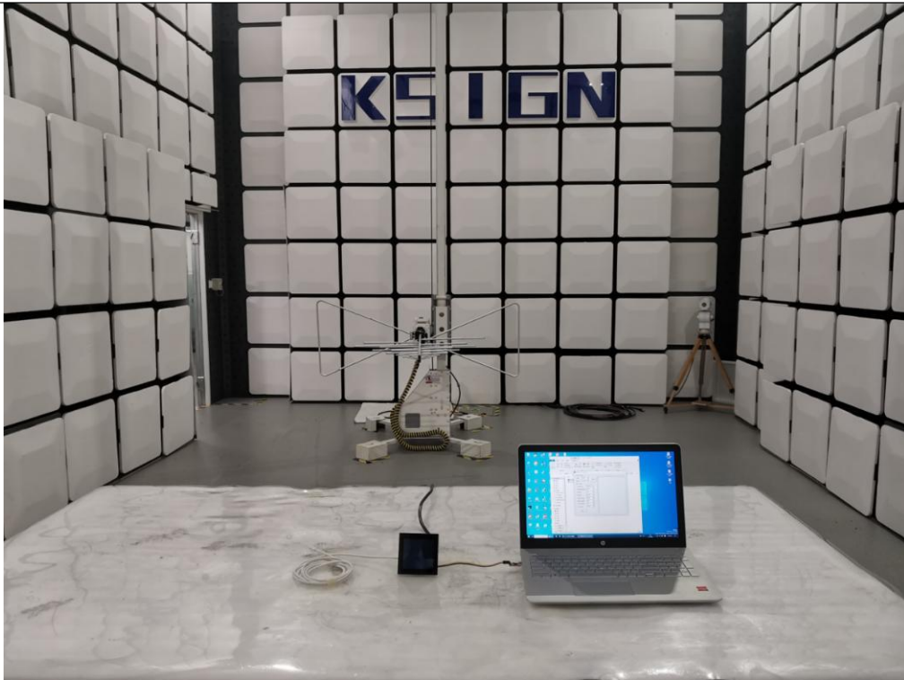
Radiated Measurement (Above 1GHz)
