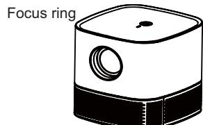
Focus: When the image is blurred (as shown on the right), adjust the focus ring to obtain a satisfactory image imaging effect. If you cannot obtain satisfactory clarity through adjustment, please move the product forward or backward as appropriate.
