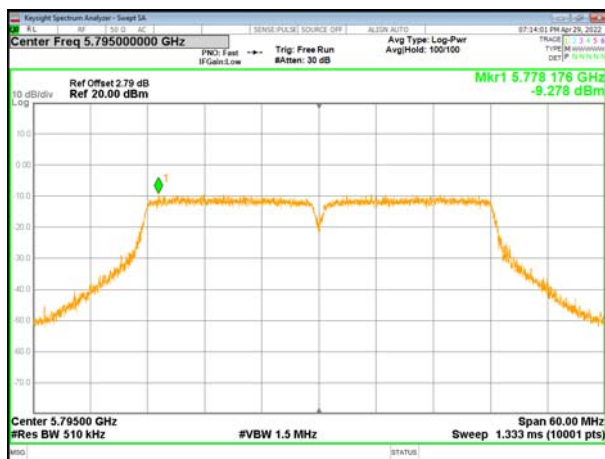
(802.11ac40) PSD plot on channel 159
