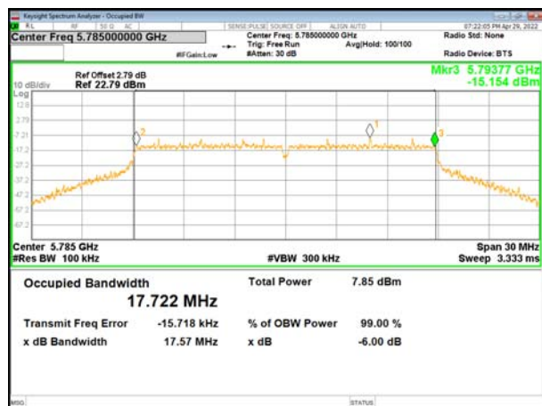
(802.11ac20) plot on channel 165
