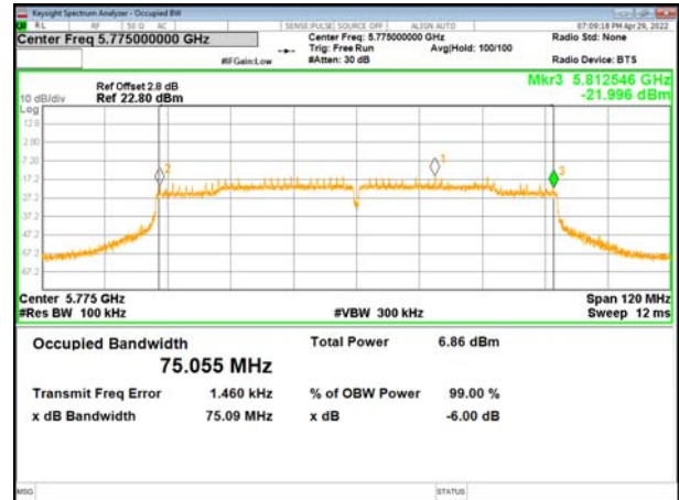
(802.11 ac80) plot on channel 155
