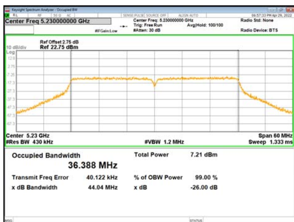
(802.11ac40) plot on channel 46
