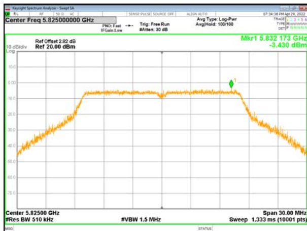
(802.11a) PSD plot on channel 165
