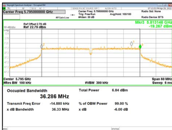
(802.11 ac40) plot on channel 159
