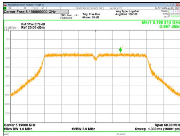
(802.11n40) PSD plot on channel 46
