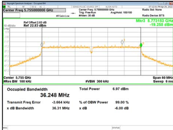
(802.11 ac40) plot on channel 159
