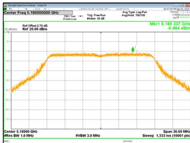
(802.11n20) PSD plot on channel 40
