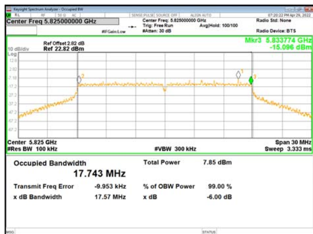
(802.11ac20) plot on channel 165
