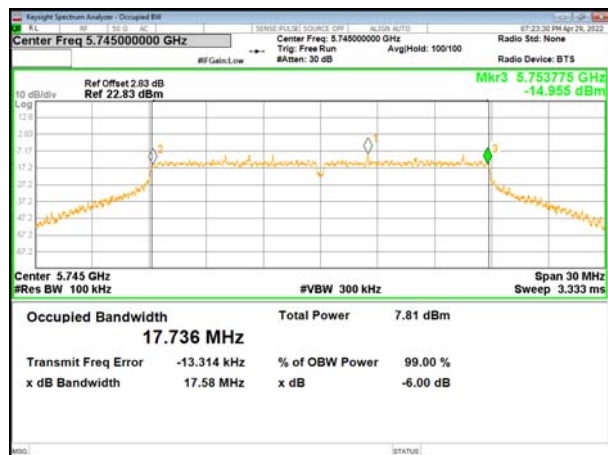
(802.11ac20) plot on channel 157
