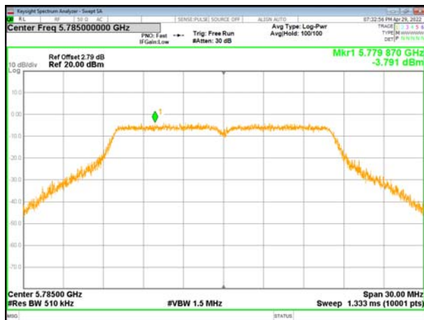
(802.11a) PSD plot on channel 165
