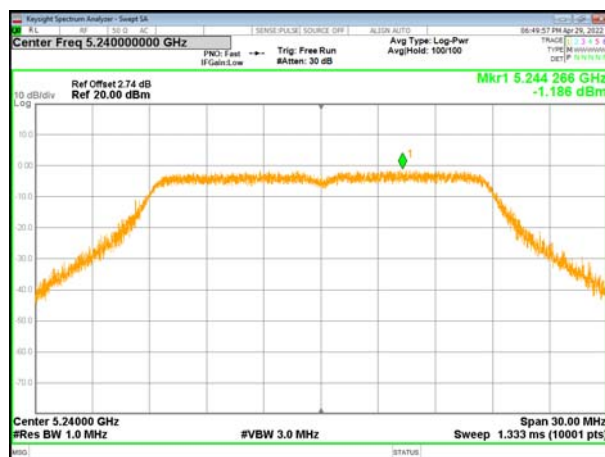
(802.11n20) PSD plot on channel 48
