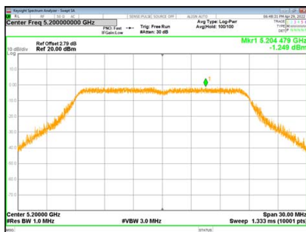
(802.11n20) PSD plot on channel 40
