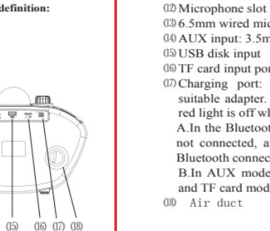
7. Based on the special debugging method of karaoke speakers, in order to have a better low-frequency experience, it is recommended to place the speakers on the desktop against the wall. The sound effect is best when the speaker duct is 5cm away from the wall.
