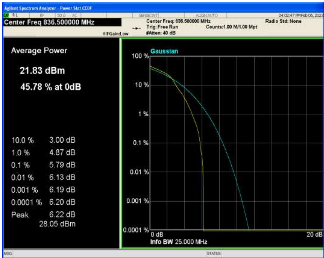
Band5 16QAM BW=1.4MHz Channel=20643 RB Size=1 Position=#0
