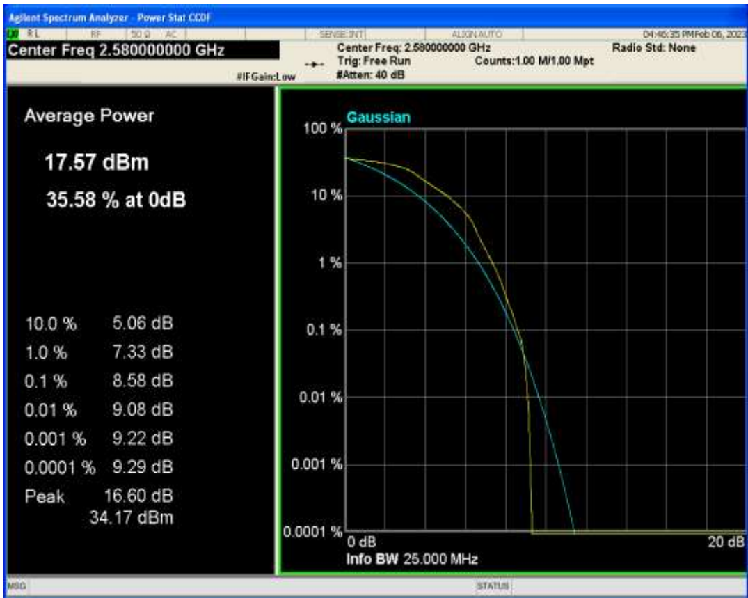
Band38 QPSK BW=20MHz Channel=38000 RB Size=1 Position=#0
