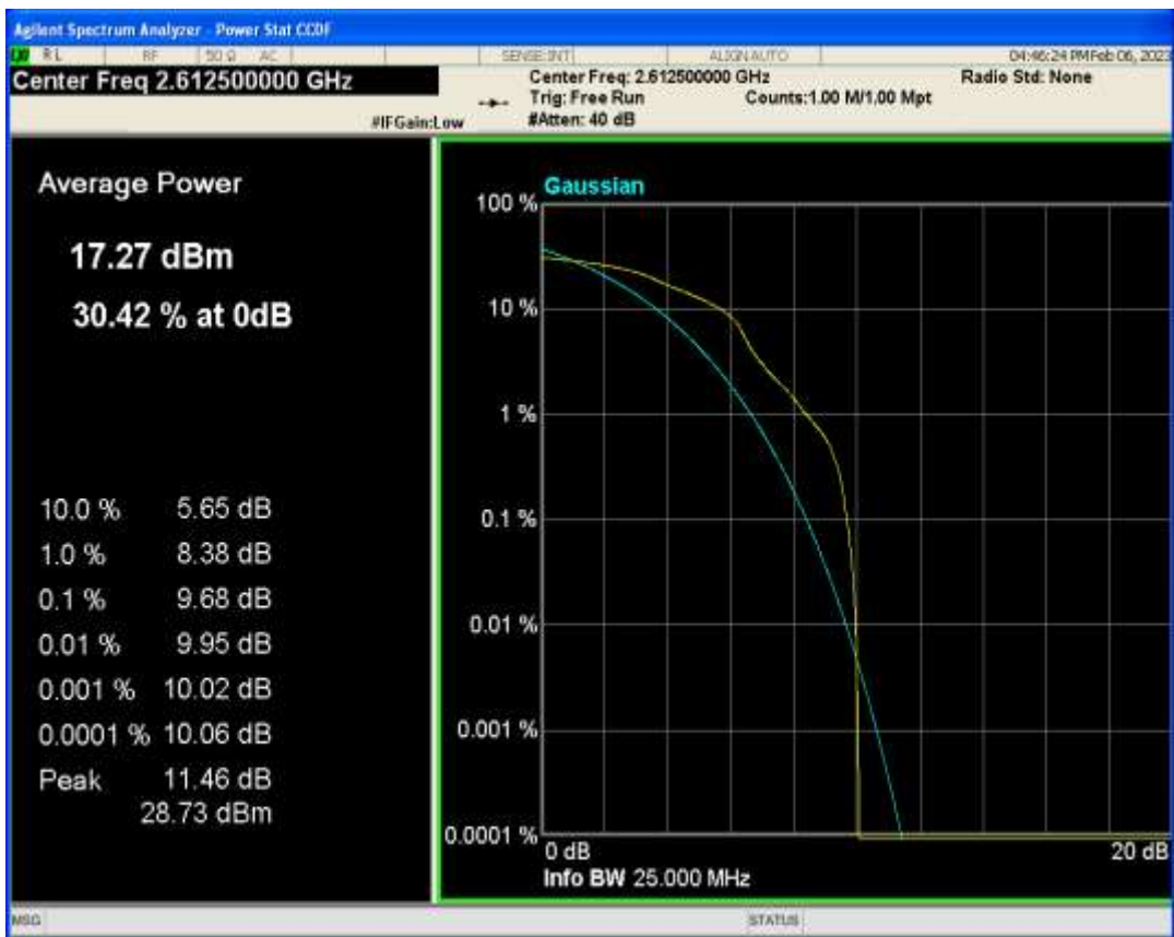
Band38 16QAM BW=20MHz Channel=37850 RB Size=1 Position=#0
