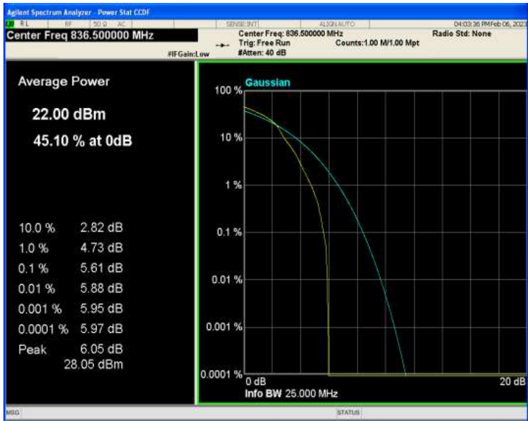
Band5 16QAM BW=5MHz Channel=20625 RB Size=1 Position=#0
