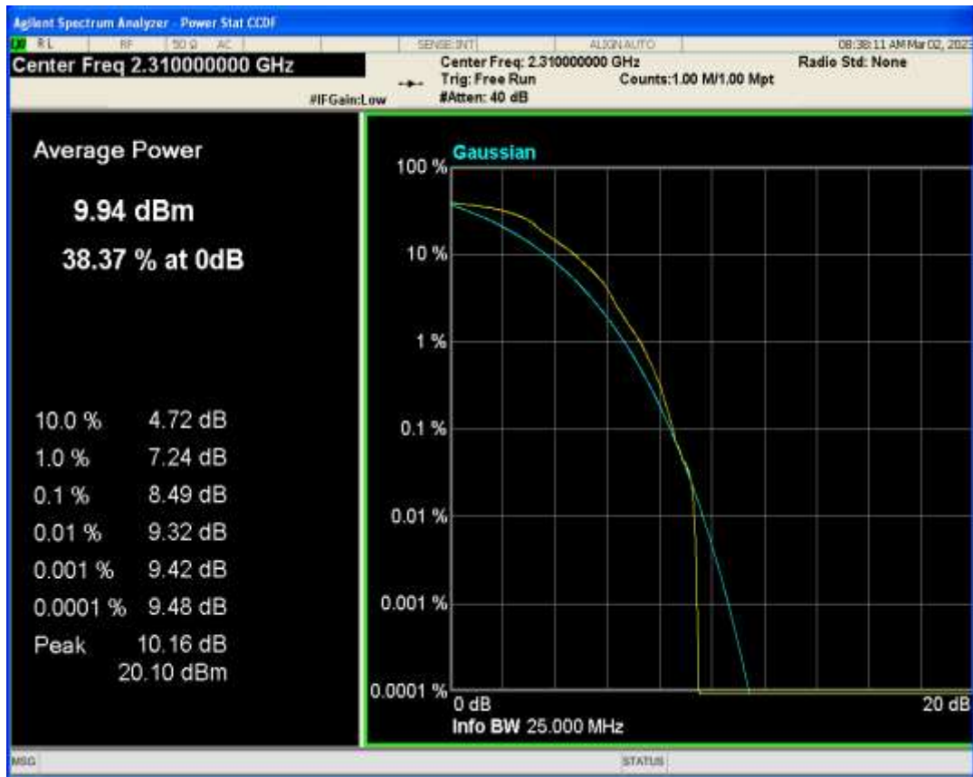
Band40(2305-2315) QPSK BW=5MHz Channel=38775 RB Size=1 Position=#0
