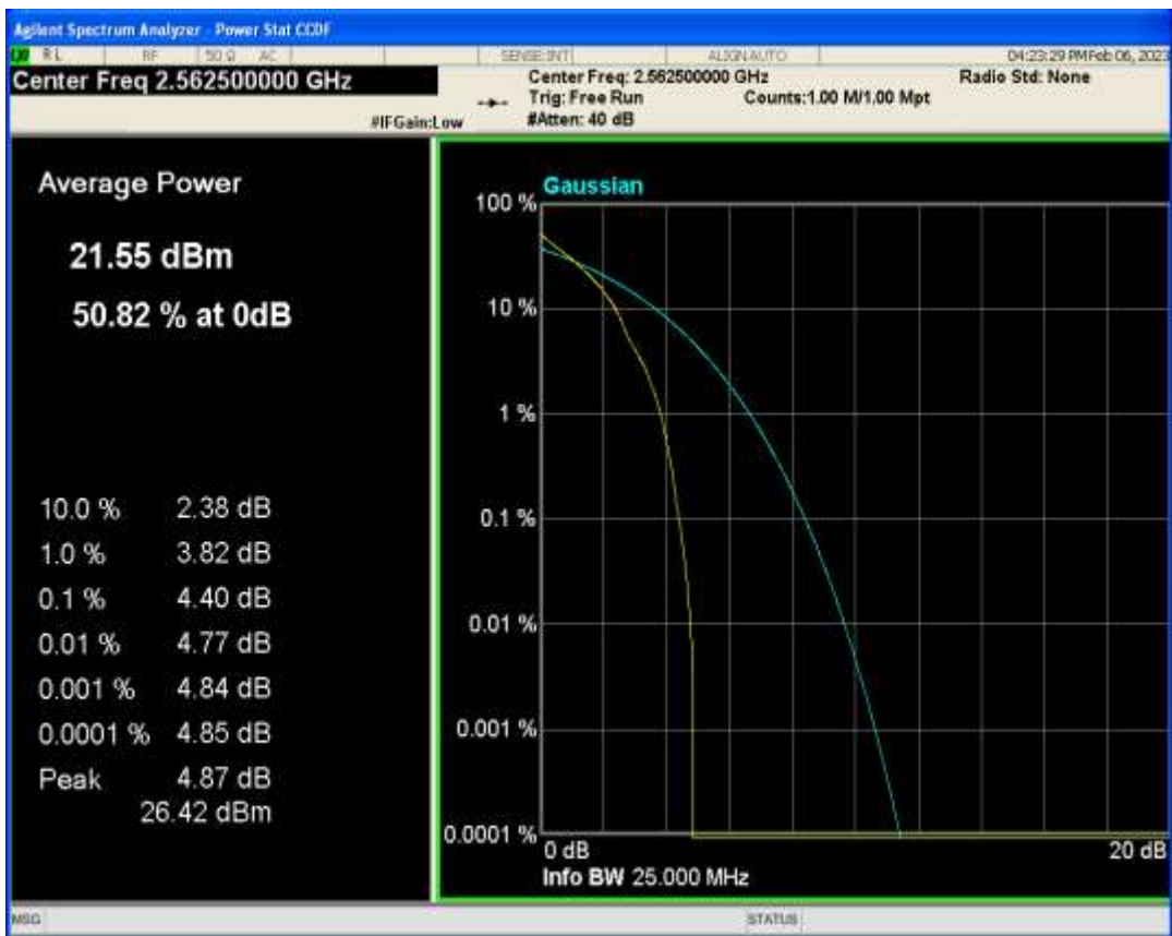
Band7 QPSK BW=20MHz Channel=20850 RB Size=1 Position=#0
