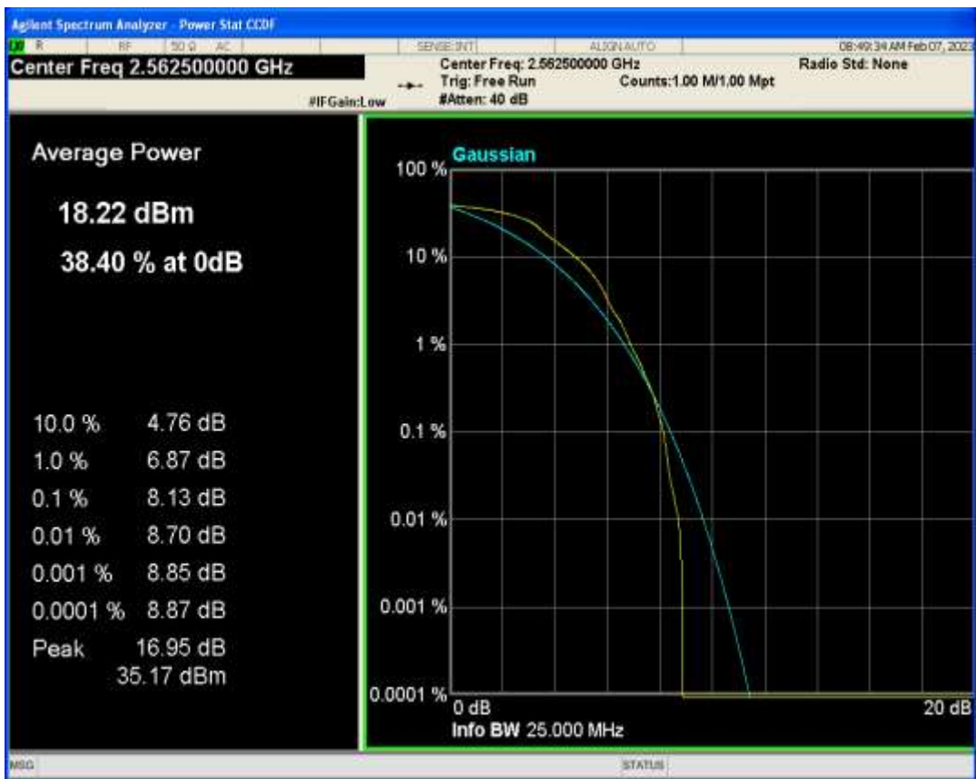
Band41(2555-2655) QPSK BW=15MHz Channel=40740 RB Size=1 Position=#0
