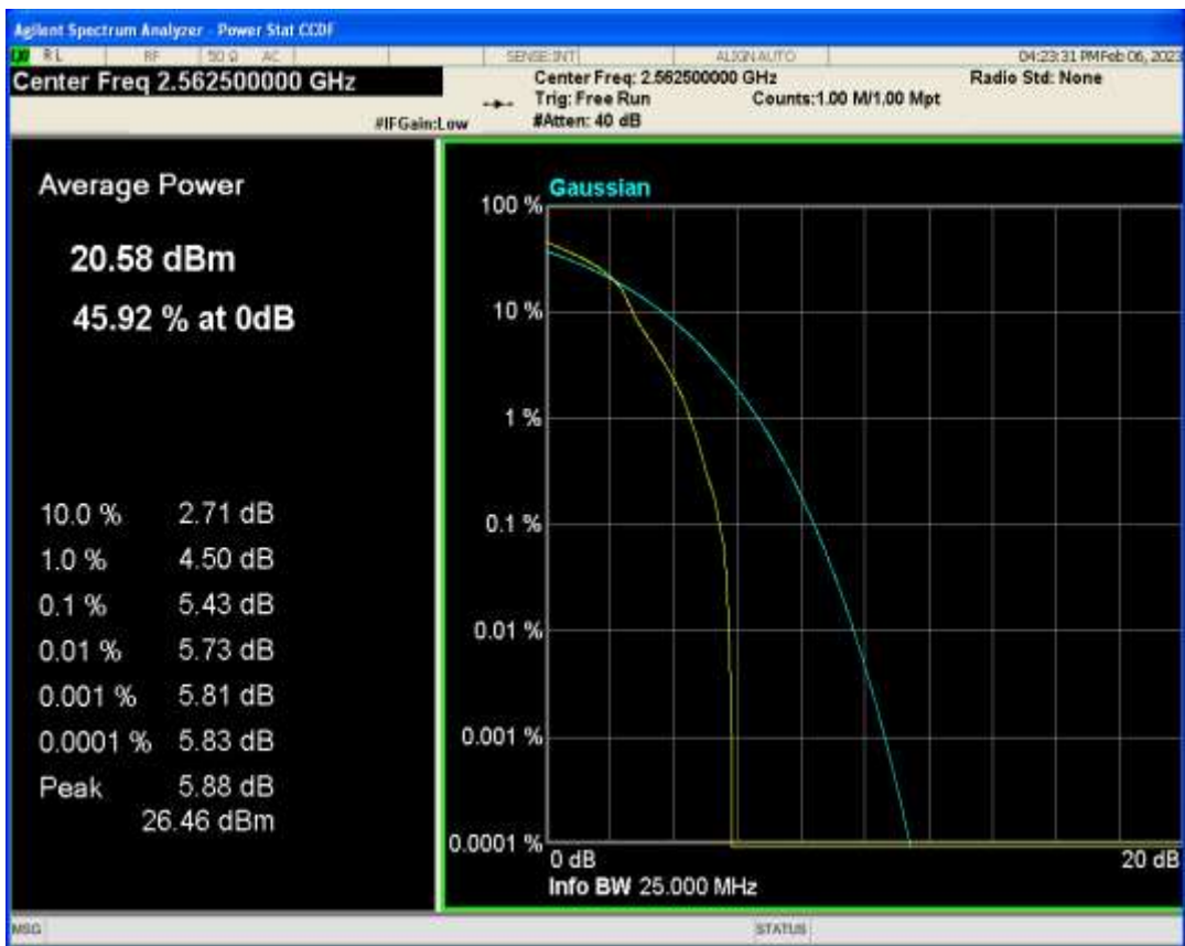
Band7 16QAM BW=20MHz Channel=20850 RB Size=1 Position=#0
