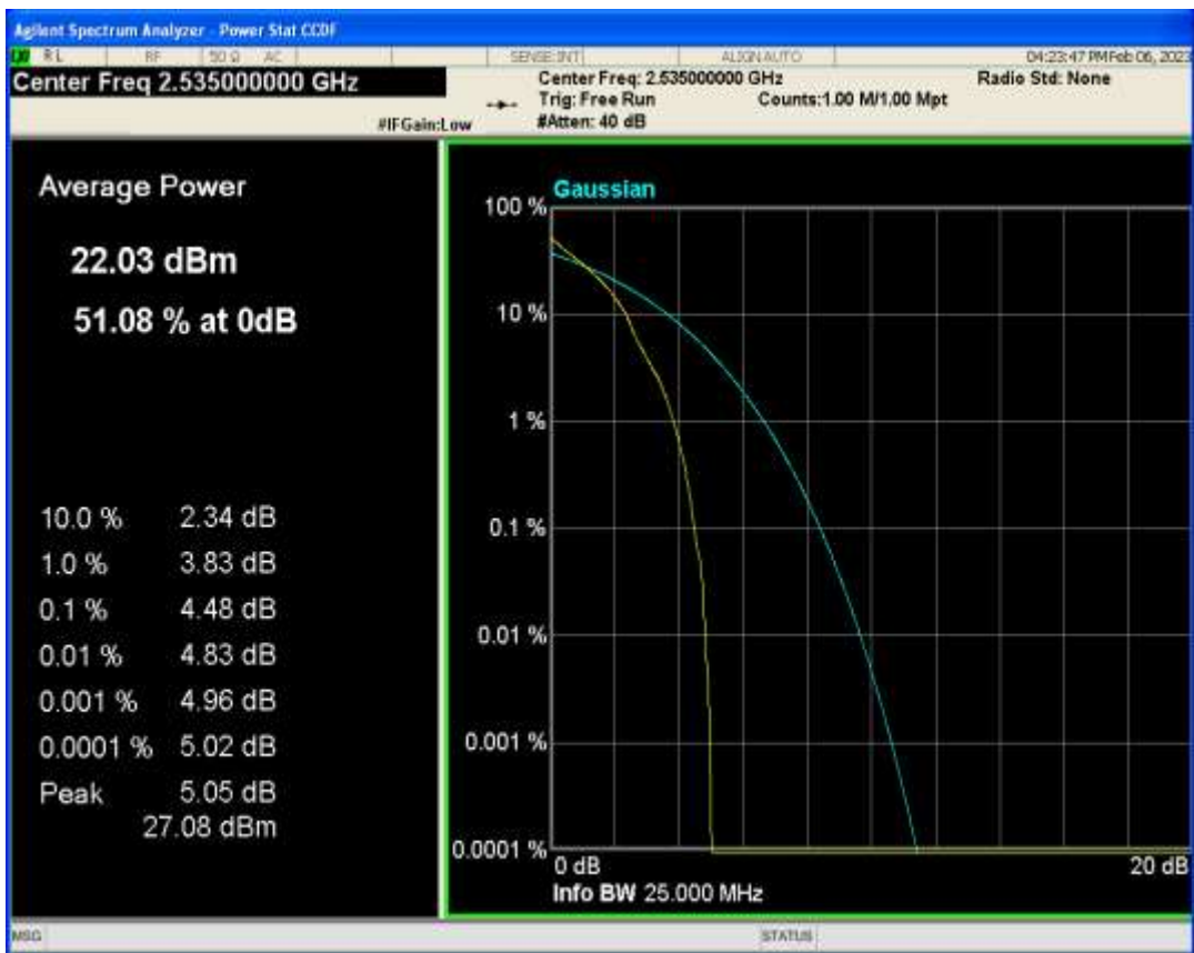
Band7 QPSK BW=20MHz Channel=21350 RB Size=1 Position=#0
