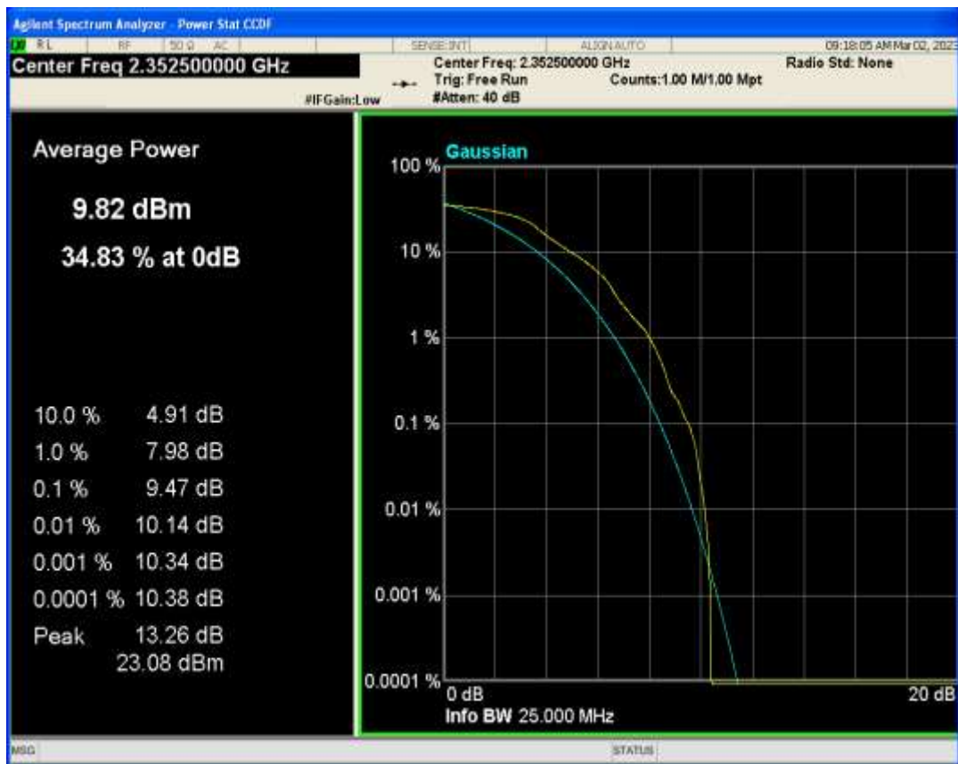
Band40(2350-2360) QPSK BW=5MHz Channel=39200 RB Size=1 Position=#0
