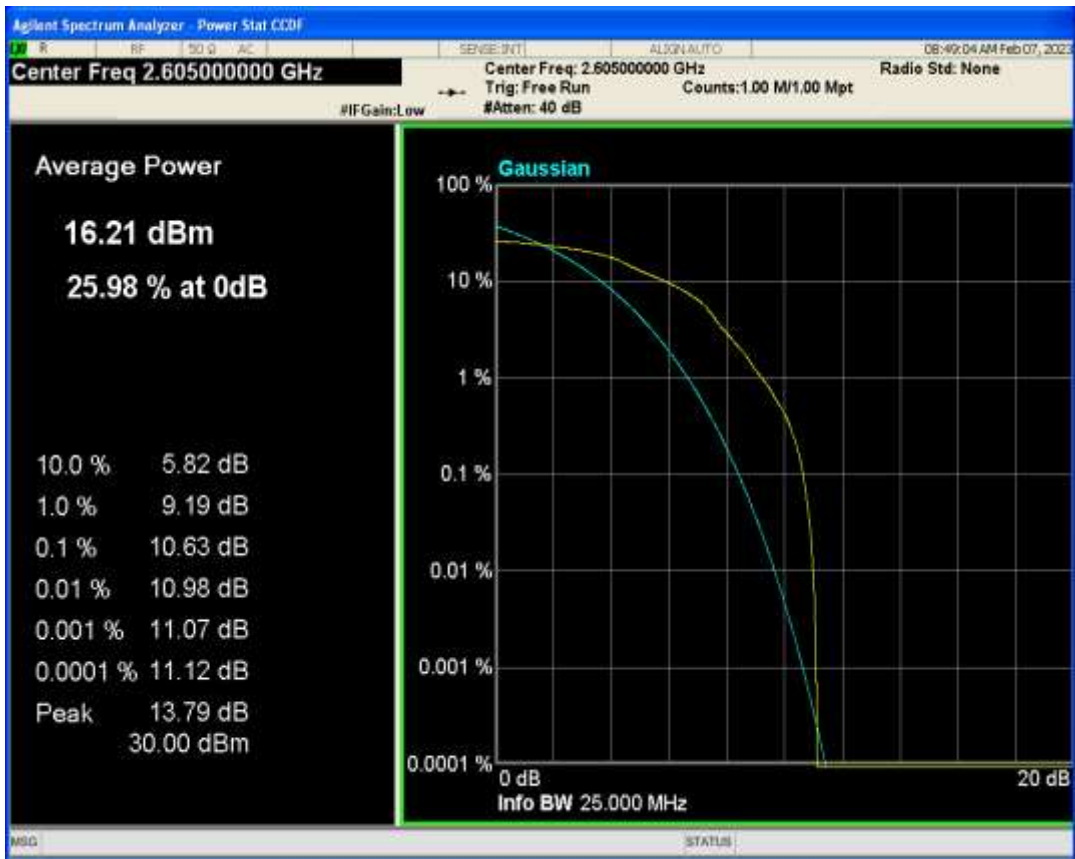
Band41(2555-2655) 16QAM BW=5MHz Channel=41215 RB Size=1 Position=#0
