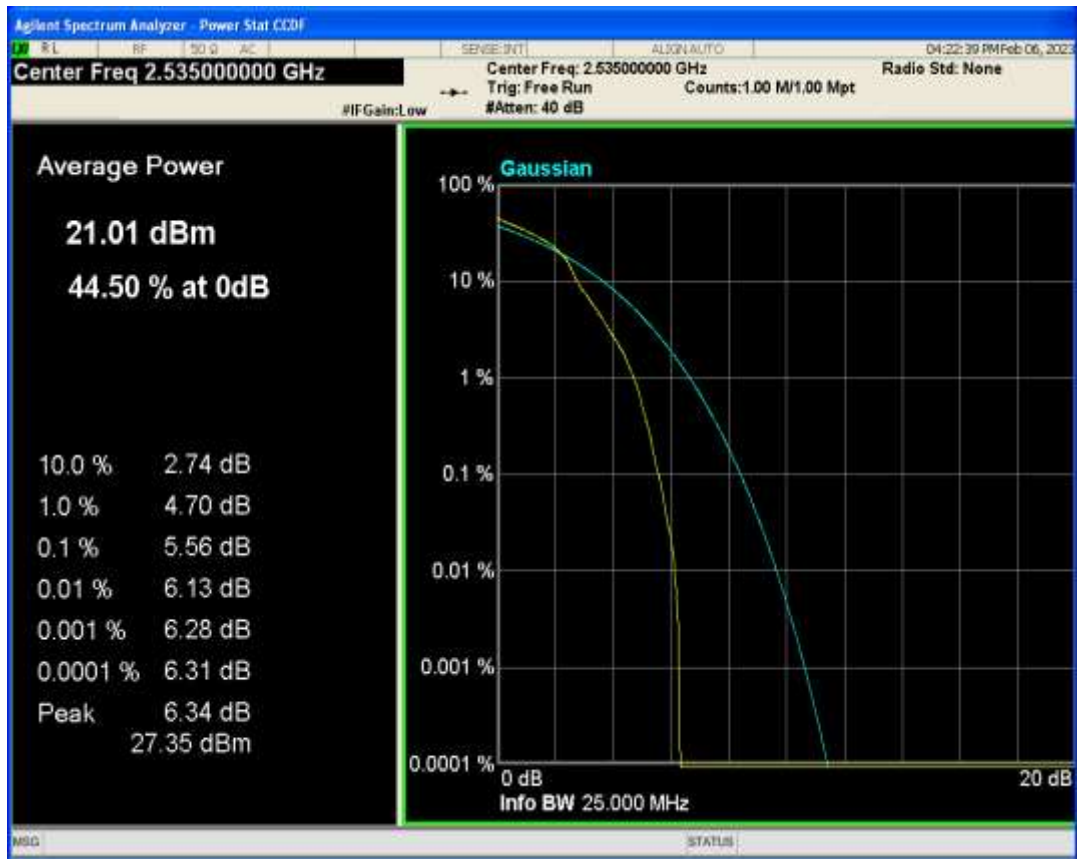
Band7 16QAM BW=5MHz Channel=21425 RB Size=1 Position=#0
