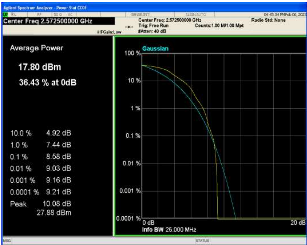
Band38 QPSK BW=5MHz Channel=38000 RB Size=1 Position=#0
