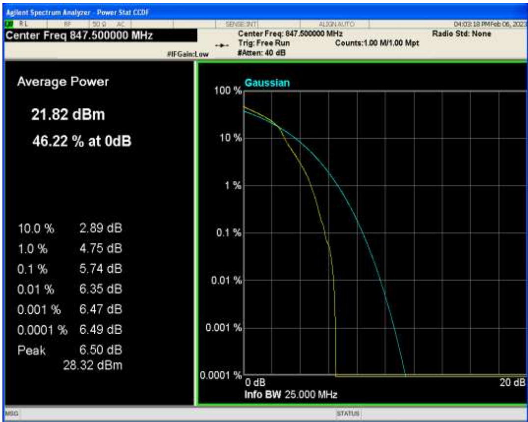
Band5 16QAM BW=5MHz Channel=20425 RB Size=1 Position=#0
