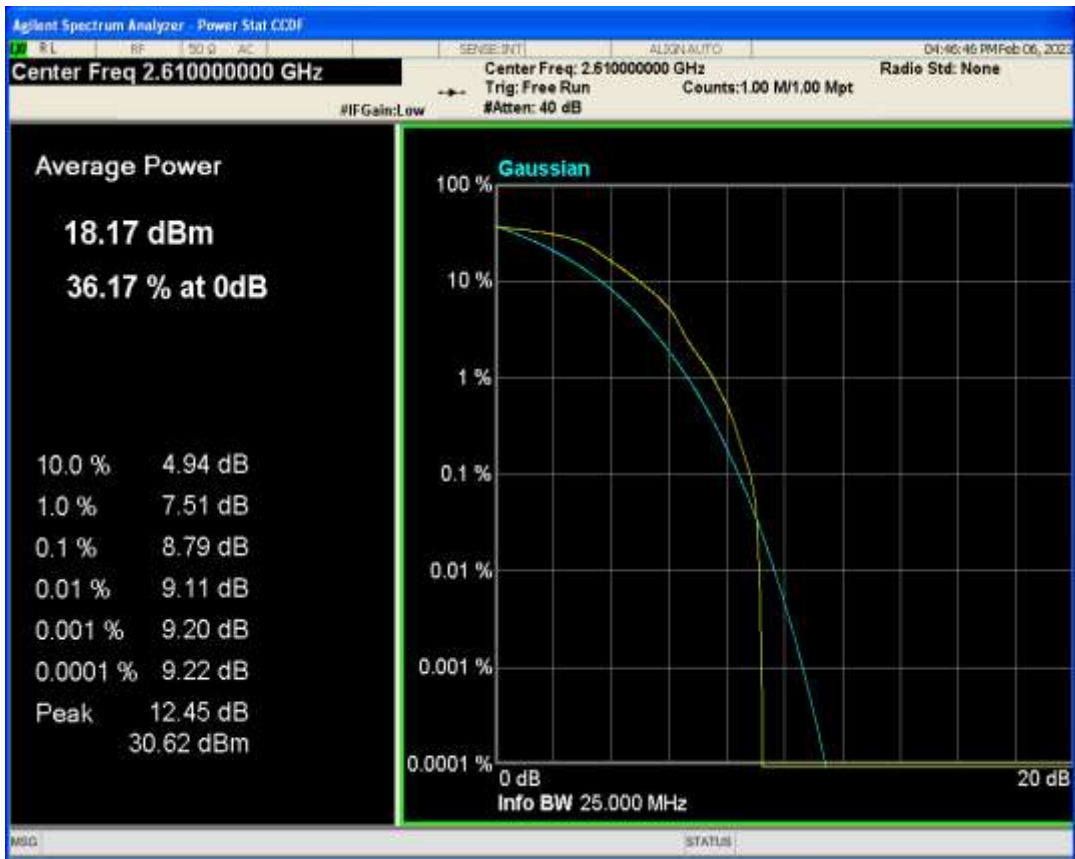
Band38 QPSK BW=5MHz Channel=37775 RB Size=1 Position=#0
