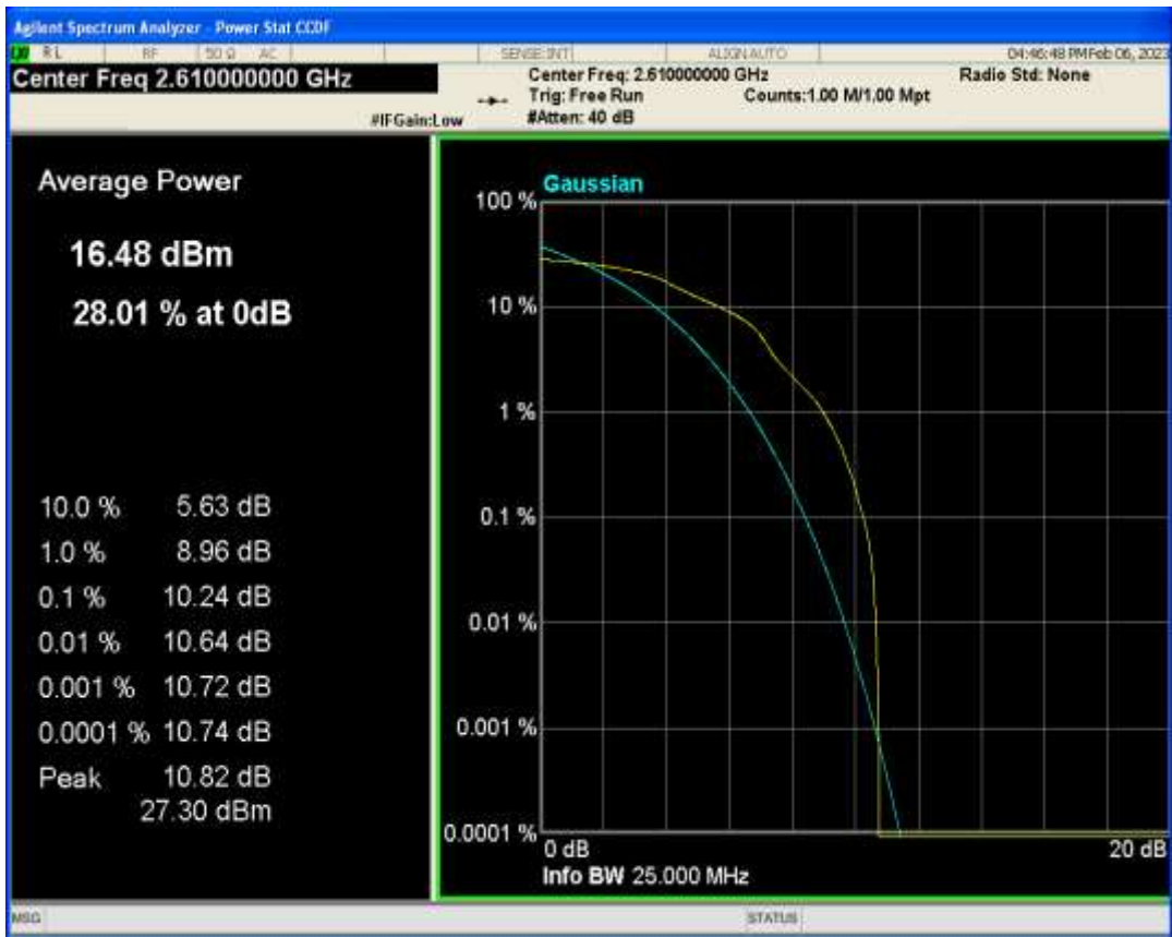
Band38 16QAM BW=5MHz Channel=37775 RB Size=1 Position=#0
