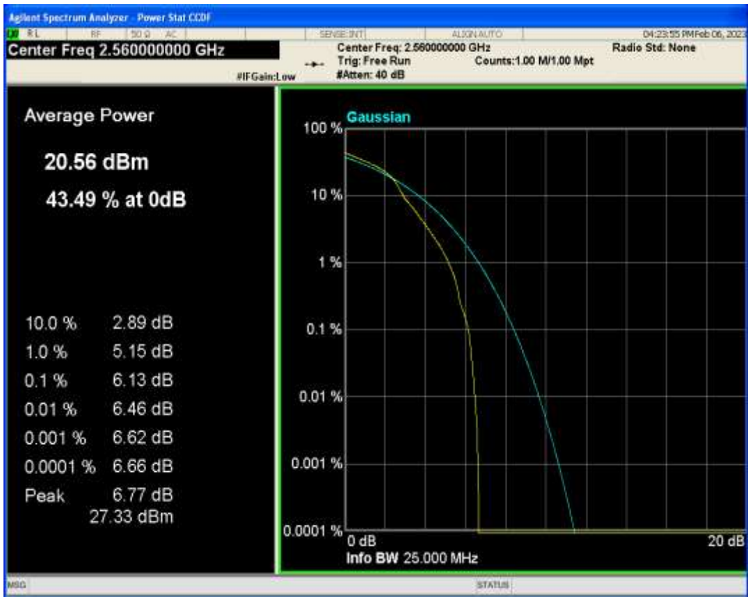
Band7 16QAM BW=5MHz Channel=20775 RB Size=1 Position=#0
