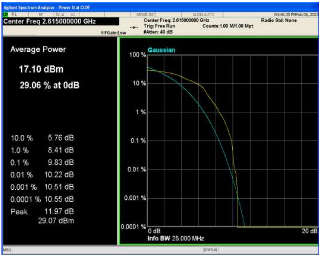
Band38 16QAM BW=15MHz Channel=37825 RB Size=1 Position=#0
