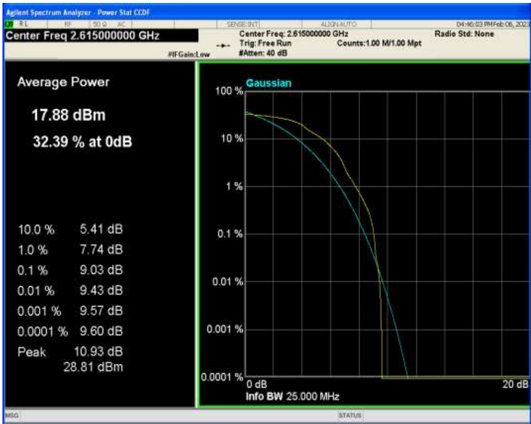
Band38 QPSK BW=15MHz Channel=37825 RB Size=1 Position=#0
