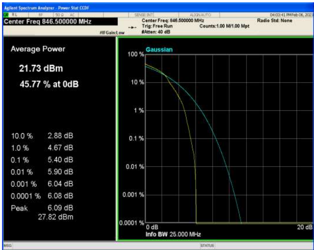
Band5 QPSK BW=1.4MHz Channel=20407 RB Size=1 Position=#0
