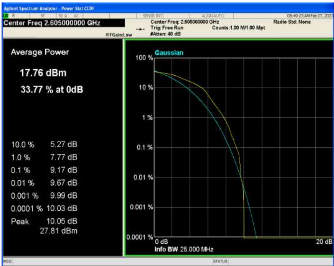
Band41(2555-2655) 16QAM BW=10MHz Channel=41190 RB Size=1 Position=#0
