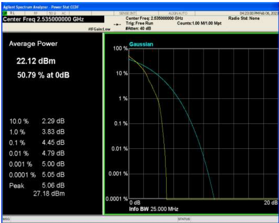
Band7 QPSK BW=10MHz Channel=21400 RB Size=1 Position=#0
