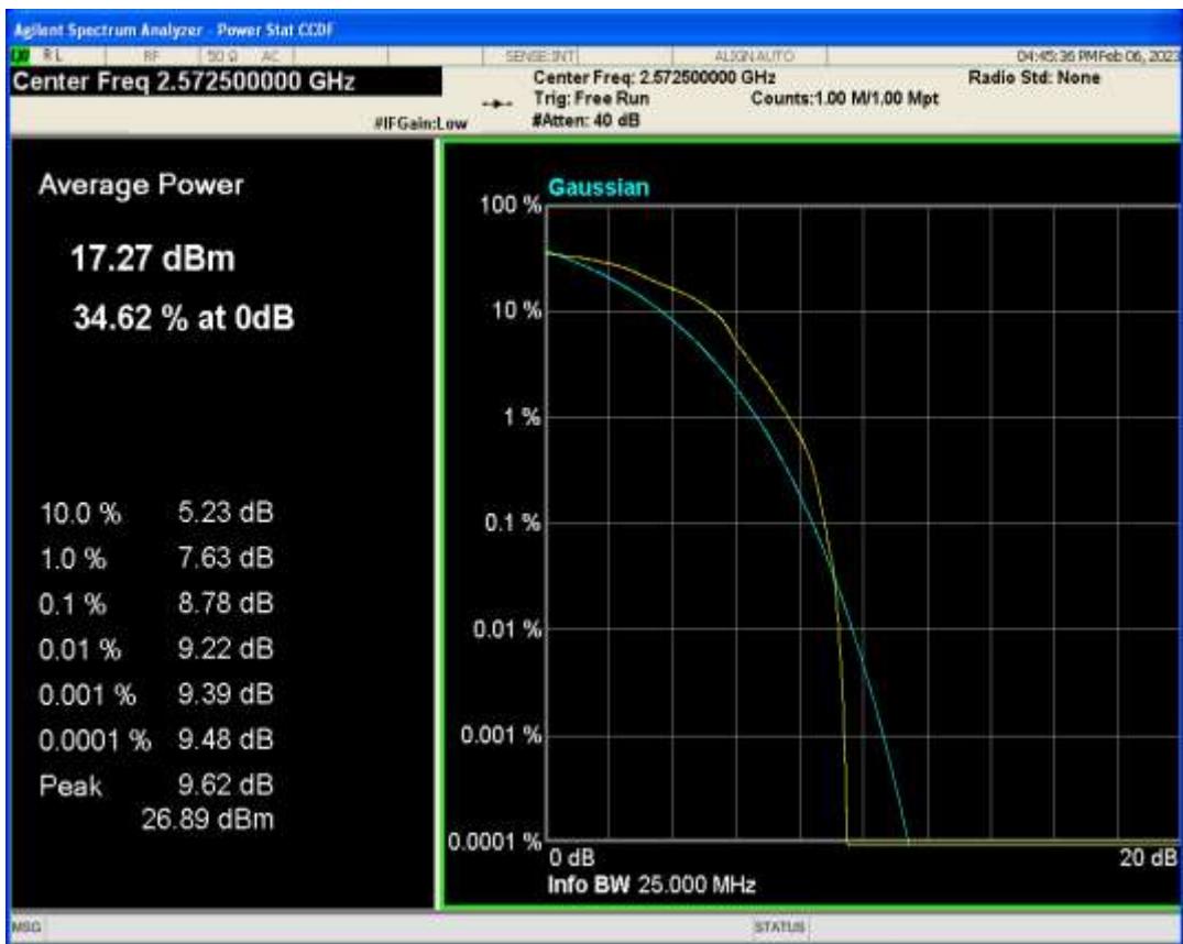
Band38 16QAM BW=5MHz Channel=38000 RB Size=1 Position=#0
