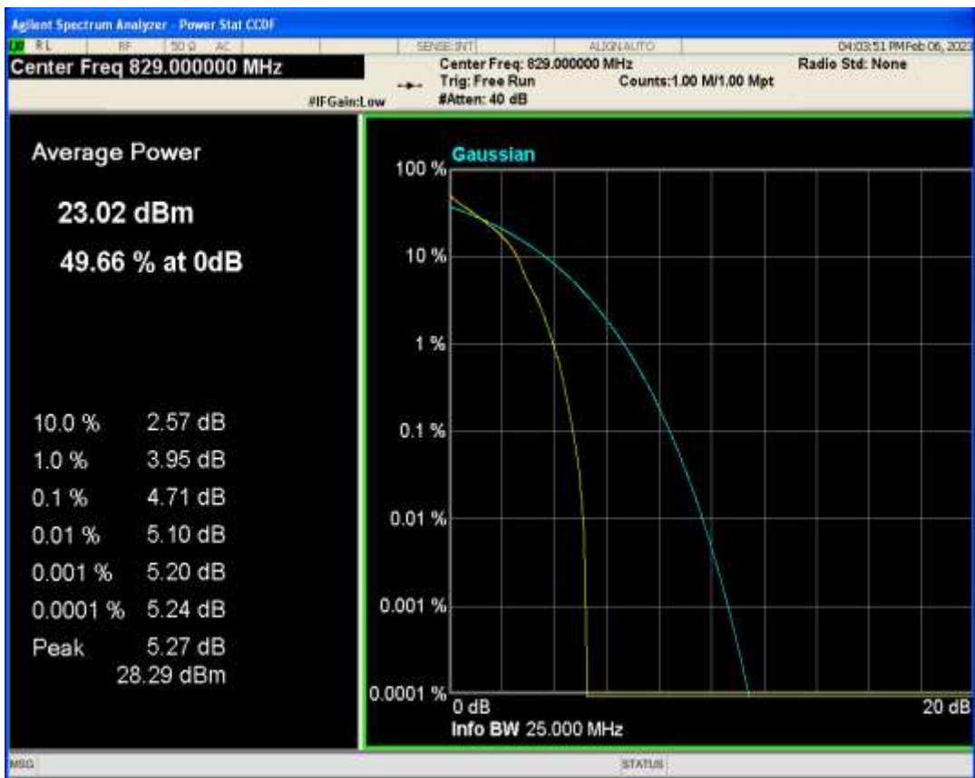
Band5 QPSK BW=10MHz Channel=20525 RB Size=1 Position=#0
