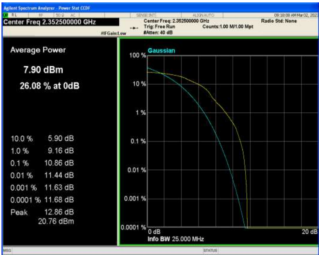
Band40(2350-2360) 16QAM BW=5MHz Channel=39200 RB Size=1 Position=#0
