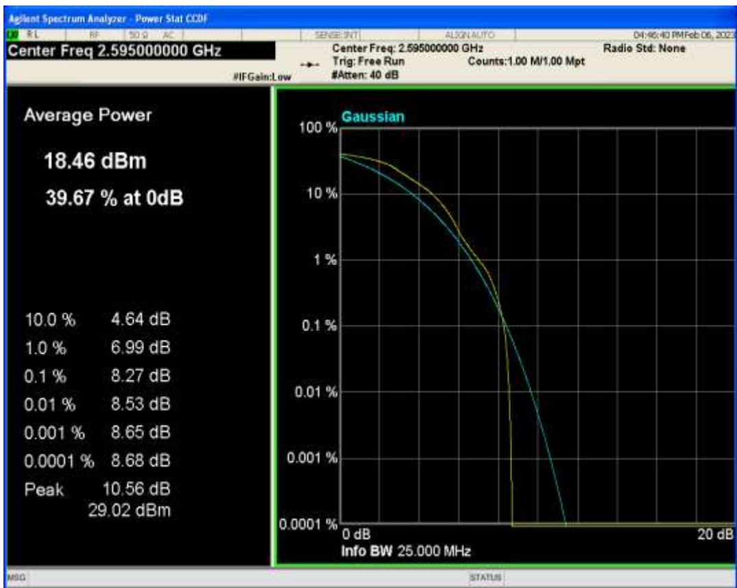
Band38 QPSK BW=20MHz Channel=38150 RB Size=1 Position=#0
