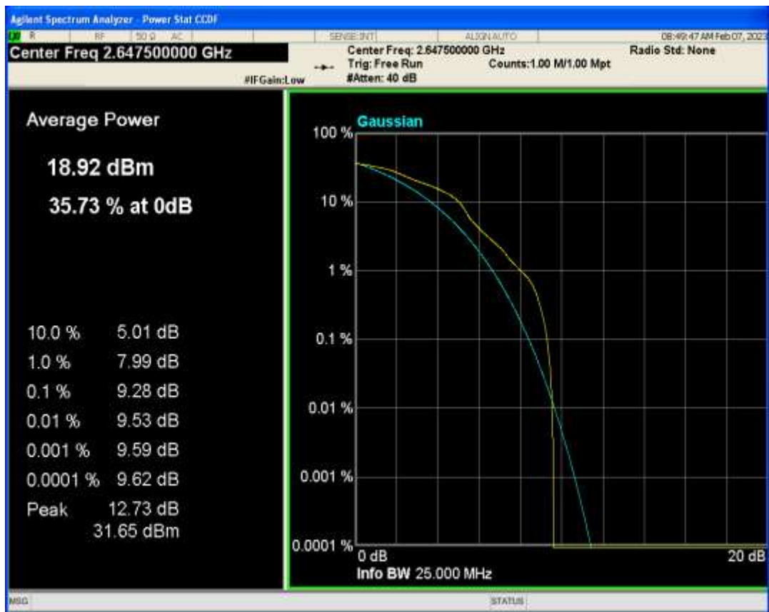
Band41(2555-2655) 16QAM BW=20MHz Channel=40340 RB Size=1 Position=#0
