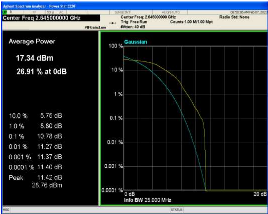
Band41(2555-2655) QPSK BW=5MHz Channel=40265 RB Size=1 Position=#0
