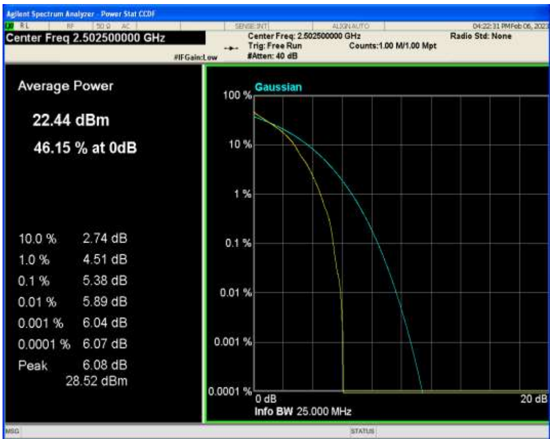
Band7 QPSK BW=5MHz Channel=21100 RB Size=1 Position=#0
