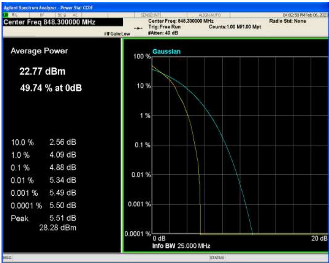
Band5 QPSK BW=10MHz Channel=20450 RB Size=1 Position=#0
