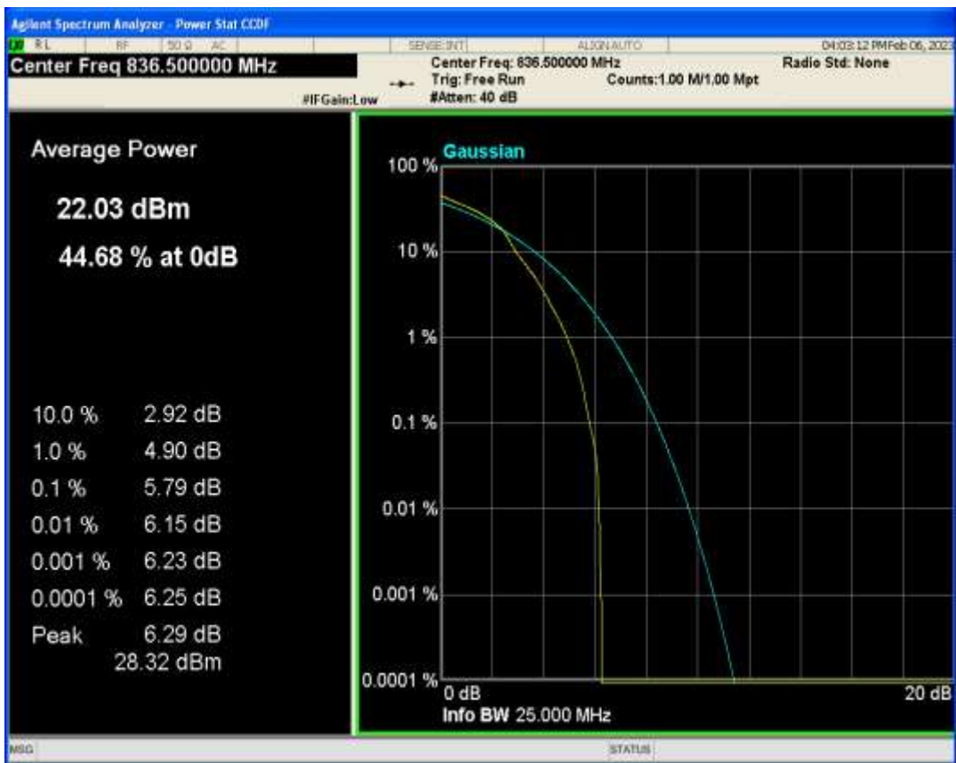
Band5 16QAM BW=3MHz Channel=20635 RB Size=1 Position=#0
