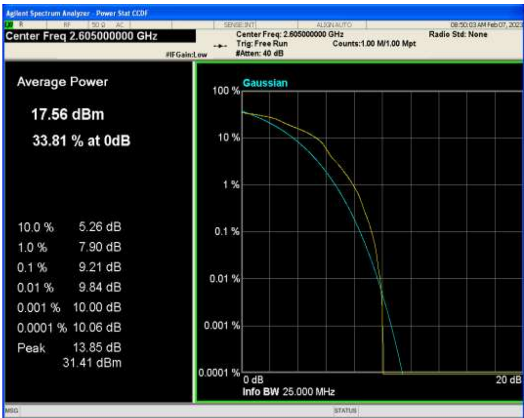
Band41(2555-2655) 16QAM BW=20MHz Channel=41140 RB Size=1 Position=#0
