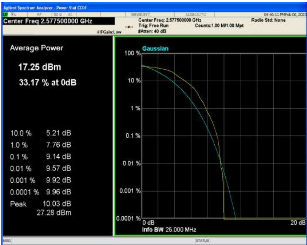
Band38 QPSK BW=15MHz Channel=38000 RB Size=1 Position=#0
