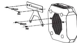
1. Locate the VESA mount screw holes on the back of the Mini PC. They are located near the middle of the device.
