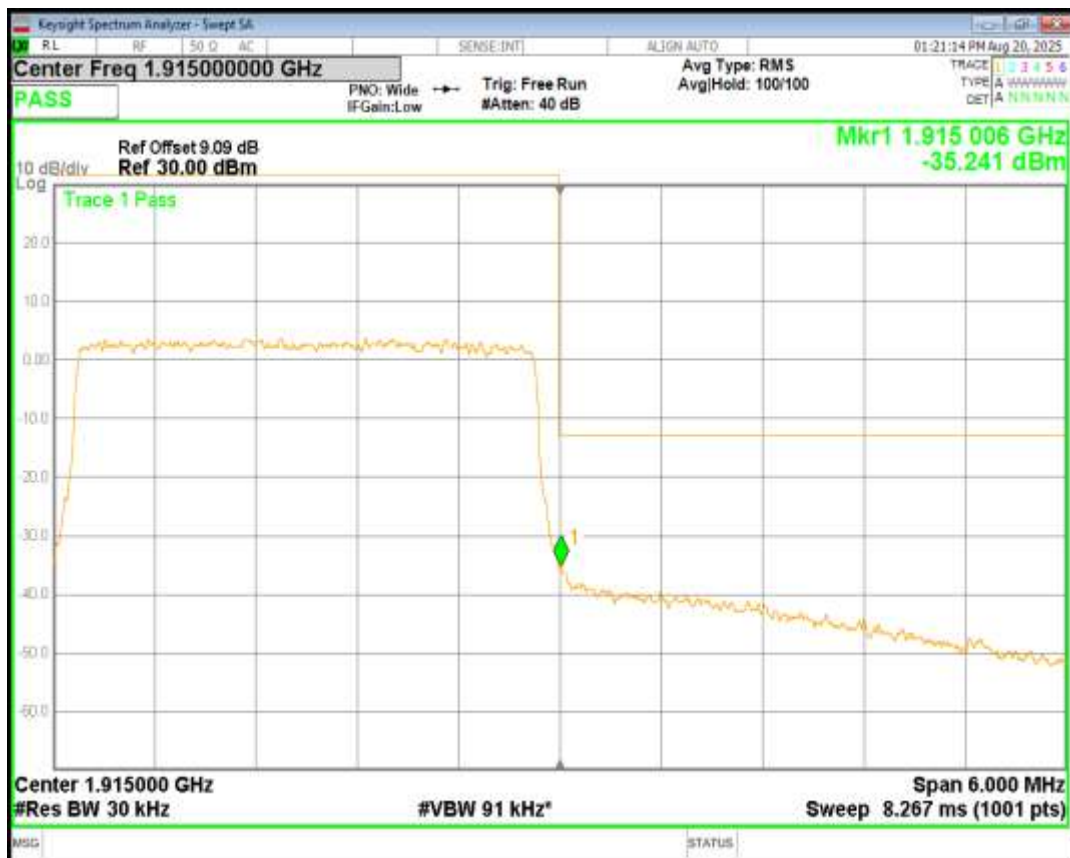
Band25 QPSK BW=5MHz Channel=26065 RB Size=25 Position=#0
