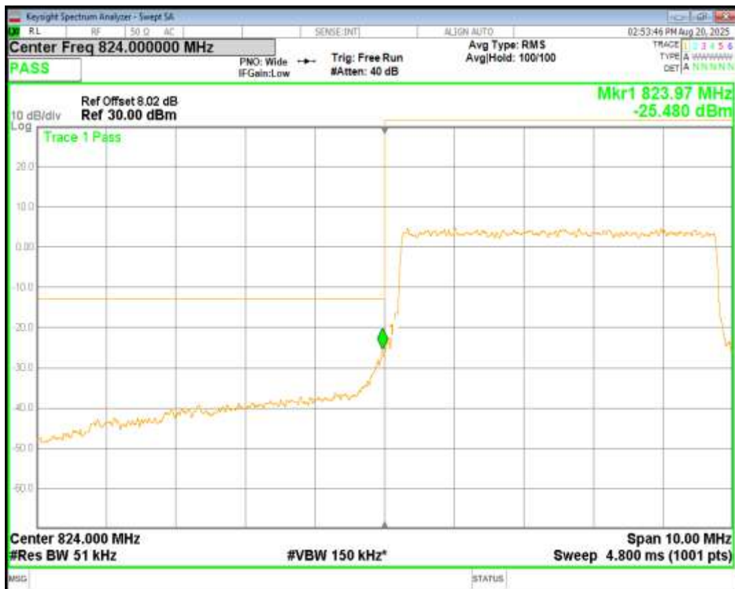
Band26(824-849) QPSK BW=5MHz Channel=27015 RB Size=25 Position=#0
