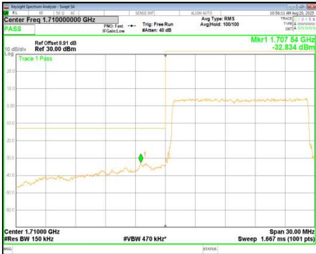
Band4 16QAM BW=15MHz Channel=20025 RB Size=75 Position=#0
