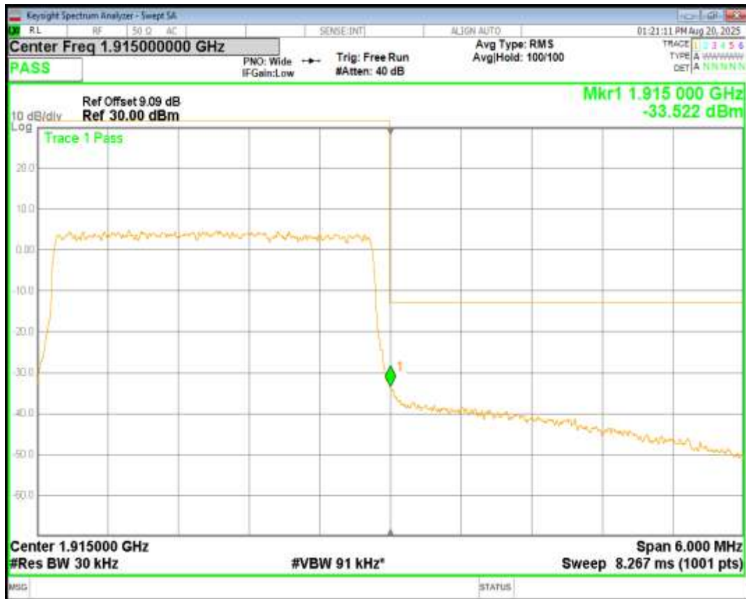
Band25 16QAM BW=3MHz Channel=26675 RB Size=15 Position=#0
