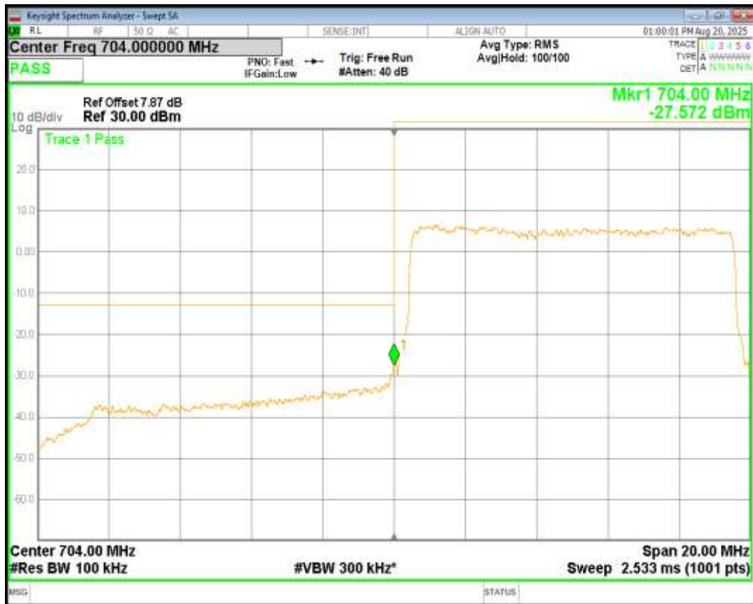
Band17 16QAM BW=10MHz Channel=23780 RB Size=50 Position=#0
