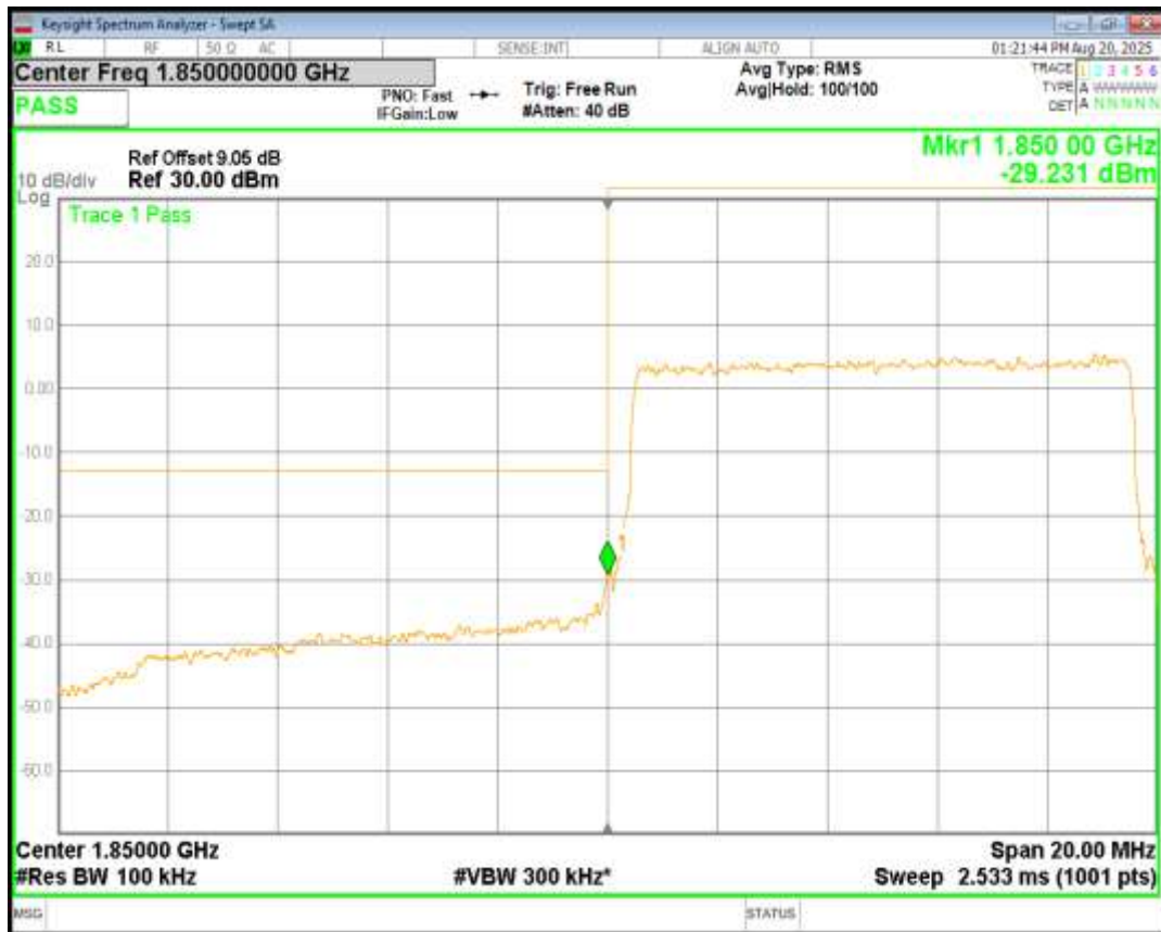
Band25 16QAM BW=10MHz Channel=26090 RB Size=50 Position=#0
