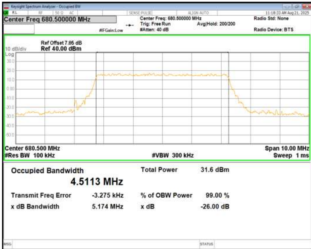
Band71 16QAM BW=5MHz Channel=133297 RB Size=25 Position=#0
