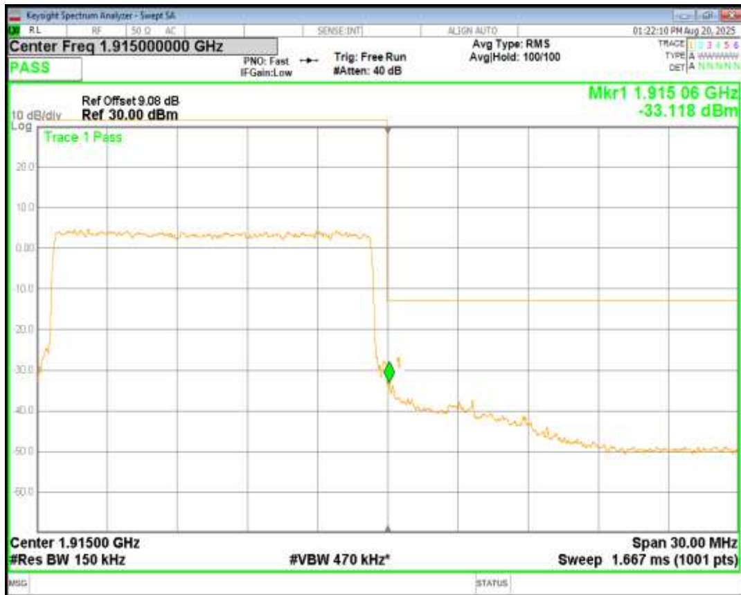
Band25 16QAM BW=15MHz Channel=26615 RB Size=75 Position=#0
