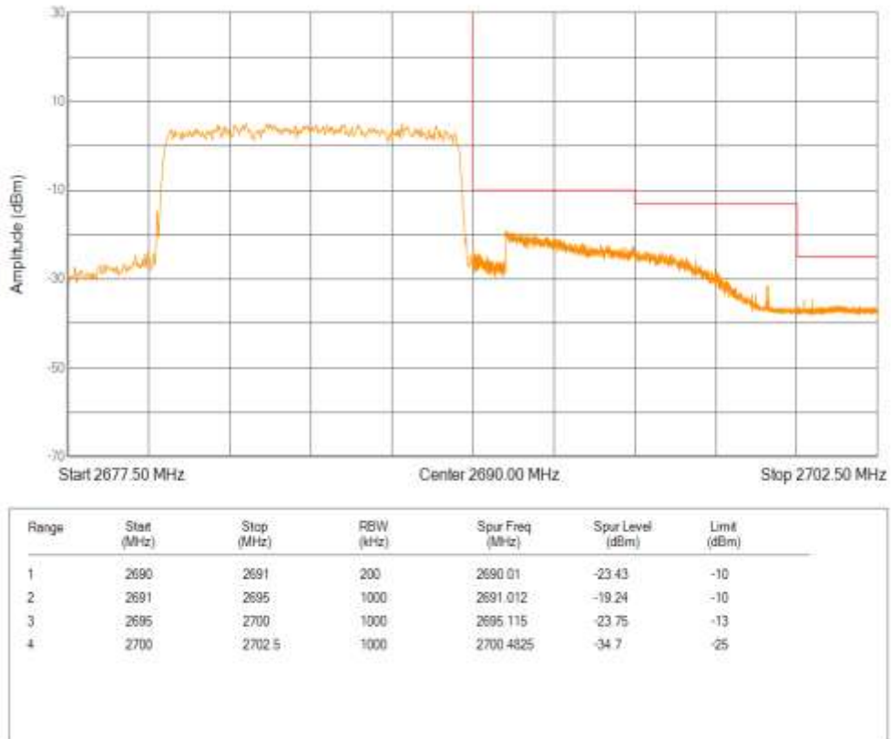
Band41 16QAM BW=10MHz Channel=41540 RB Size=50 Position=#0
