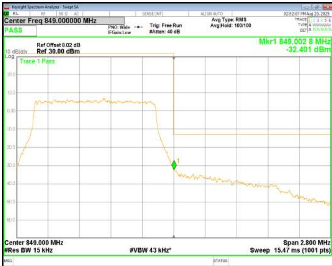
Band26(824-849) 16QAM BW=1.4MHz Channel=27033 RB Size=6 Position=#0
