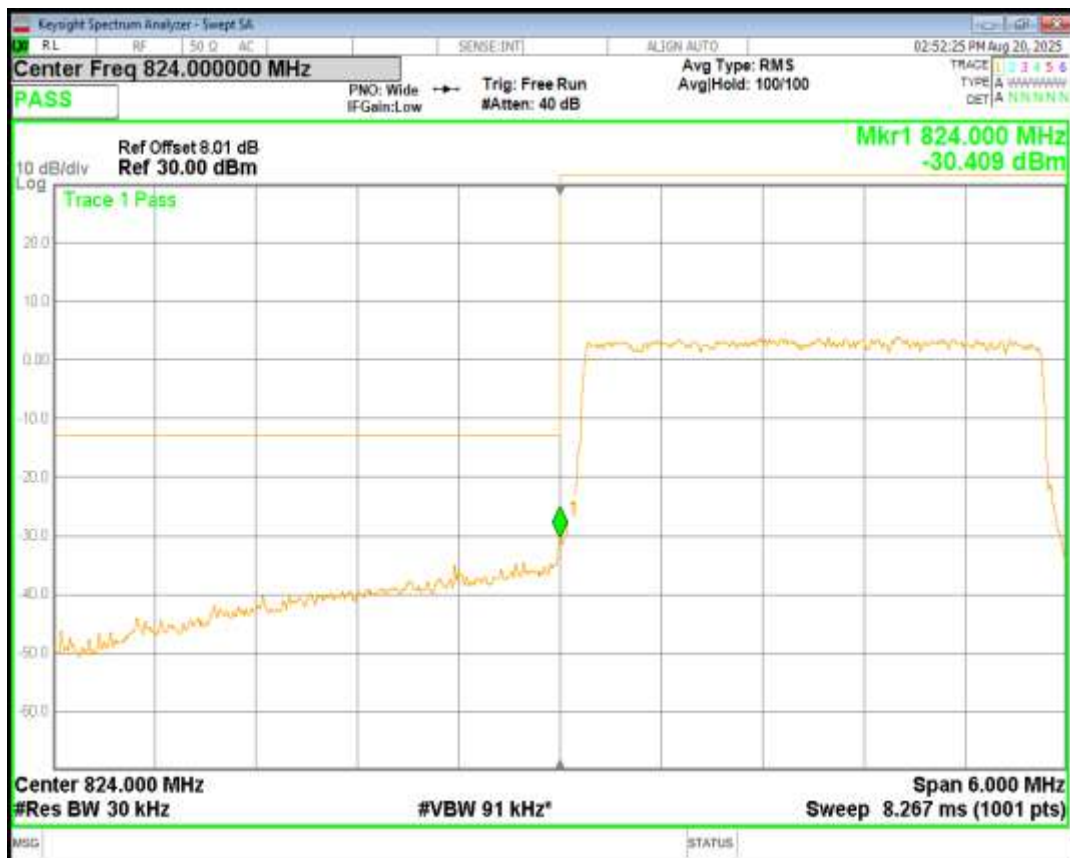
Band26(824-849) QPSK BW=3MHz Channel=27025 RB Size=15 Position=#0
