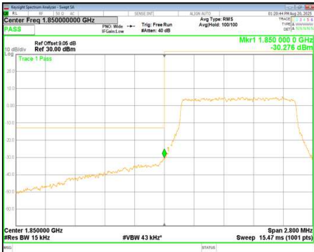
Band25 QPSK BW=1.4MHz Channel=26683 RB Size=6 Position=#0
