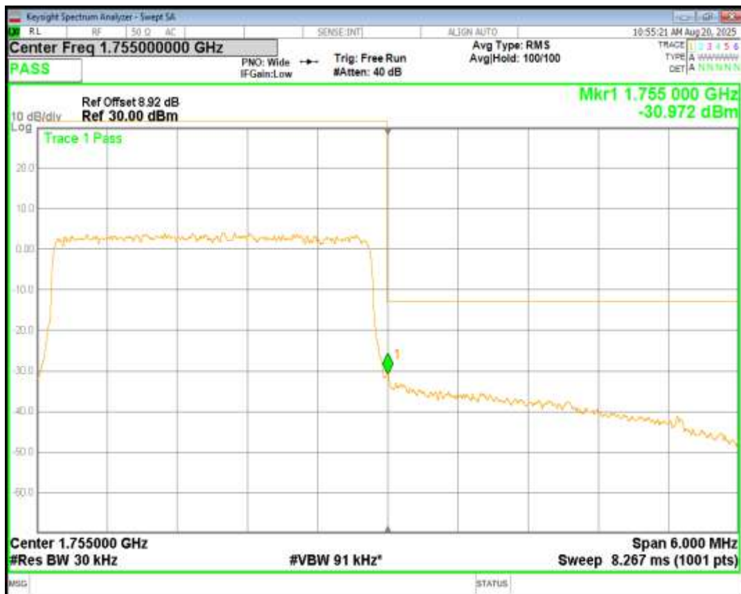
Band4 QPSK BW=5MHz Channel=19975 RB Size=25 Position=#0
