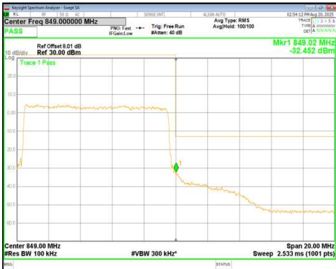
Band26(824-849) QPSK BW=15MHz Channel=26865 RB Size=75 Position=#0
