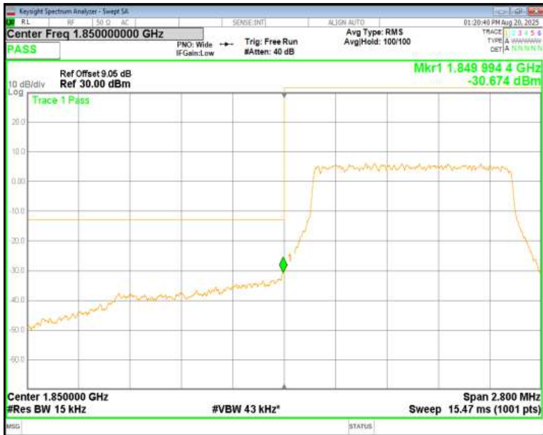
Band25 16QAM BW=1.4MHz Channel=26047 RB Size=6 Position=#0
