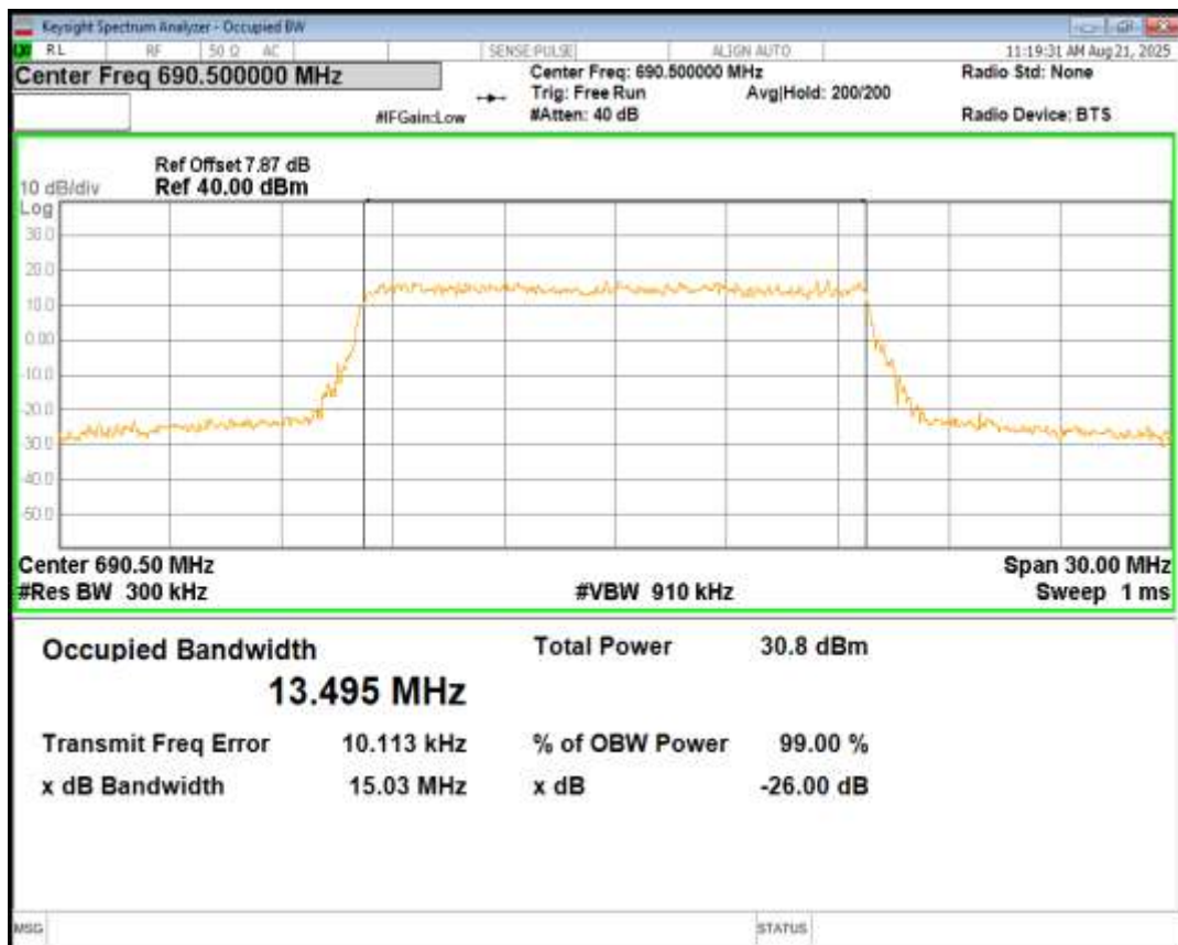
Band71 QPSK BW=20MHz Channel=133222 RB Size=100 Position=#0
