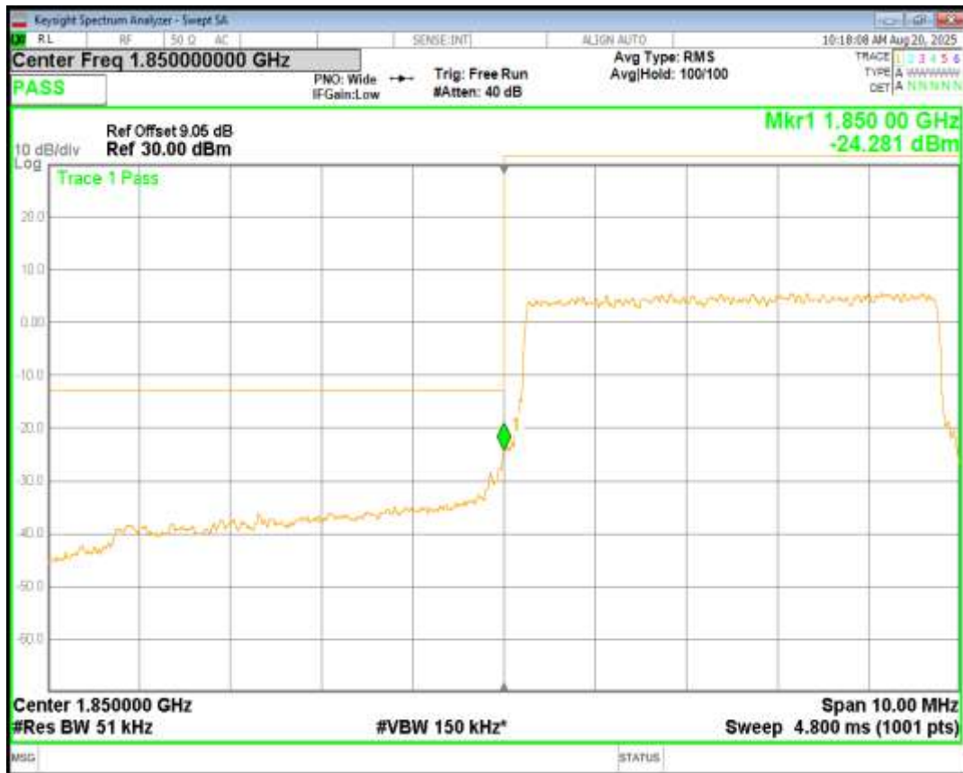
Band2 16QAM BW=5MHz Channel=18625 RB Size=25 Position=#0
