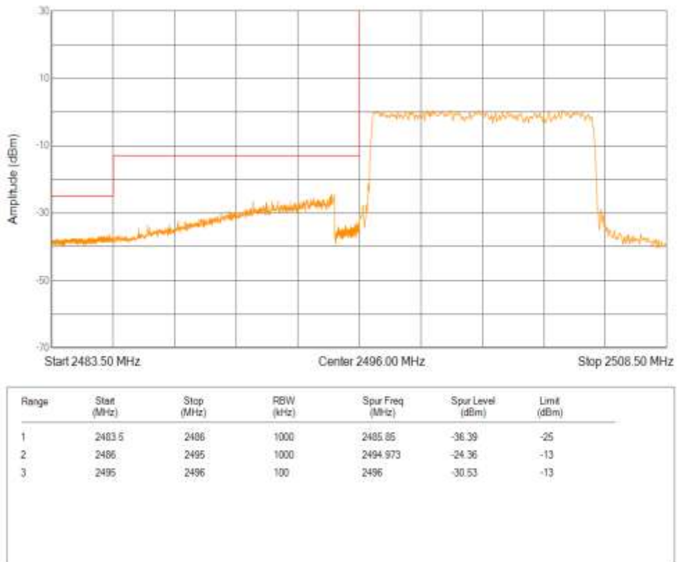
Band41 QPSK BW=10MHz Channel=41540 RB Size=50 Position=#0
