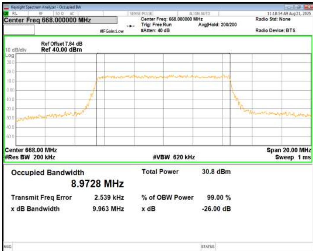
Band71 QPSK BW=10MHz Channel=133297 RB Size=50 Position=#0
