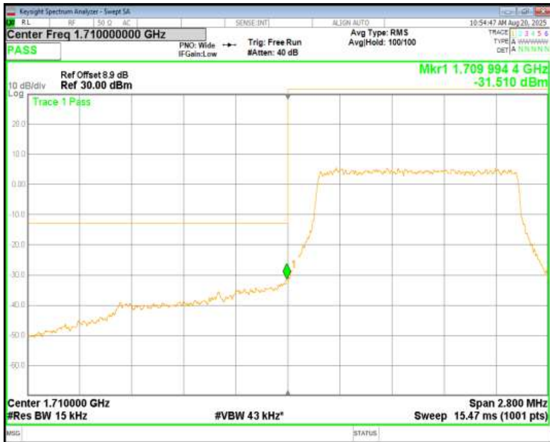
Band4 16QAM BW=1.4MHz Channel=19957 RB Size=6 Position=#0
