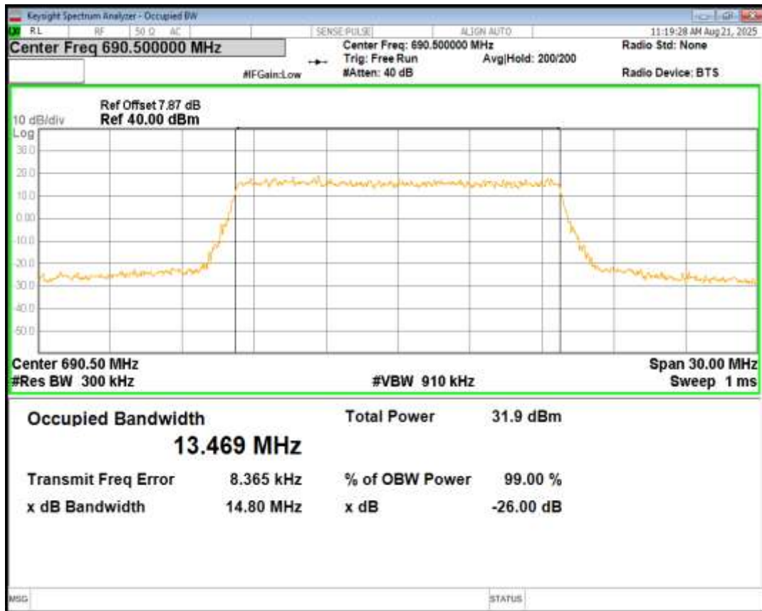
Band71 16QAM BW=15MHz Channel=133397 RB Size=75 Position=#0
