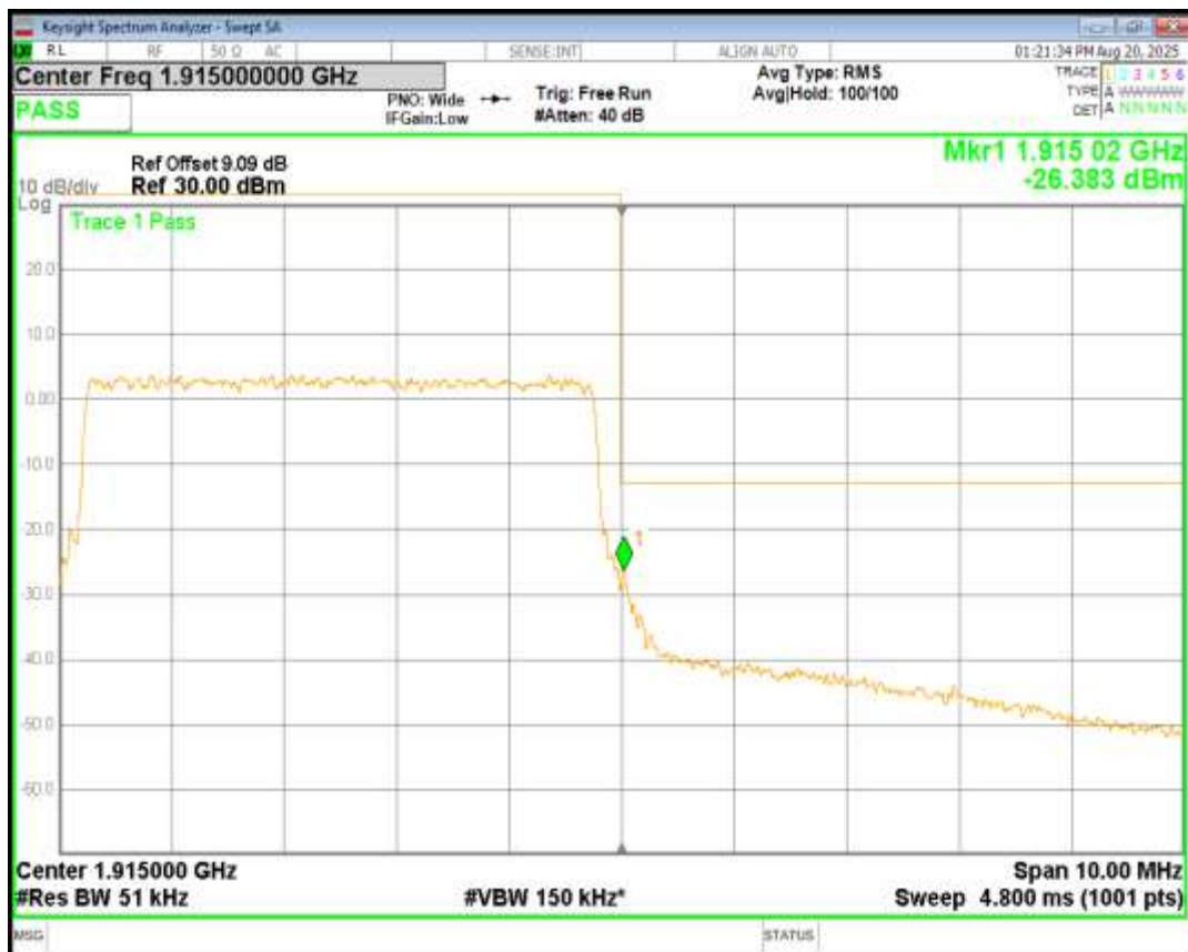
Band25 QPSK BW=10MHz Channel=26090 RB Size=50 Position=#0
