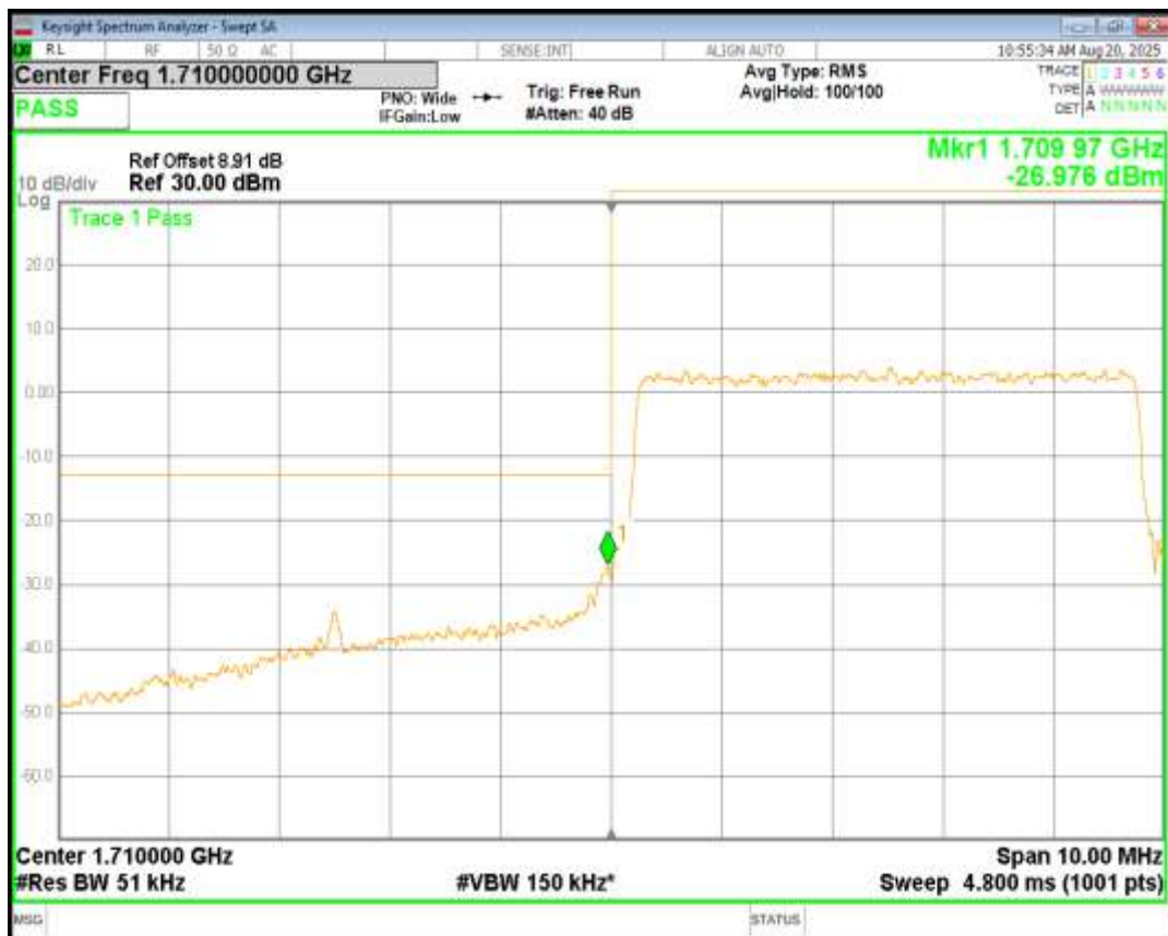
Band4 QPSK BW=5MHz Channel=20375 RB Size=25 Position=#0
