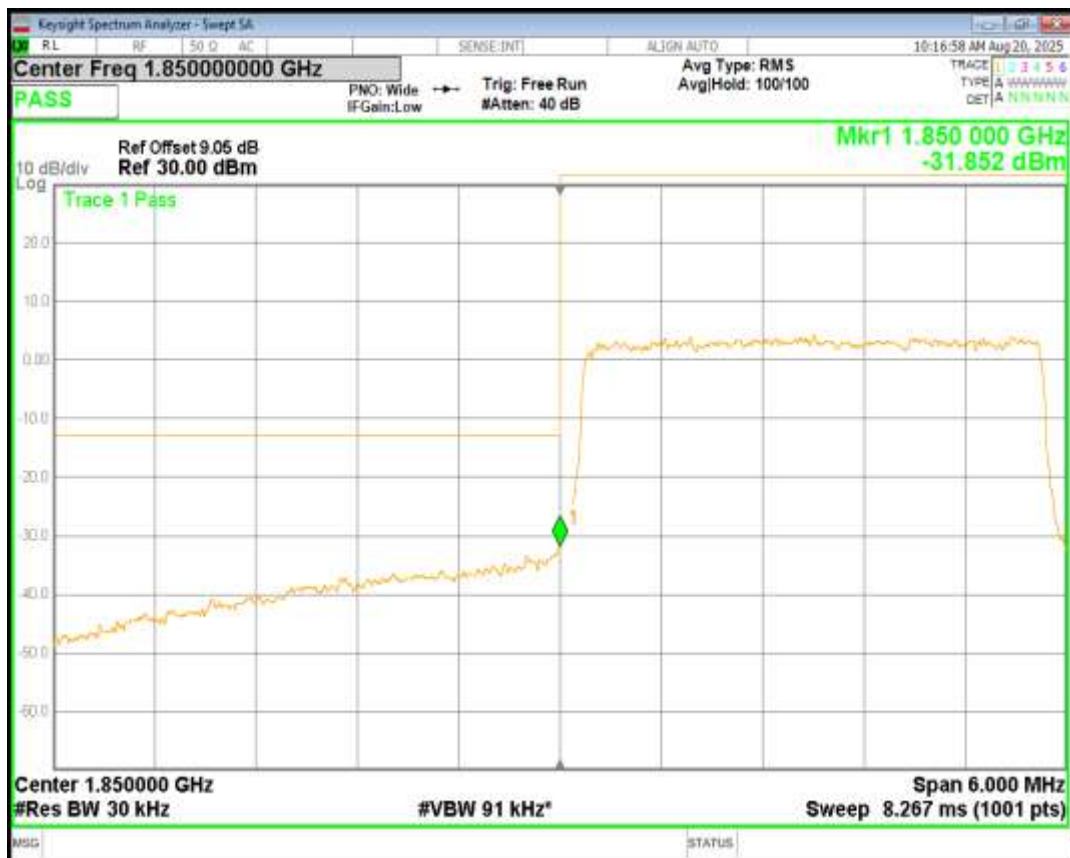
Band2 QPSK BW=3MHz Channel=19185 RB Size=15 Position=#0
