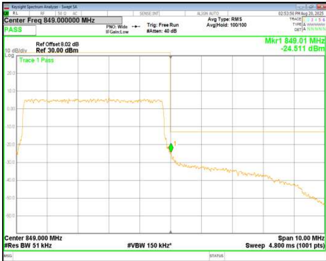
Band26(824-849) 16QAM BW=5MHz Channel=27015 RB Size=25 Position=#0
