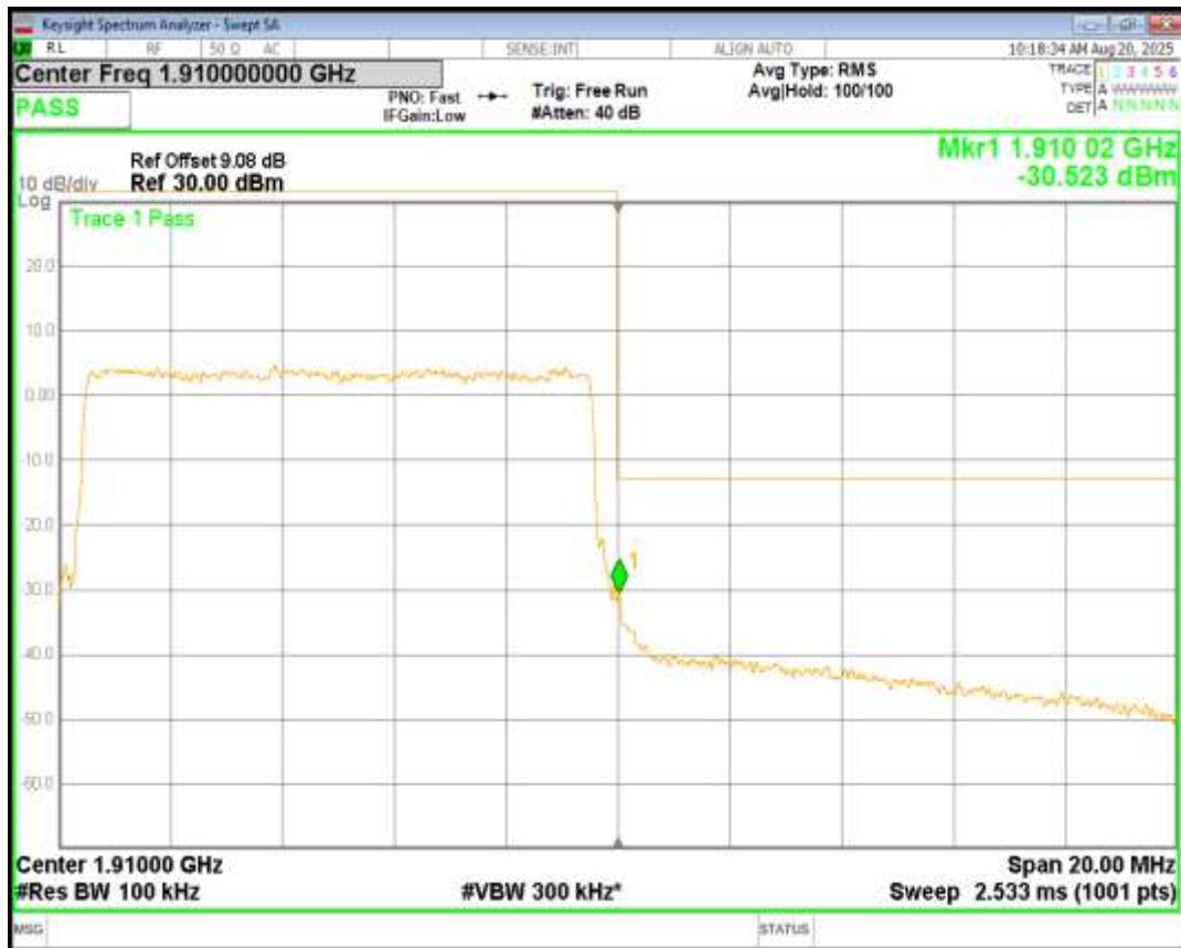
Band2 16QAM BW=10MHz Channel=19150 RB Size=50 Position=#0
