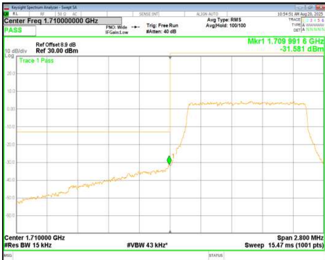
Band4 QPSK BW=1.4MHz Channel=20393 RB Size=6 Position=#0
