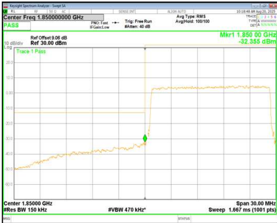
Band2 16QAM BW=15MHz Channel=18675 RB Size=75 Position=#0
