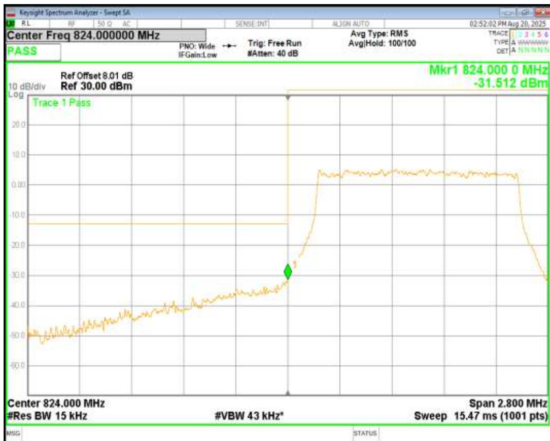
Band26(824-849) QPSK BW=1.4MHz Channel=27033 RB Size=6 Position=#0
