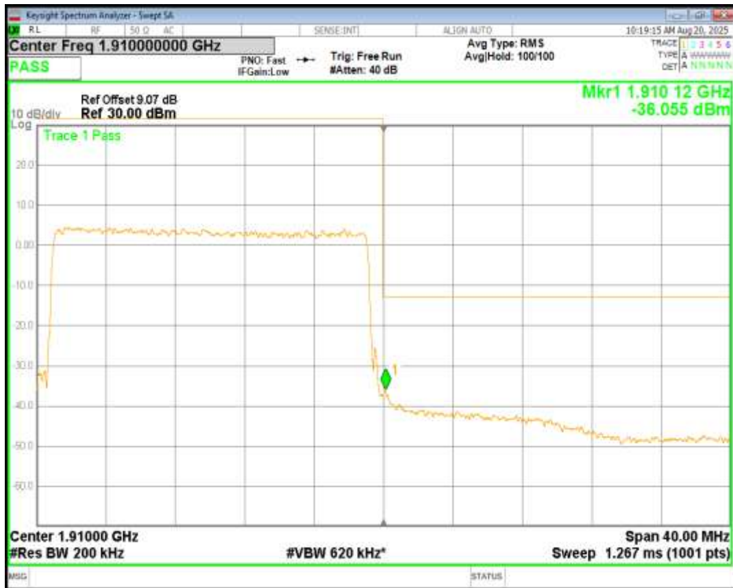
Band2 16QAM BW=20MHz Channel=19100 RB Size=100 Position=#0
