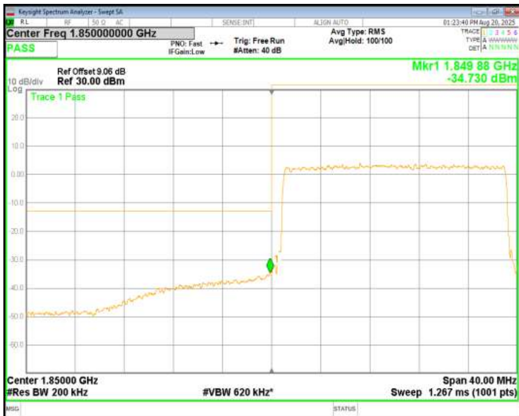
Band25 QPSK BW=20MHz Channel=26590 RB Size=100 Position=#0
