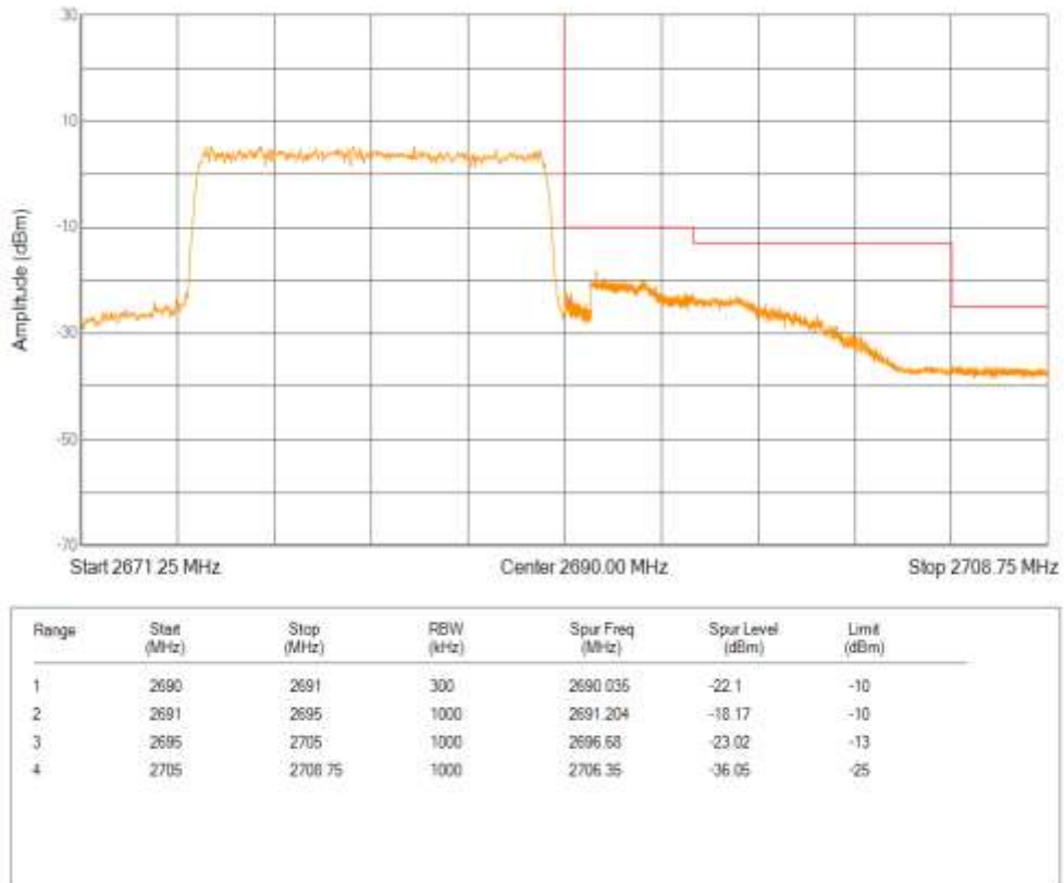
Band41 16QAM BW=15MHz Channel=41515 RB Size=75 Position=#0
