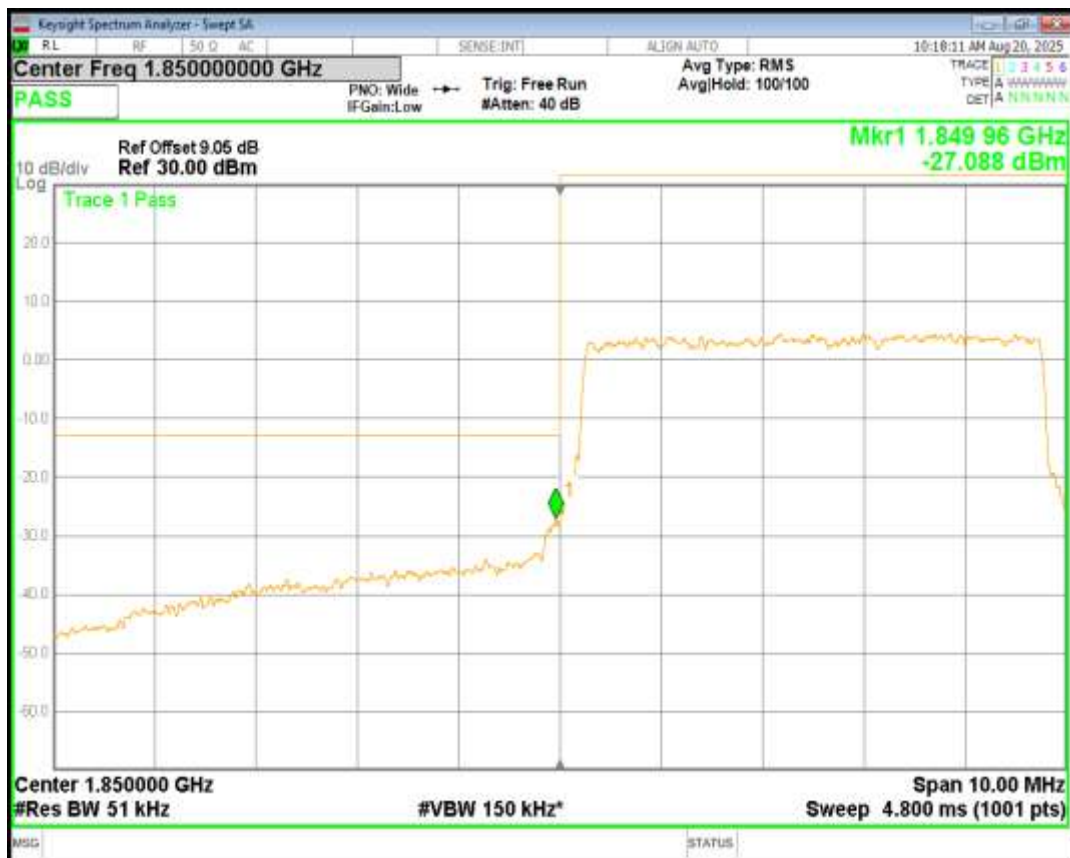
Band2 QPSK BW=5MHz Channel=19175 RB Size=25 Position=#0
