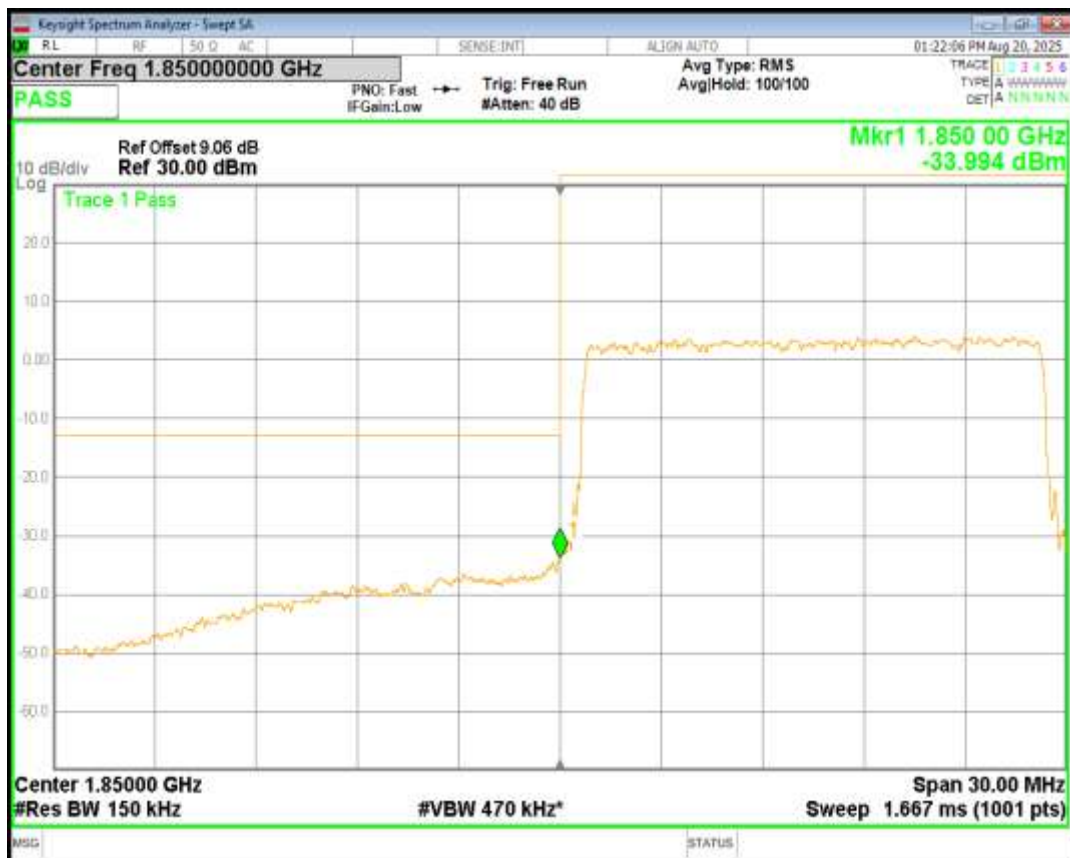
Band25 QPSK BW=15MHz Channel=26615 RB Size=75 Position=#0
