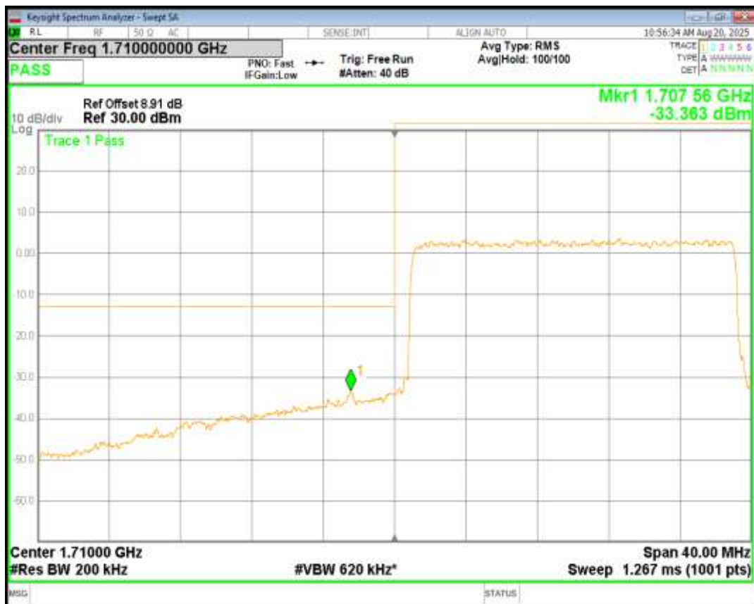
Band4 QPSK BW=20MHz Channel=20300 RB Size=100 Position=#0
