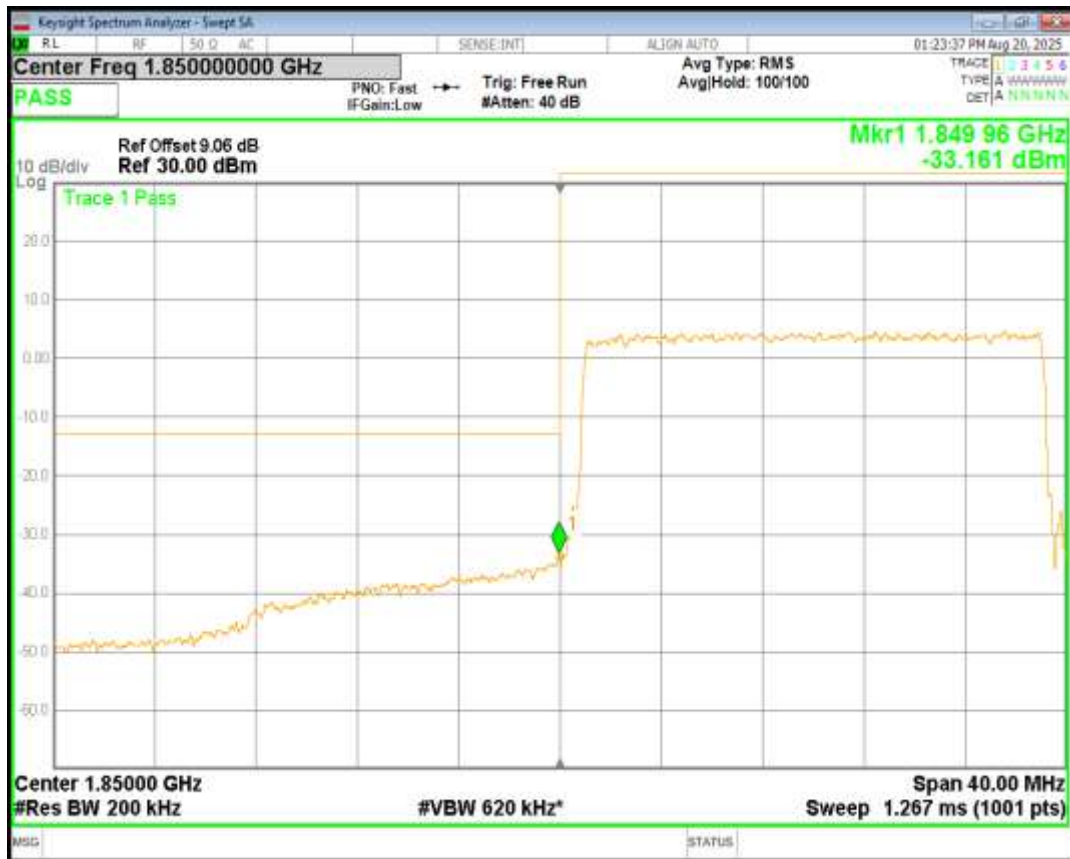
Band25 16QAM BW=20MHz Channel=26140 RB Size=100 Position=#0
