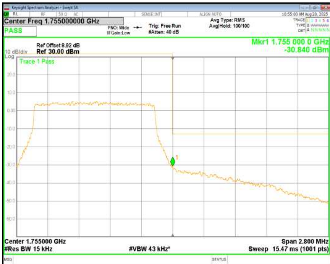
Band4 QPSK BW=3MHz Channel=19965 RB Size=15 Position=#0
