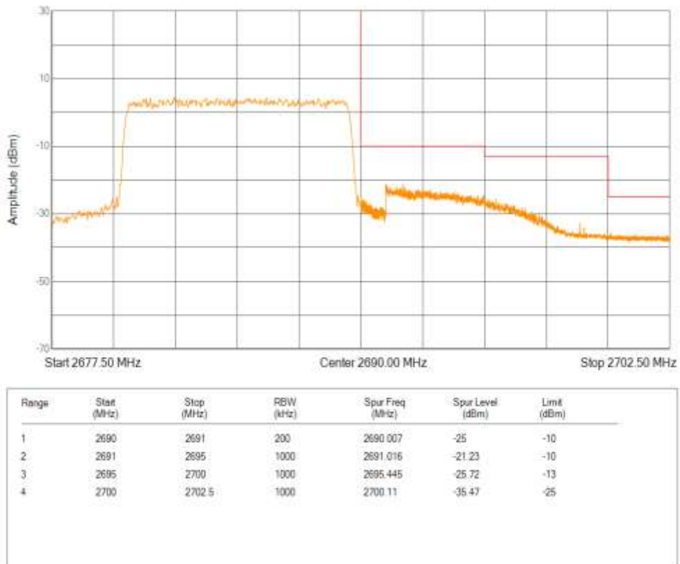
Band41 QPSK BW=15MHz Channel=39725 RB Size=75 Position=#0
