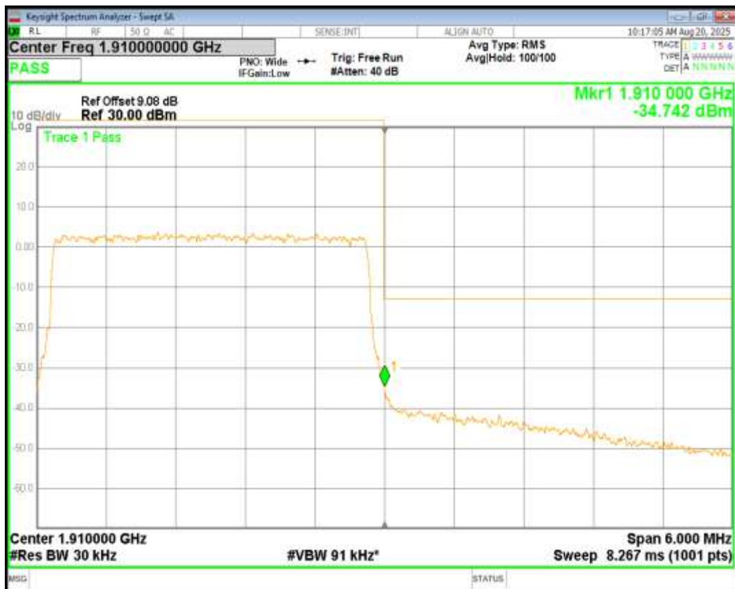
Band2 QPSK BW=5MHz Channel=18625 RB Size=25 Position=#0
