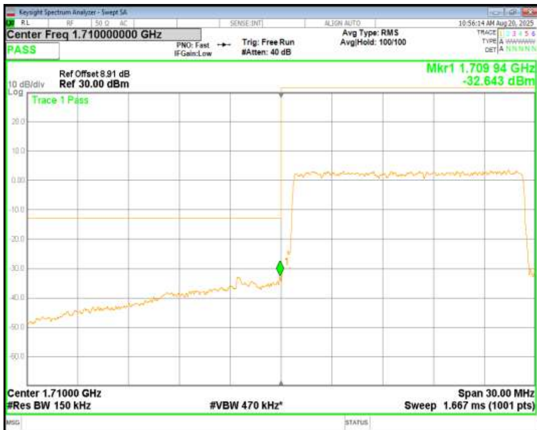
Band4 QPSK BW=15MHz Channel=20325 RB Size=75 Position=#0
