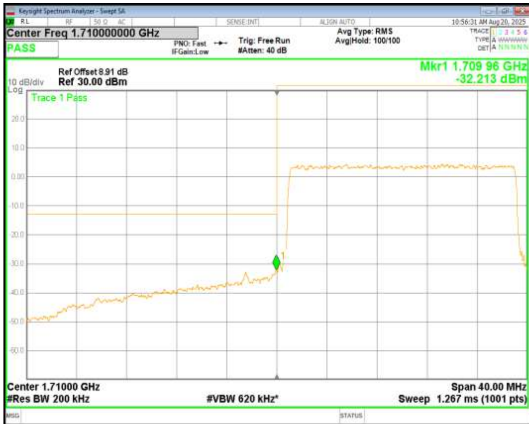
Band4 16QAM BW=20MHz Channel=20050 RB Size=100 Position=#0
