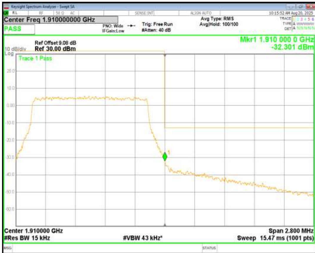
Band2 16QAM BW=1.4MHz Channel=19193 RB Size=6 Position=#0
