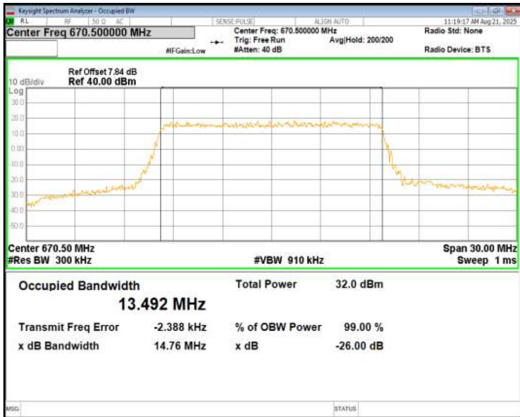
Band71 16QAM BW=15MHz Channel=133197 RB Size=75 Position=#0
