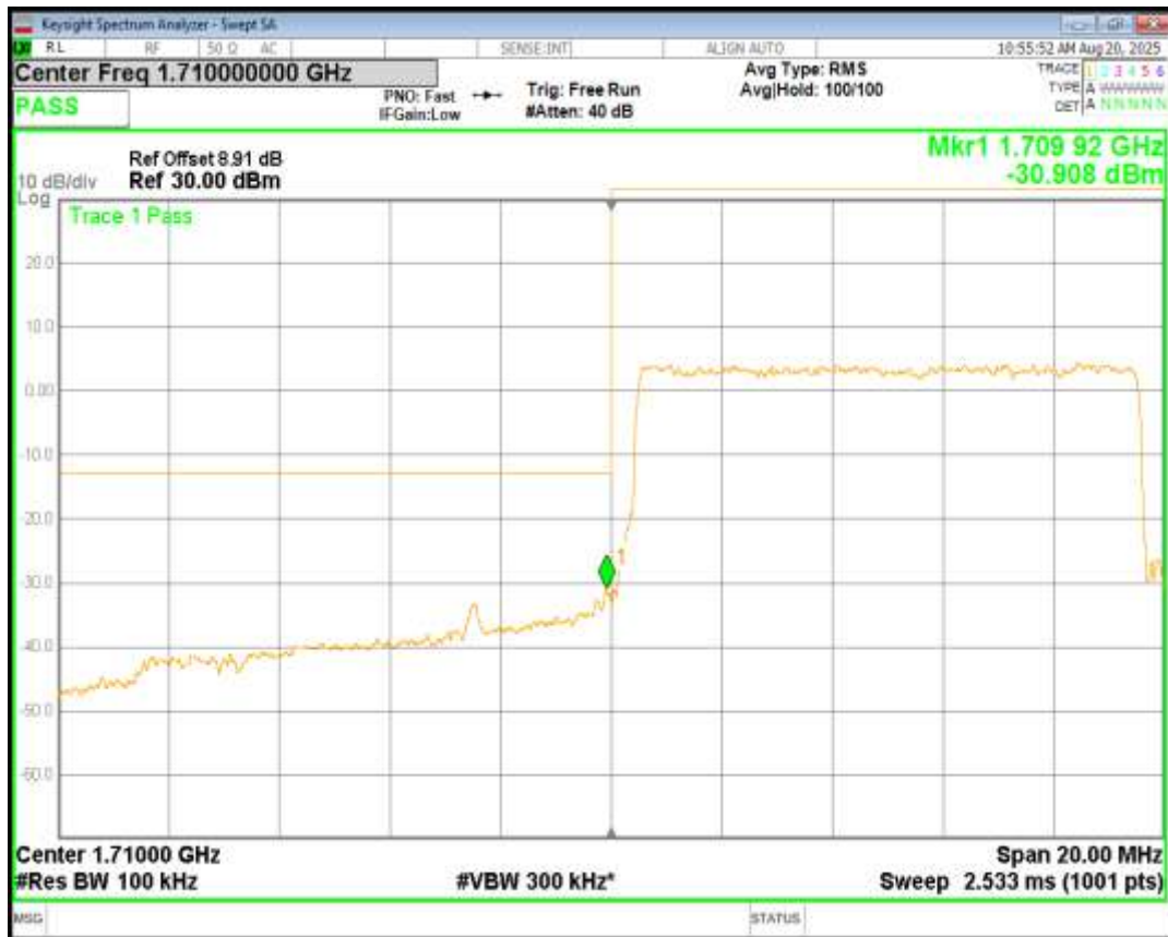
Band4 16QAM BW=10MHz Channel=20000 RB Size=50 Position=#0
