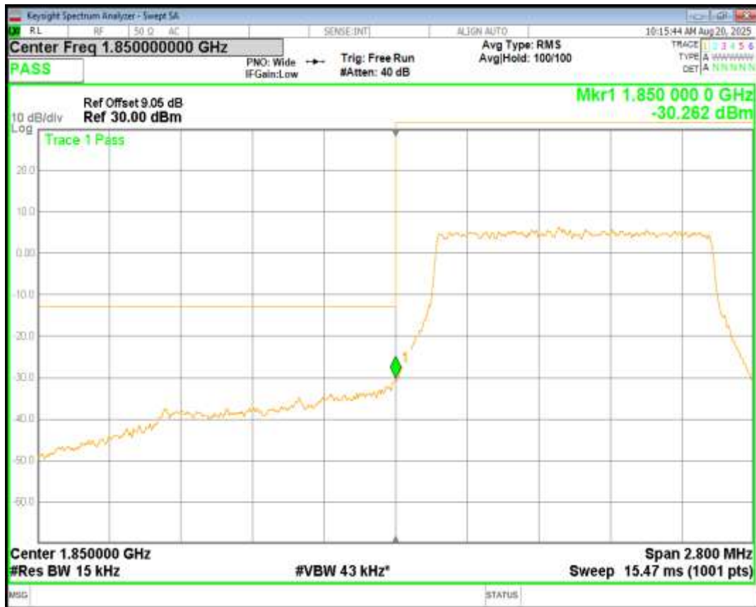
Band2 16QAM BW=1.4MHz Channel=18607 RB Size=6 Position=#0
