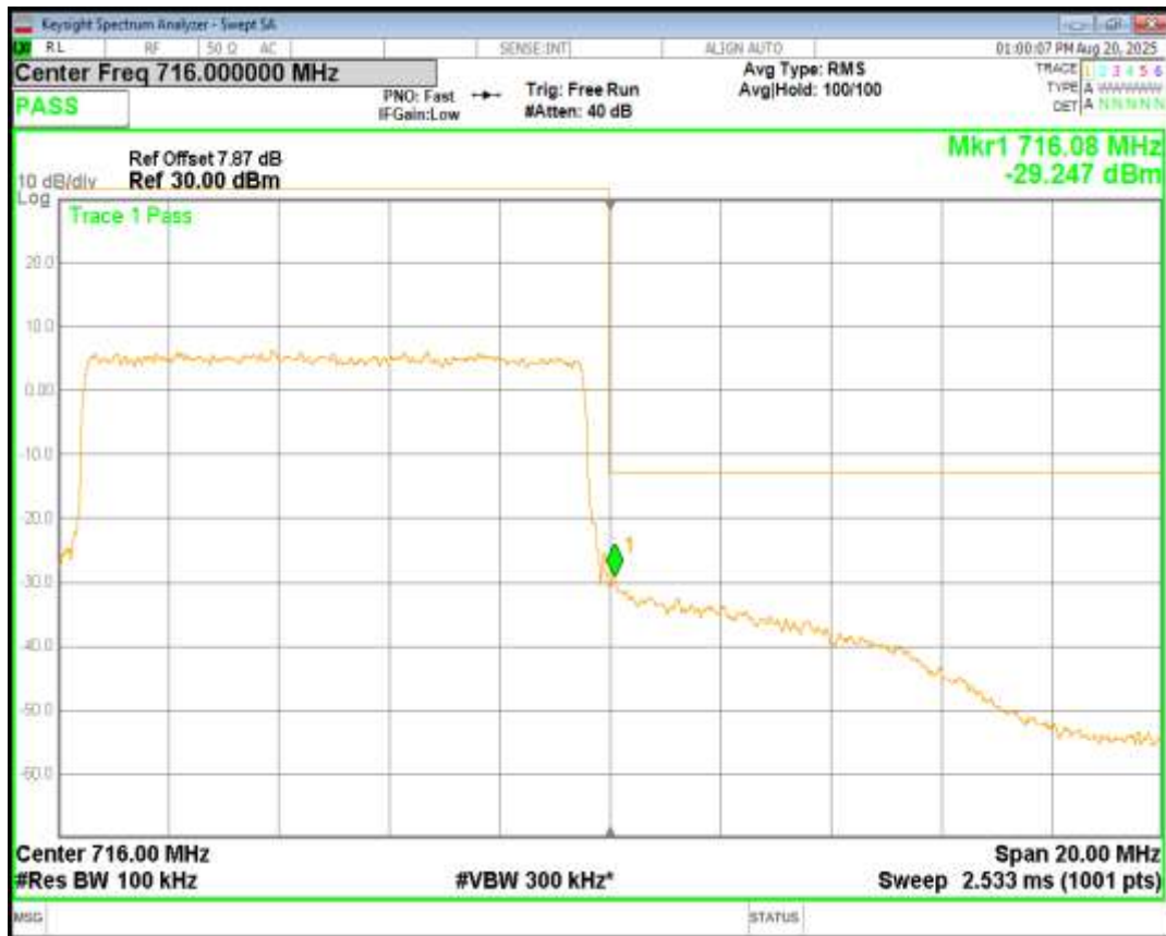
Band17 16QAM BW=10MHz Channel=23800 RB Size=50 Position=#0
