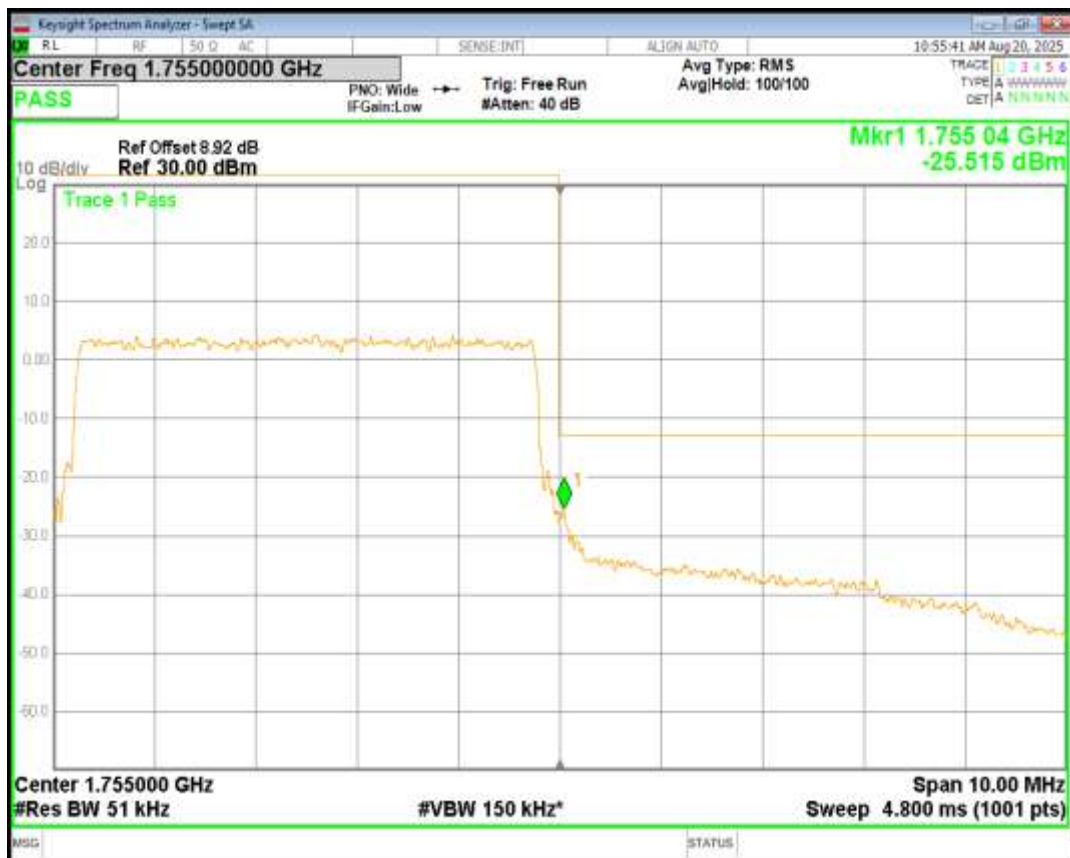
Band4 QPSK BW=10MHz Channel=20000 RB Size=50 Position=#0
