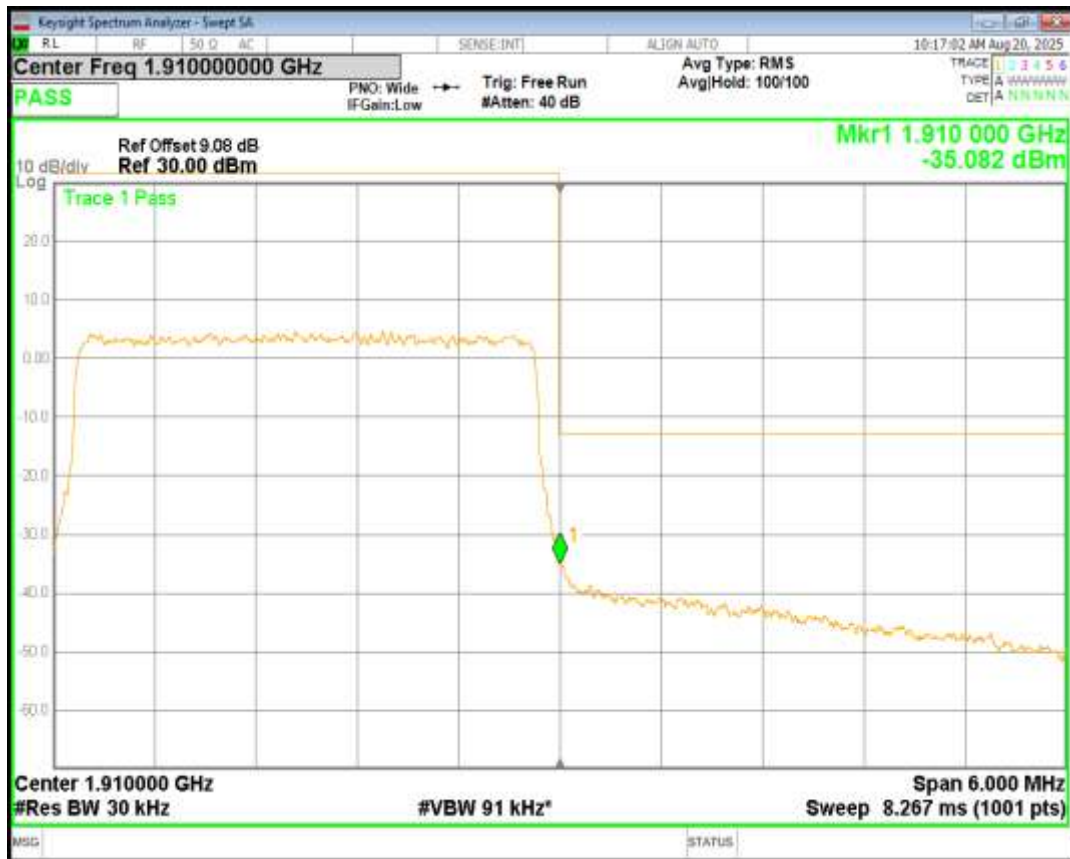
Band2 16QAM BW=3MHz Channel=19185 RB Size=15 Position=#0
