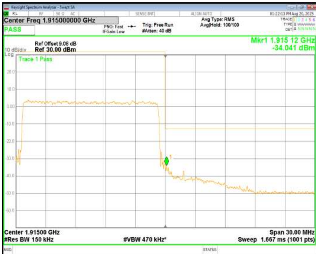
Band25 QPSK BW=20MHz Channel=26140 RB Size=100 Position=#0
