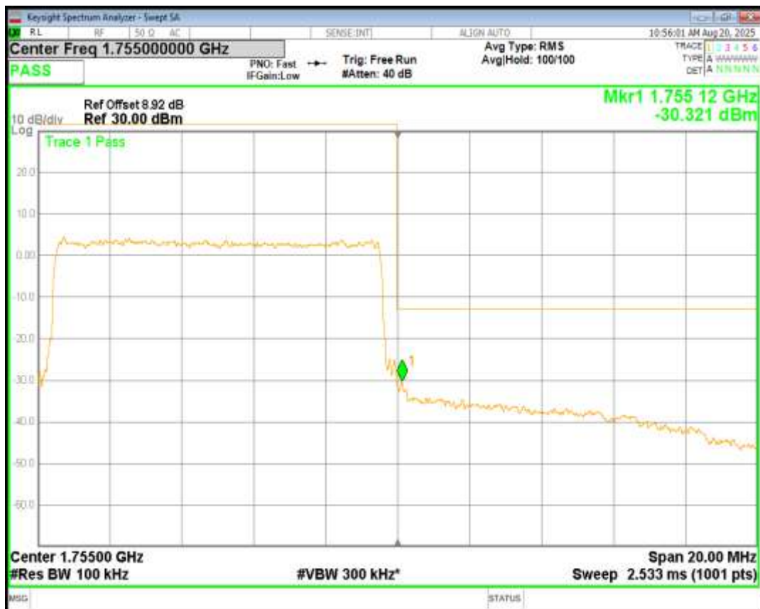
Band4 QPSK BW=15MHz Channel=20025 RB Size=75 Position=#0
