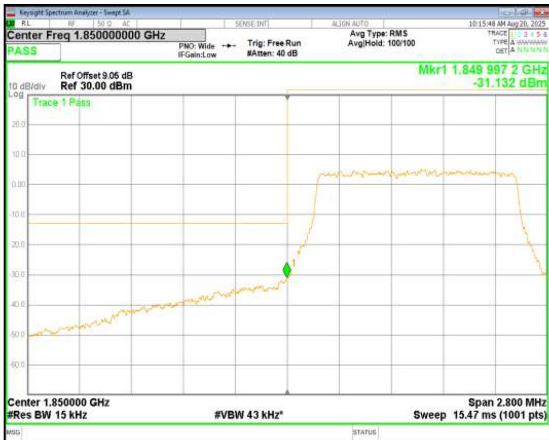
Band2 QPSK BW=1.4MHz Channel=19193 RB Size=6 Position=#0
