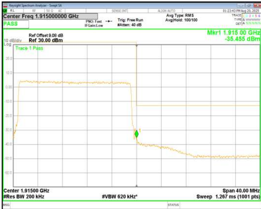
Band25 16QAM BW=20MHz Channel=26590 RB Size=100 Position=#0
