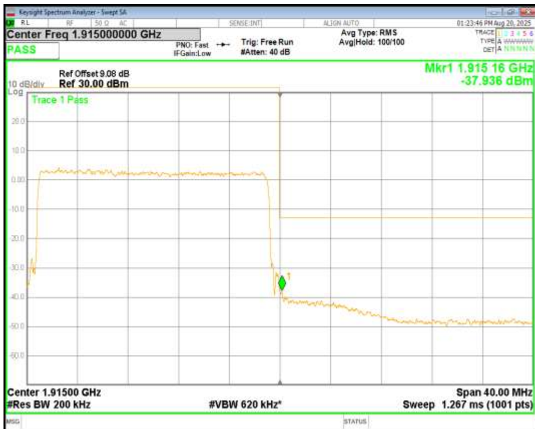
Band26(814-824) QPSK BW=1.4MHz Channel=26697 RB Size=6 Position=#0
