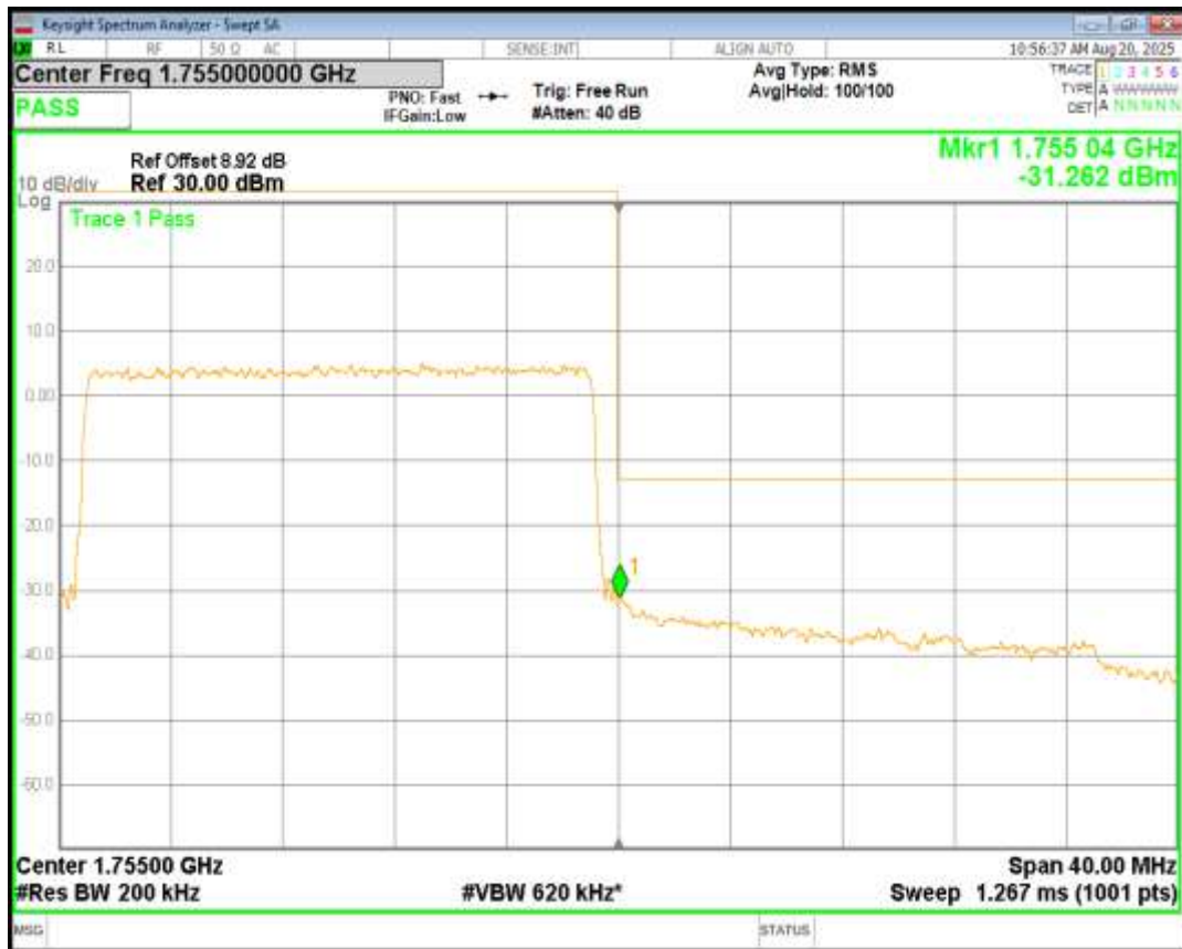
Band4 16QAM BW=20MHz Channel=20300 RB Size=100 Position=#0
