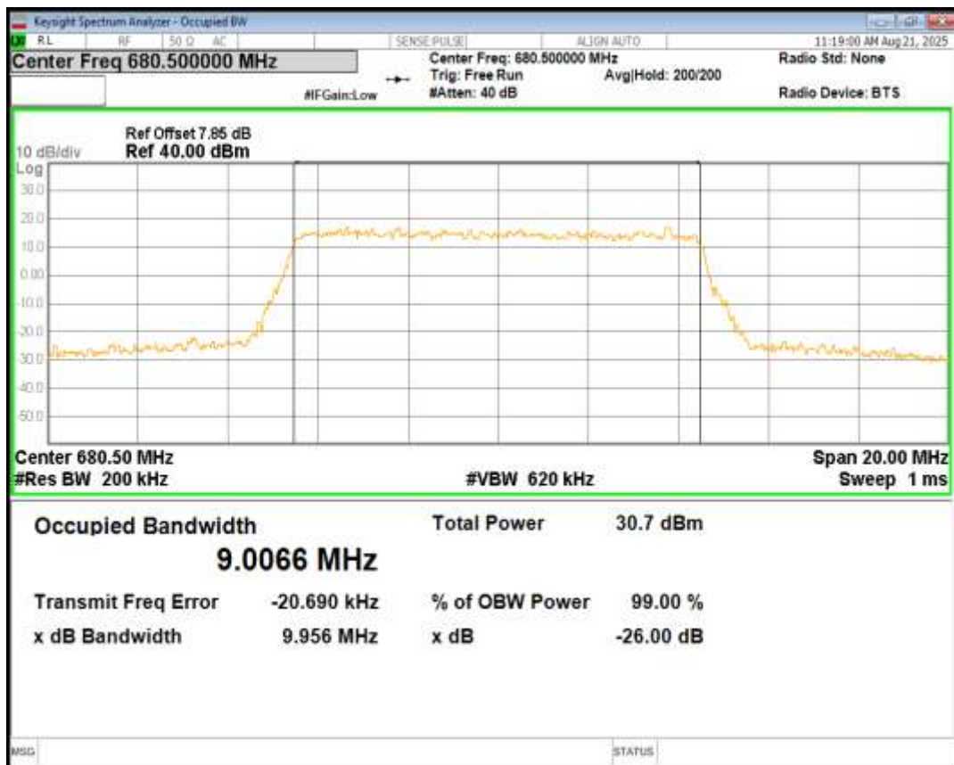
Band71 QPSK BW=10MHz Channel=133422 RB Size=50 Position=#0
