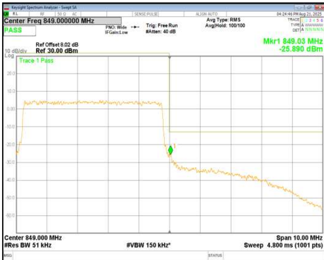
Band5 QPSK BW=10MHz Channel=20450 RB Size=50 Position=#0
