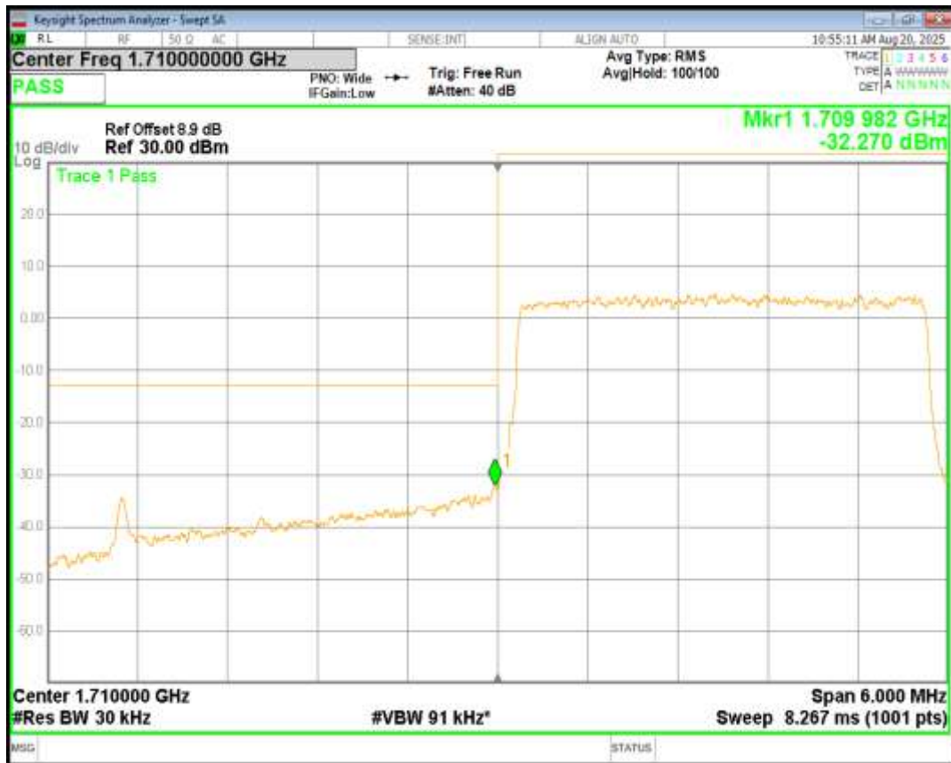
Band4 16QAM BW=3MHz Channel=19965 RB Size=15 Position=#0
