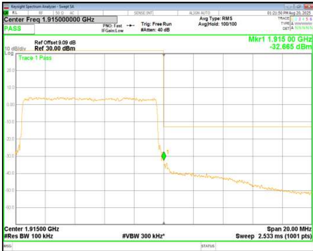
Band25 16QAM BW=10MHz Channel=26640 RB Size=50 Position=#0
