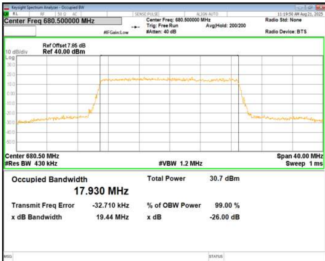
Band71 QPSK BW=20MHz Channel=133372 RB Size=100 Position=#0
