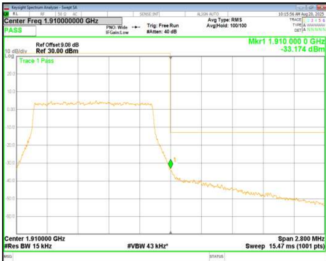
Band2 QPSK BW=3MHz Channel=18615 RB Size=15 Position=#0
