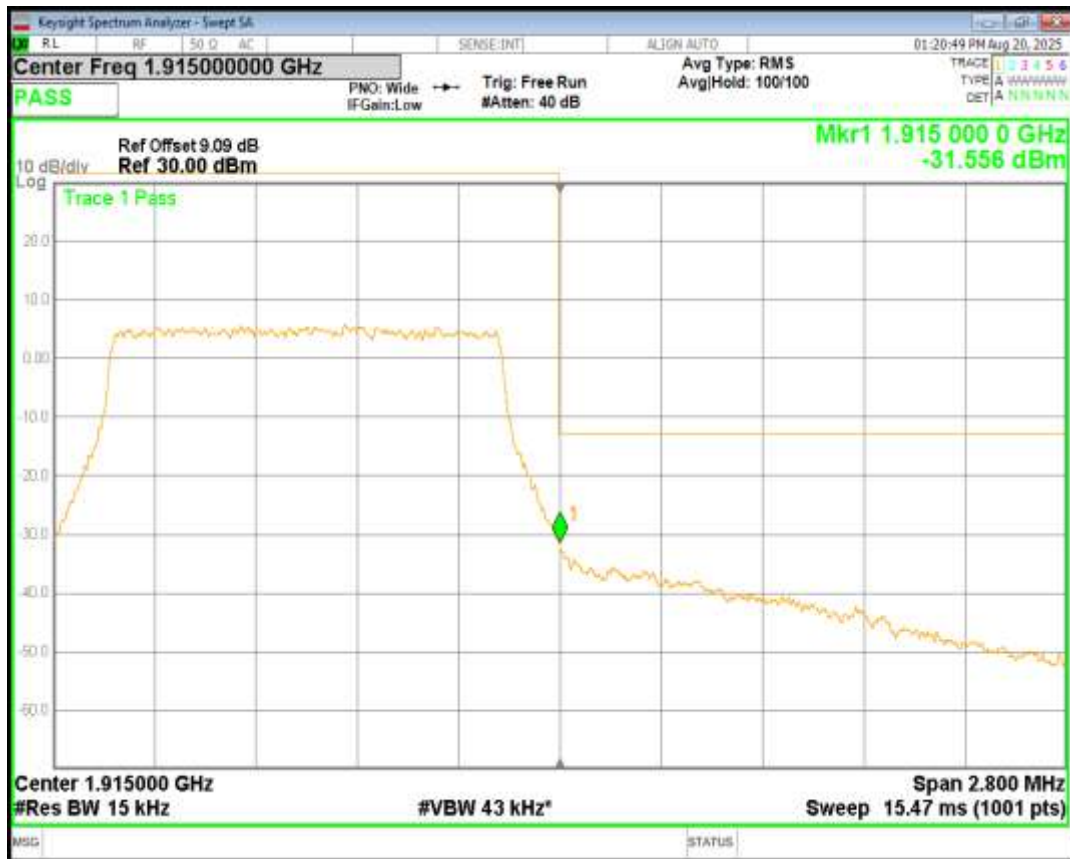
Band25 16QAM BW=1.4MHz Channel=26683 RB Size=6 Position=#0
