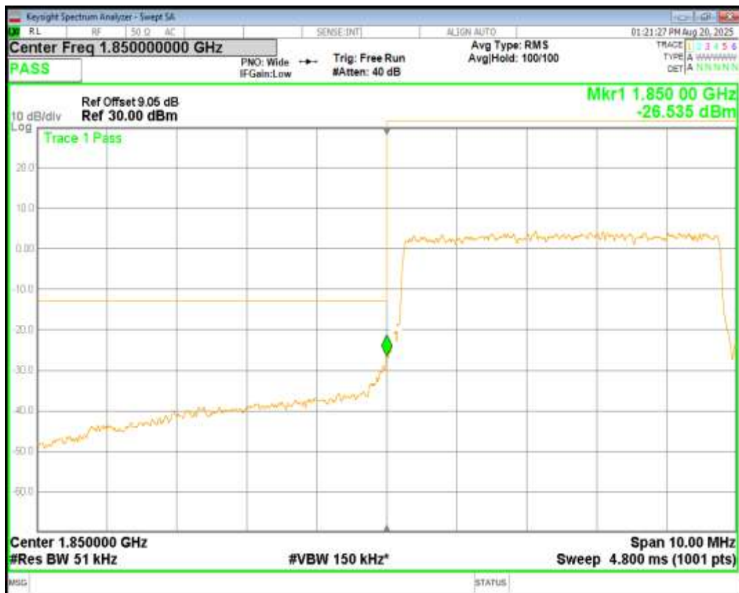
Band25 QPSK BW=5MHz Channel=26665 RB Size=25 Position=#0
