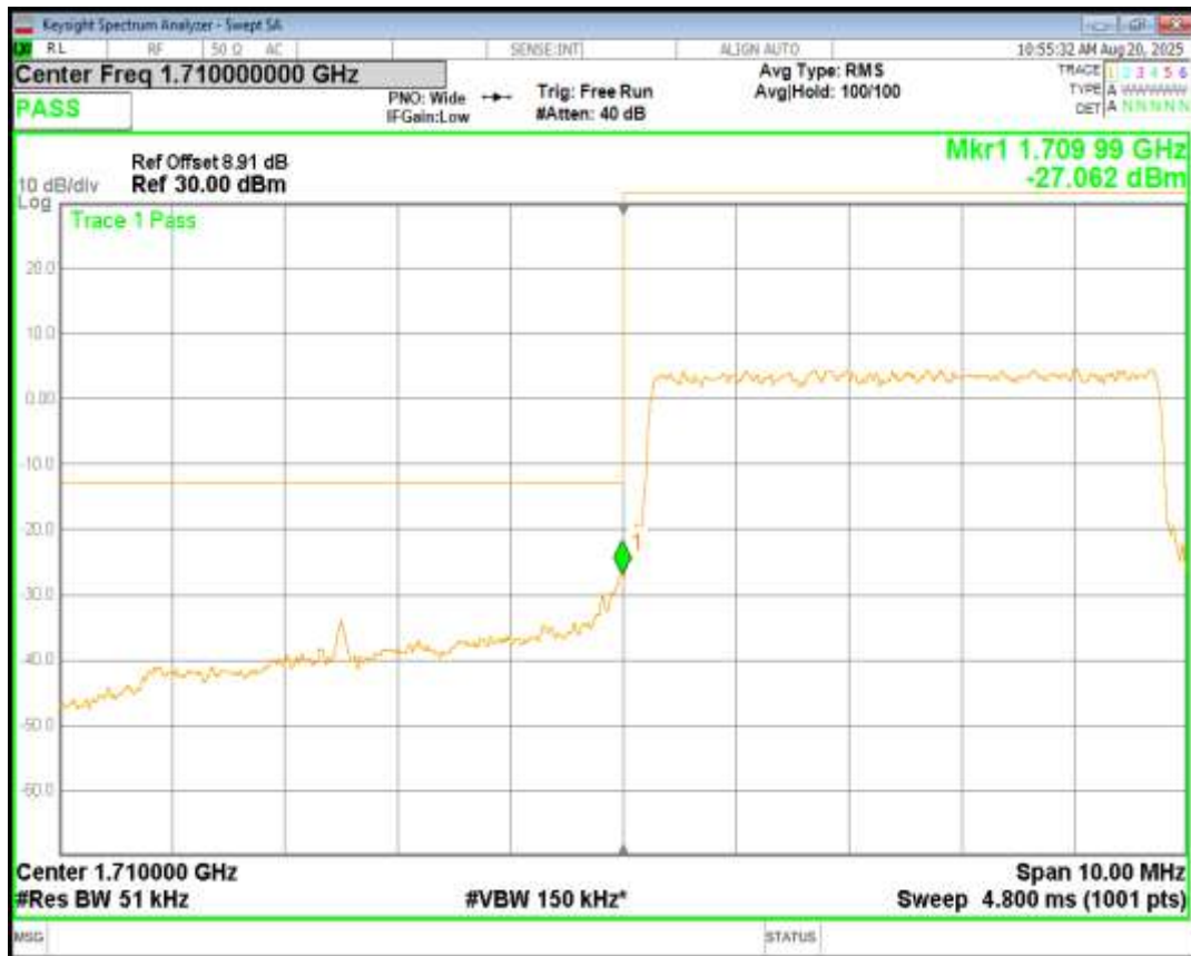
Band4 16QAM BW=5MHz Channel=19975 RB Size=25 Position=#0
