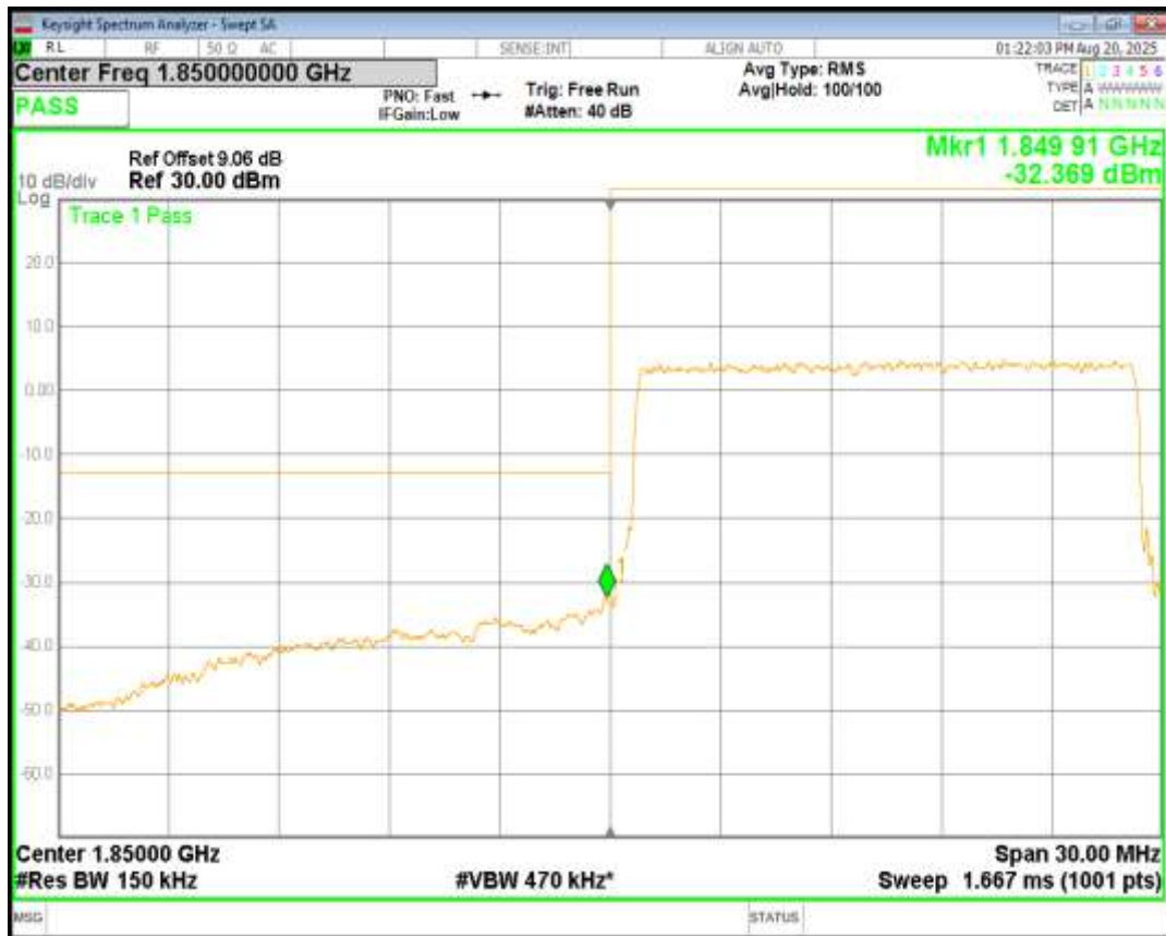
Band25 16QAM BW=15MHz Channel=26115 RB Size=75 Position=#0
