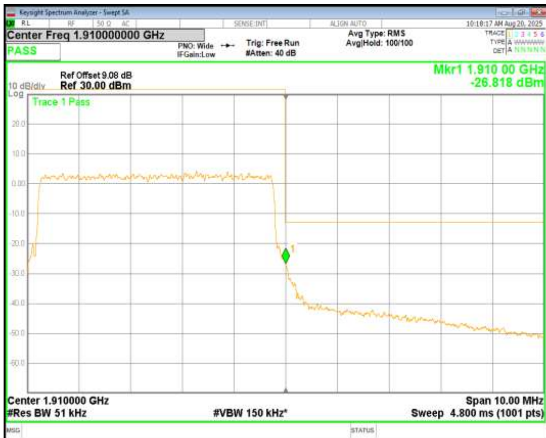
Band2 QPSK BW=10MHz Channel=18650 RB Size=50 Position=#0
