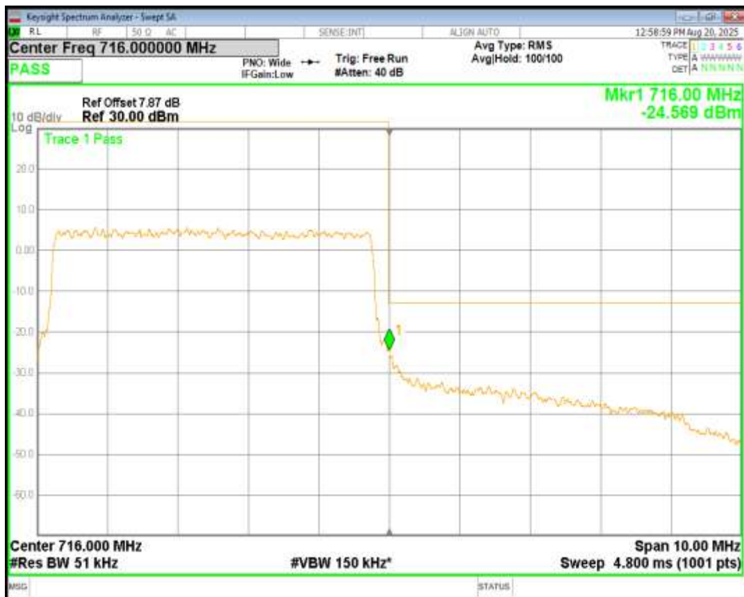
Band17 QPSK BW=10MHz Channel=23780 RB Size=50 Position=#0
