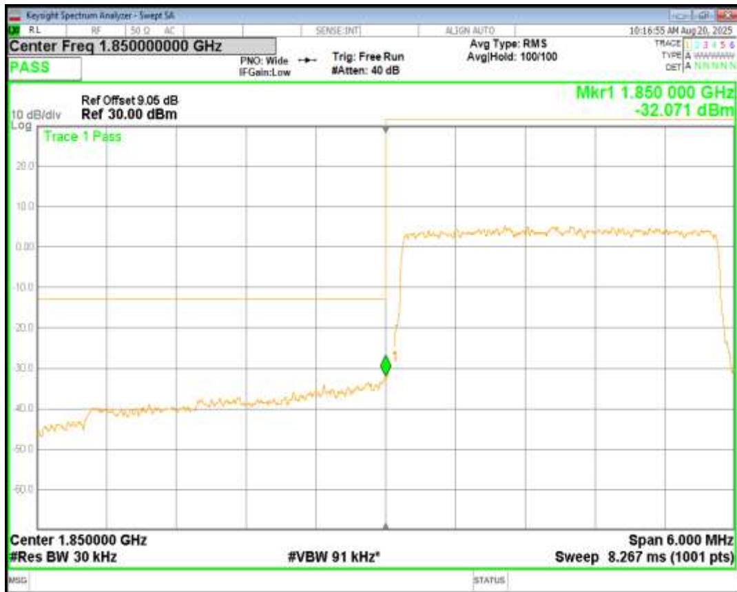
Band2 16QAM BW=3MHz Channel=18615 RB Size=15 Position=#0
