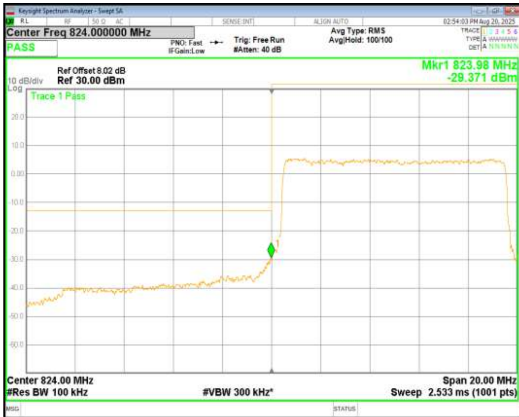
Band26(824-849) 16QAM BW=10MHz Channel=26840 RB Size=50 Position=#0
