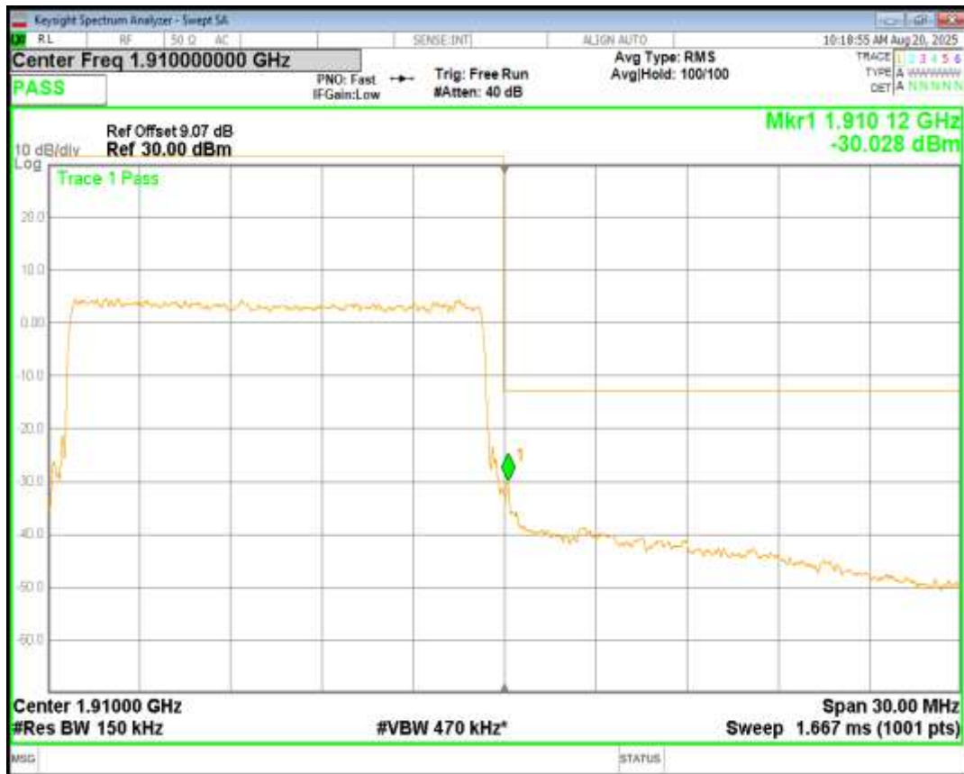
Band2 16QAM BW=15MHz Channel=19125 RB Size=75 Position=#0
