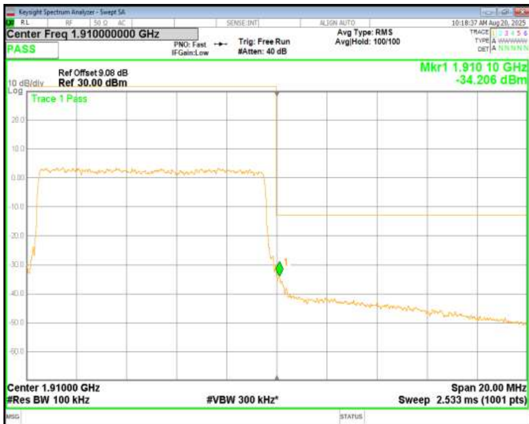
Band2 QPSK BW=15MHz Channel=18675 RB Size=75 Position=#0
