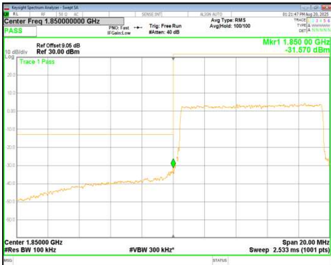
Band25 QPSK BW=10MHz Channel=26640 RB Size=50 Position=#0
