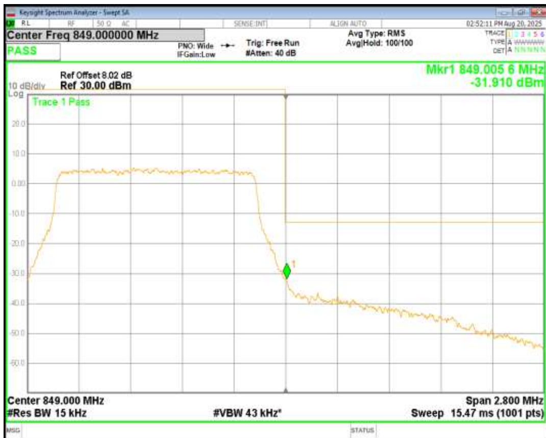
Band26(824-849) QPSK BW=3MHz Channel=26805 RB Size=15 Position=#0
