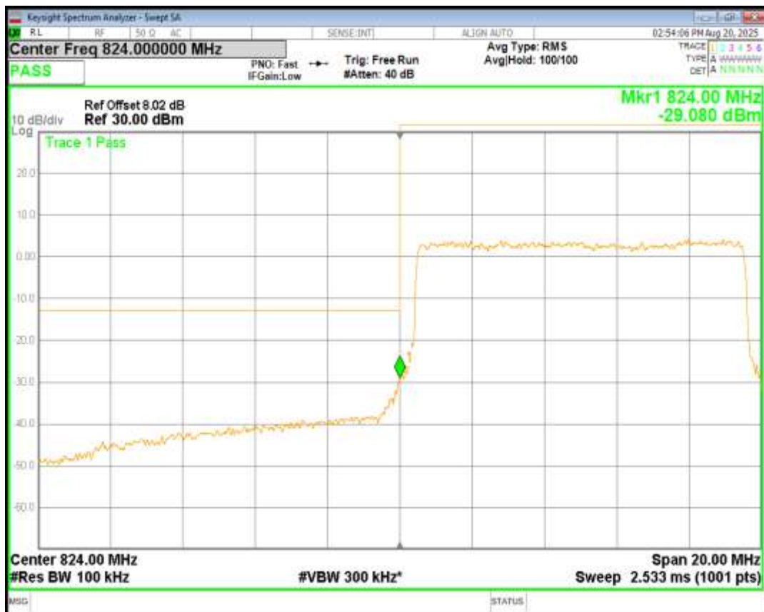
Band26(824-849) QPSK BW=10MHz Channel=26990 RB Size=50 Position=#0
