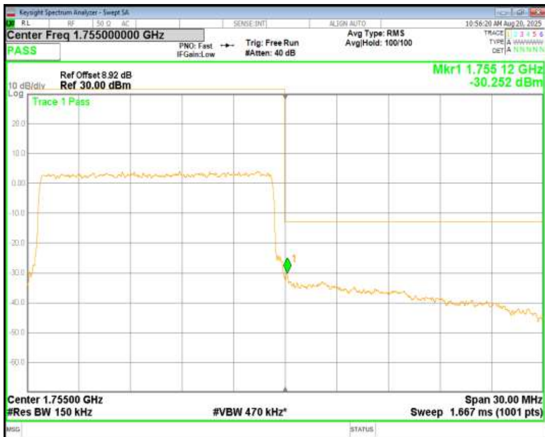
Band4 QPSK BW=20MHz Channel=20050 RB Size=100 Position=#0
