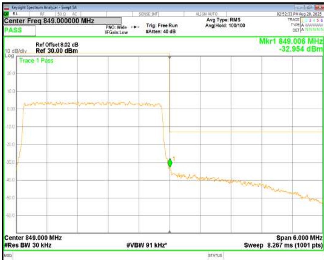
Band26(824-849) QPSK BW=5MHz Channel=26815 RB Size=25 Position=#0
