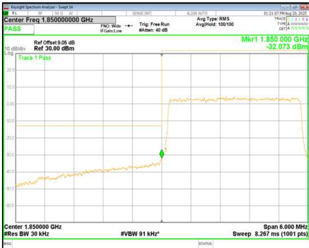
Band25 QPSK BW=3MHz Channel=26675 RB Size=15 Position=#0
