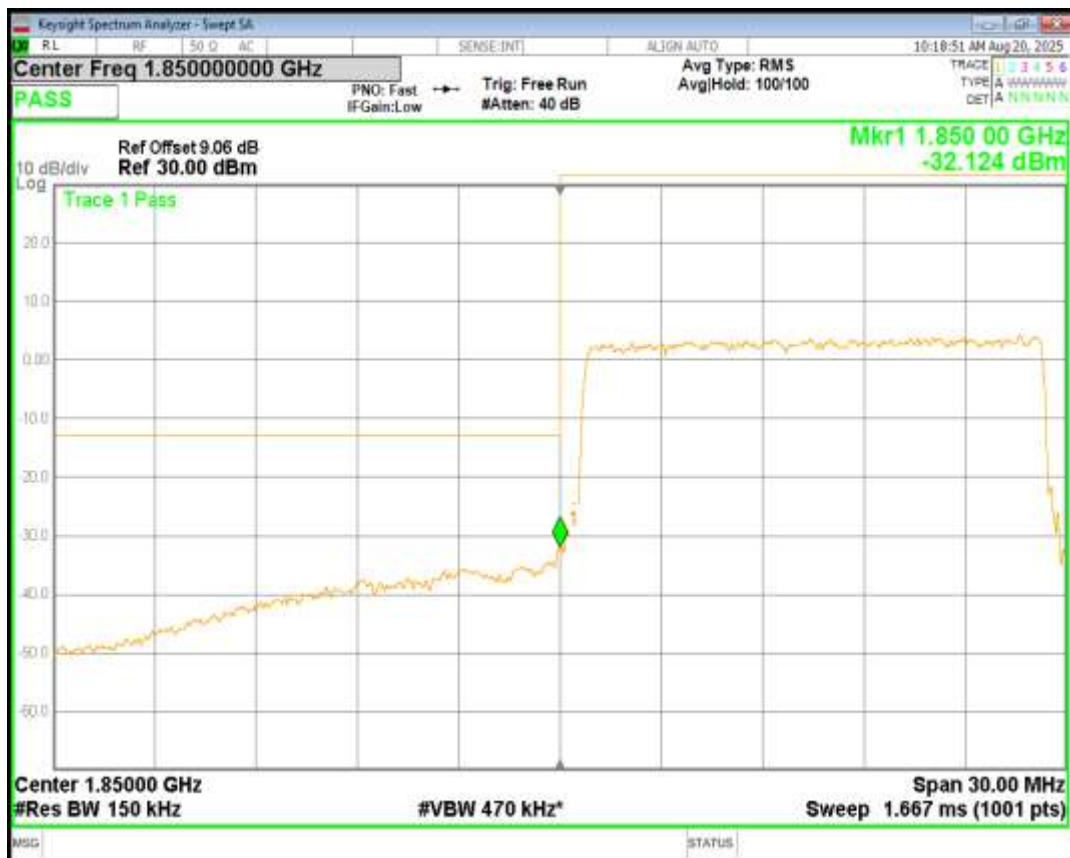
Band2 QPSK BW=15MHz Channel=19125 RB Size=75 Position=#0
