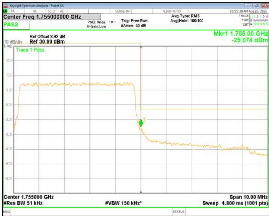
Band4 16QAM BW=5MHz Channel=20375 RB Size=25 Position=#0
