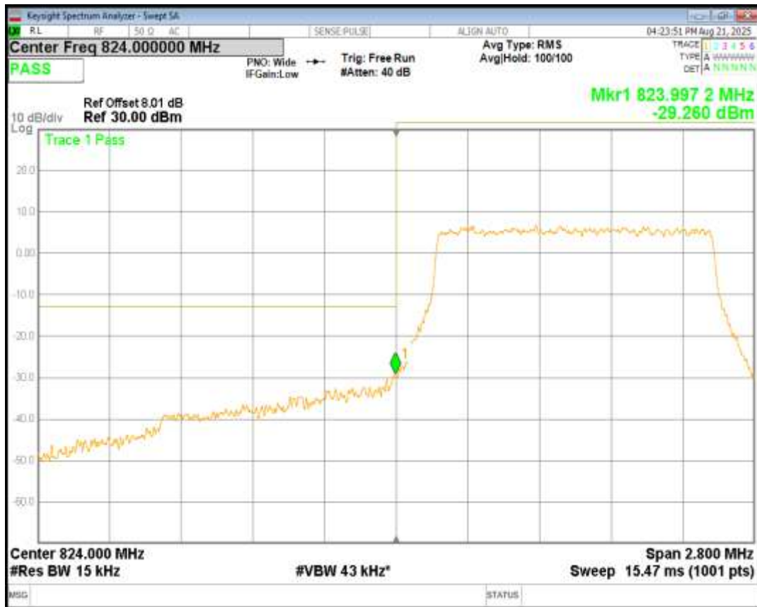
Band5 16QAM BW=1.4MHz Channel=20407 RB Size=6 Position=#0
