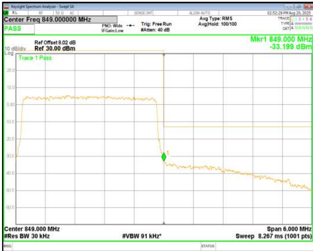
Band26(824-849) 16QAM BW=3MHz Channel=27025 RB Size=15 Position=#0
