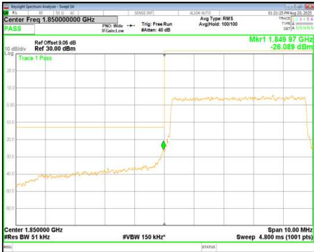
Band25 16QAM BW=5MHz Channel=26065 RB Size=25 Position=#0
