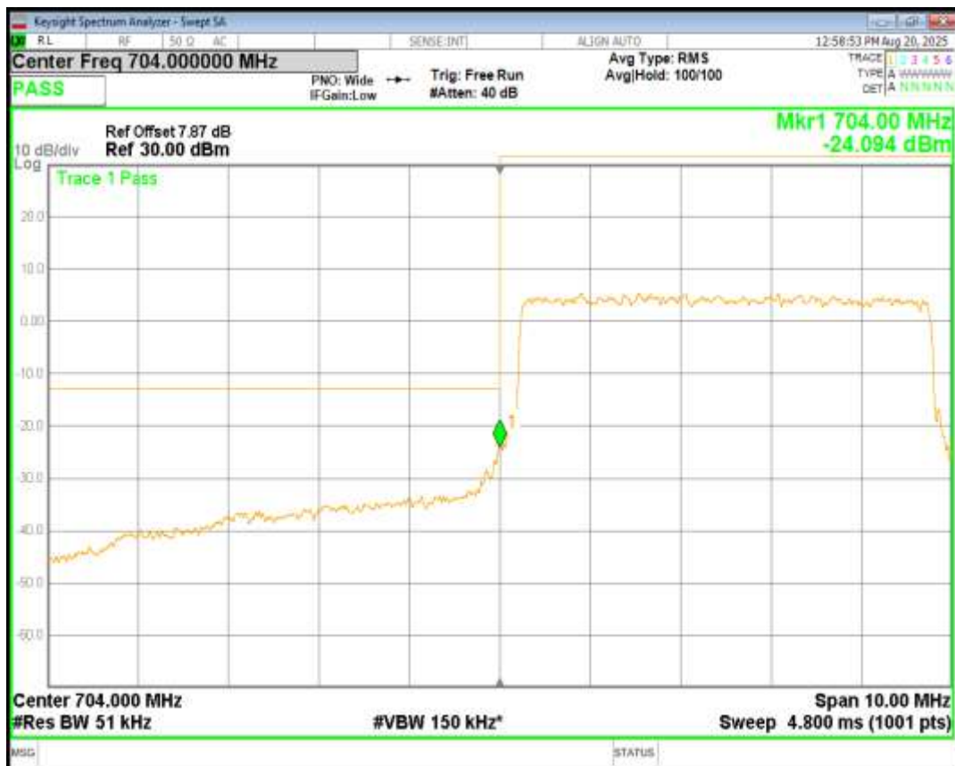
Band17 QPSK BW=5MHz Channel=23825 RB Size=25 Position=#0
