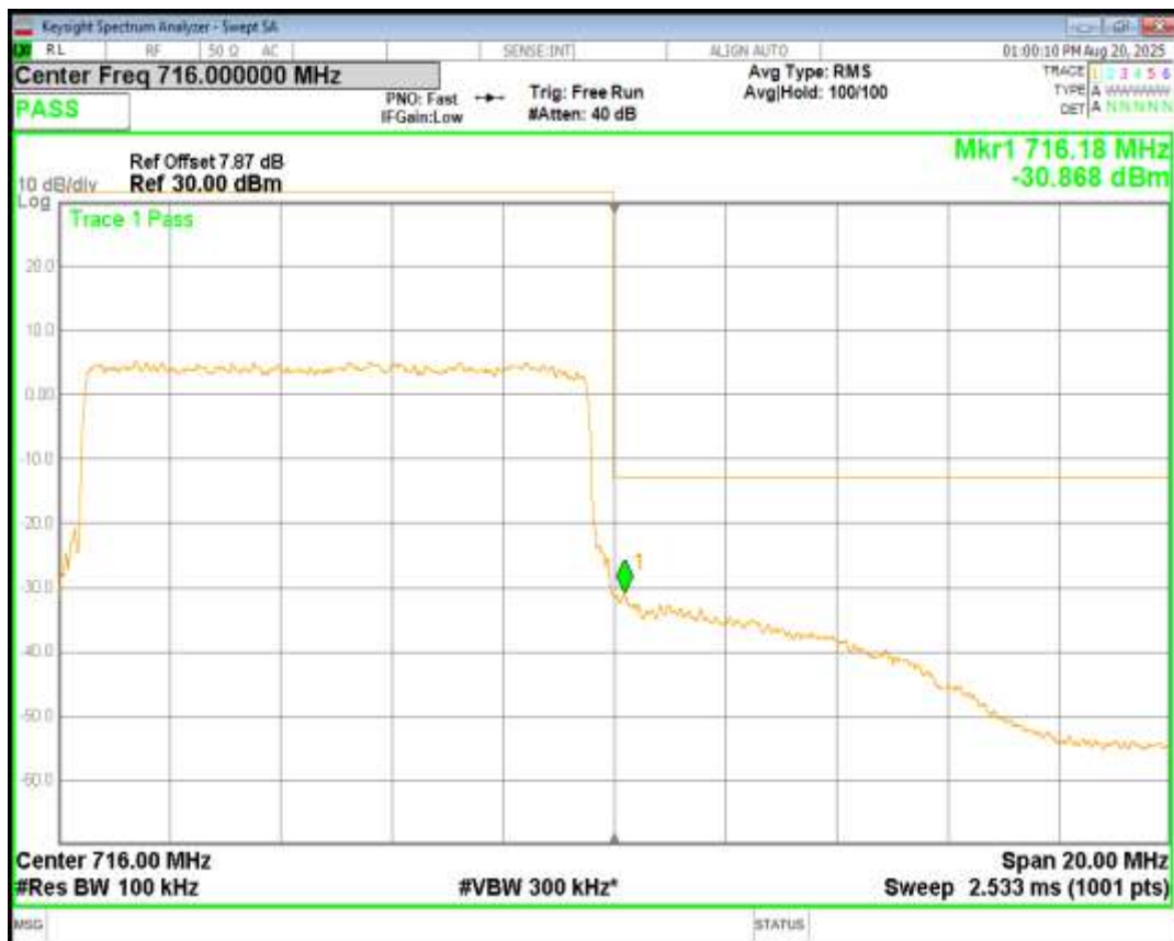
Band2 QPSK BW=1.4MHz Channel=18607 RB Size=6 Position=#0
