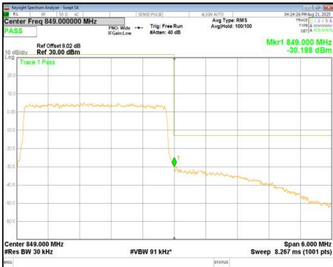
Band5 QPSK BW=5MHz Channel=20425 RB Size=25 Position=#0
