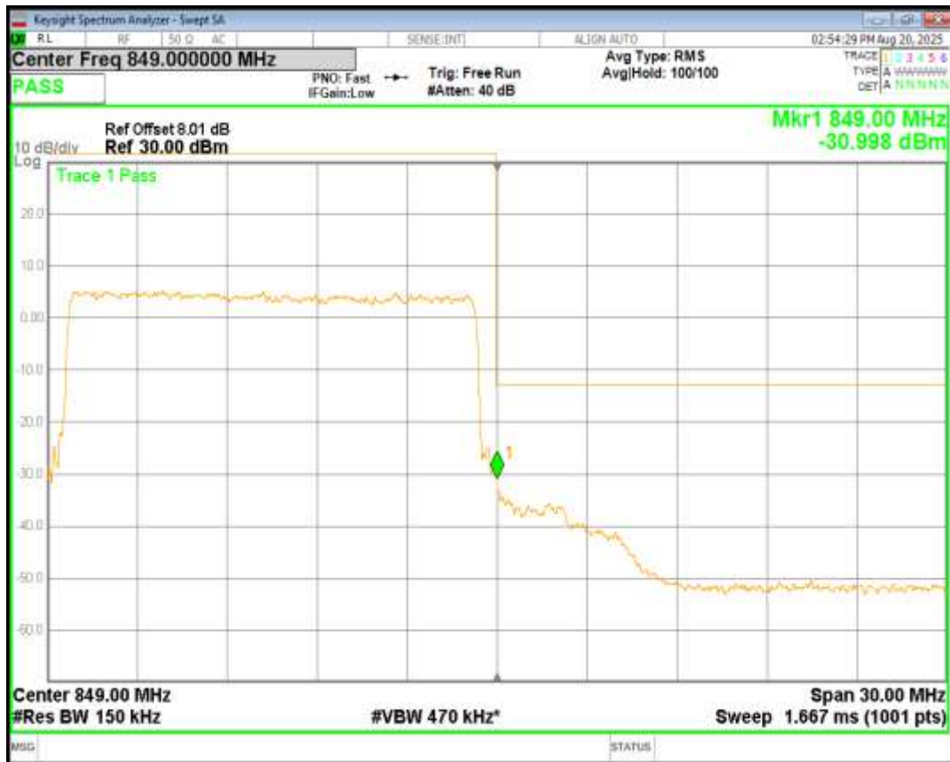
Band26(824-849) 16QAM BW=15MHz Channel=26965 RB Size=75 Position=#0
