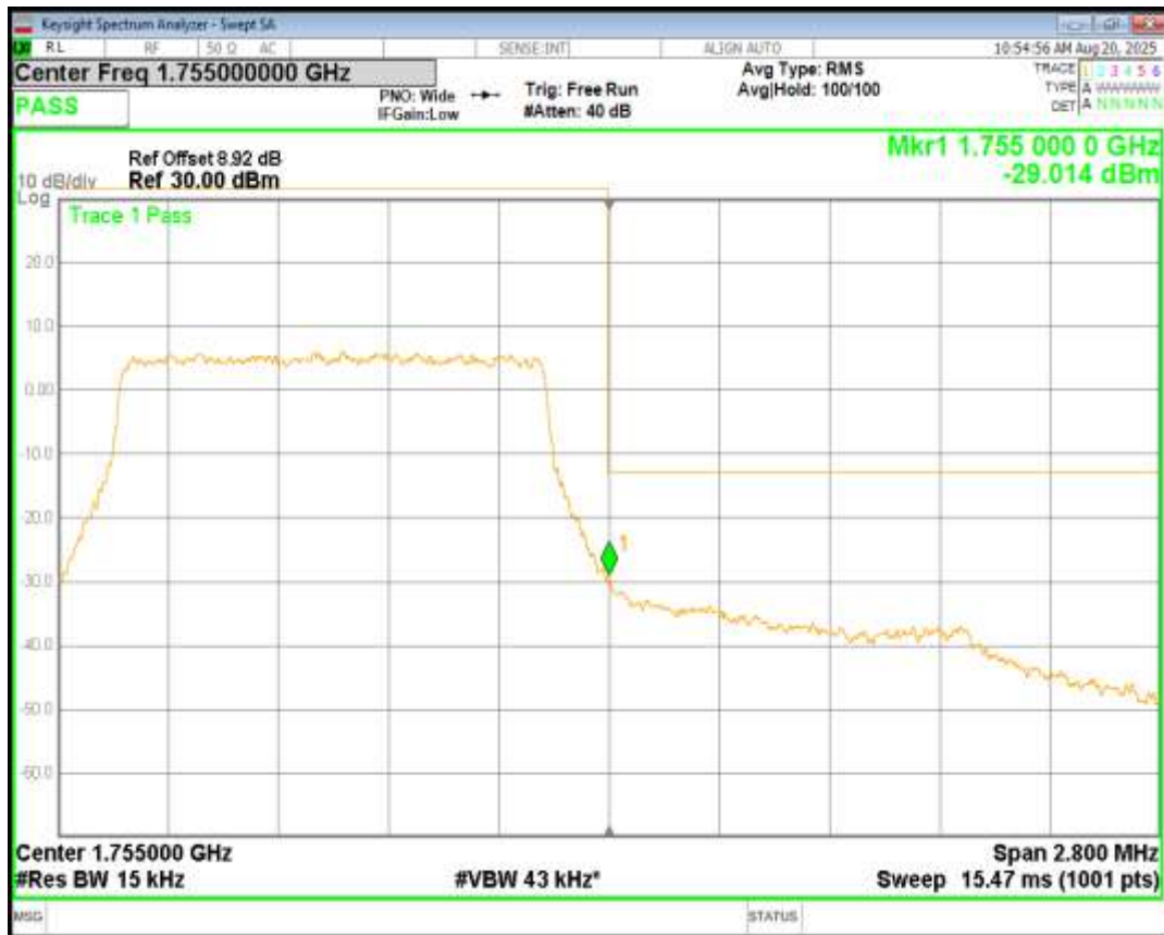
Band4 16QAM BW=1.4MHz Channel=20393 RB Size=6 Position=#0
