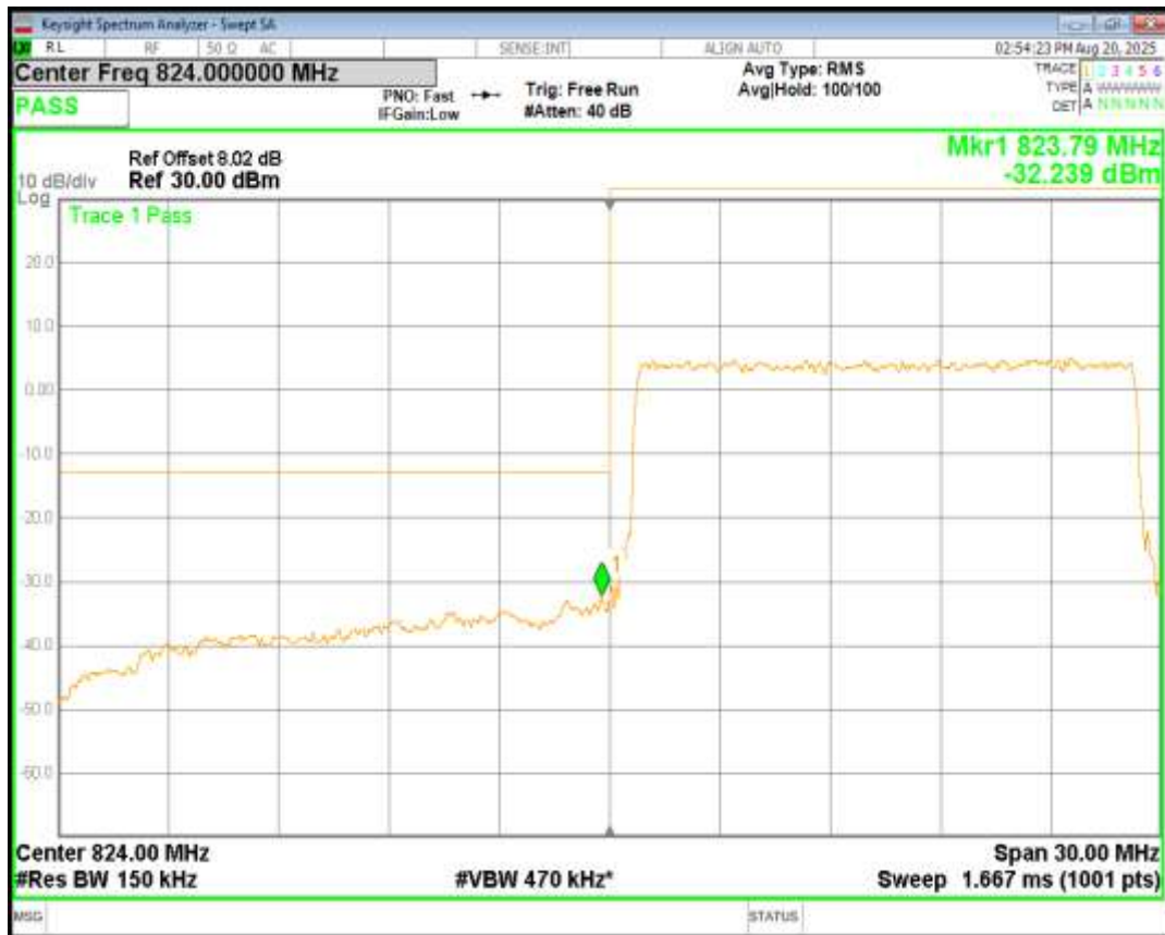
Band26(824-849) 16QAM BW=15MHz Channel=26865 RB Size=75 Position=#0
