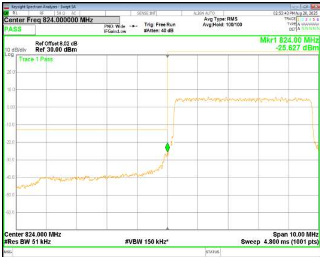
Band26(824-849) 16QAM BW=5MHz Channel=26815 RB Size=25 Position=#0
