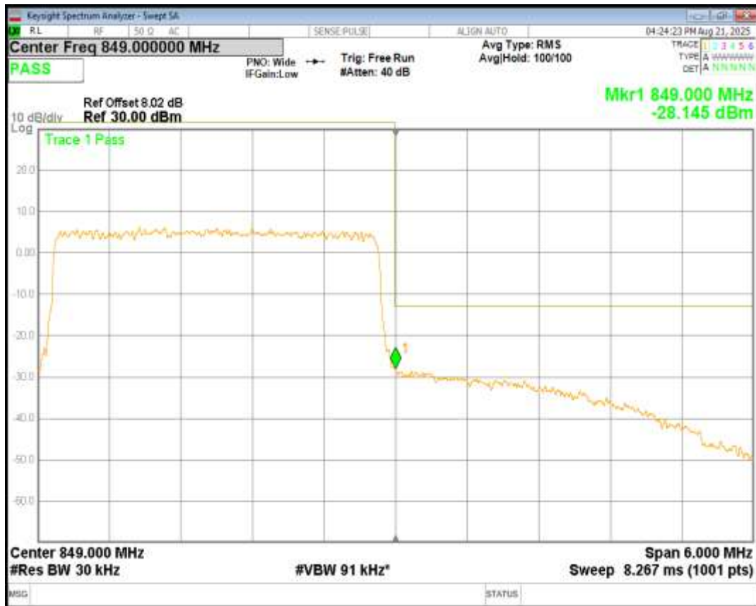
Band5 16QAM BW=3MHz Channel=20635 RB Size=15 Position=#0
