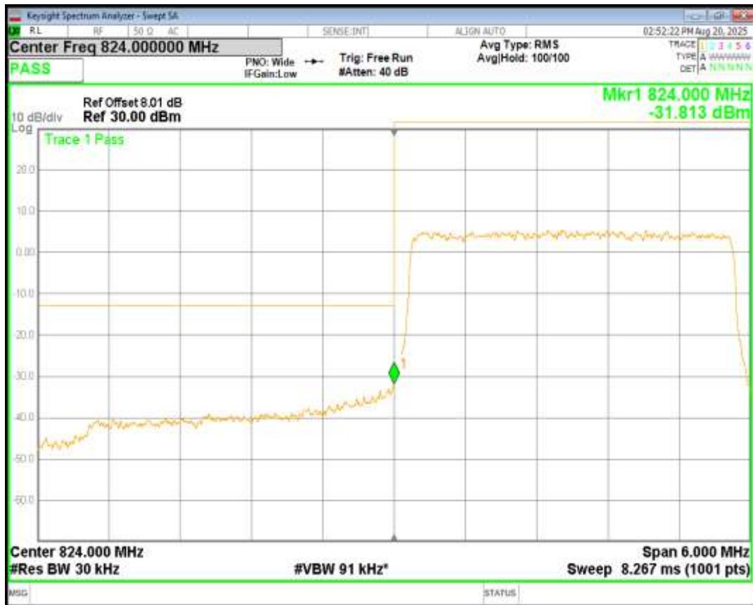
Band26(824-849) 16QAM BW=3MHz Channel=26805 RB Size=15 Position=#0
