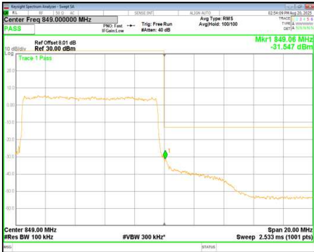
Band26(824-849) 16QAM BW=10MHz Channel=26990 RB Size=50 Position=#0
