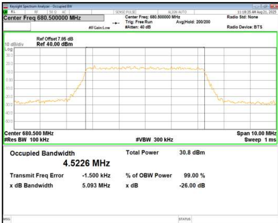
Band71 QPSK BW=5MHz Channel=133447 RB Size=25 Position=#0
