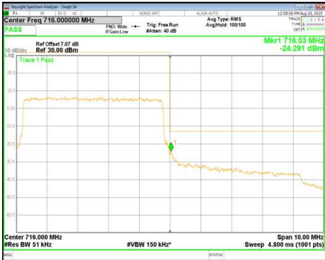
Band17 16QAM BW=5MHz Channel=23825 RB Size=25 Position=#0
