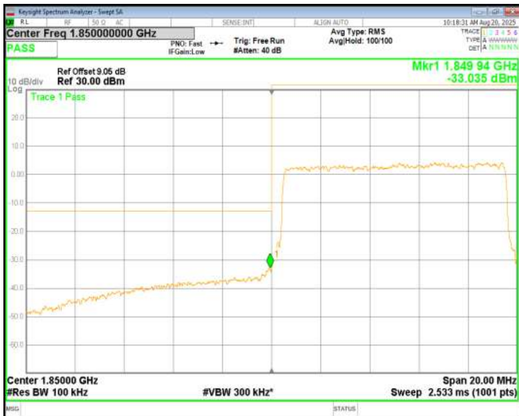
Band2 QPSK BW=10MHz Channel=19150 RB Size=50 Position=#0
