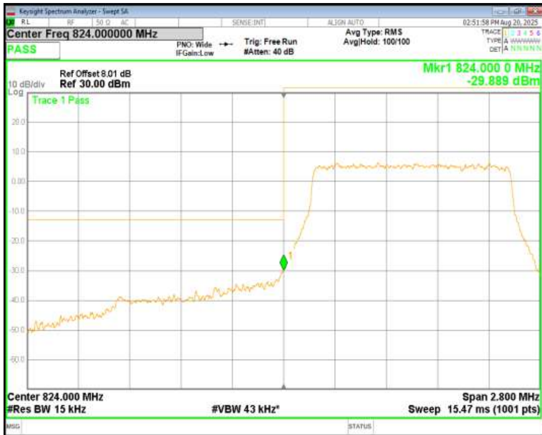
Band26(824-849) 16QAM BW=1.4MHz Channel=26797 RB Size=6 Position=#0
