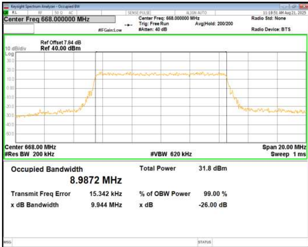
Band71 16QAM BW=10MHz Channel=133172 RB Size=50 Position=#0
