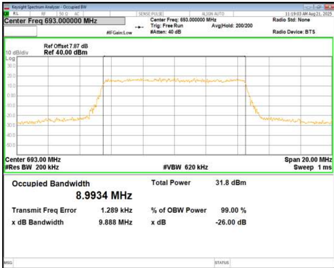
Band71 16QAM BW=10MHz Channel=133422 RB Size=50 Position=#0
