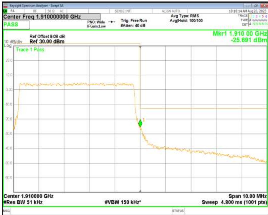
Band2 16QAM BW=5MHz Channel=19175 RB Size=25 Position=#0
