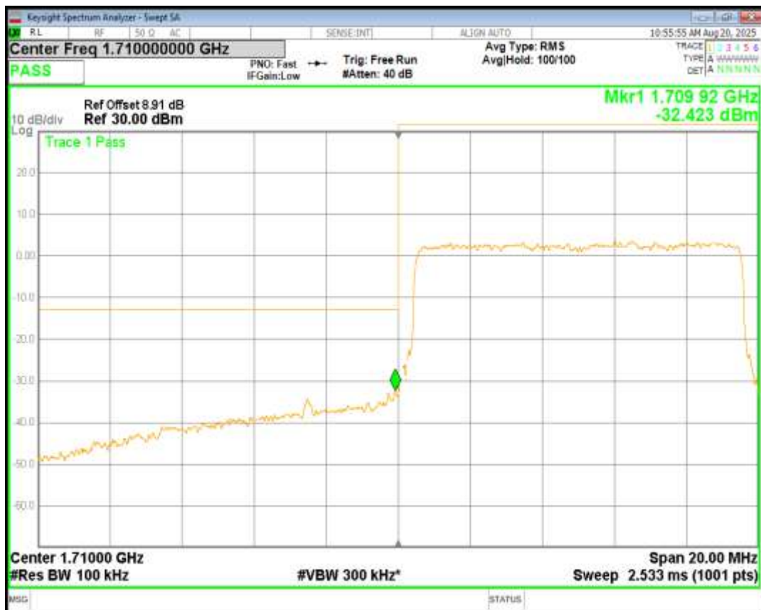
Band4 QPSK BW=10MHz Channel=20350 RB Size=50 Position=#0
