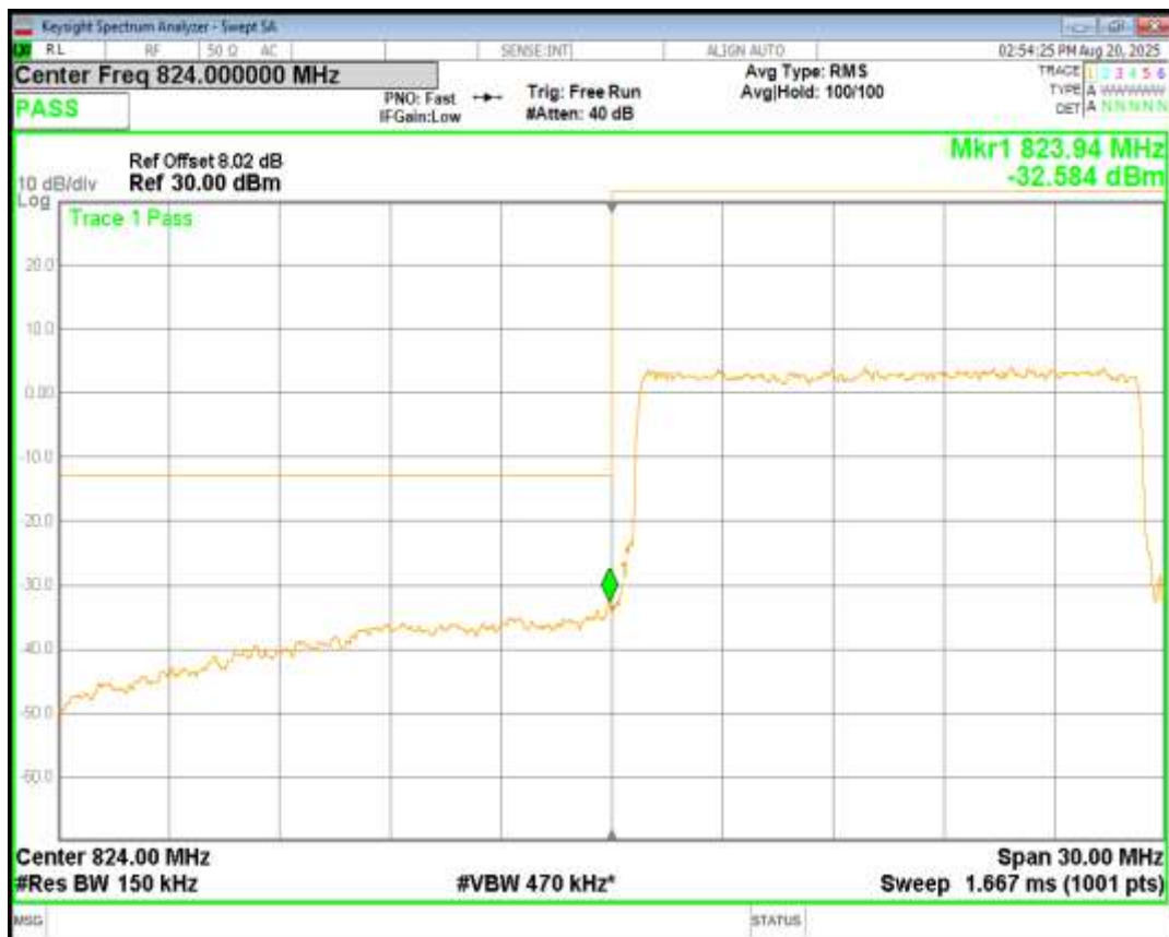
Band26(824-849) QPSK BW=15MHz Channel=26965 RB Size=75 Position=#0
