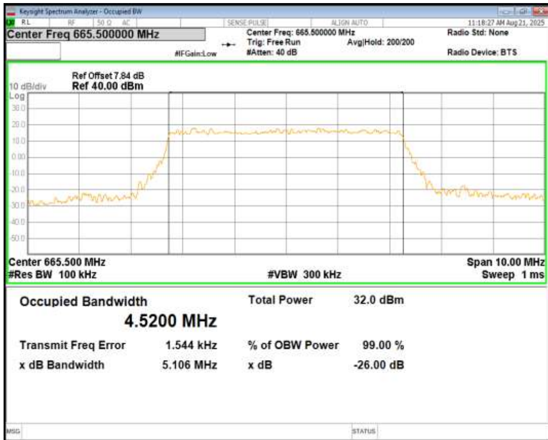
Band71 16QAM BW=5MHz Channel=133147 RB Size=25 Position=#0
