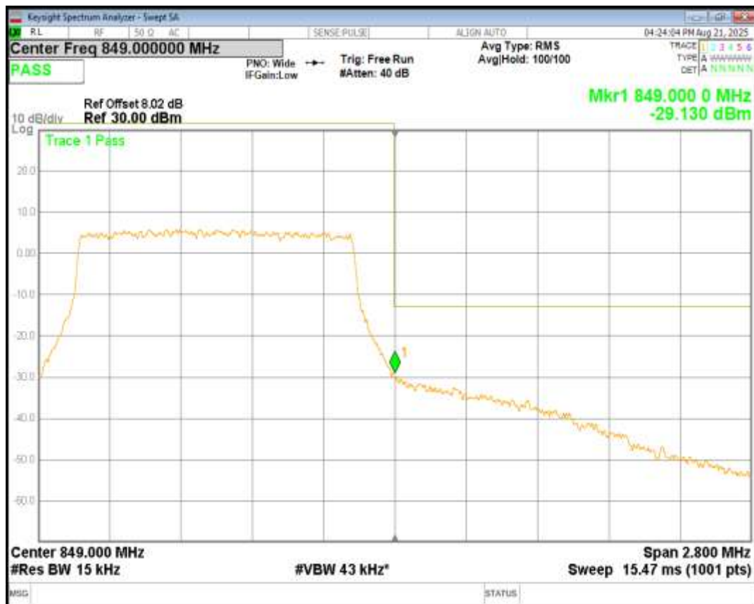
Band5 QPSK BW=3MHz Channel=20415 RB Size=15 Position=#0
