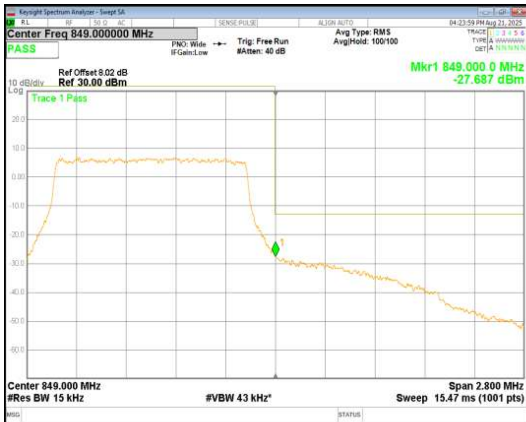
Band5 16QAM BW=1.4MHz Channel=20643 RB Size=6 Position=#0
