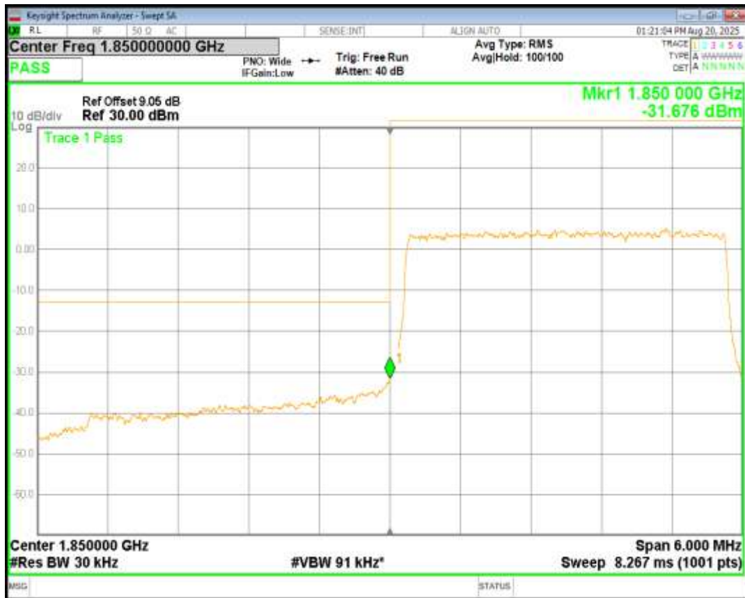
Band25 16QAM BW=3MHz Channel=26055 RB Size=15 Position=#0
