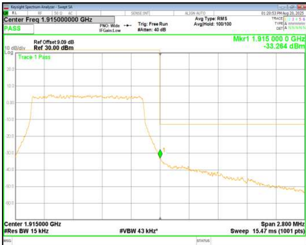
Band25 QPSK BW=3MHz Channel=26055 RB Size=15 Position=#0
