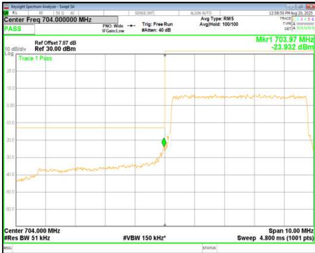
Band17 16QAM BW=5MHz Channel=23755 RB Size=25 Position=#0
