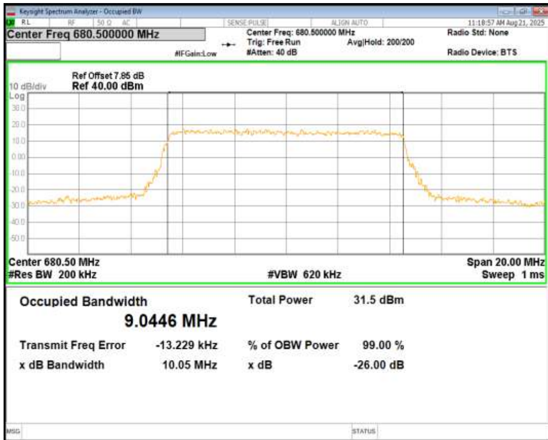
Band71 16QAM BW=10MHz Channel=133297 RB Size=50 Position=#0
