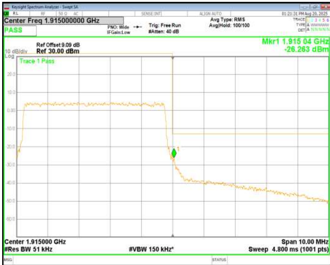
Band25 16QAM BW=5MHz Channel=26665 RB Size=25 Position=#0
