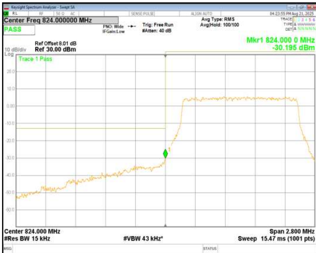
Band5 QPSK BW=1.4MHz Channel=20643 RB Size=6 Position=#0
