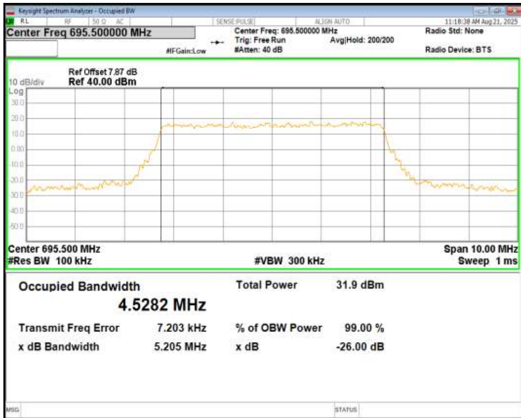
Band71 16QAM BW=5MHz Channel=133447 RB Size=25 Position=#0
