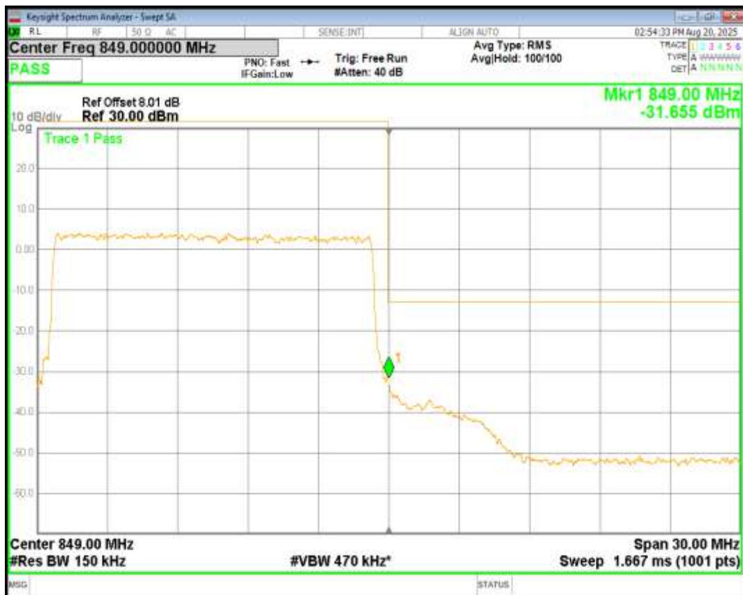
Band4 QPSK BW=1.4MHz Channel=19957 RB Size=6 Position=#0
