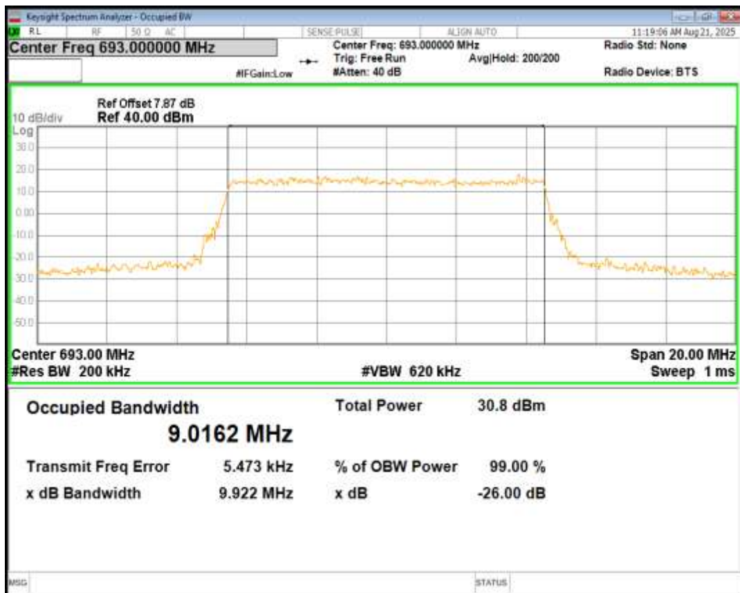
Band71 QPSK BW=15MHz Channel=133197 RB Size=75 Position=#0
