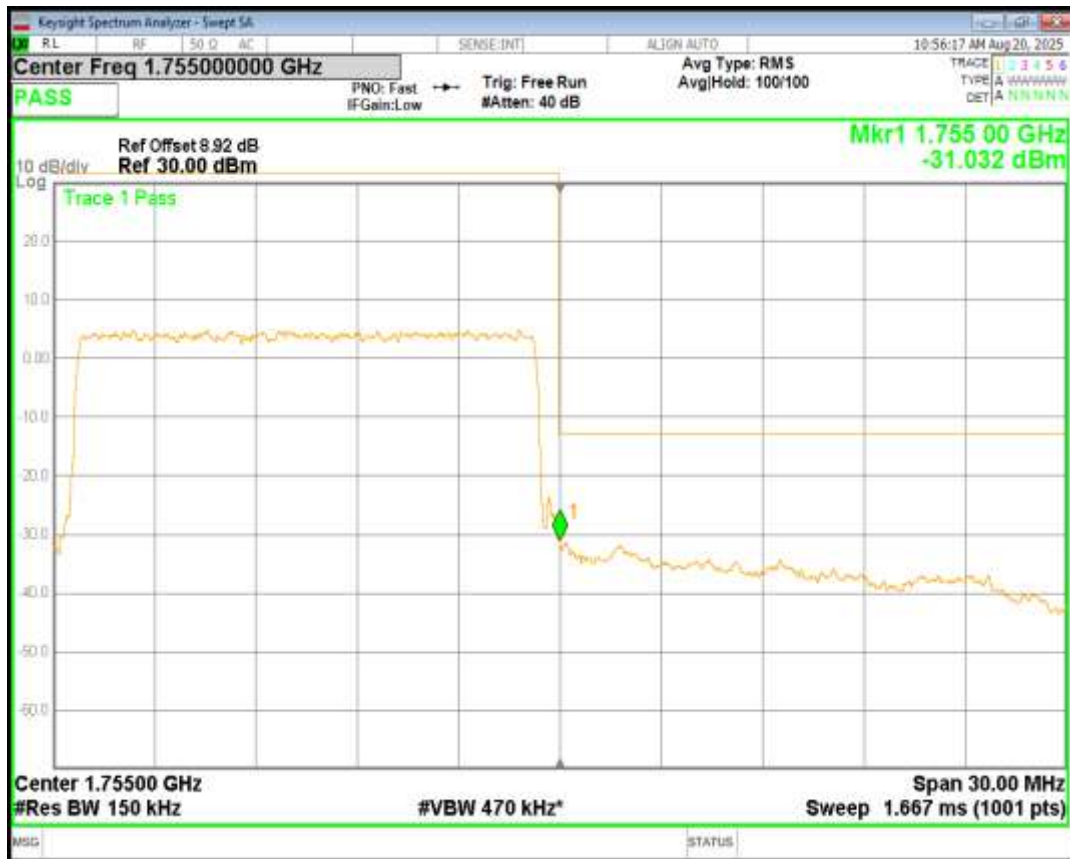
Band4 16QAM BW=15MHz Channel=20325 RB Size=75 Position=#0
