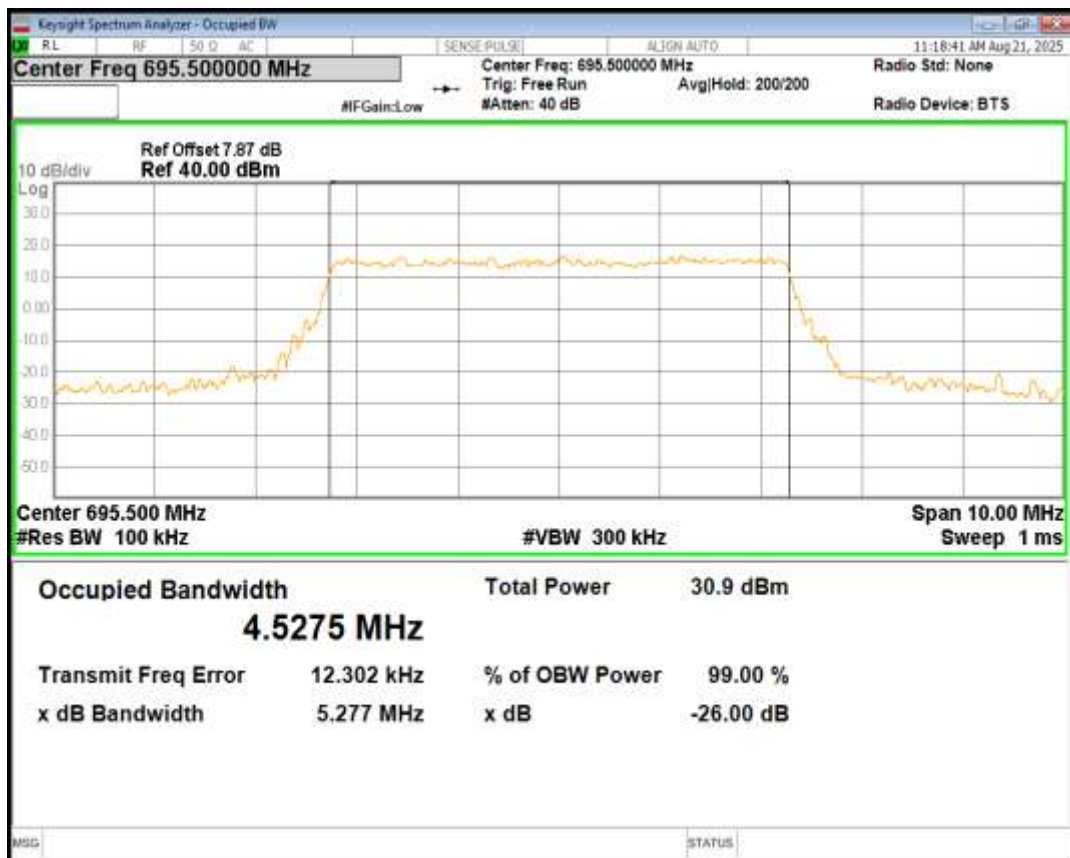
Band71 QPSK BW=10MHz Channel=133172 RB Size=50 Position=#0
