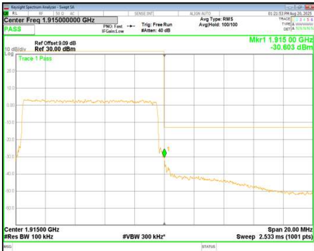
Band25 QPSK BW=15MHz Channel=26115 RB Size=75 Position=#0
