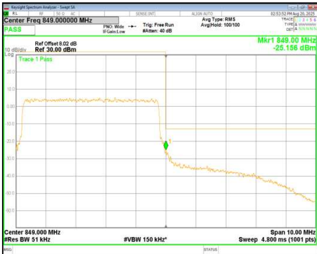
Band26(824-849) QPSK BW=10MHz Channel=26840 RB Size=50 Position=#0
