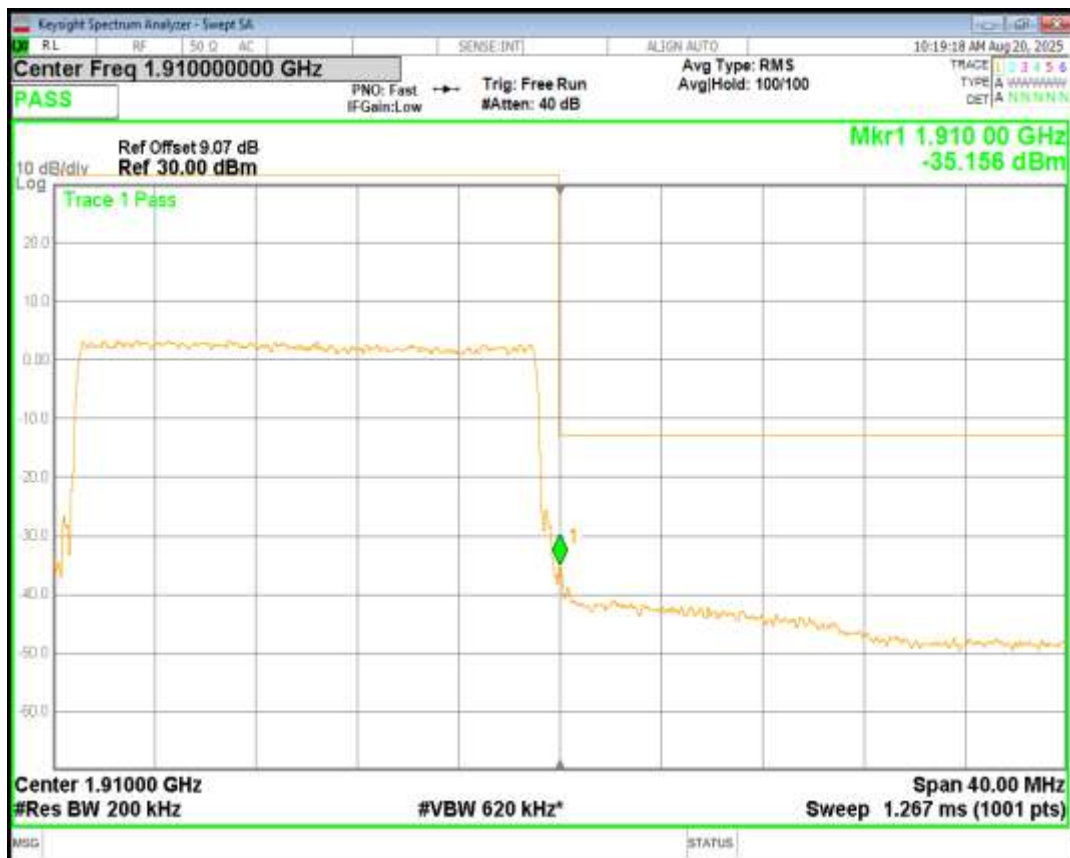
Band25 QPSK BW=1.4MHz Channel=26047 RB Size=6 Position=#0
