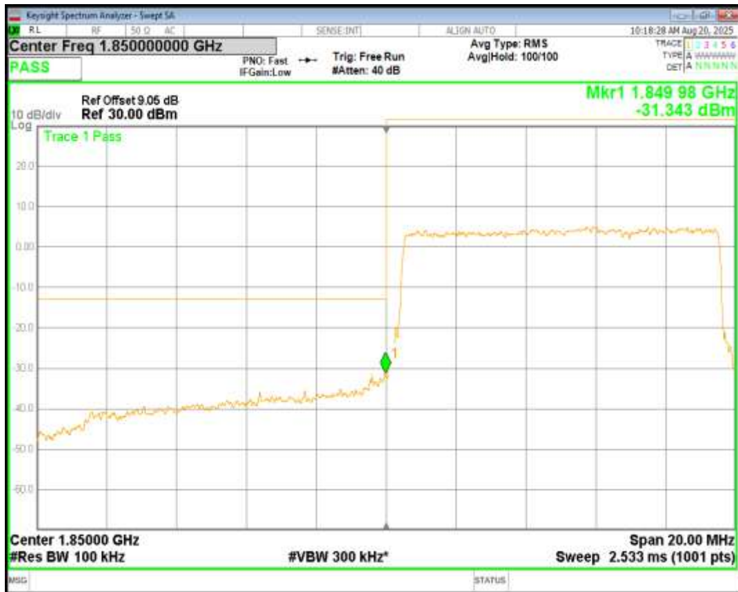
Band2 16QAM BW=10MHz Channel=18650 RB Size=50 Position=#0
