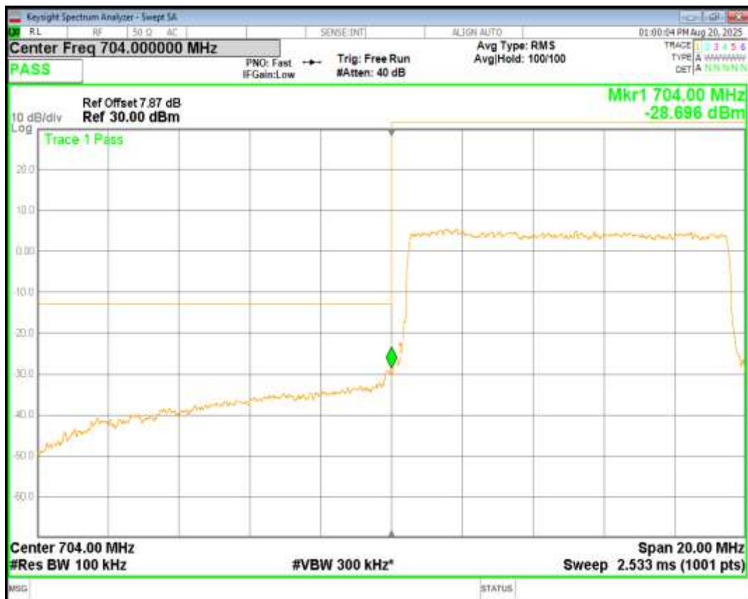
Band17 QPSK BW=10MHz Channel=23800 RB Size=50 Position=#0
