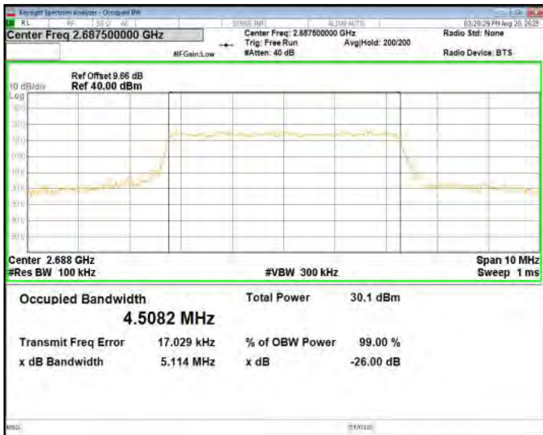
Band41 QPSK BW=10MHz Channel=39700 RB Size=50 Position=#0
