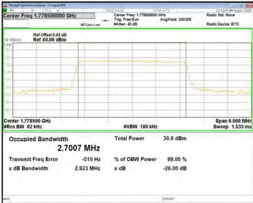
Band66 16QAM BW=3MHz Channel=132657 RB Size=15 Position=#0
