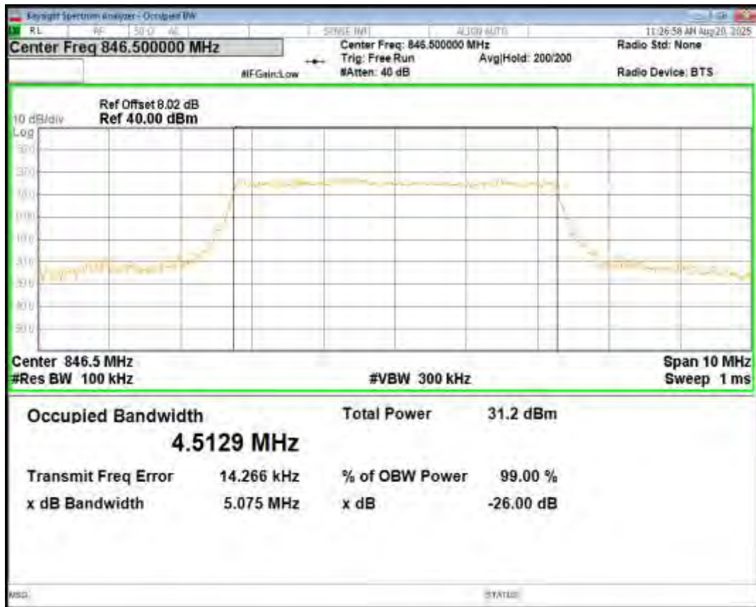
Band5 16QAM BW=5MHz Channel=20625 RB Size=25 Position=#0
