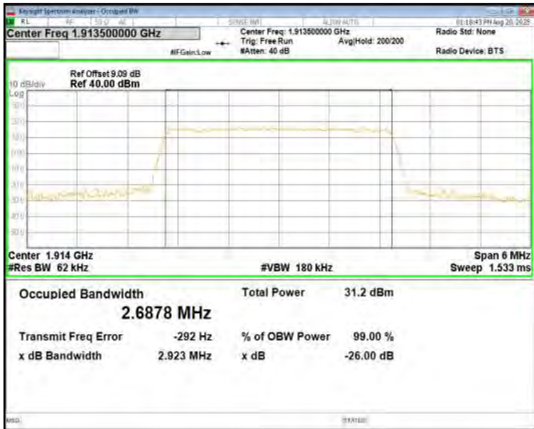
Band25 16QAM BW=3MHz Channel=26675 RB Size=15 Position=#0
