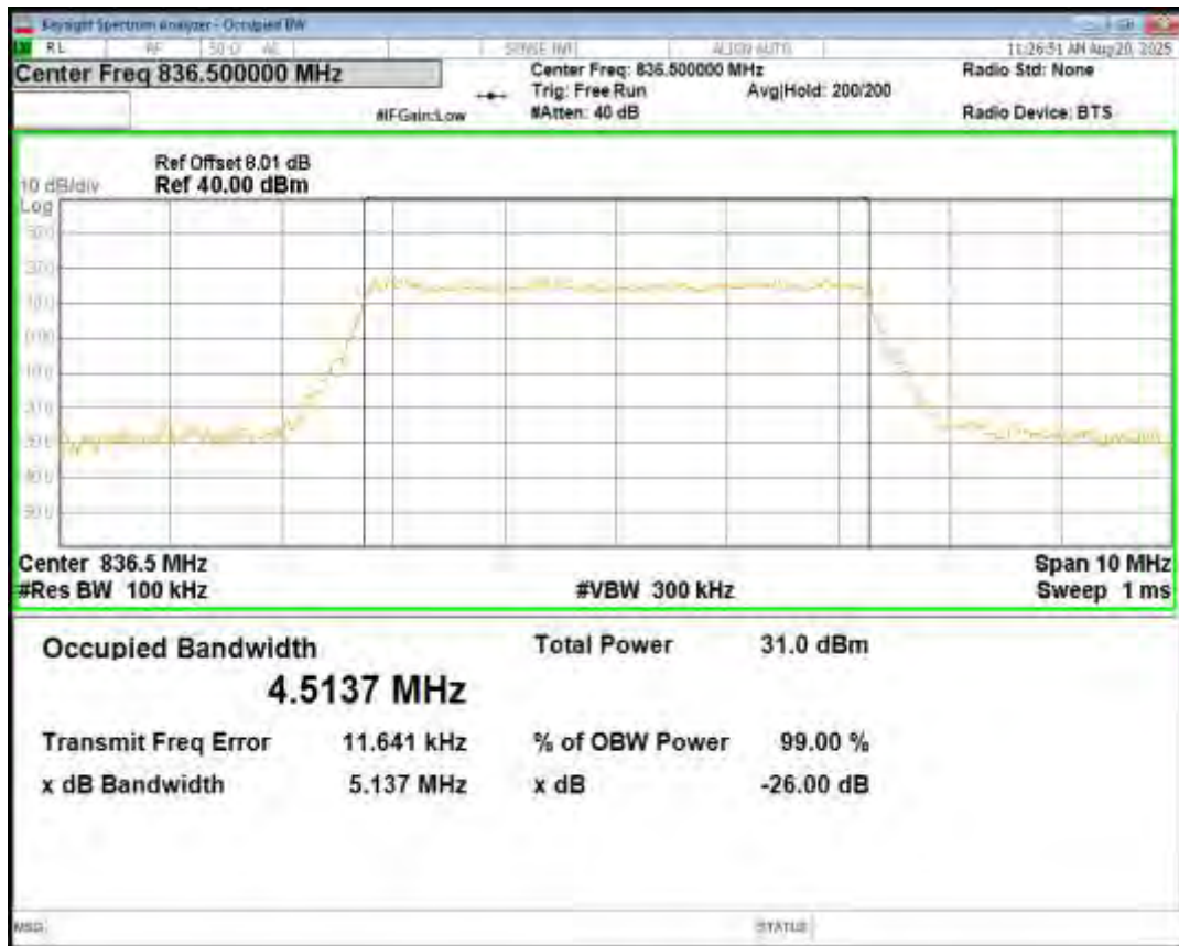
Band5 16QAM BW=5MHz Channel=20525 RB Size=25 Position=#0
