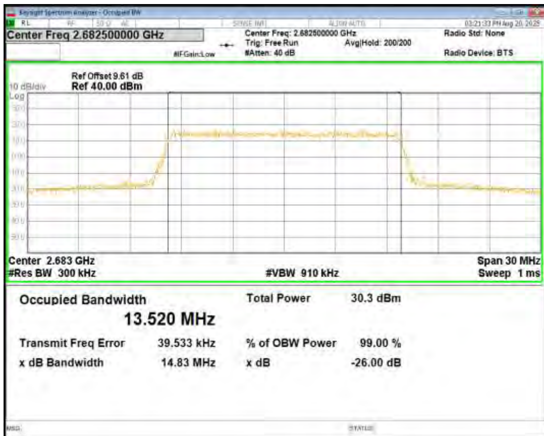
Band41 QPSK BW=20MHz Channel=39750 RB Size=100 Position=#0
