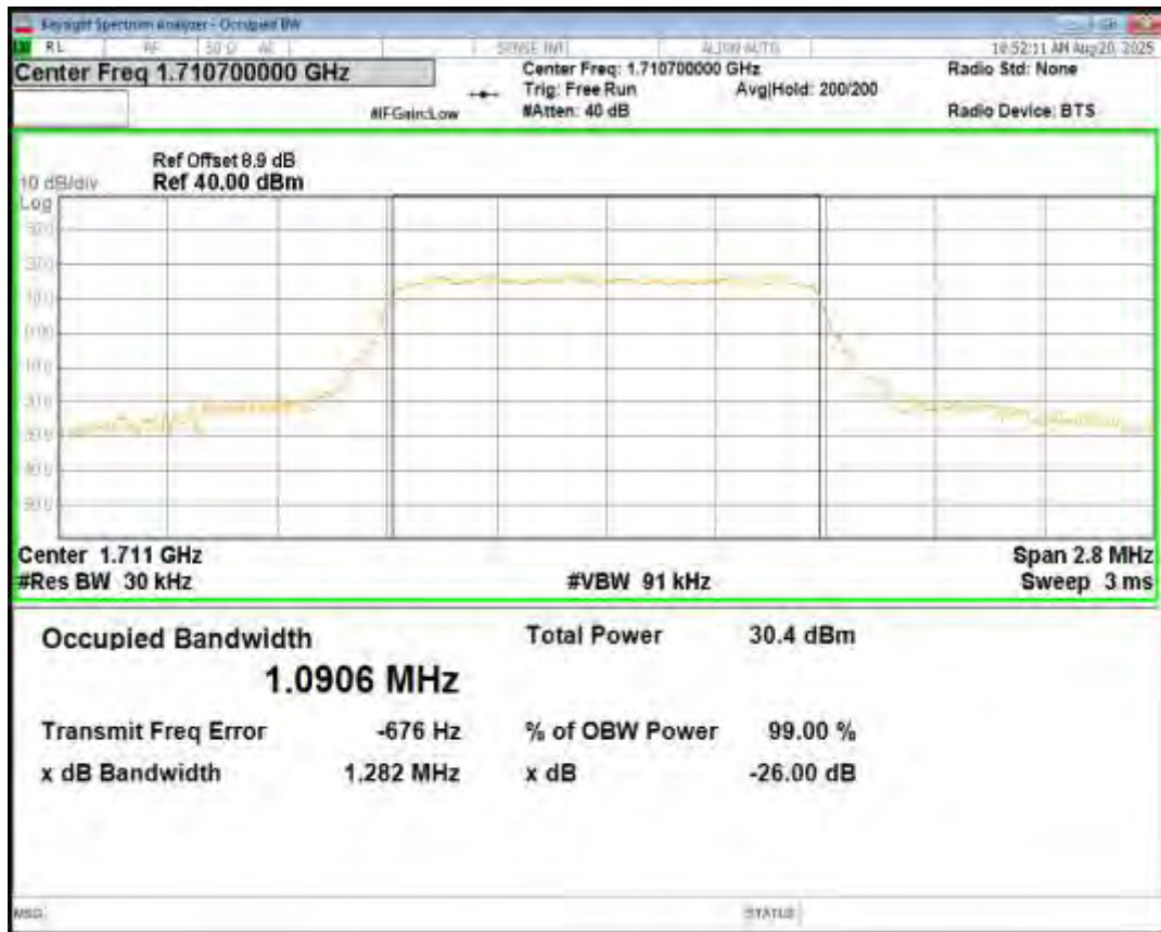
Band4 16QAM BW=1.4MHz Channel=19957 RB Size=6 Position=#0
