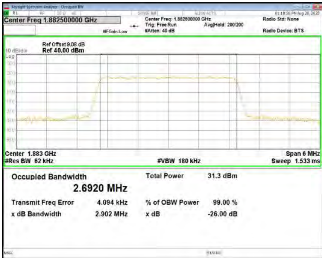
Band25 16QAM BW=3MHz Channel=26365 RB Size=15 Position=#0
