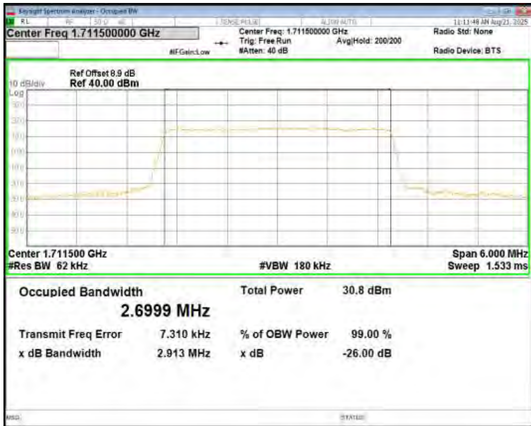
Band66 16QAM BW=3MHz Channel=131987 RB Size=15 Position=#0
