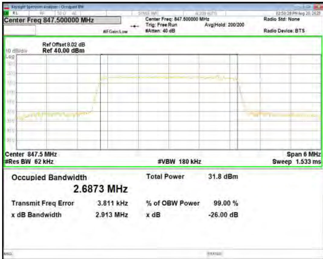
Band26(824-849) 16QAM BW=3MHz Channel=27025 RB Size=15 Position=#0
