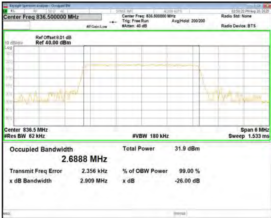
Band26(824-849) 16QAM BW=3MHz Channel=26915 RB Size=15 Position=#0
