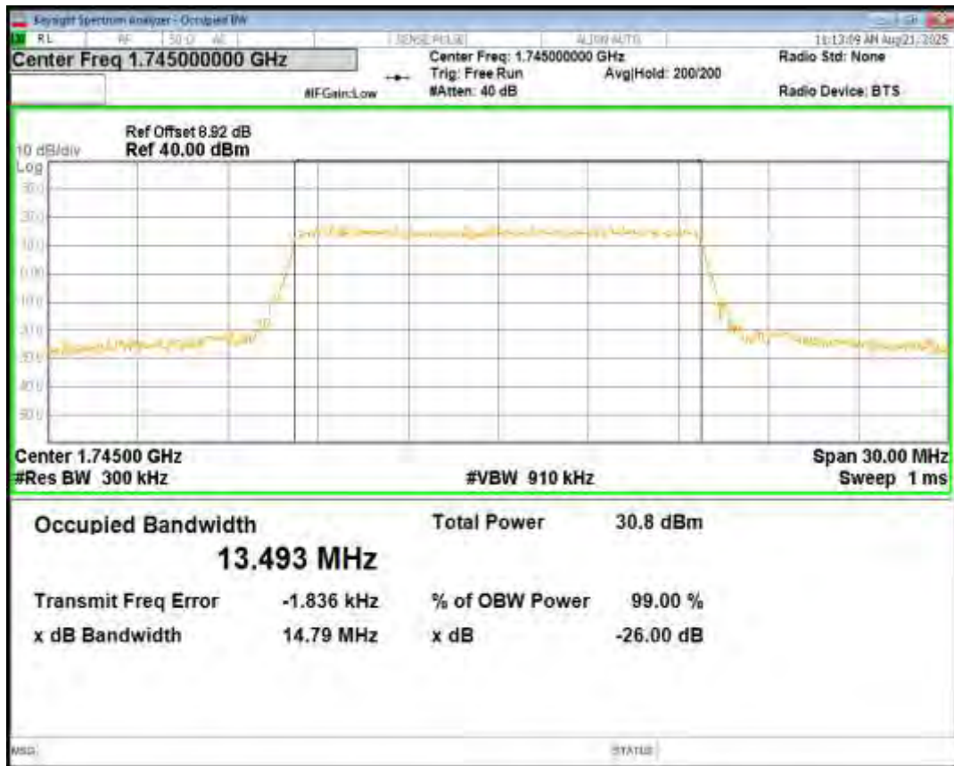
Band66 16QAM BW=15MHz Channel=132322 RB Size=75 Position=#0
