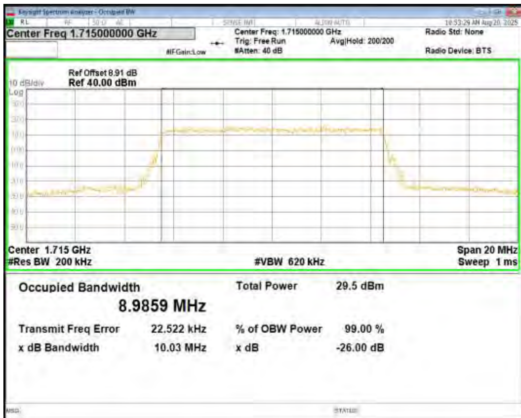
Band4 QPSK BW=10MHz Channel=20175 RB Size=50 Position=#0
