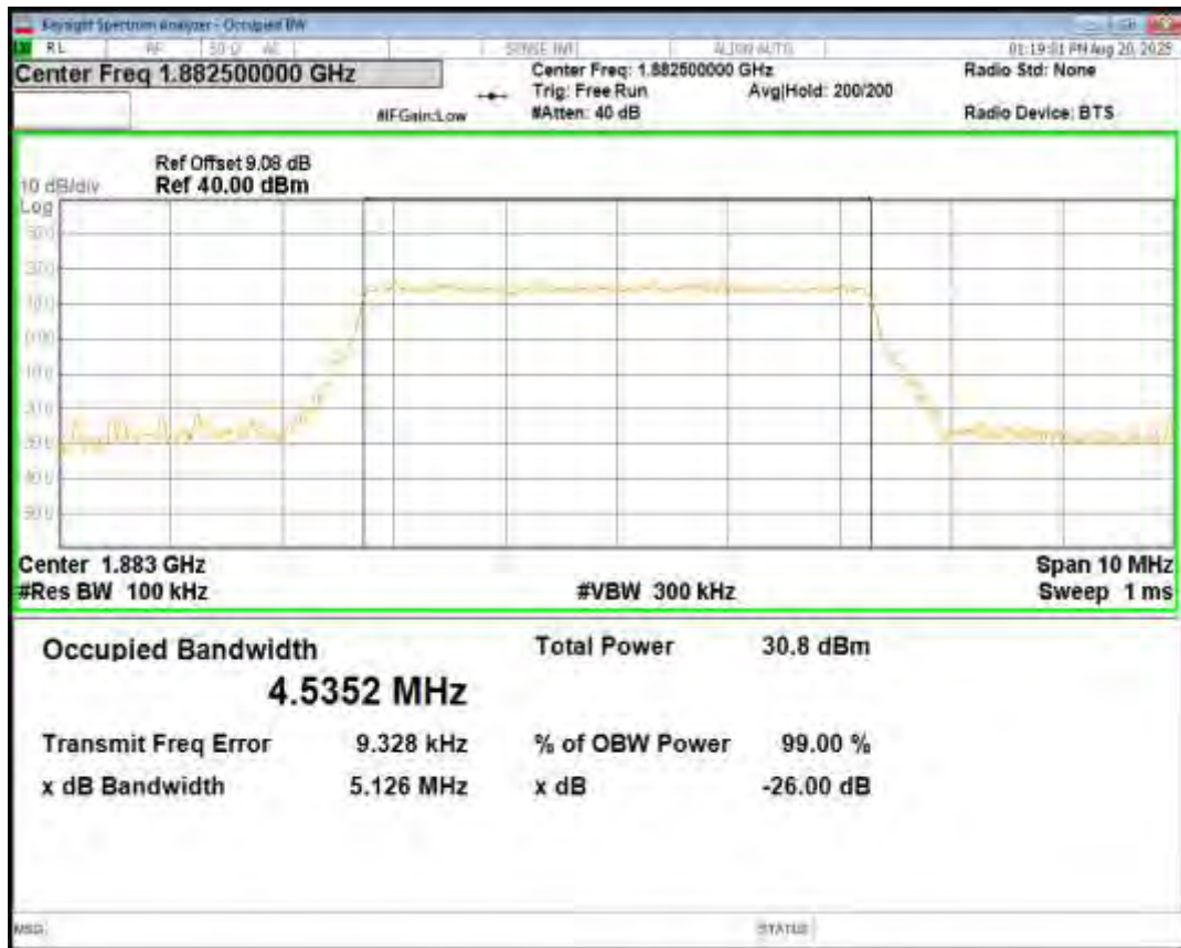
Band25 16QAM BW=5MHz Channel=26365 RB Size=25 Position=#0
