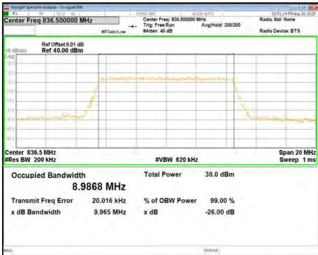
Band26(824-849) QPSK BW=10MHz Channel=26990 RB Size=50 Position=#0
