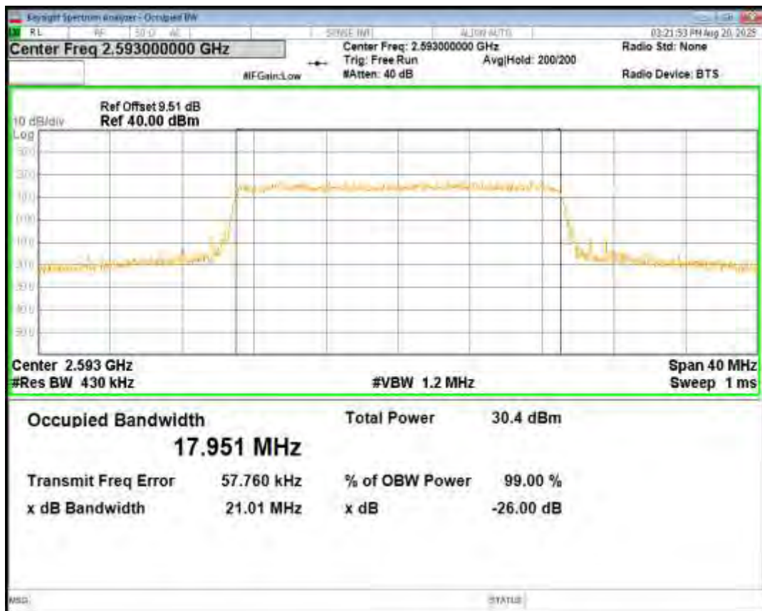
Band41 QPSK BW=20MHz Channel=41490 RB Size=100 Position=#0
