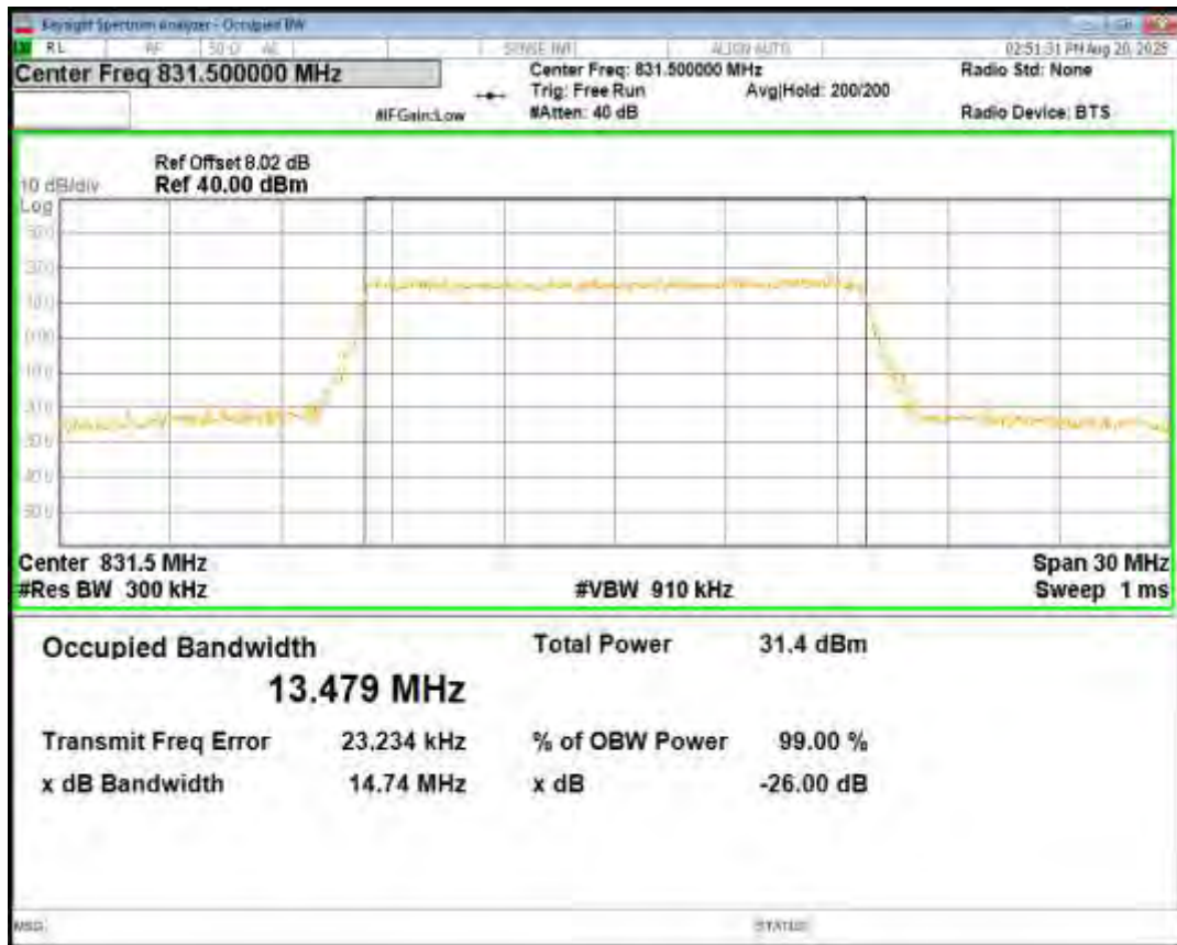
Band26(824-849) 16QAM BW=15MHz Channel=26865 RB Size=75 Position=#0
