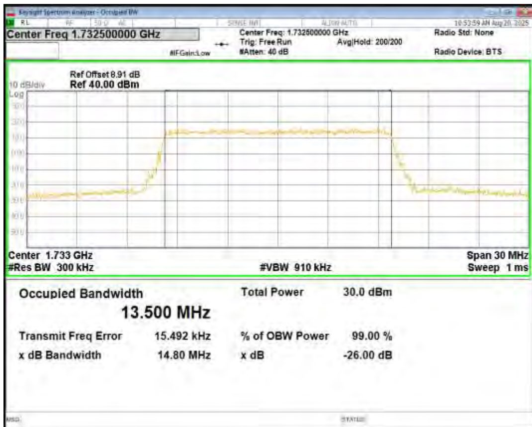
Band4 QPSK BW=15MHz Channel=20325 RB Size=75 Position=#0
