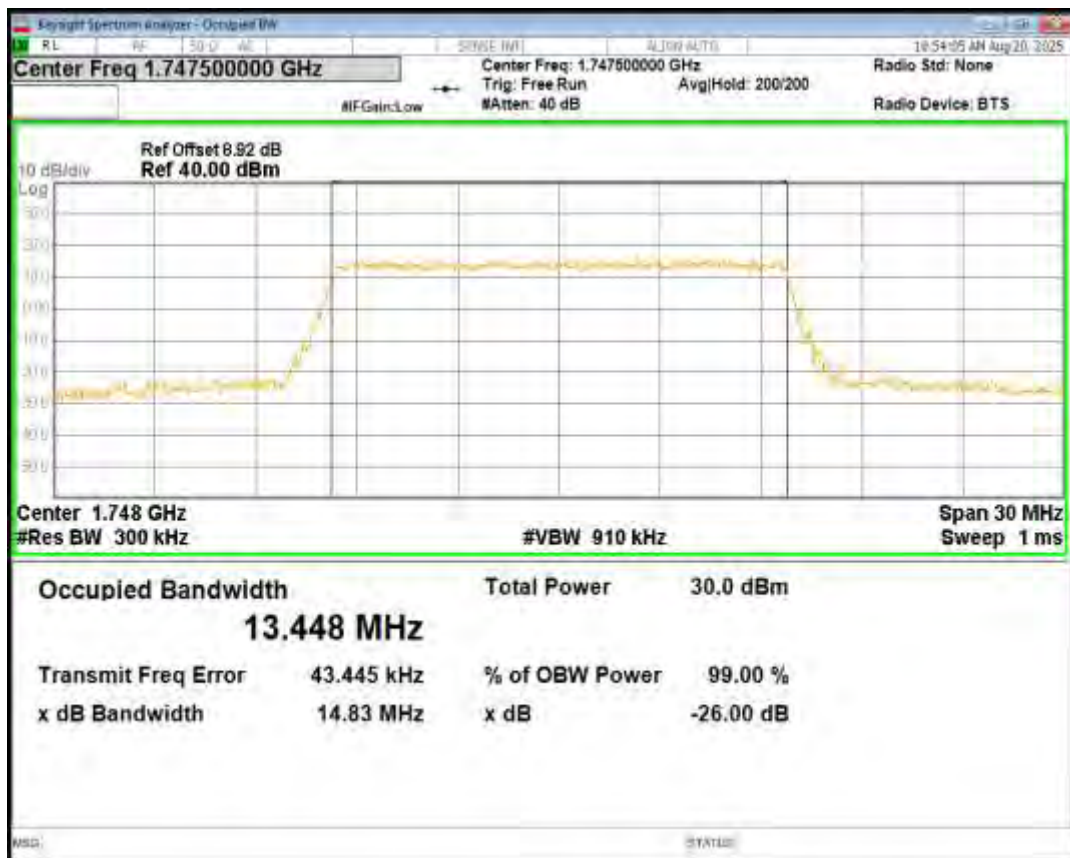
Band4 QPSK BW=20MHz Channel=20050 RB Size=100 Position=#0
