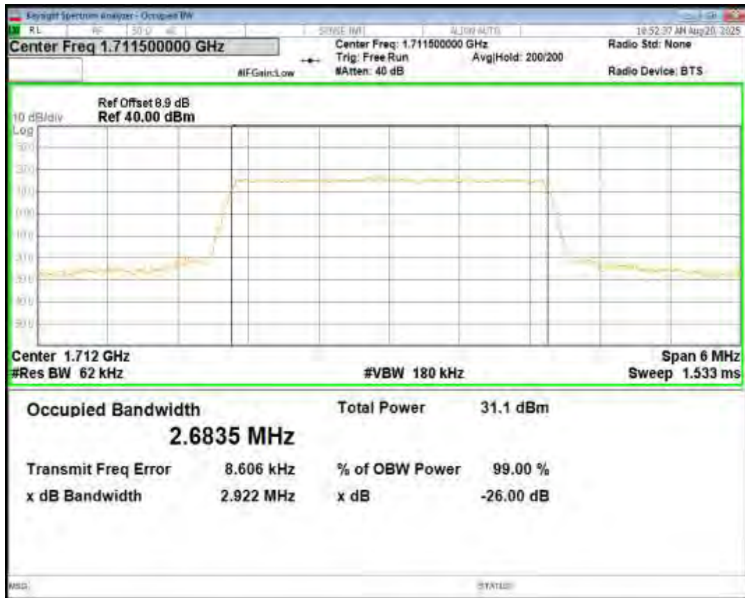
Band4 16QAM BW=3MHz Channel=19965 RB Size=15 Position=#0
