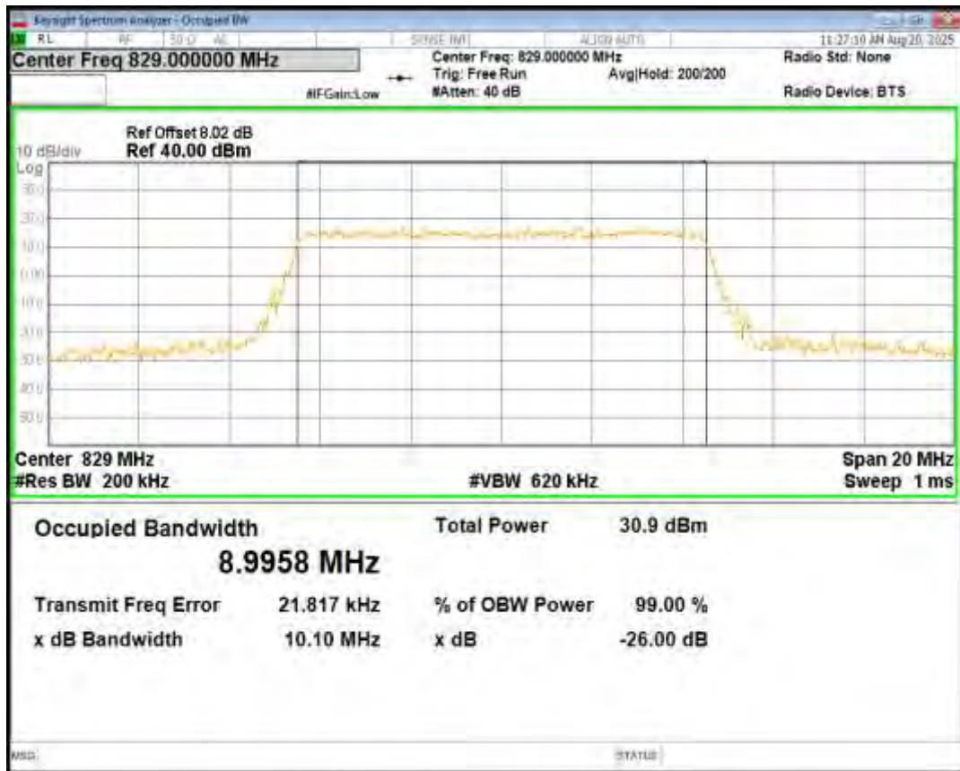
Band5 16QAM BW=10MHz Channel=20450 RB Size=50 Position=#0
