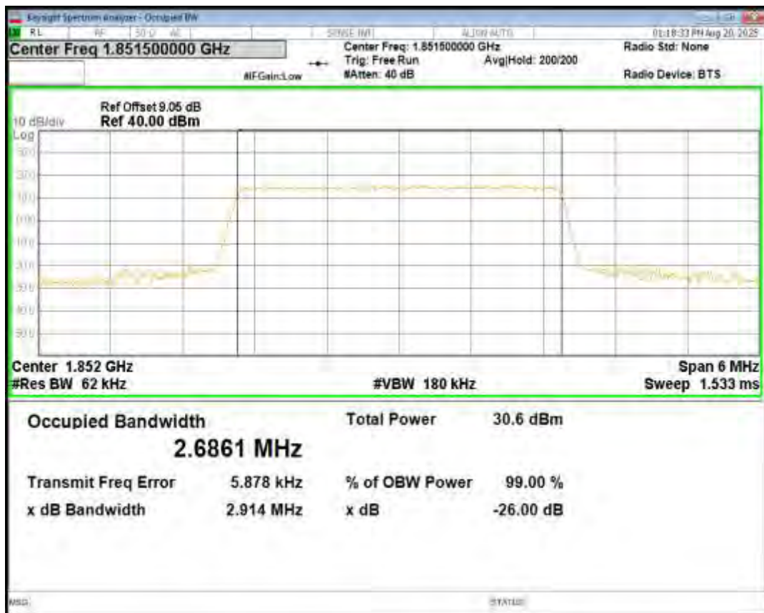
Band25 QPSK BW=3MHz Channel=26365 RB Size=15 Position=#0
