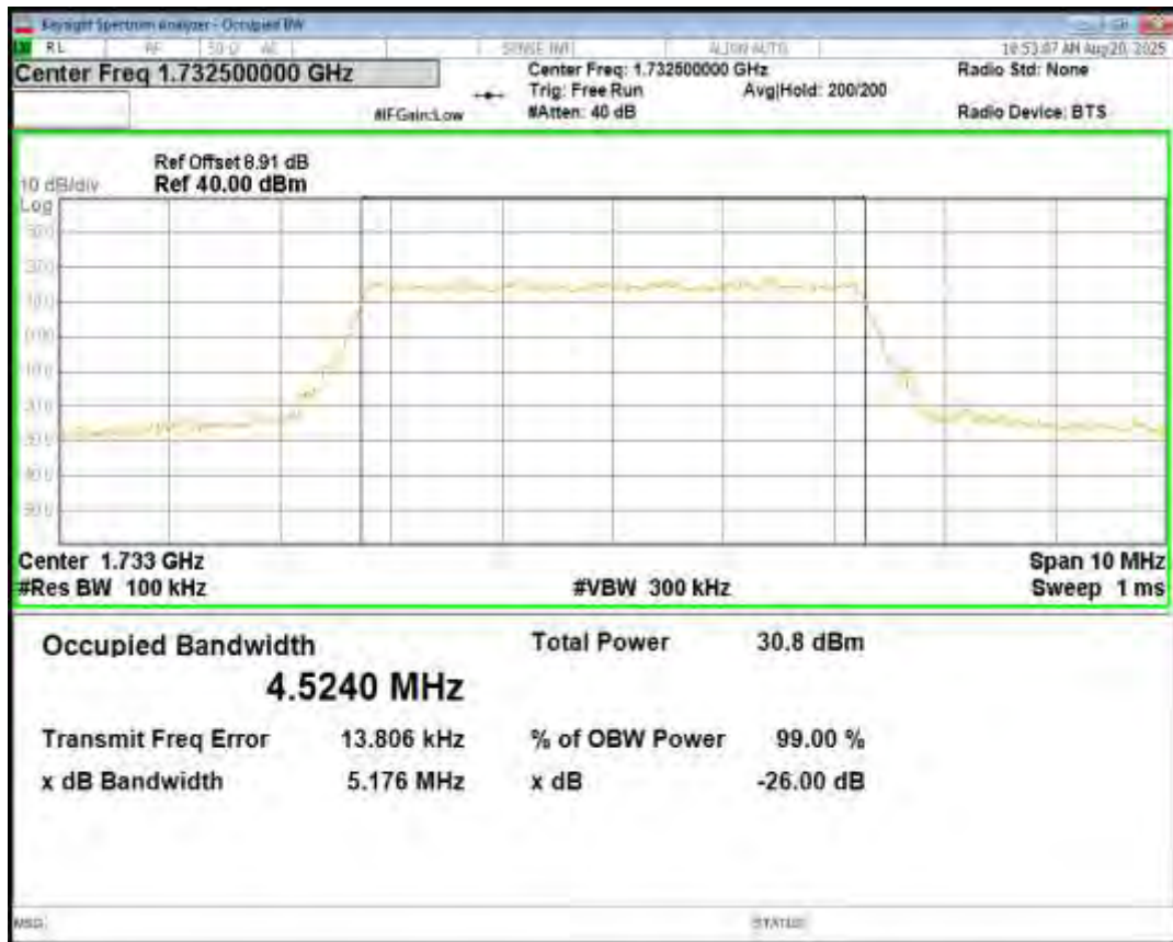
Band4 16QAM BW=5MHz Channel=20175 RB Size=25 Position=#0
