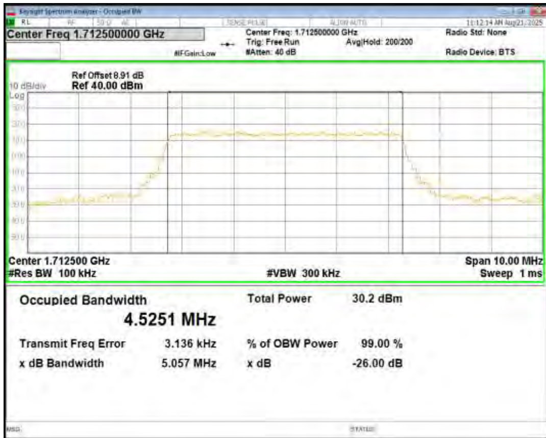
Band66 16QAM BW=5MHz Channel=131997 RB Size=25 Position=#0
