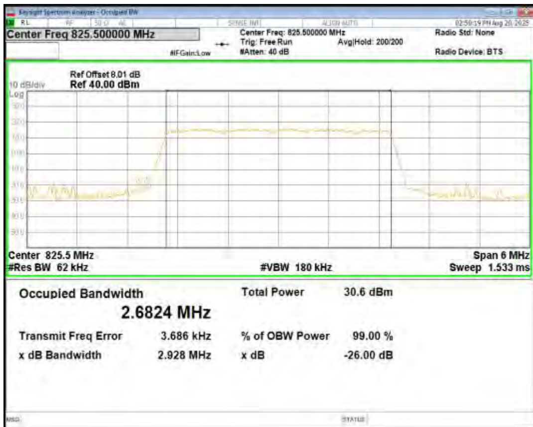
Band26(824-849) QPSK BW=3MHz Channel=26915 RB Size=15 Position=#0
