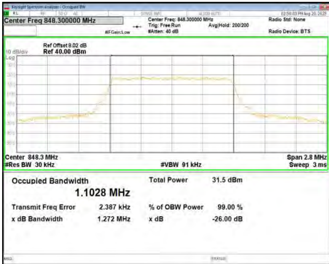
Band26(824-849) 16QAM BW=1.4MHz Channel=27033 RB Size=6 Position=#0
