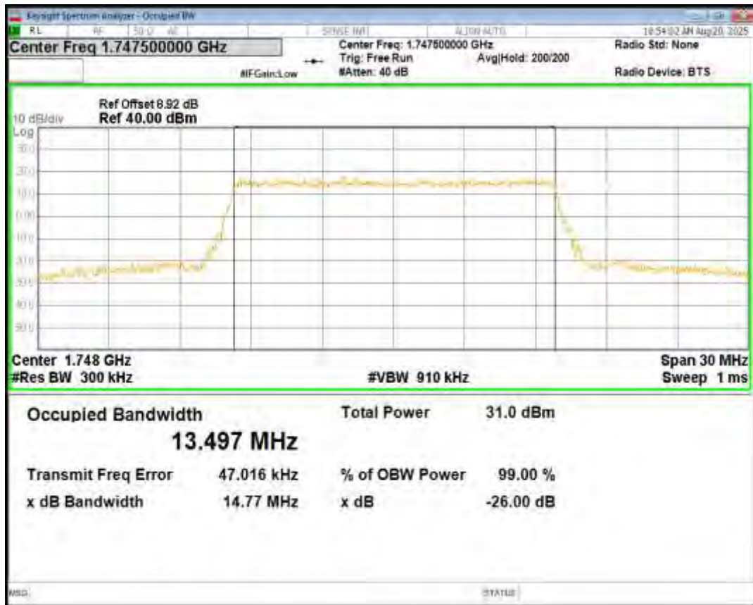
Band4 16QAM BW=15MHz Channel=20325 RB Size=75 Position=#0
