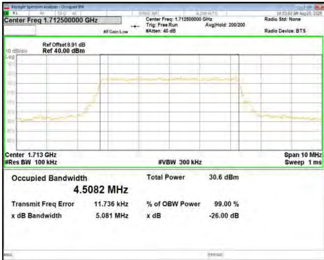
Band4 16QAM BW=5MHz Channel=19975 RB Size=25 Position=#0
