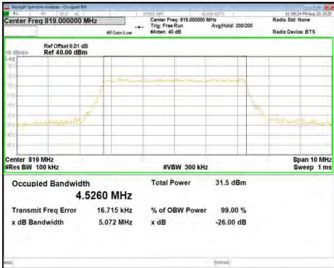
Band26(814-824) 16QAM BW=5MHz Channel=26740 RB Size=25 Position=#0
