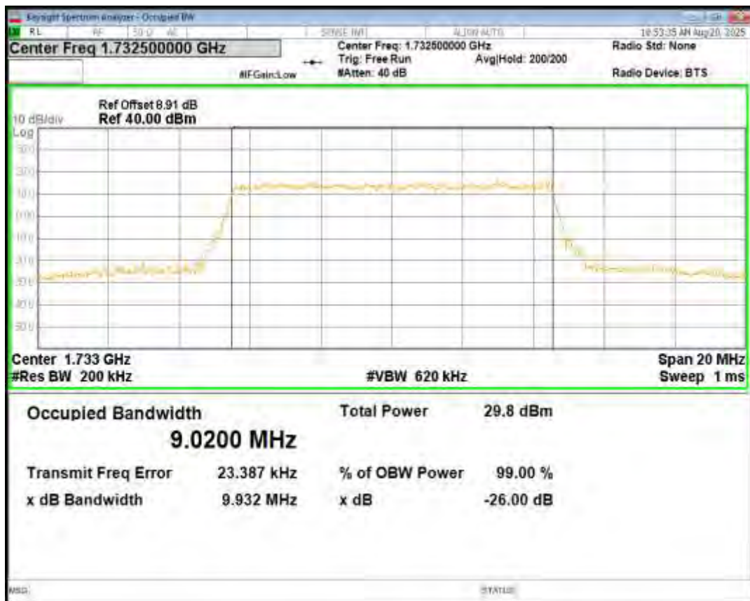
Band4 QPSK BW=10MHz Channel=20350 RB Size=50 Position=#0
