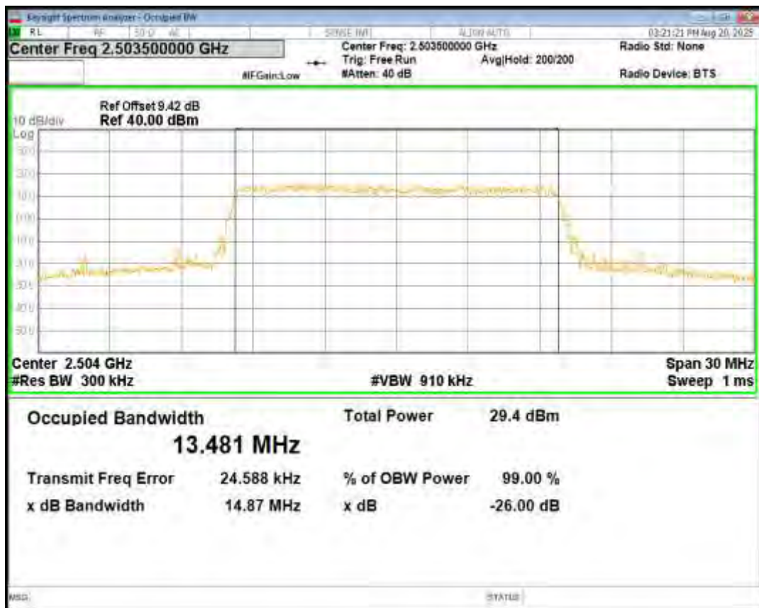
Band41 QPSK BW=15MHz Channel=40620 RB Size=75 Position=#0
