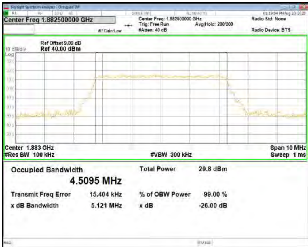
Band25 QPSK BW=5MHz Channel=26665 RB Size=25 Position=#0
