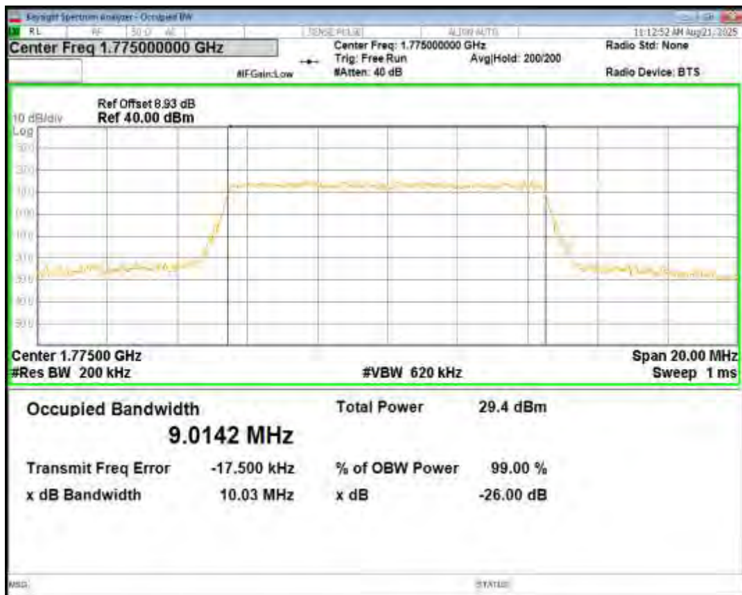
Band66 QPSK BW=15MHz Channel=132047 RB Size=75 Position=#0
