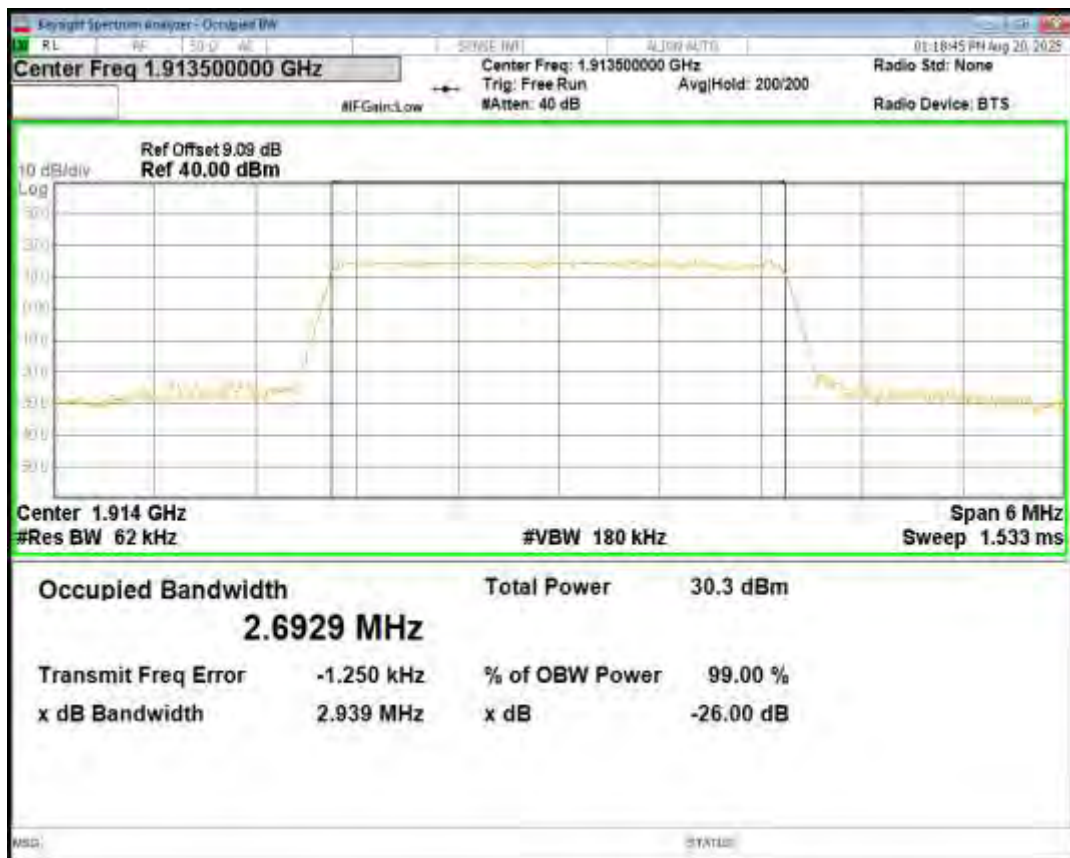
Band25 QPSK BW=5MHz Channel=26065 RB Size=25 Position=#0
