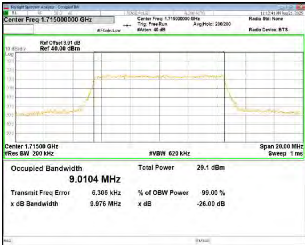
Band66 QPSK BW=10MHz Channel=132322 RB Size=50 Position=#0
