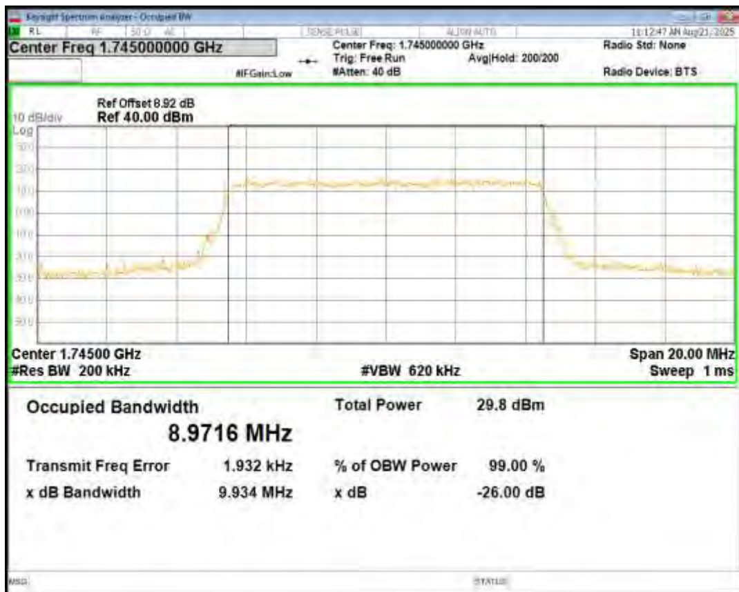
Band66 QPSK BW=10MHz Channel=132622 RB Size=50 Position=#0
