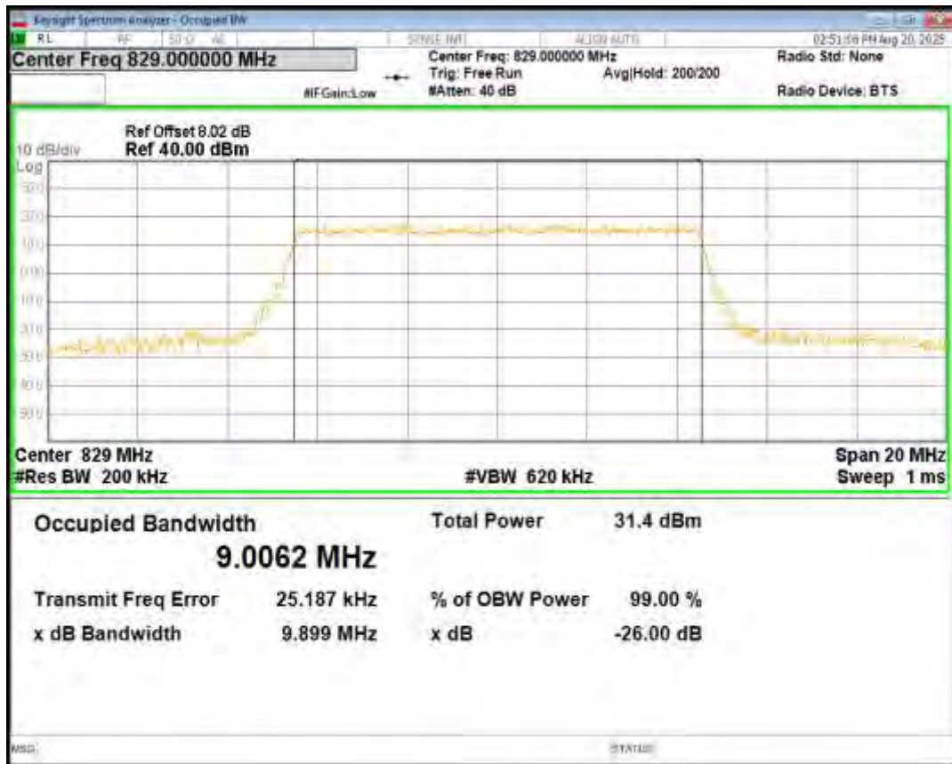
Band26(824-849) 16QAM BW=10MHz Channel=26840 RB Size=50 Position=#0
