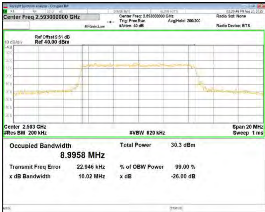
Band41 QPSK BW=10MHz Channel=41540 RB Size=50 Position=#0
