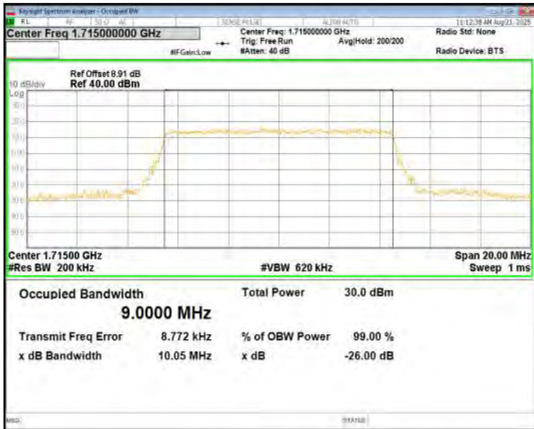
Band66 16QAM BW=10MHz Channel=132022 RB Size=50 Position=#0
