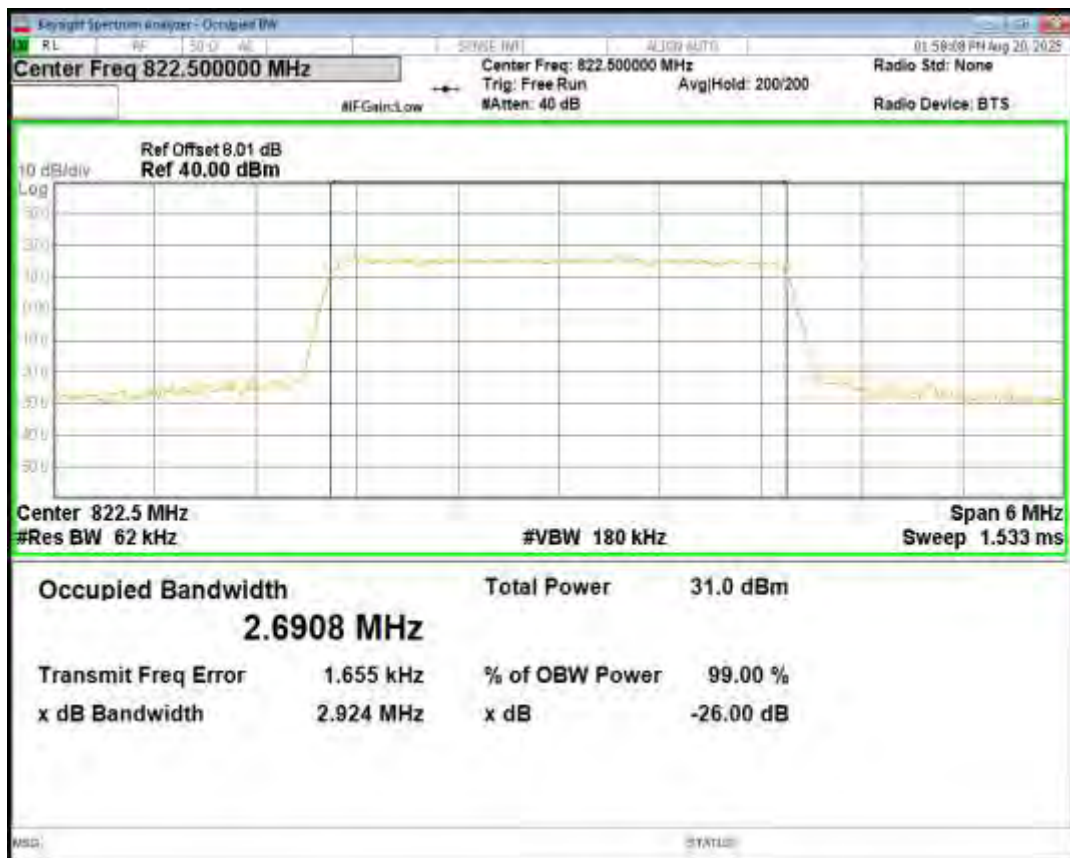
Band26(814-824) QPSK BW=5MHz Channel=26715 RB Size=25 Position=#0
