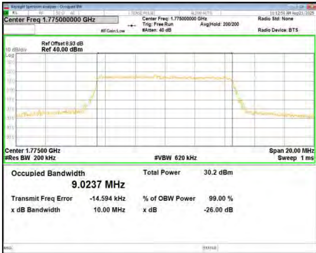
Band66 16QAM BW=10MHz Channel=132622 RB Size=50 Position=#0
