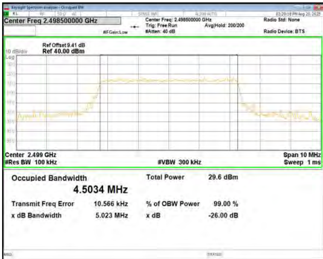
Band41 QPSK BW=5MHz Channel=40620 RB Size=25 Position=#0
