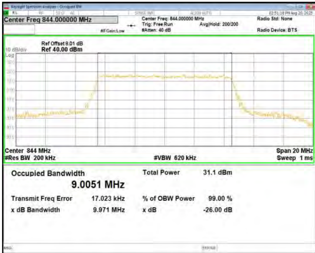
Band26(824-849) 16QAM BW=10MHz Channel=26990 RB Size=50 Position=#0
