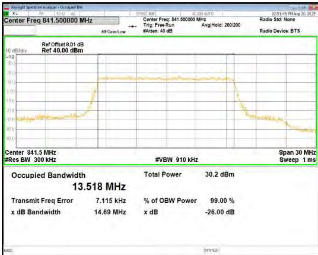
Band4 QPSK BW=1.4MHz Channel=19957 RB Size=6 Position=#0
