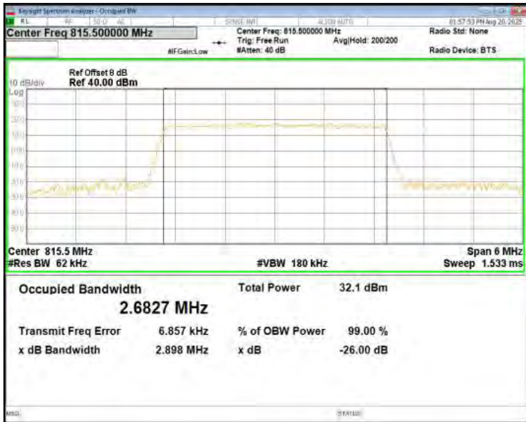
Band26(814-824) 16QAM BW=3MHz Channel=26705 RB Size=15 Position=#0
