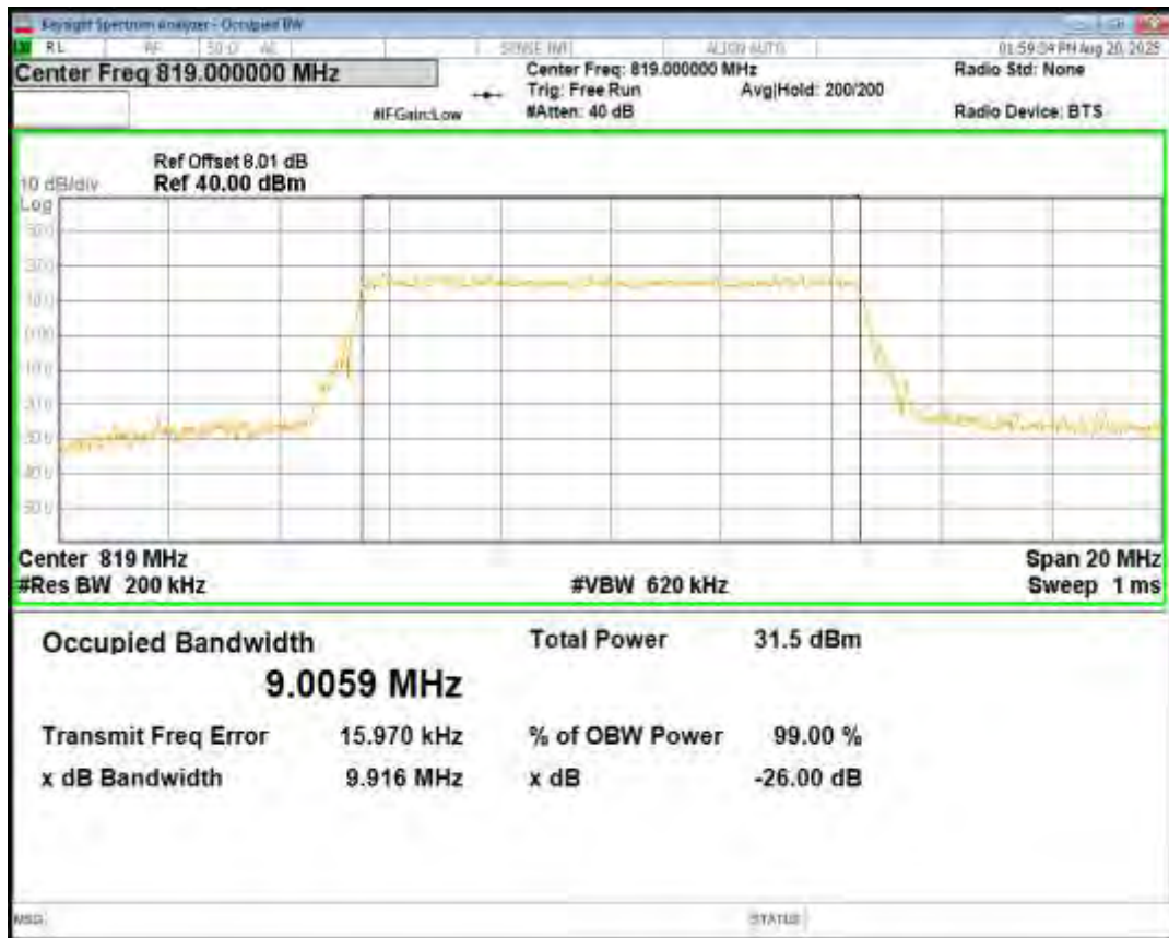
Band26(814-824) 16QAM BW=10MHz Channel=26740 RB Size=50 Position=#0
