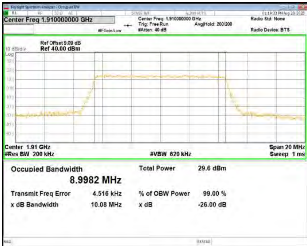
Band25 QPSK BW=15MHz Channel=26115 RB Size=75 Position=#0
