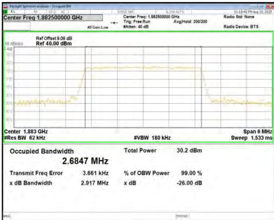
Band25 QPSK BW=3MHz Channel=26675 RB Size=15 Position=#0
