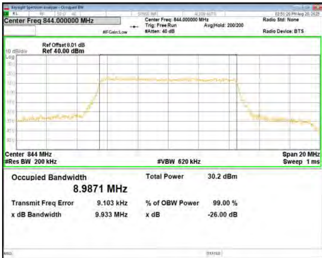
Band26(824-849) QPSK BW=15MHz Channel=26865 RB Size=75 Position=#0
