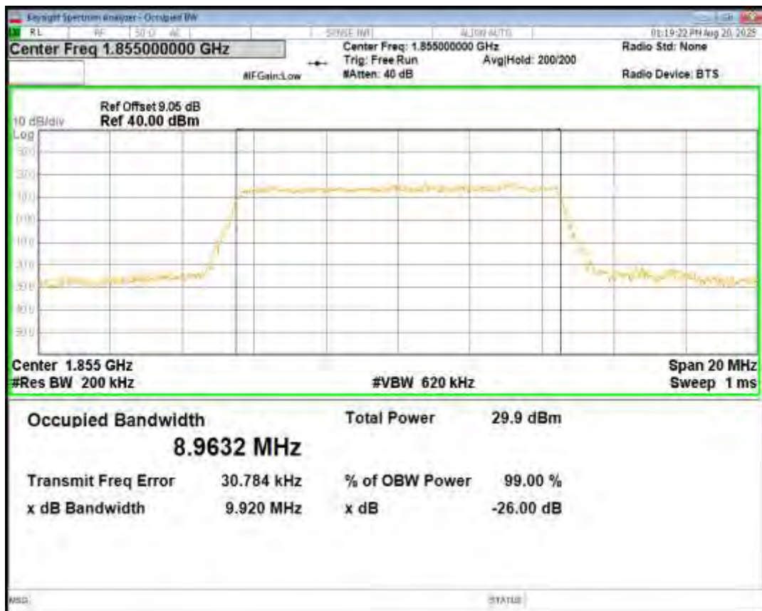
Band25 QPSK BW=10MHz Channel=26365 RB Size=50 Position=#0
