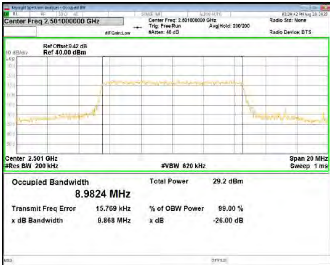
Band41 QPSK BW=10MHz Channel=40620 RB Size=50 Position=#0
