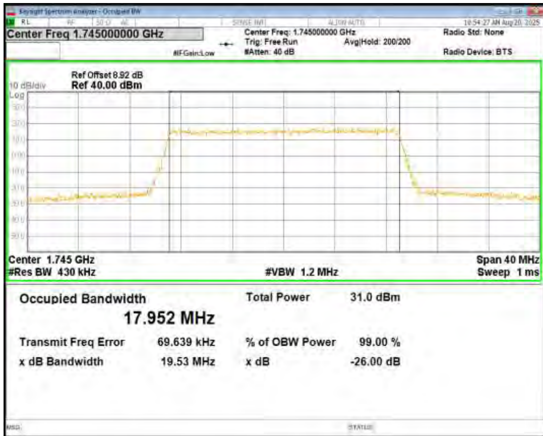
Band4 16QAM BW=20MHz Channel=20300 RB Size=100 Position=#0
