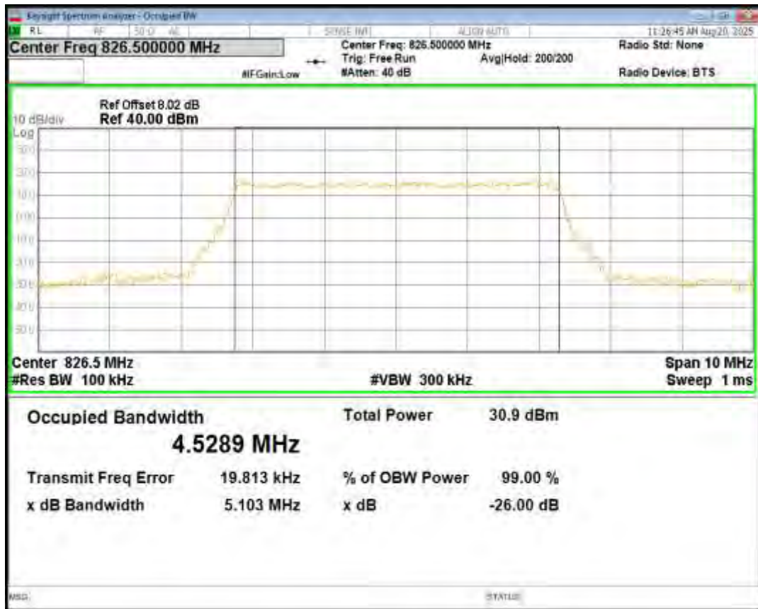
Band5 16QAM BW=5MHz Channel=20425 RB Size=25 Position=#0
