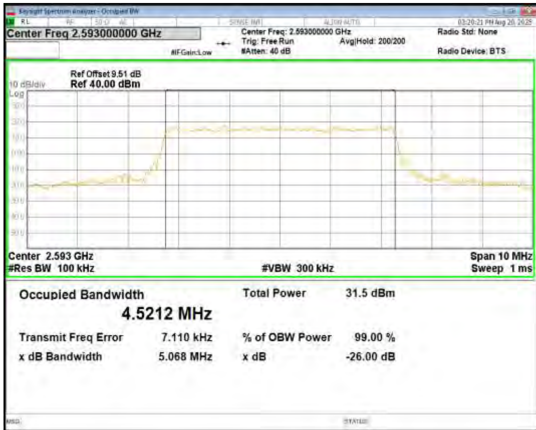
Band41 16QAM BW=5MHz Channel=40620 RB Size=25 Position=#0
