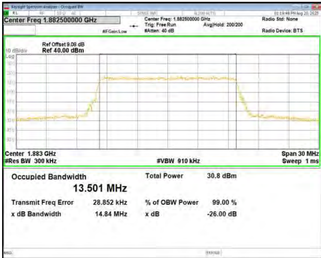
Band25 16QAM BW=15MHz Channel=26365 RB Size=75 Position=#0
