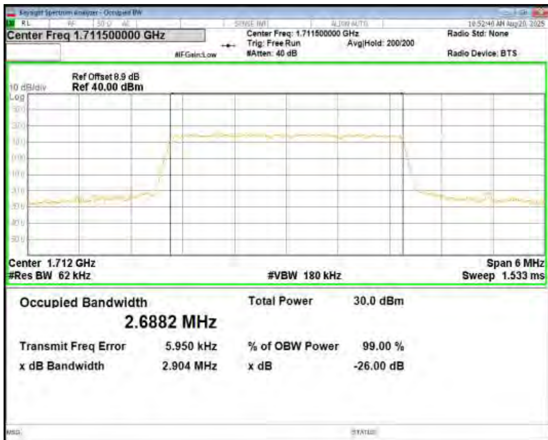
Band4 QPSK BW=3MHz Channel=20175 RB Size=15 Position=#0
