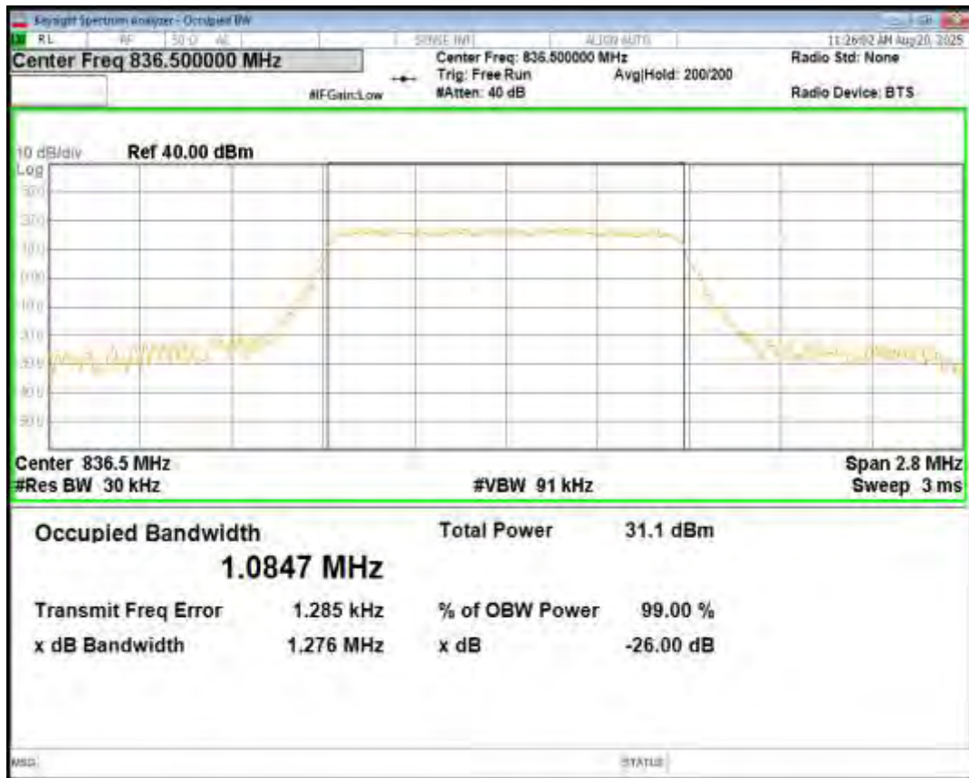
Band5 16QAM BW=1.4MHz Channel=20525 RB Size=6 Position=#0
