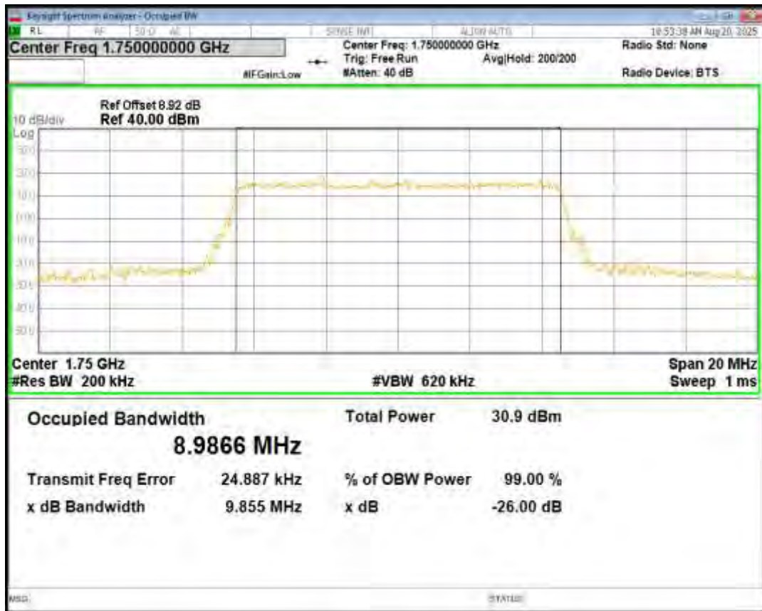
Band4 16QAM BW=10MHz Channel=20350 RB Size=50 Position=#0
