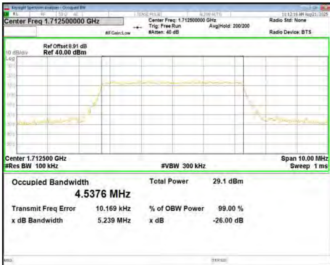
Band66 QPSK BW=5MHz Channel=132322 RB Size=25 Position=#0
