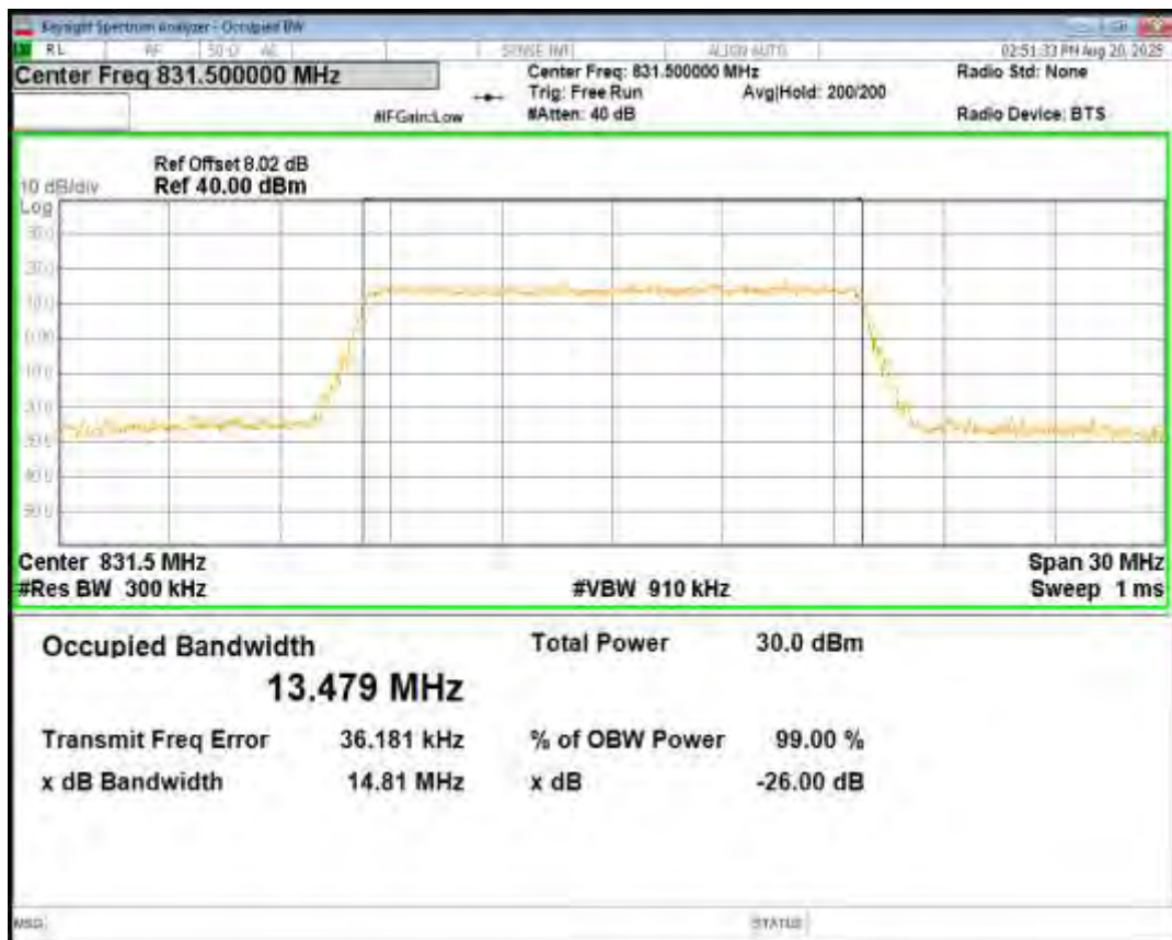
Band26(824-849) QPSK BW=15MHz Channel=26915 RB Size=75 Position=#0
