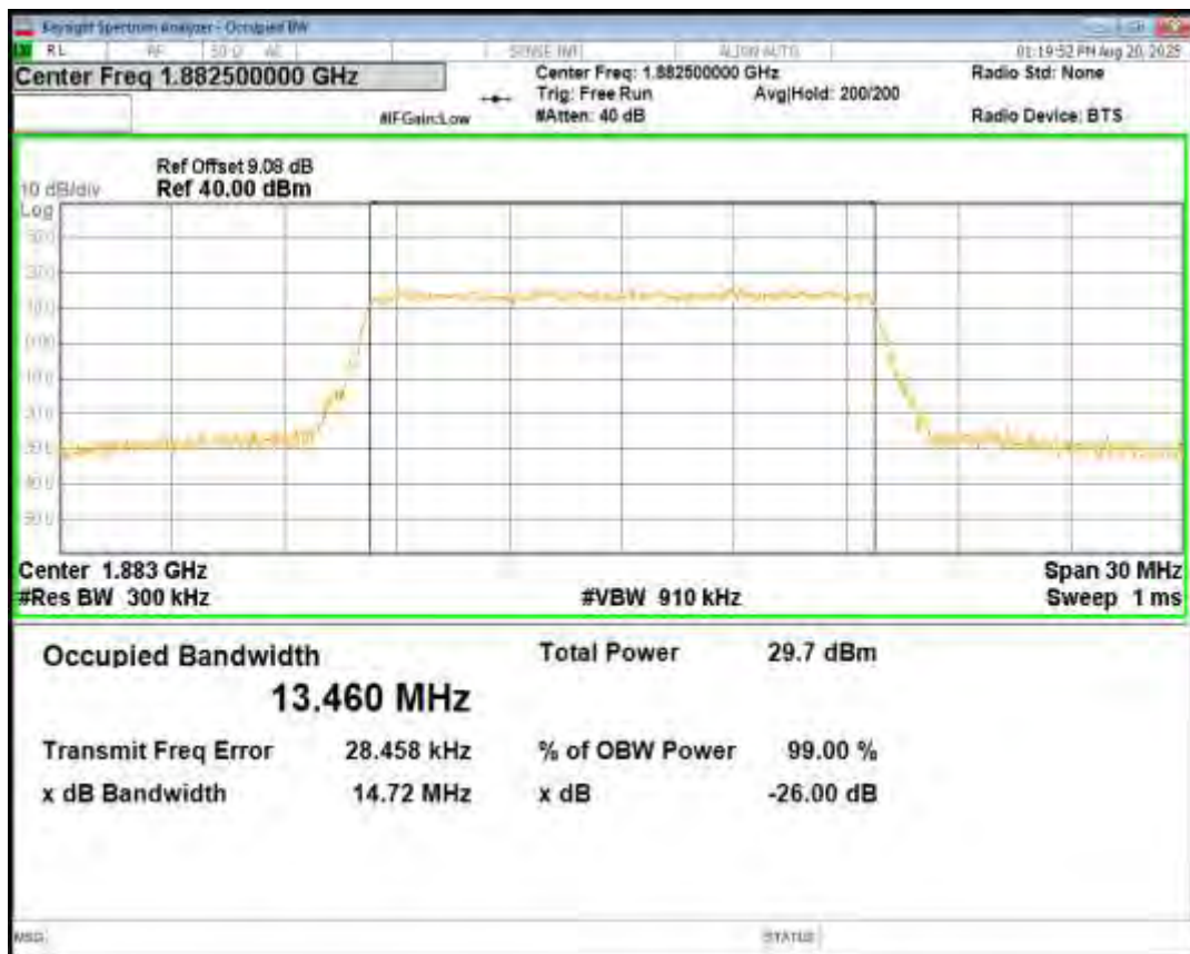
Band25 QPSK BW=15MHz Channel=26615 RB Size=75 Position=#0
