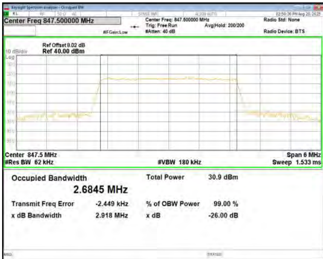
Band26(824-849) QPSK BW=5MHz Channel=26815 RB Size=25 Position=#0
