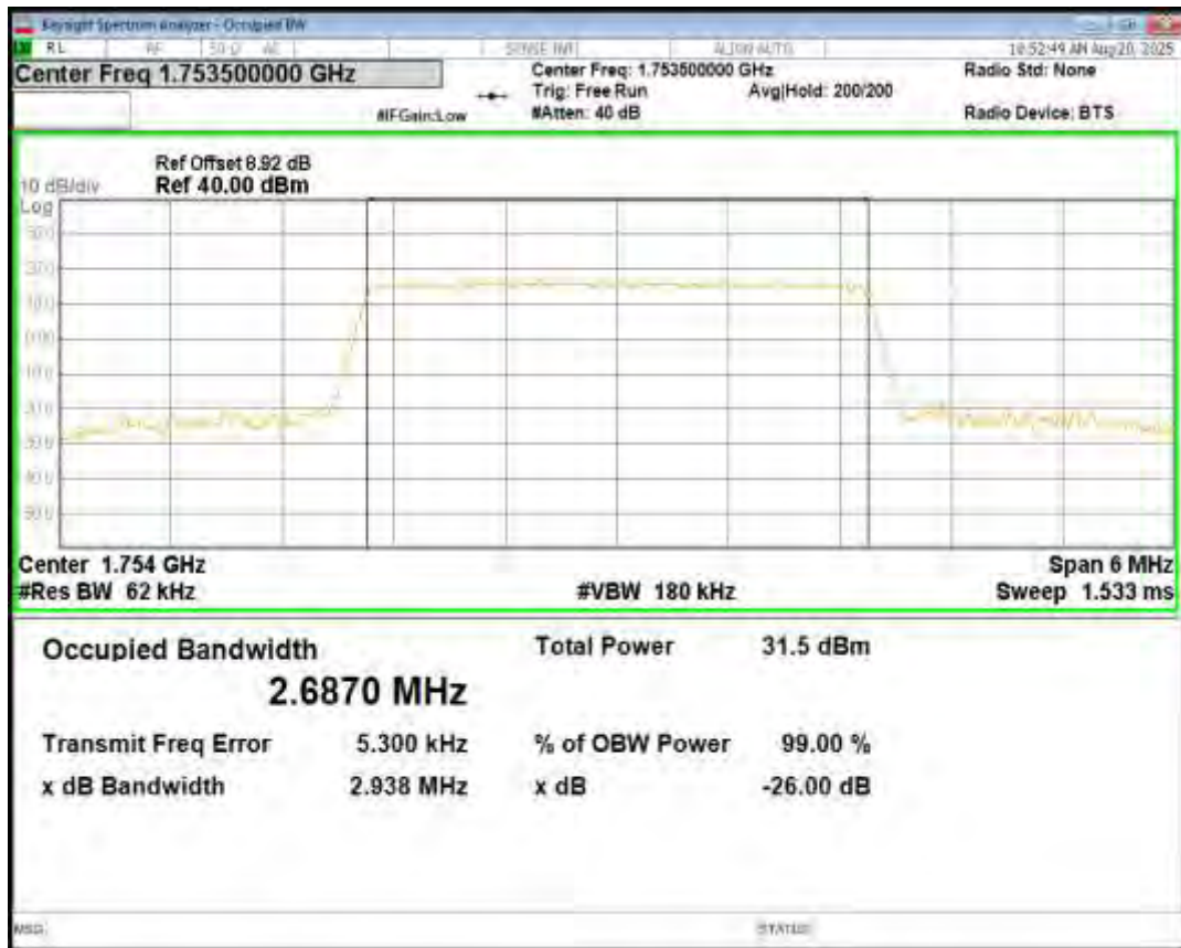
Band4 16QAM BW=3MHz Channel=20385 RB Size=15 Position=#0
