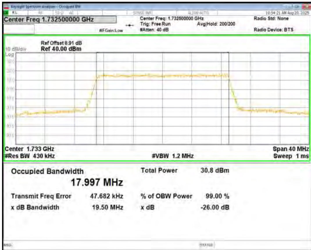
Band4 16QAM BW=20MHz Channel=20175 RB Size=100 Position=#0
