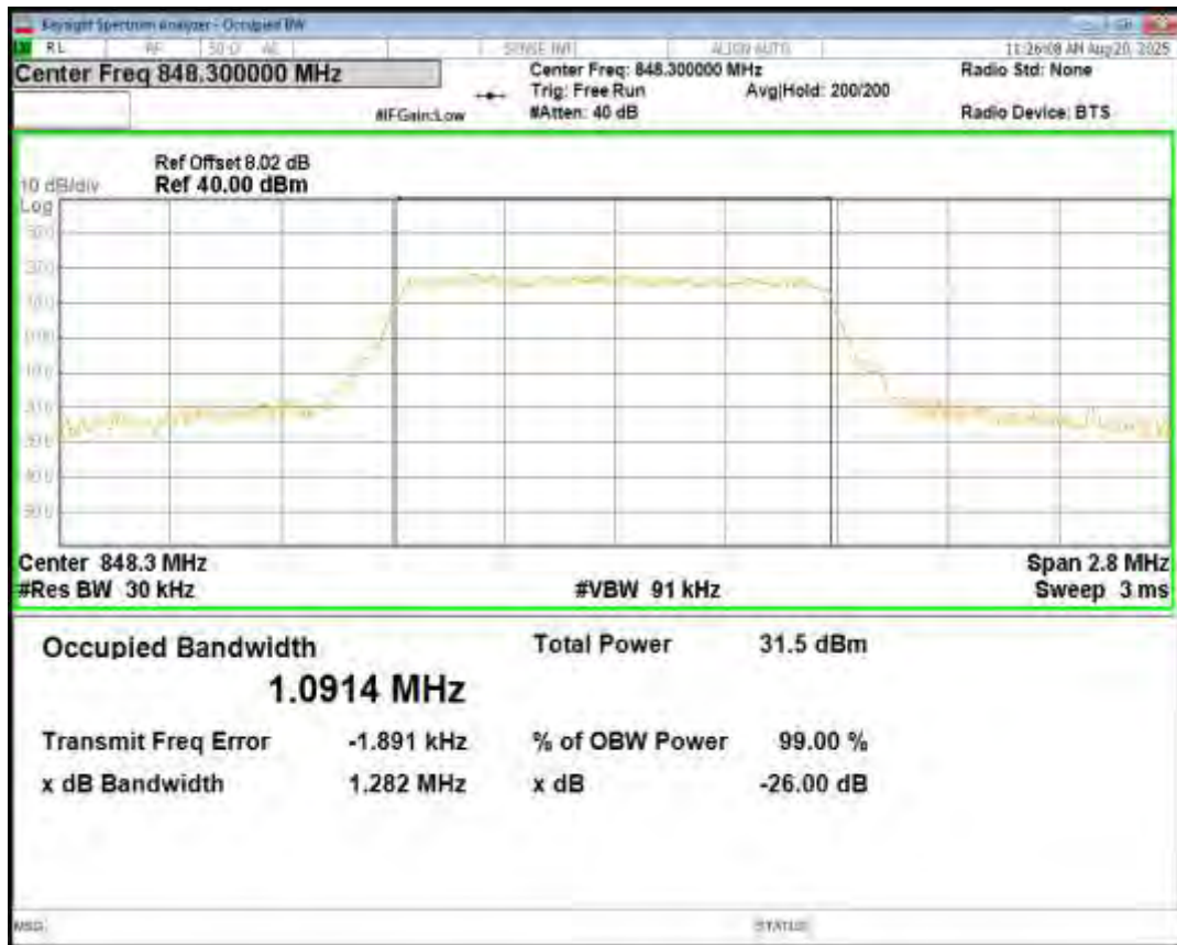
Band5 16QAM BW=1.4MHz Channel=20643 RB Size=6 Position=#0
