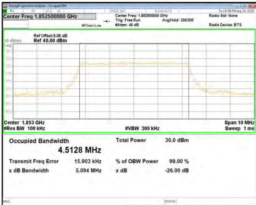
Band25 QPSK BW=5MHz Channel=26365 RB Size=25 Position=#0
