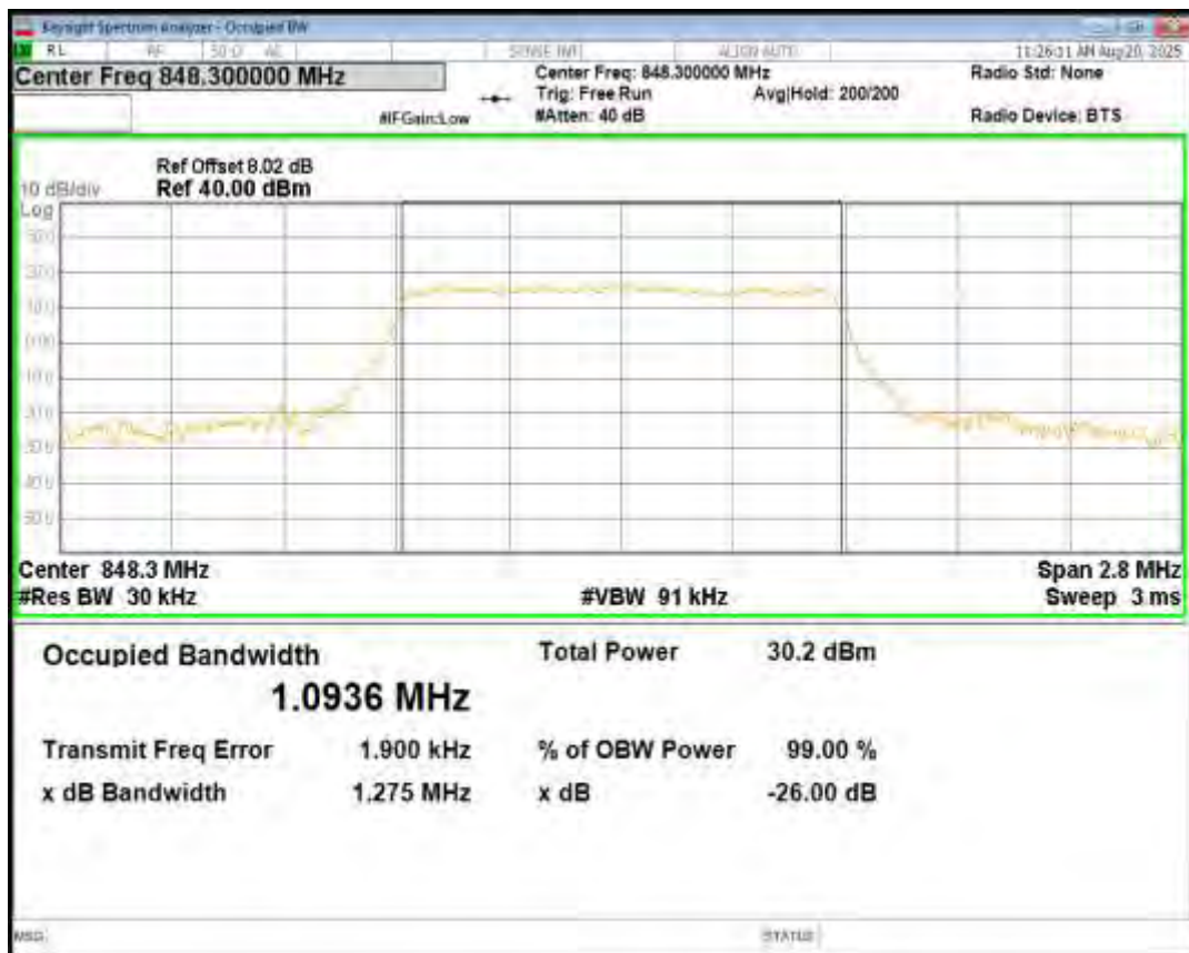
Band5 QPSK BW=3MHz Channel=20415 RB Size=15 Position=#0
