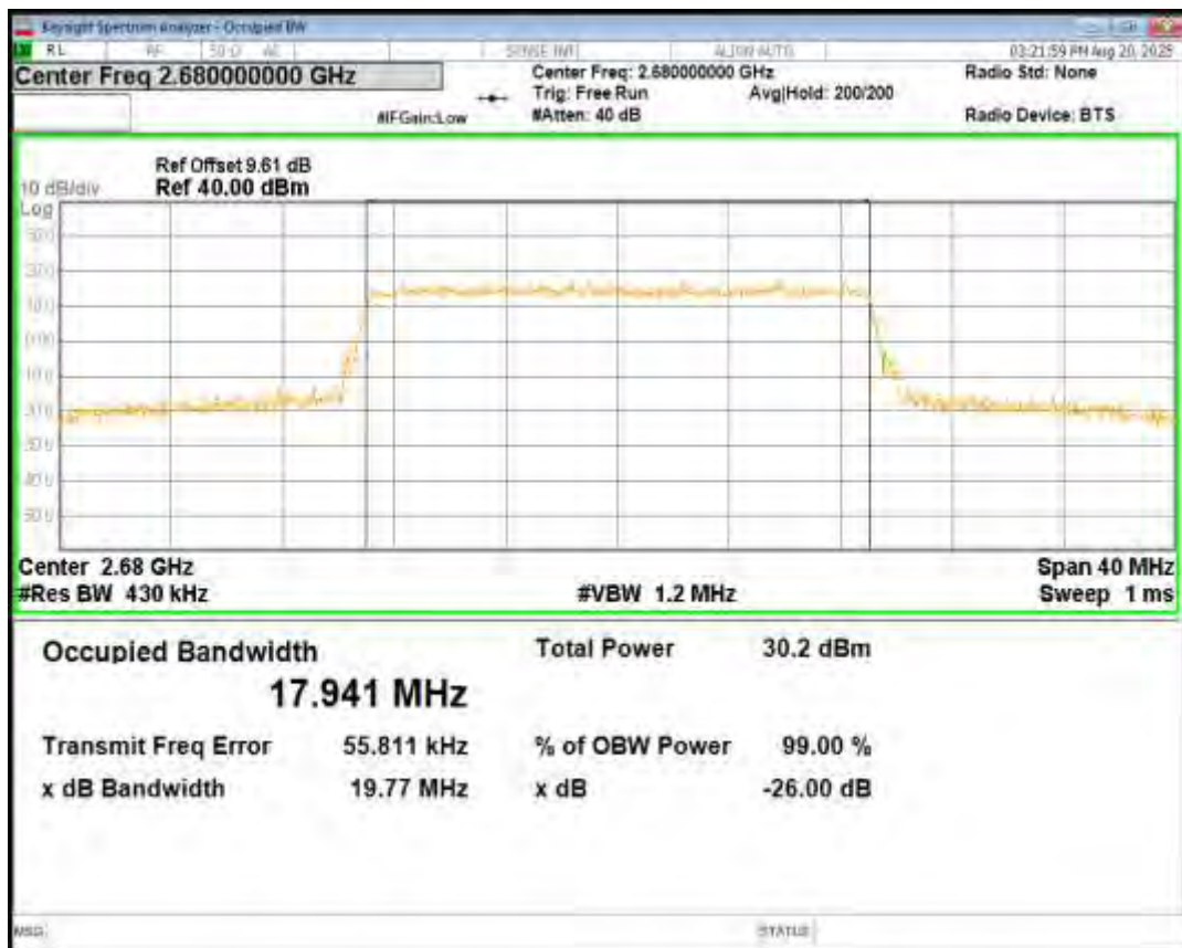
Band5 QPSK BW=1.4MHz Channel=20407 RB Size=6 Position=#0
