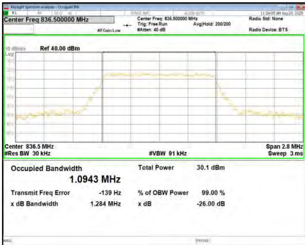
Band5 QPSK BW=1.4MHz Channel=20643 RB Size=6 Position=#0
