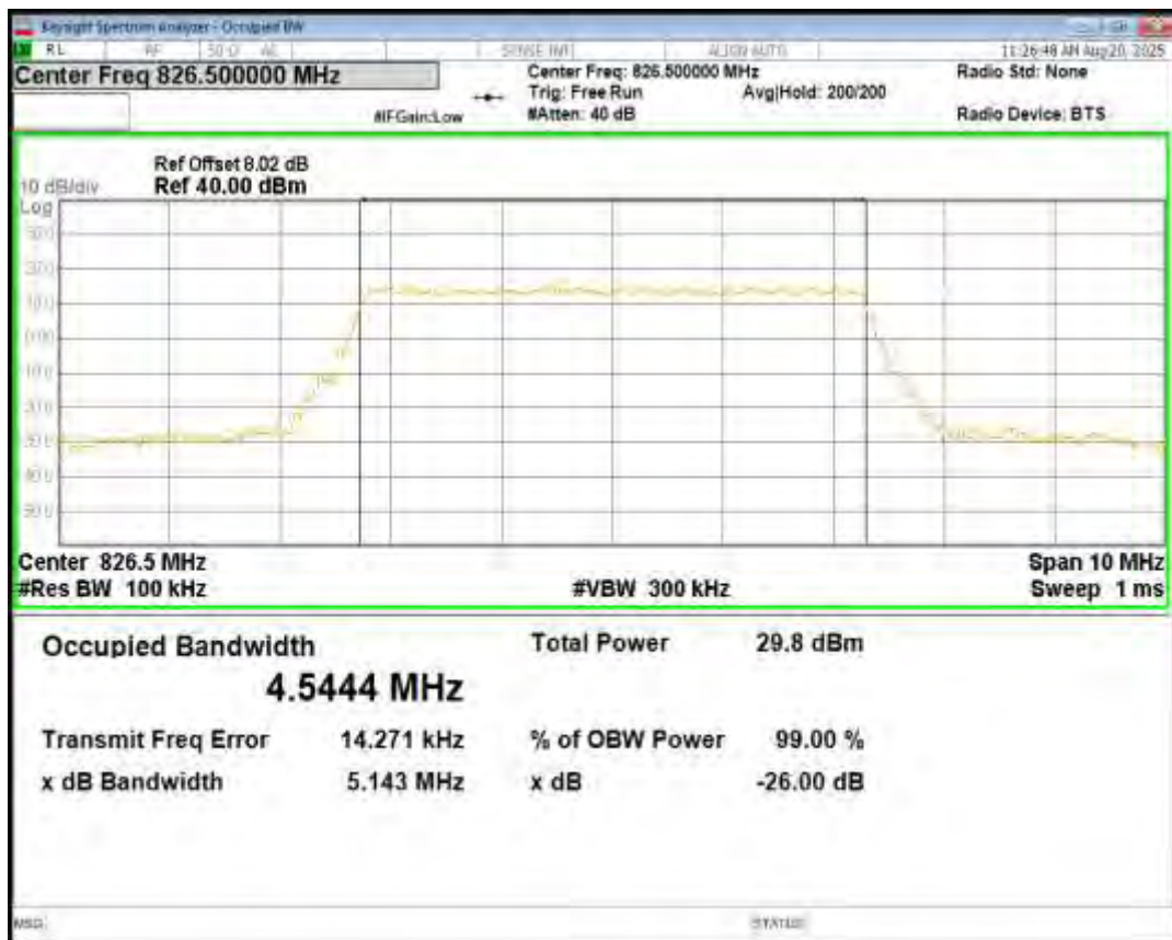
Band5 QPSK BW=5MHz Channel=20525 RB Size=25 Position=#0
