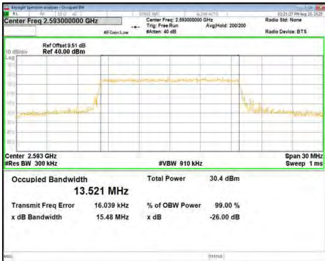
Band41 QPSK BW=15MHz Channel=41515 RB Size=75 Position=#0
