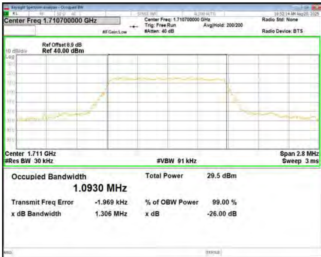
Band4 QPSK BW=1.4MHz Channel=20175 RB Size=6 Position=#0
