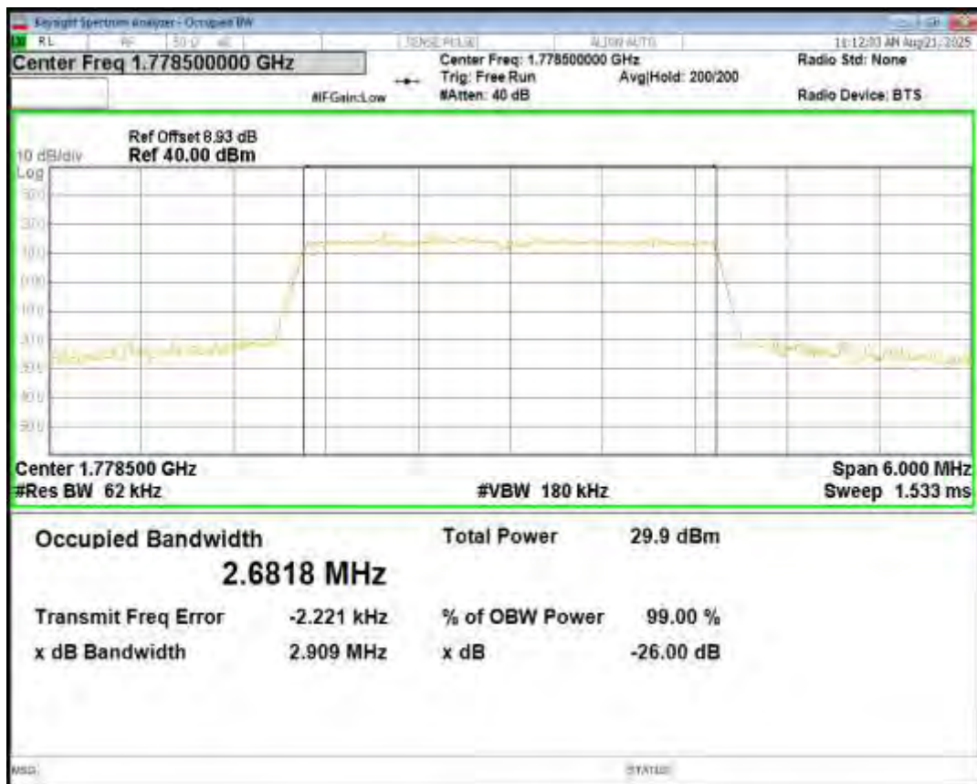
Band66 QPSK BW=5MHz Channel=131997 RB Size=25 Position=#0
