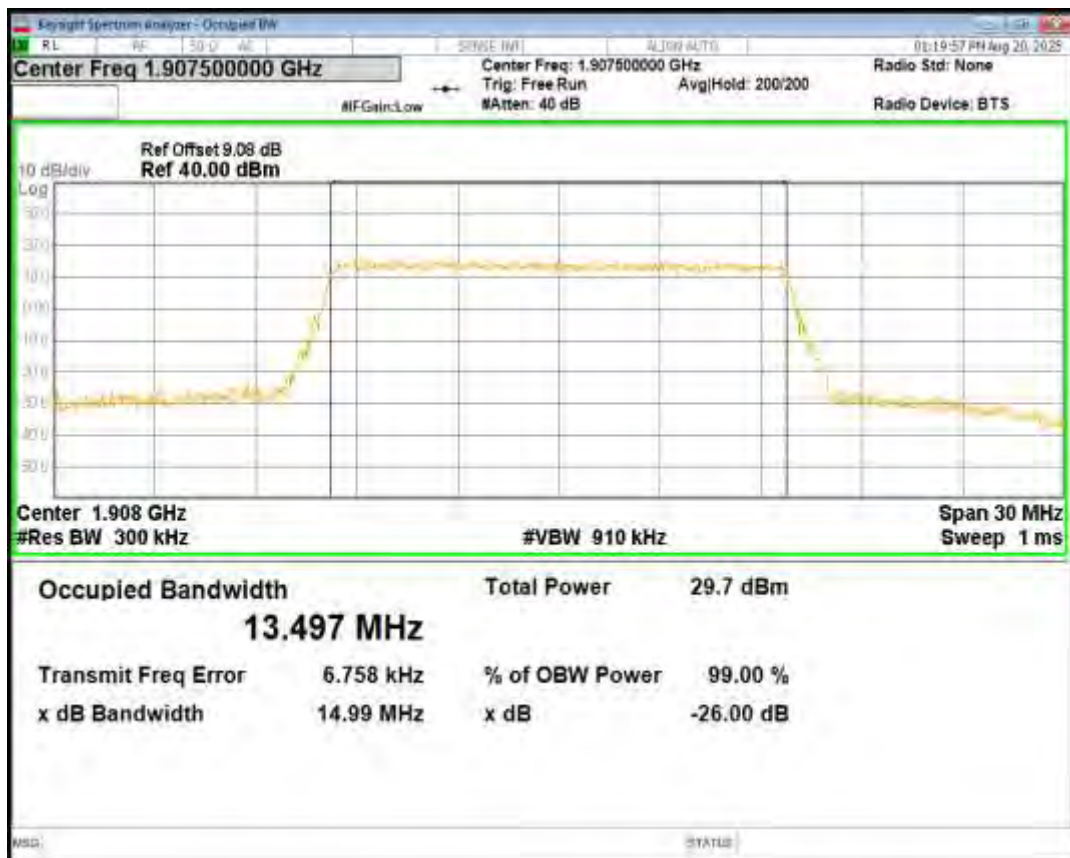
Band25 QPSK BW=20MHz Channel=26140 RB Size=100 Position=#0
