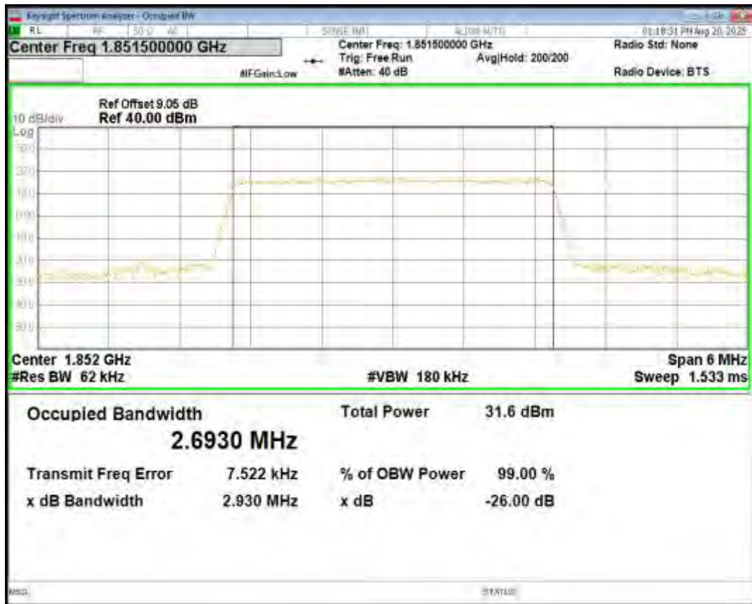
Band25 16QAM BW=3MHz Channel=26055 RB Size=15 Position=#0
