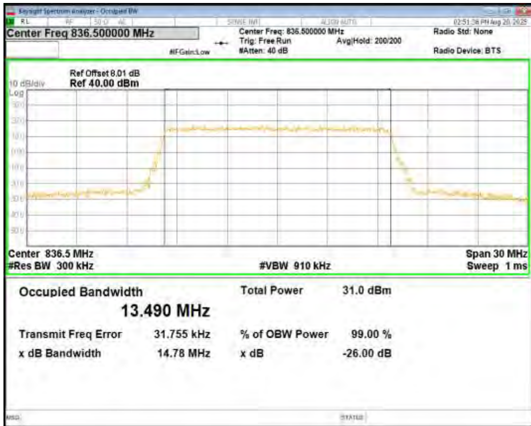
Band26(824-849) 16QAM BW=15MHz Channel=26915 RB Size=75 Position=#0
