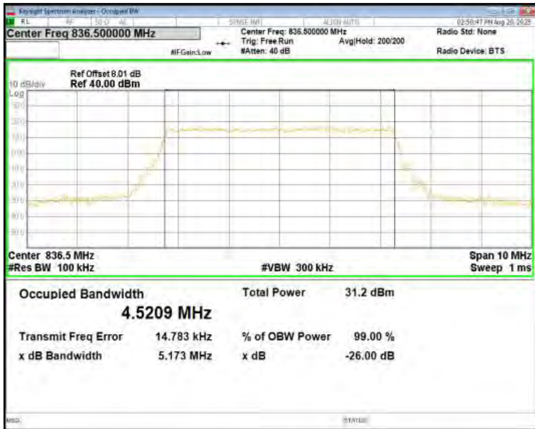
Band26(824-849) 16QAM BW=5MHz Channel=26915 RB Size=25 Position=#0
