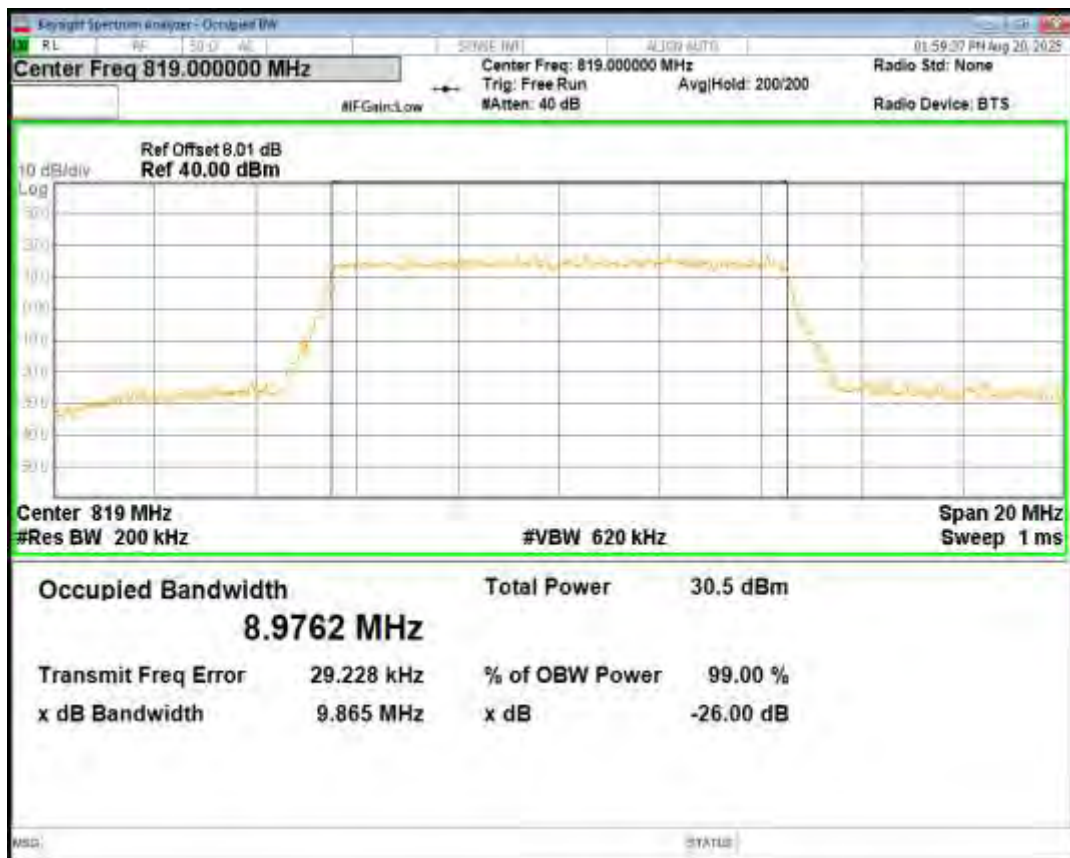
Band26(824-849) QPSK BW=1.4MHz Channel=26797 RB Size=6 Position=#0
