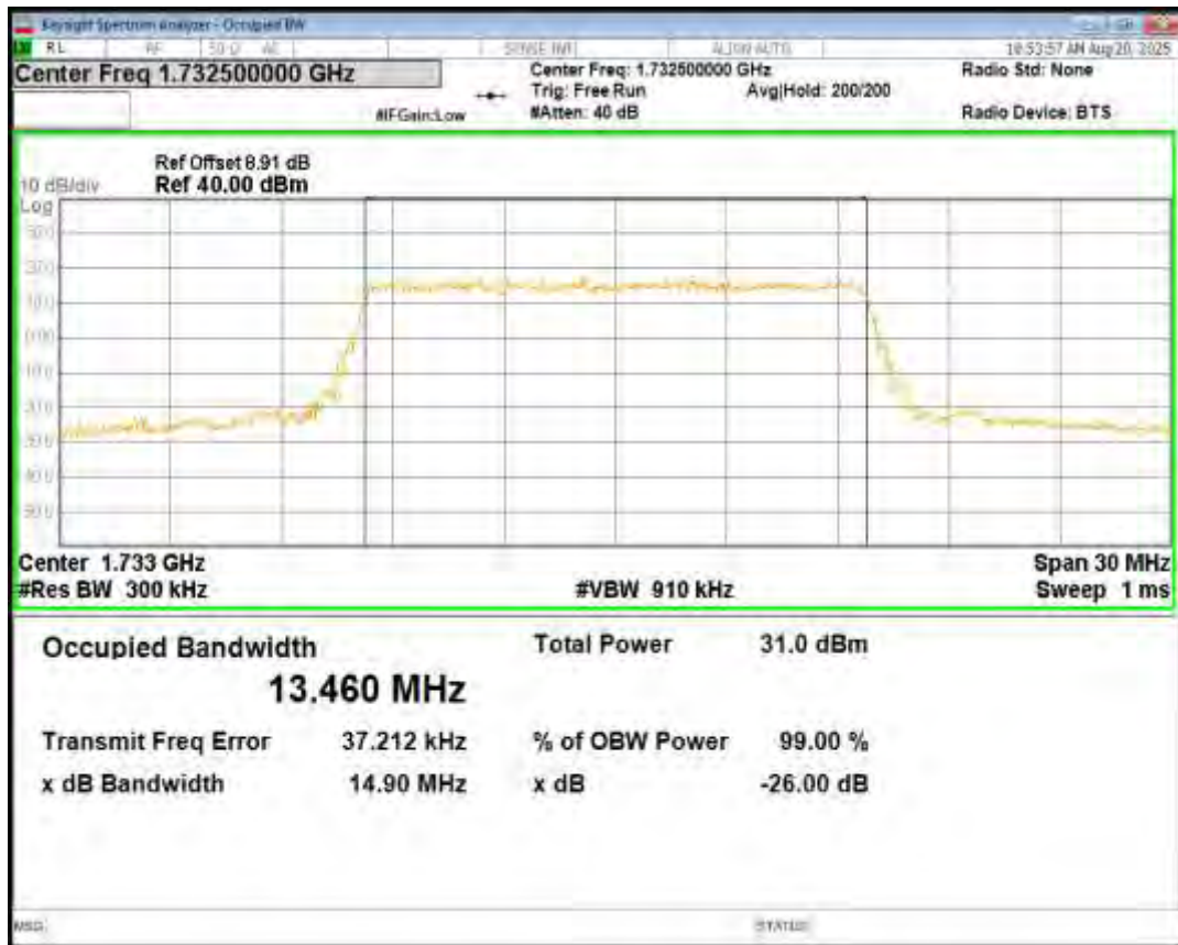
Band4 16QAM BW=15MHz Channel=20175 RB Size=75 Position=#0
