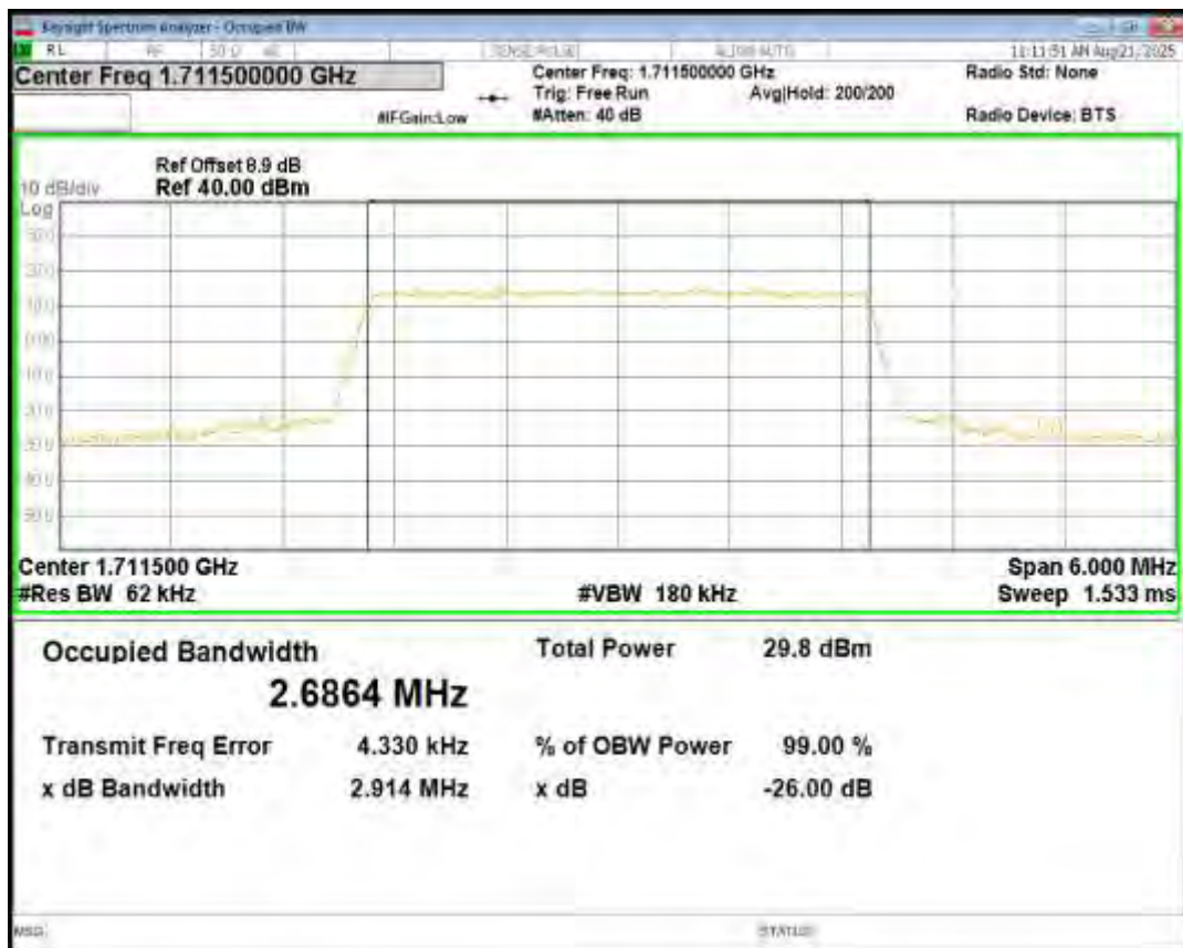
Band66 QPSK BW=3MHz Channel=132322 RB Size=15 Position=#0
