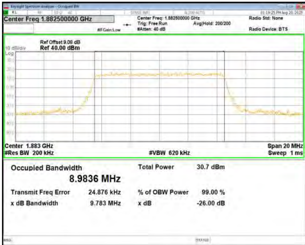
Band25 16QAM BW=10MHz Channel=26365 RB Size=50 Position=#0
