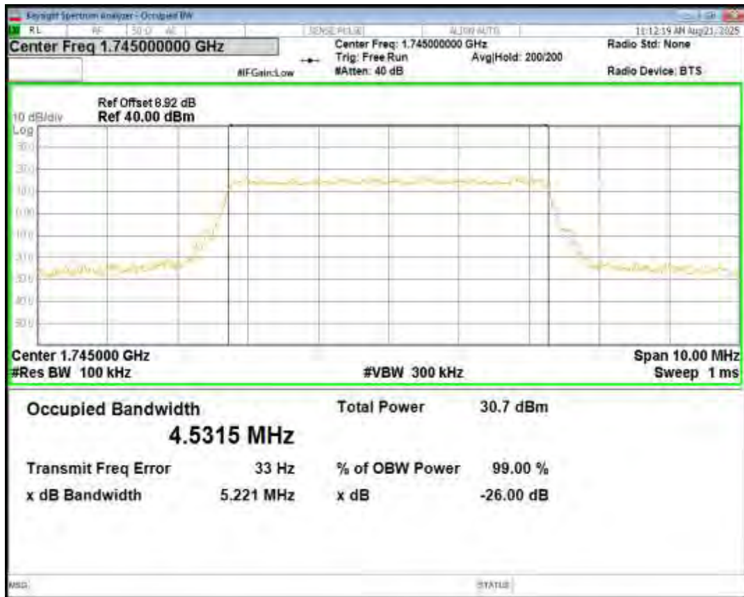
Band66 16QAM BW=5MHz Channel=132322 RB Size=25 Position=#0
