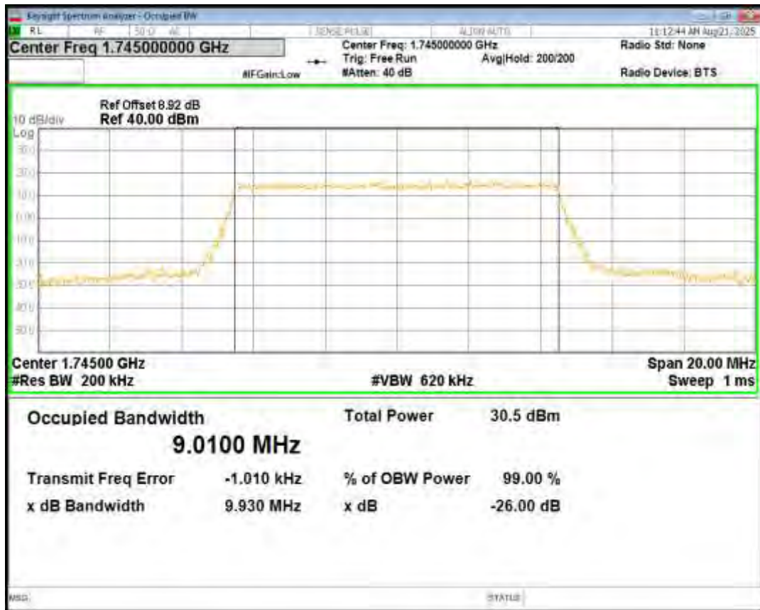
Band66 16QAM BW=10MHz Channel=132322 RB Size=50 Position=#0
