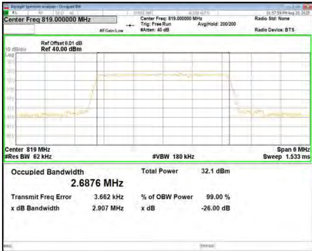
Band26(814-824) 16QAM BW=3MHz Channel=26740 RB Size=15 Position=#0
