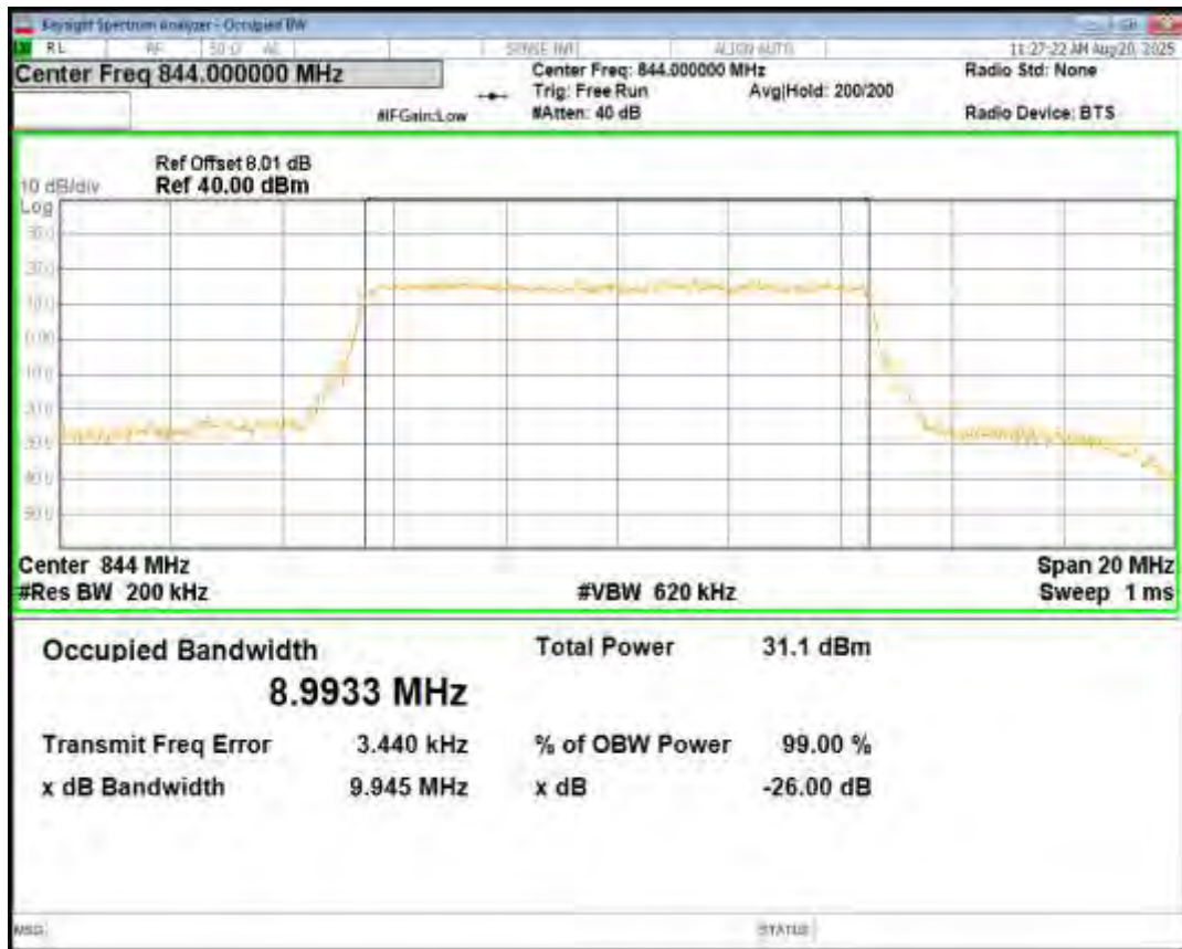
Band5 16QAM BW=10MHz Channel=20600 RB Size=50 Position=#0
