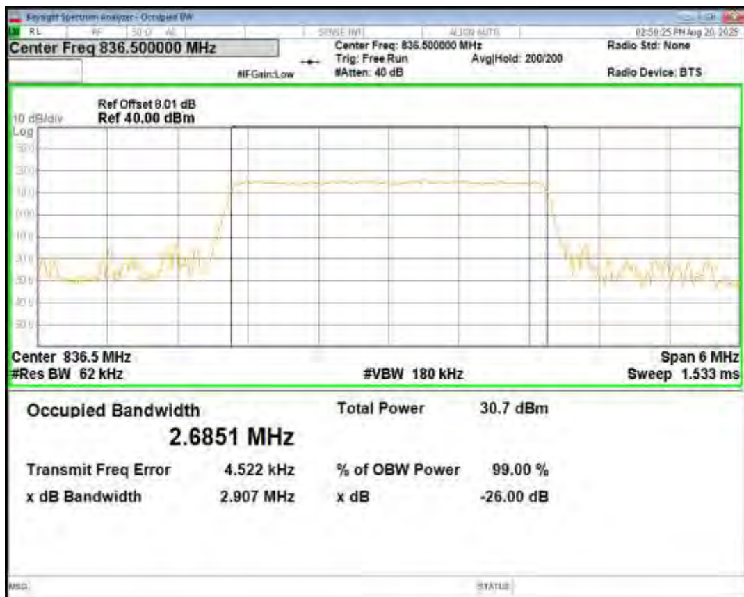
Band26(824-849) QPSK BW=3MHz Channel=27025 RB Size=15 Position=#0
