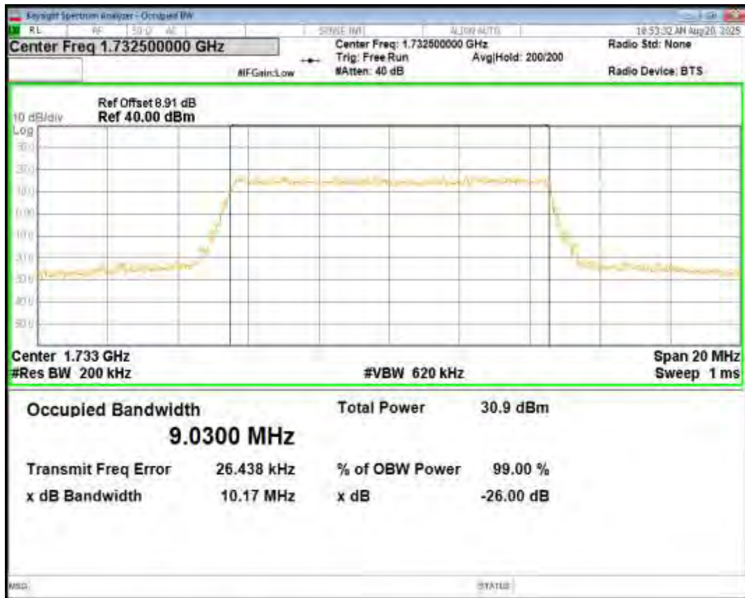
Band4 16QAM BW=10MHz Channel=20175 RB Size=50 Position=#0
