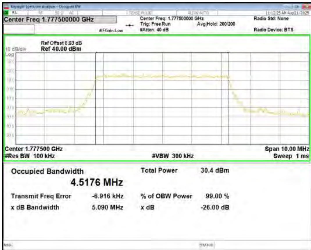
Band66 16QAM BW=5MHz Channel=132647 RB Size=25 Position=#0
