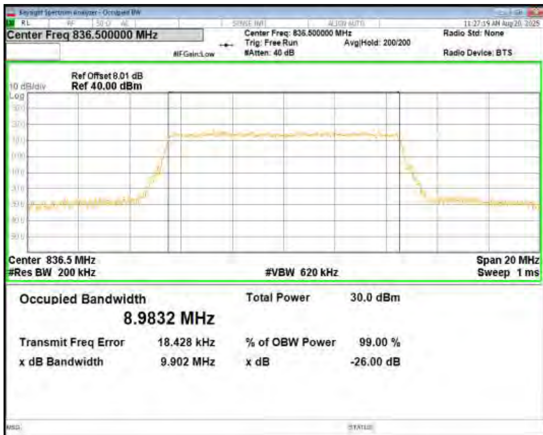
Band5 QPSK BW=10MHz Channel=20600 RB Size=50 Position=#0
