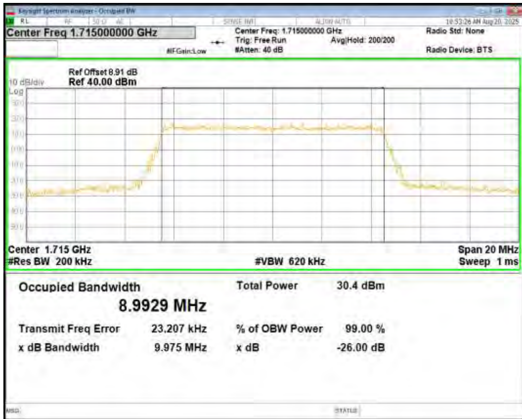
Band4 16QAM BW=10MHz Channel=20000 RB Size=50 Position=#0
