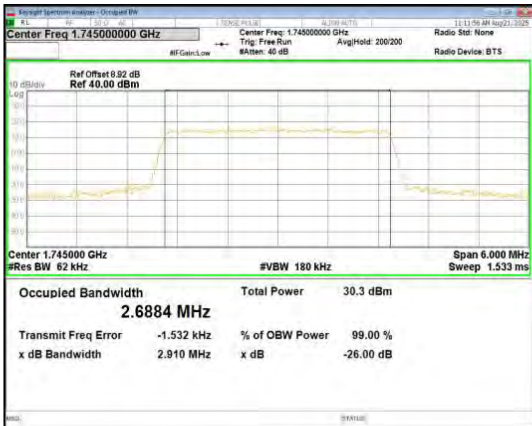
Band66 QPSK BW=3MHz Channel=132657 RB Size=15 Position=#0
