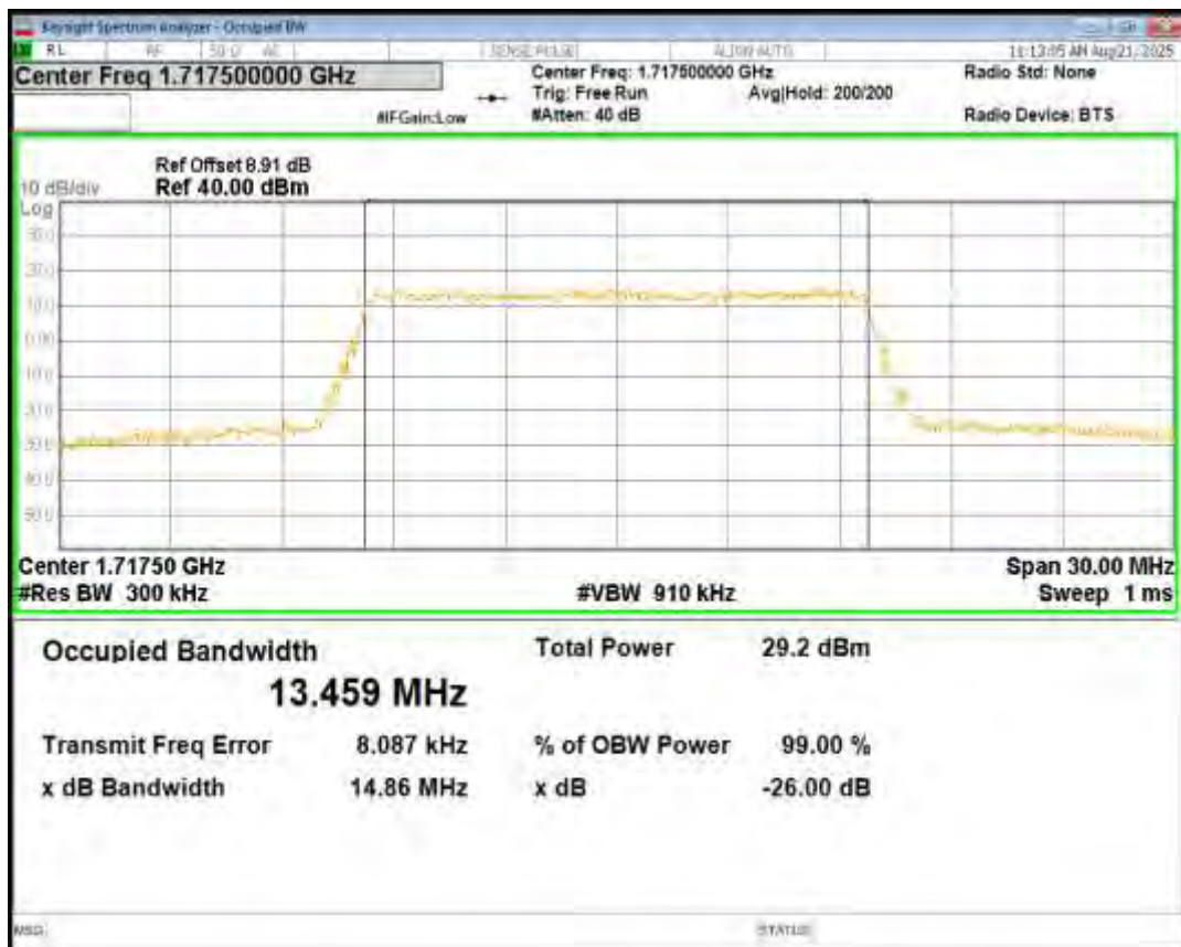
Band66 QPSK BW=15MHz Channel=132322 RB Size=75 Position=#0
