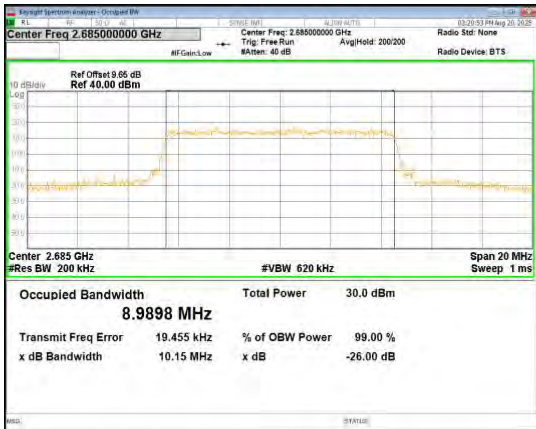
Band41 QPSK BW=15MHz Channel=39725 RB Size=75 Position=#0
