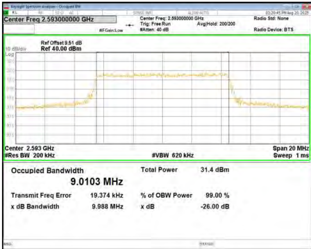
Band41 16QAM BW=10MHz Channel=40620 RB Size=50 Position=#0
