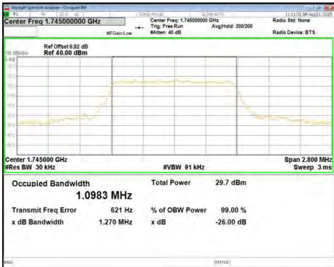
Band66 QPSK BW=1.4MHz Channel=132665 RB Size=6 Position=#0
