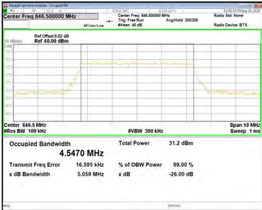
Band26(824-849) 16QAM BW=5MHz Channel=27015 RB Size=25 Position=#0
