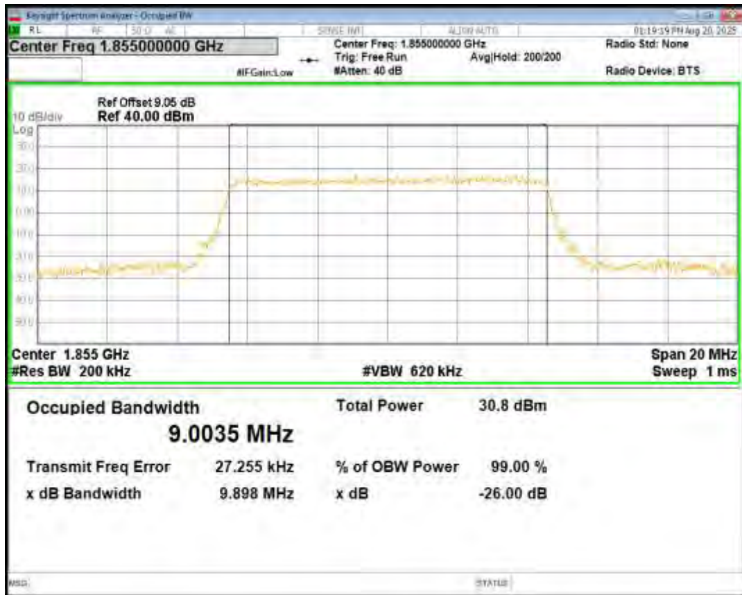
Band25 16QAM BW=10MHz Channel=26090 RB Size=50 Position=#0
