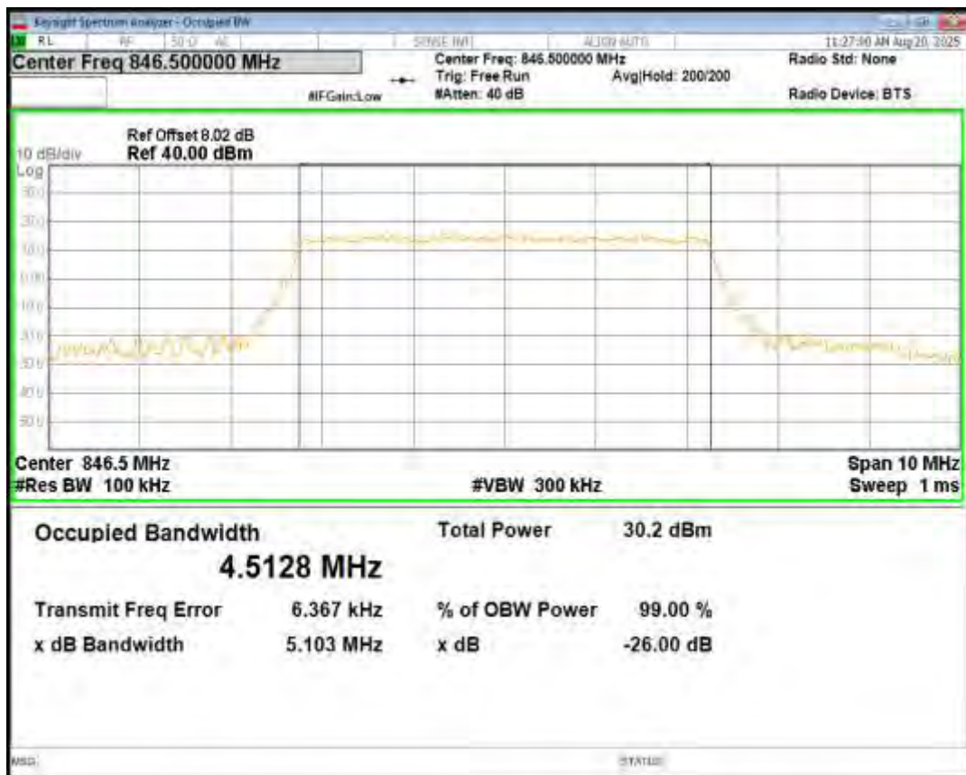
Band5 QPSK BW=10MHz Channel=20450 RB Size=50 Position=#0
