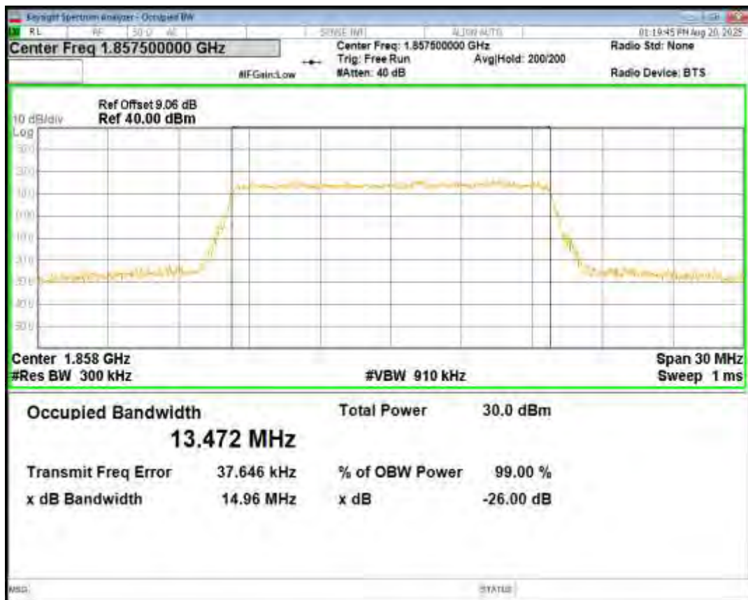
Band25 QPSK BW=15MHz Channel=26365 RB Size=75 Position=#0
