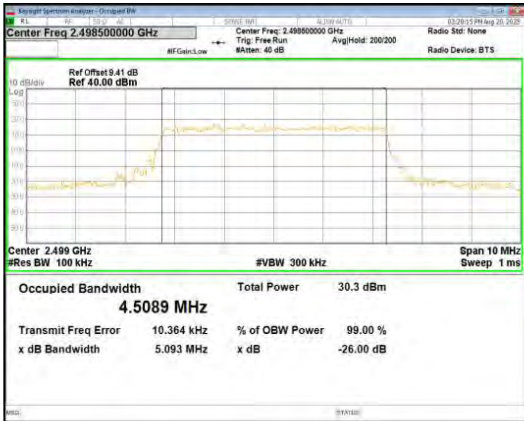
Band41 16QAM BW=5MHz Channel=39675 RB Size=25 Position=#0
