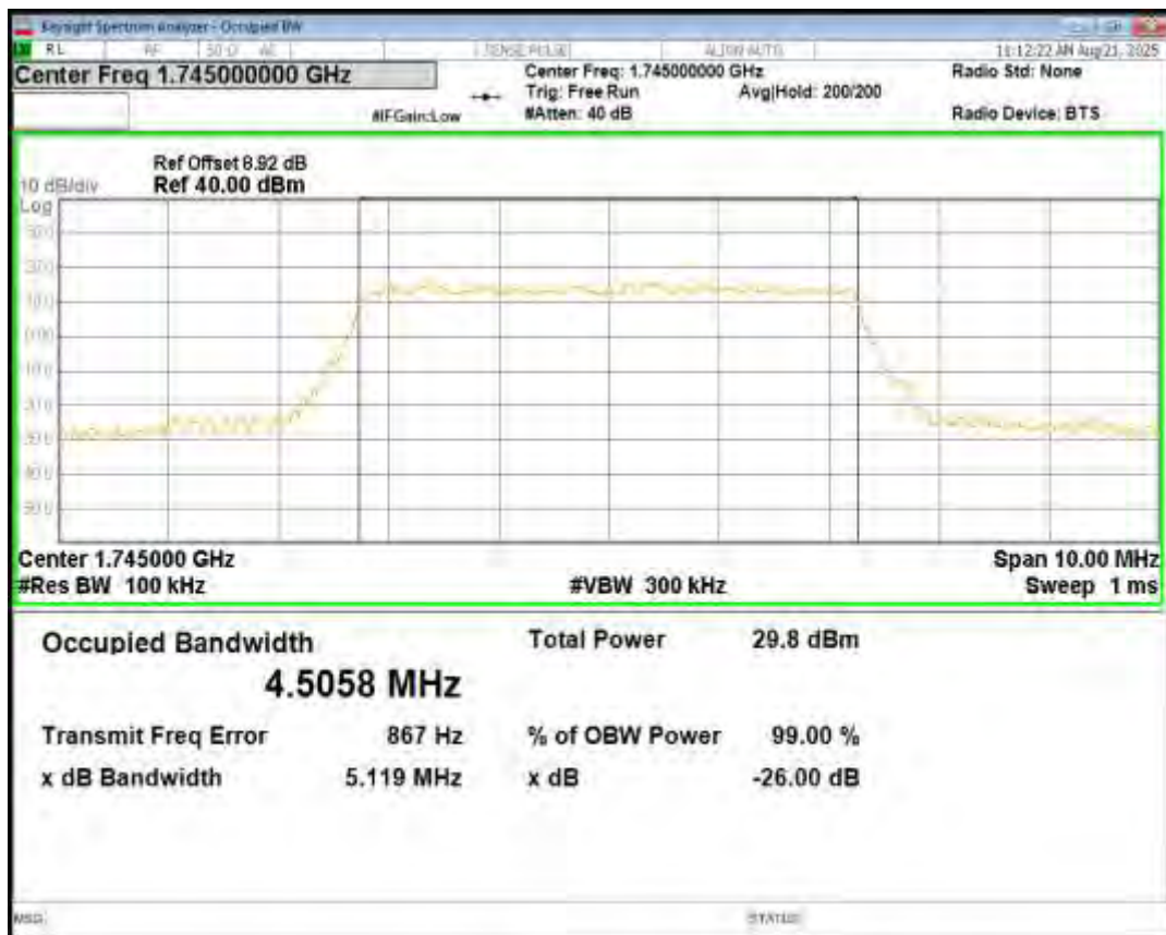
Band66 QPSK BW=5MHz Channel=132647 RB Size=25 Position=#0
