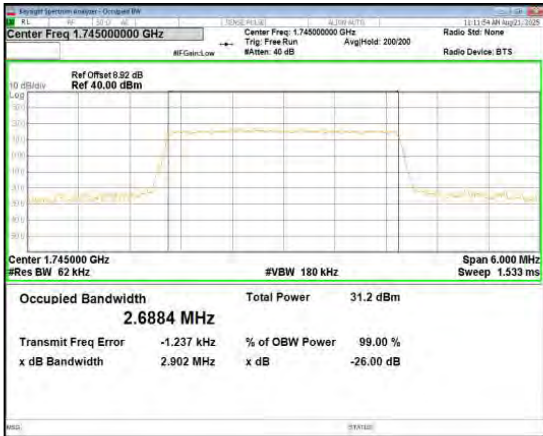
Band66 16QAM BW=3MHz Channel=132322 RB Size=15 Position=#0
