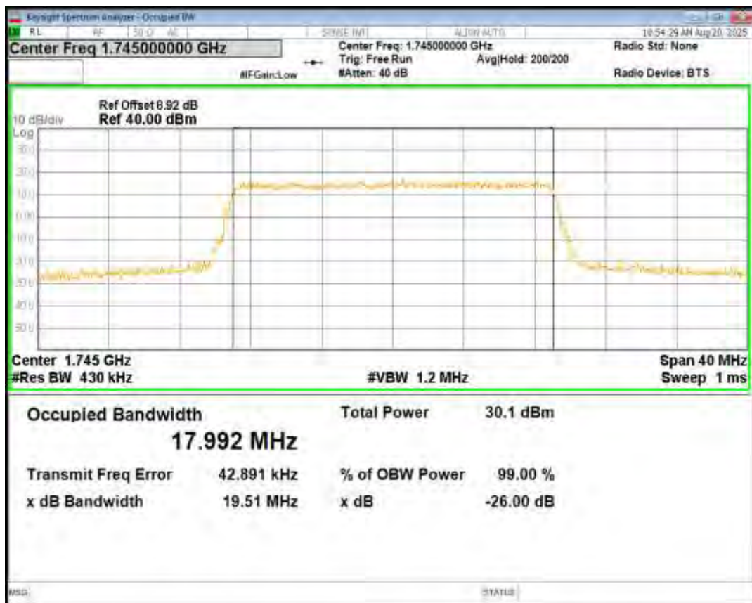
Band41 QPSK BW=5MHz Channel=39675 RB Size=25 Position=#0
