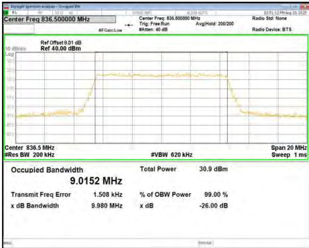
Band26(824-849) 16QAM BW=10MHz Channel=26915 RB Size=50 Position=#0
