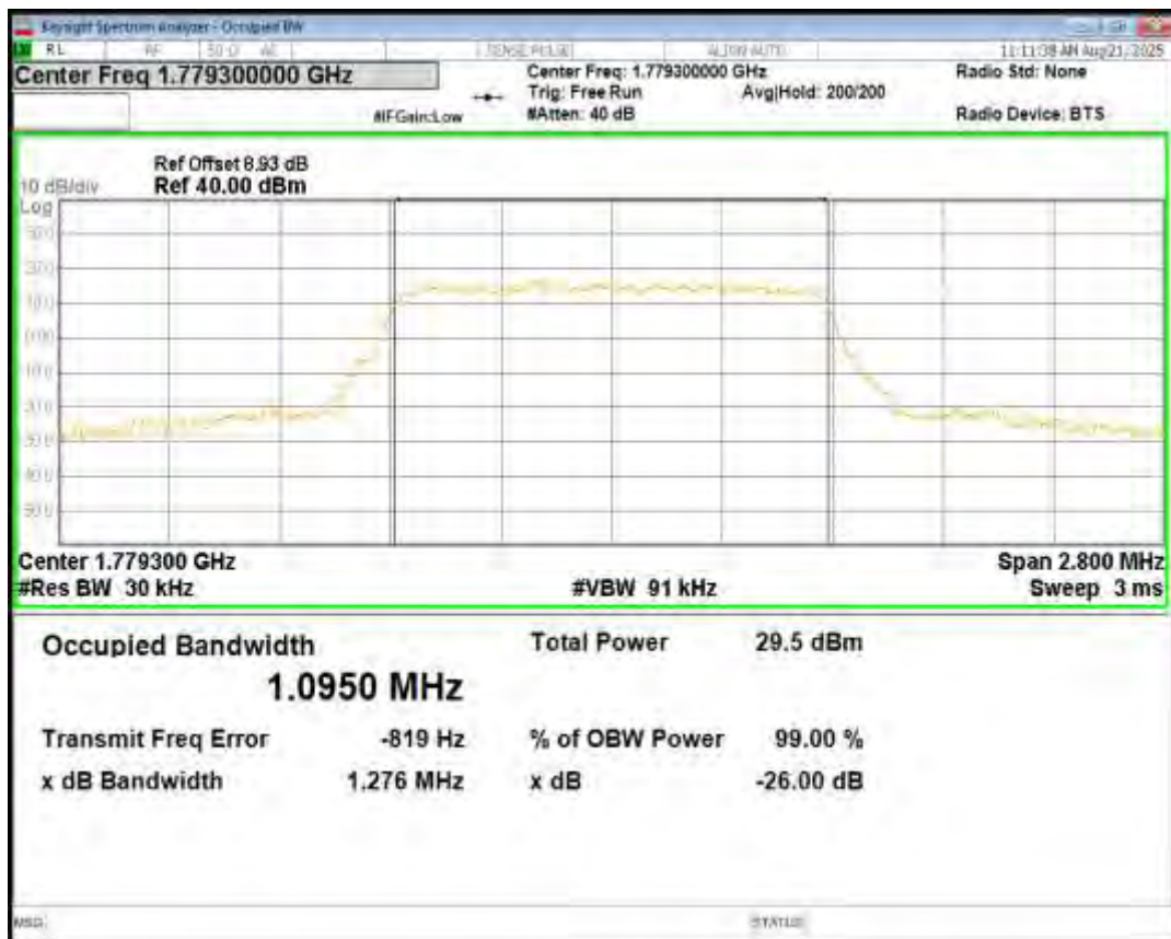
Band66 QPSK BW=3MHz Channel=131987 RB Size=15 Position=#0
