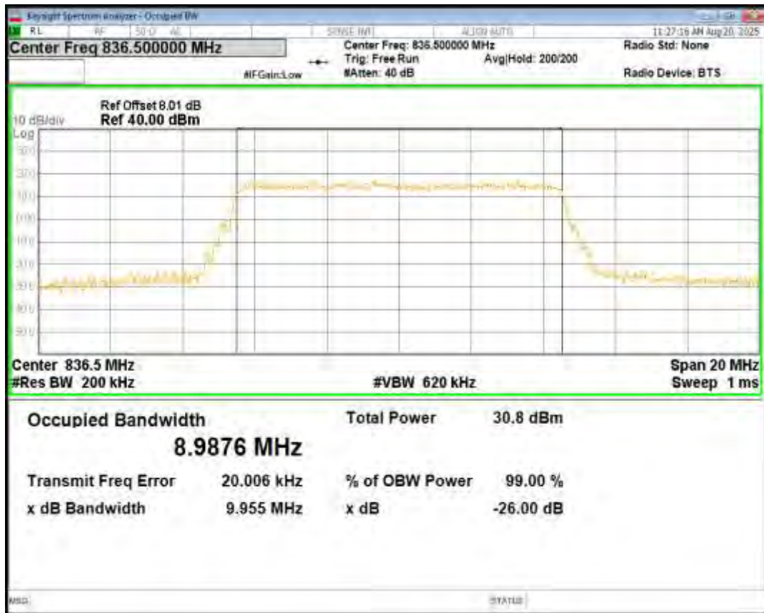
Band5 16QAM BW=10MHz Channel=20525 RB Size=50 Position=#0
