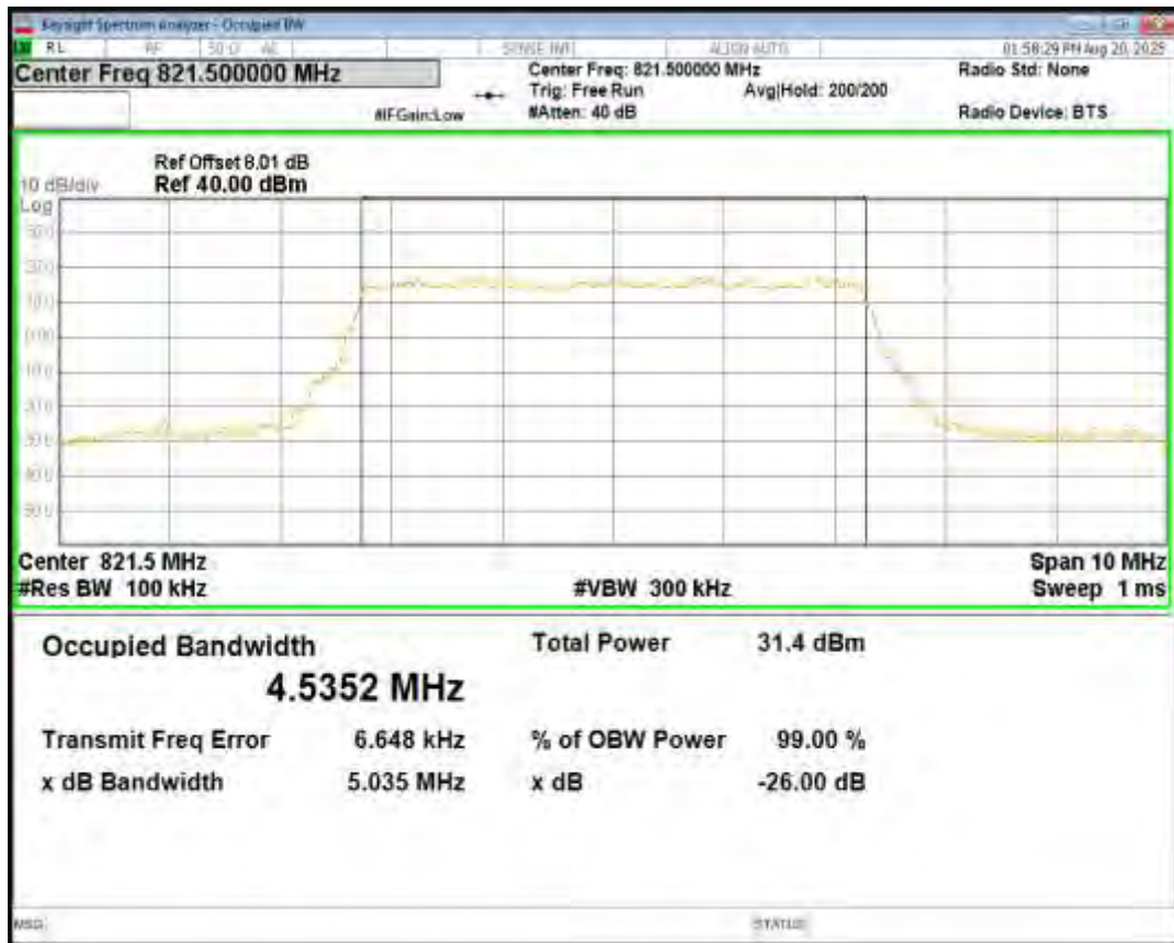
Band26(814-824) 16QAM BW=5MHz Channel=26765 RB Size=25 Position=#0
