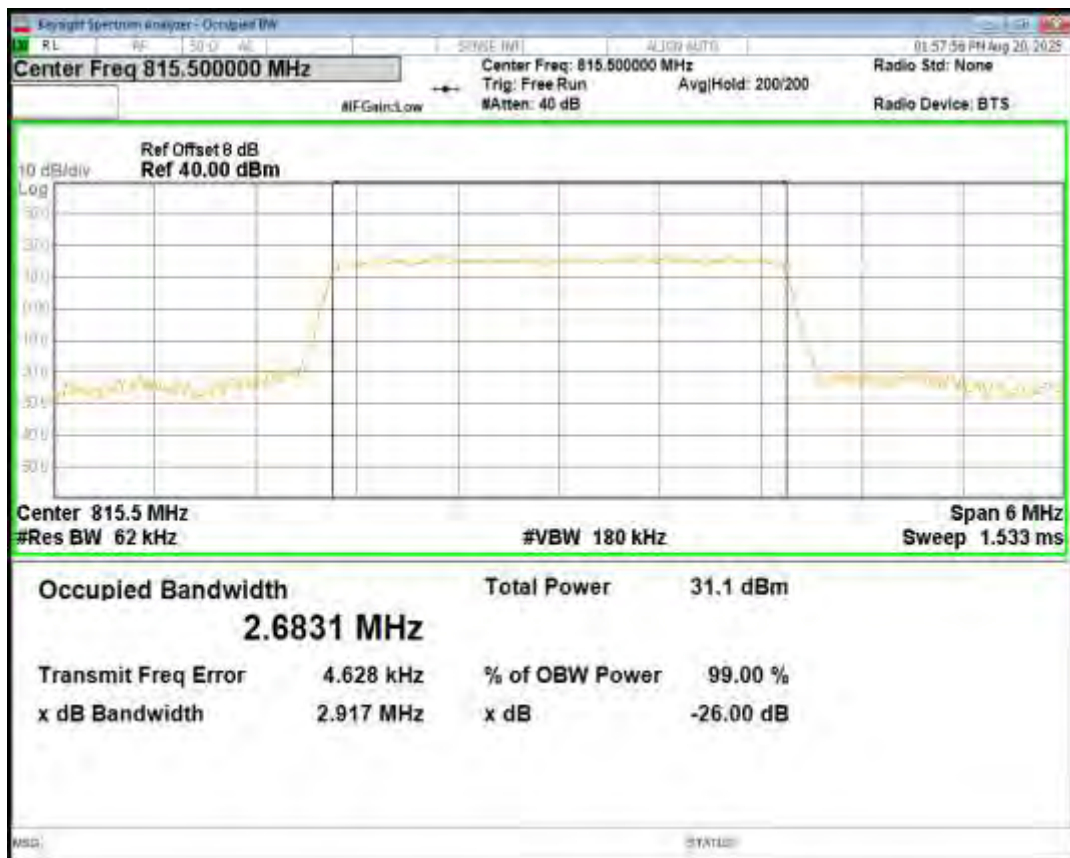
Band26(814-824) QPSK BW=3MHz Channel=26740 RB Size=15 Position=#0
