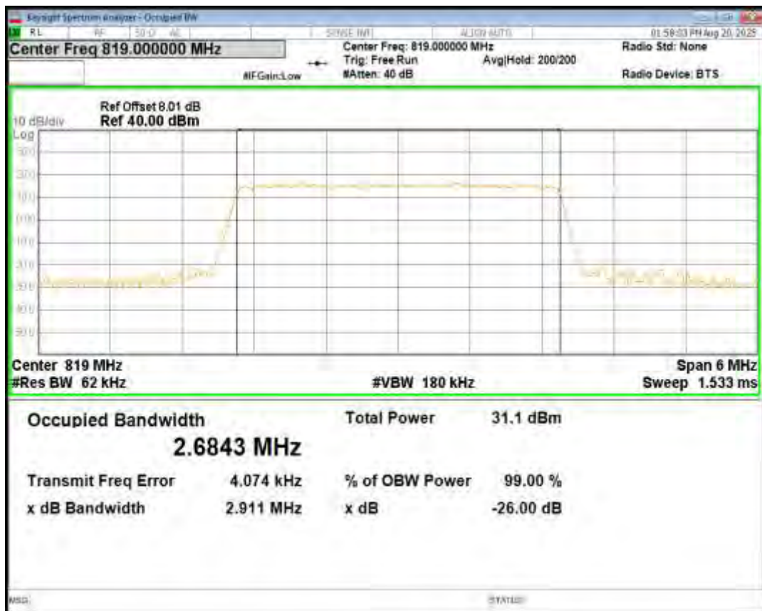
Band26(814-824) QPSK BW=3MHz Channel=26775 RB Size=15 Position=#0
