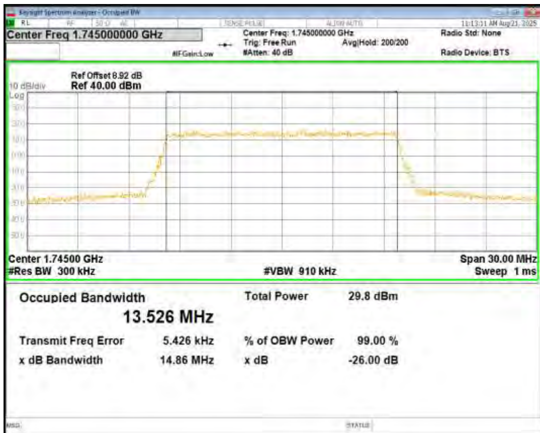
Band66 QPSK BW=15MHz Channel=132597 RB Size=75 Position=#0
