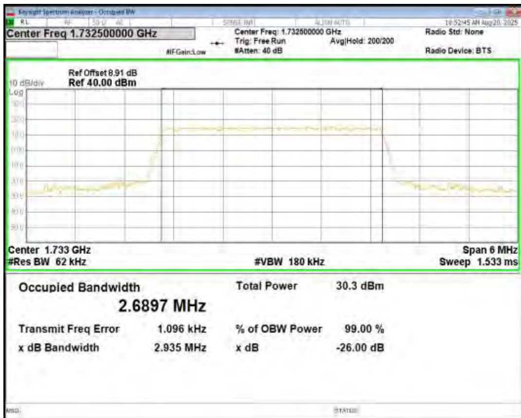
Band4 QPSK BW=3MHz Channel=20385 RB Size=15 Position=#0
