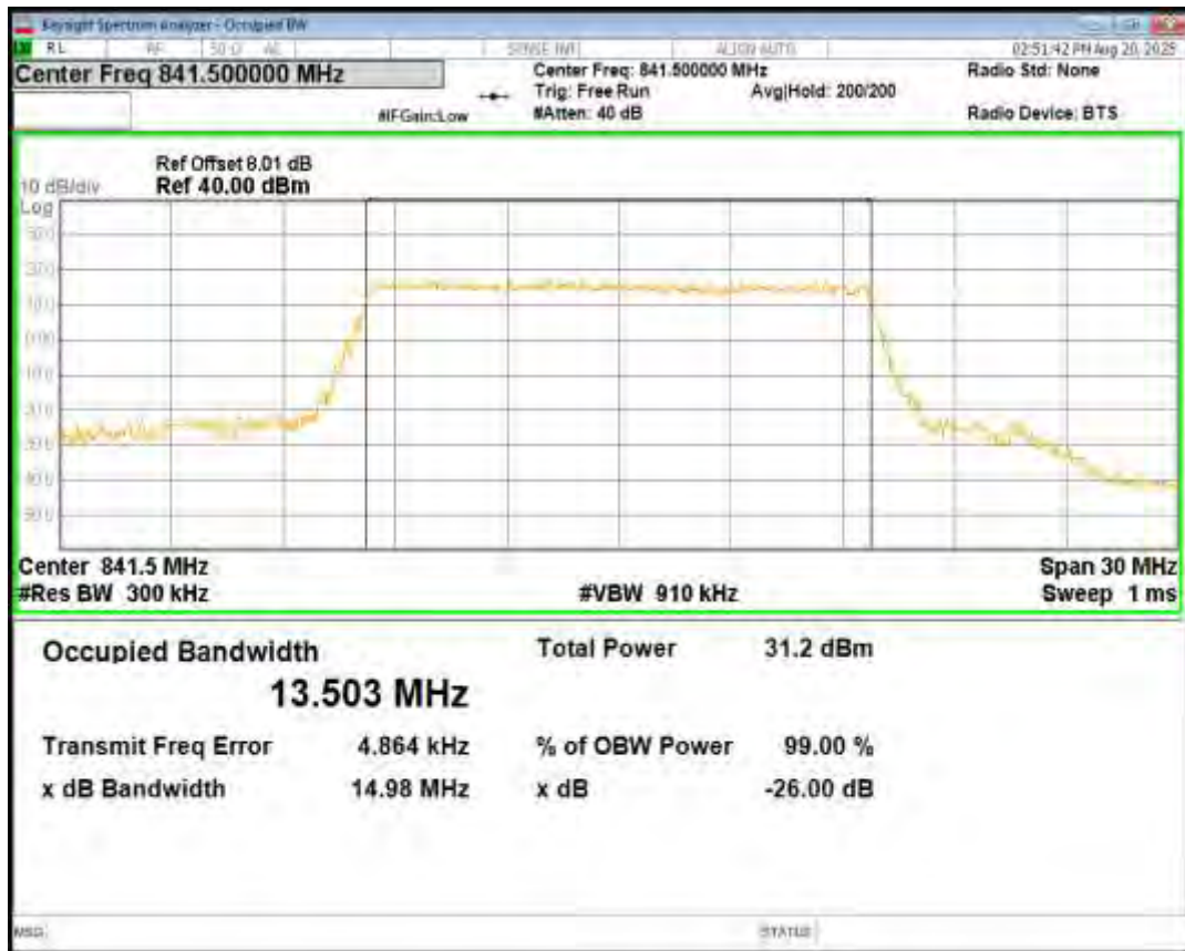
Band26(824-849) 16QAM BW=15MHz Channel=26965 RB Size=75 Position=#0
