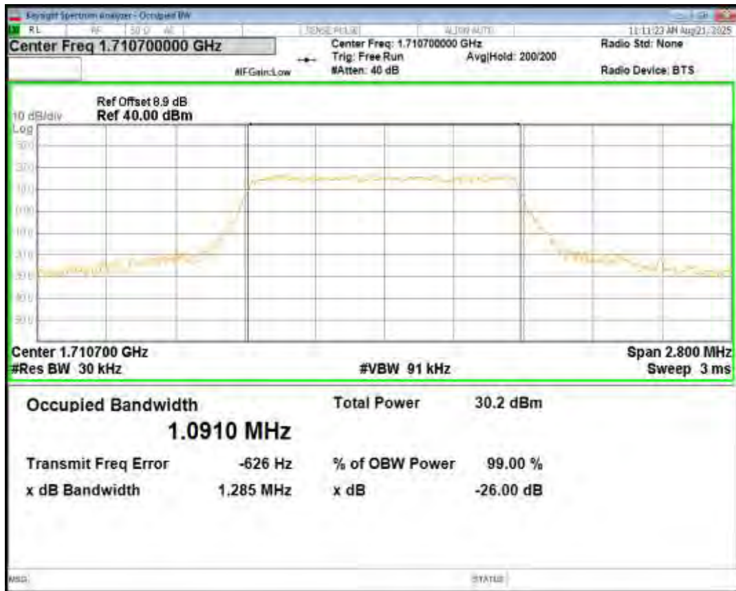
Band66 16QAM BW=1.4MHz Channel=131979 RB Size=6 Position=#0
