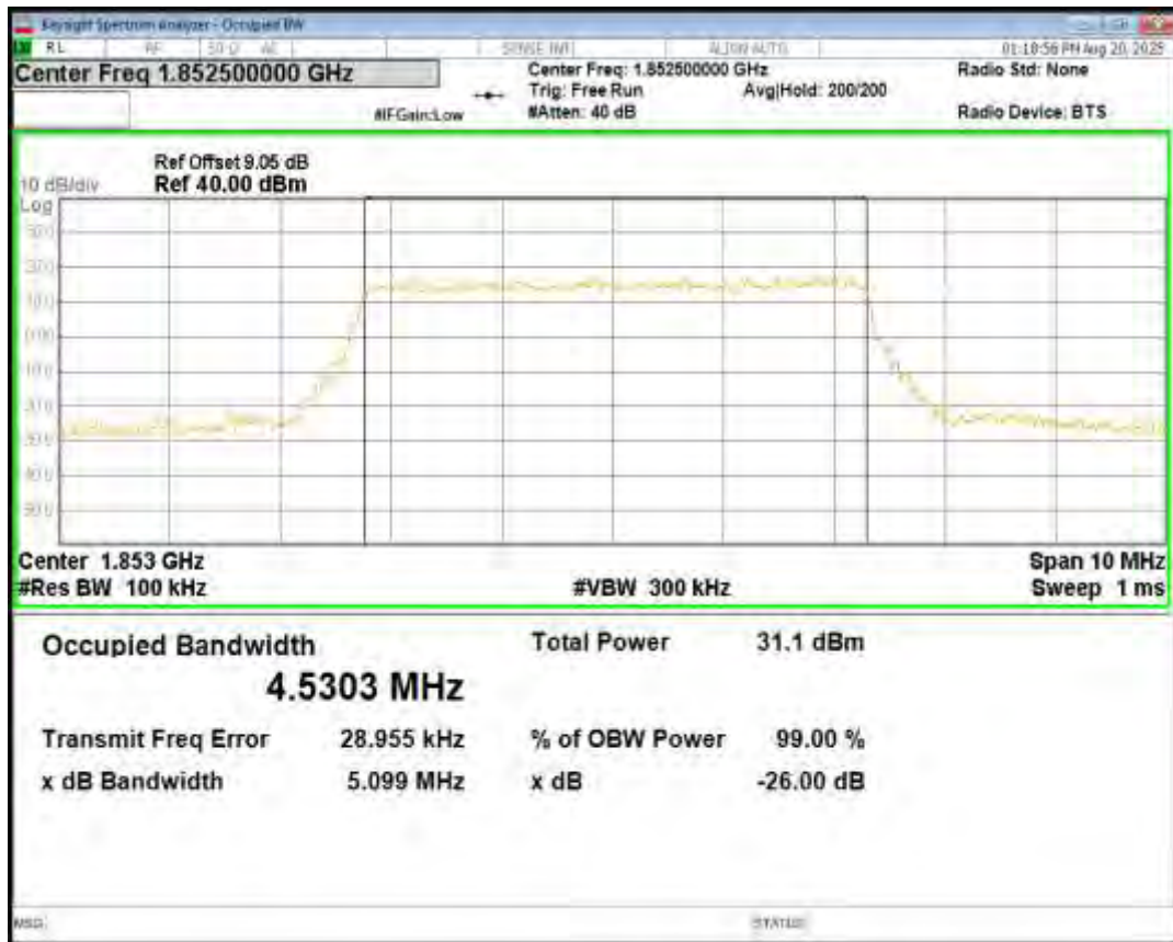
Band25 16QAM BW=5MHz Channel=26065 RB Size=25 Position=#0
