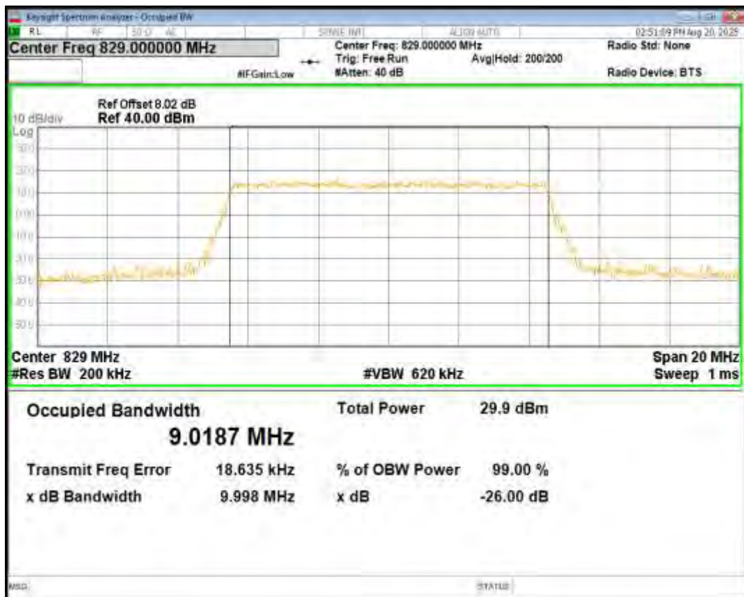
Band26(824-849) QPSK BW=10MHz Channel=26915 RB Size=50 Position=#0
