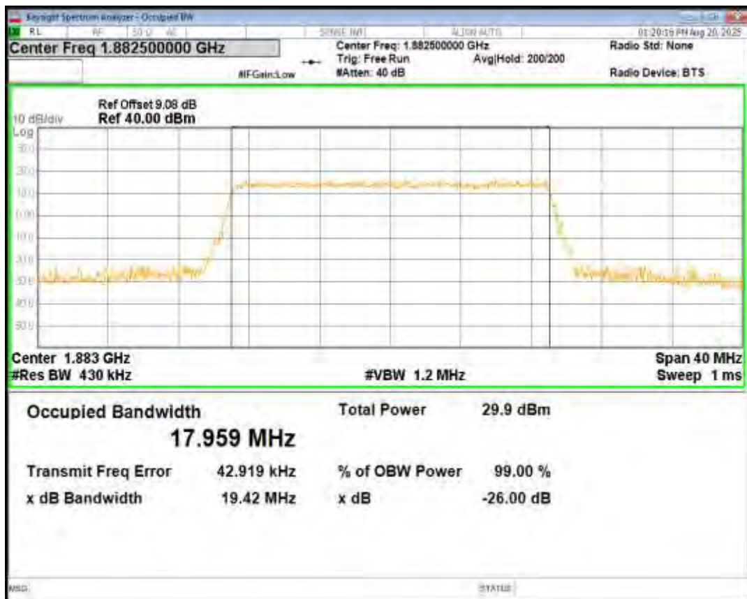
Band25 QPSK BW=20MHz Channel=26590 RB Size=100 Position=#0
