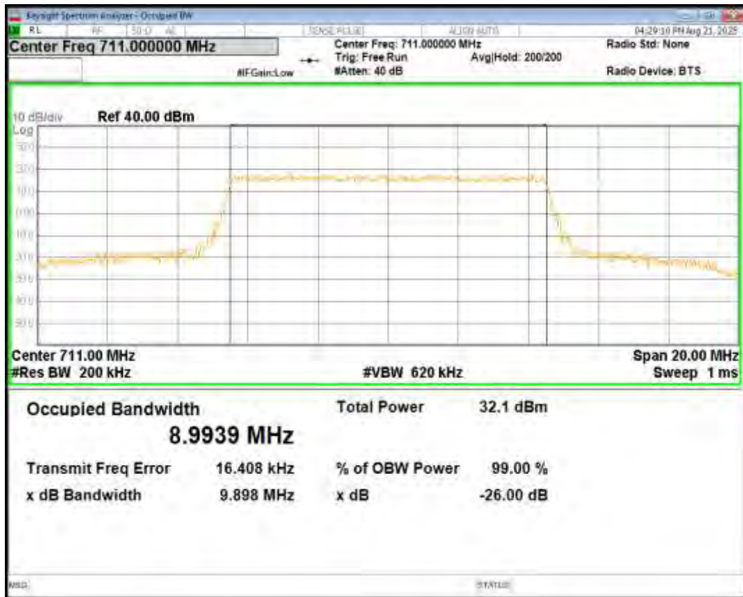
Band12 16QAM BW=10MHz Channel=23130 RB Size=50 Position=#0
