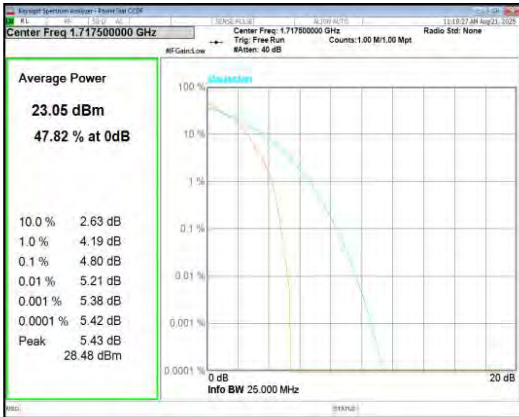
Band66 16QAM BW=15MHz Channel=132047 RB Size=1 Position=#0
