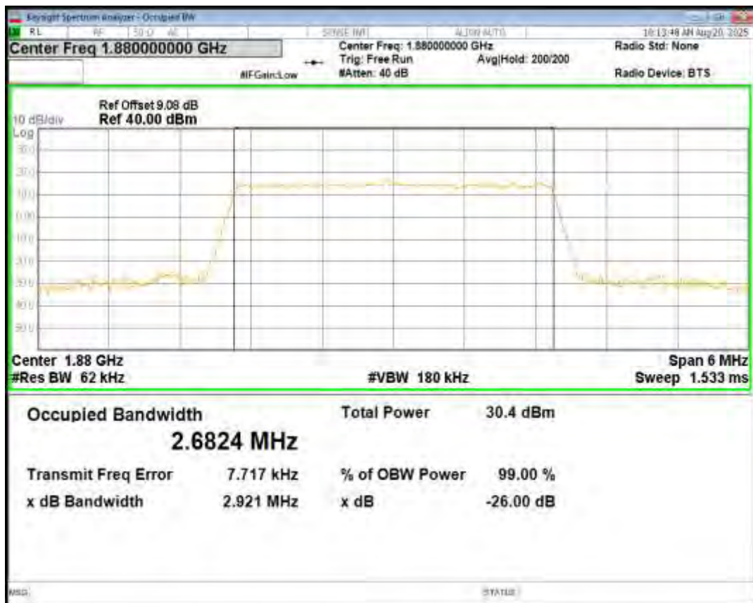
Band2 QPSK BW=3MHz Channel=19185 RB Size=15 Position=#0
