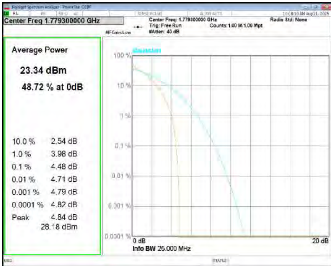
Band66 16QAM BW=1.4MHz Channel=132665 RB Size=1 Position=#0
