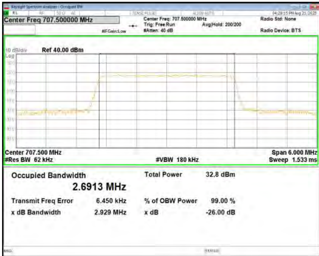
Band12 16QAM BW=3MHz Channel=23095 RB Size=15 Position=#0
