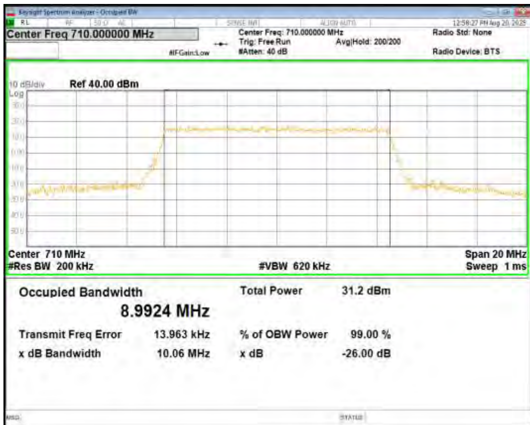
Band17 QPSK BW=10MHz Channel=23800 RB Size=50 Position=#0
