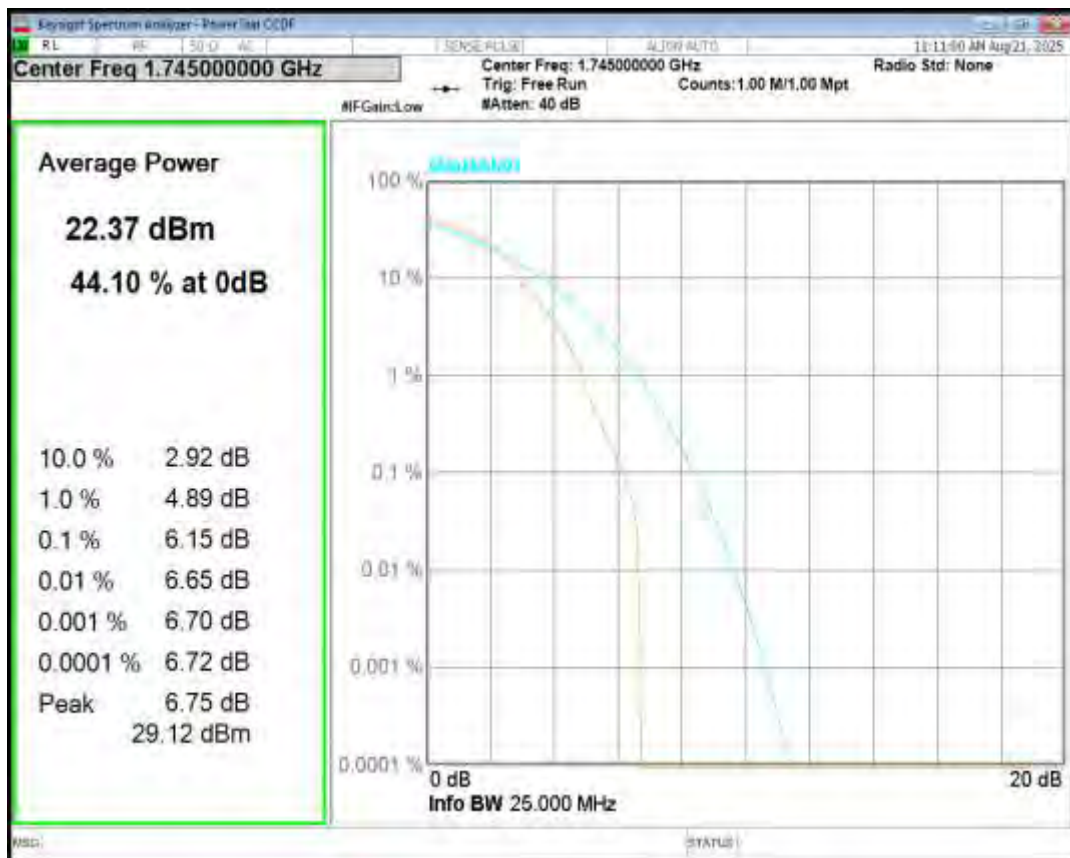
Band66 QPSK BW=20MHz Channel=132572 RB Size=1 Position=#0
