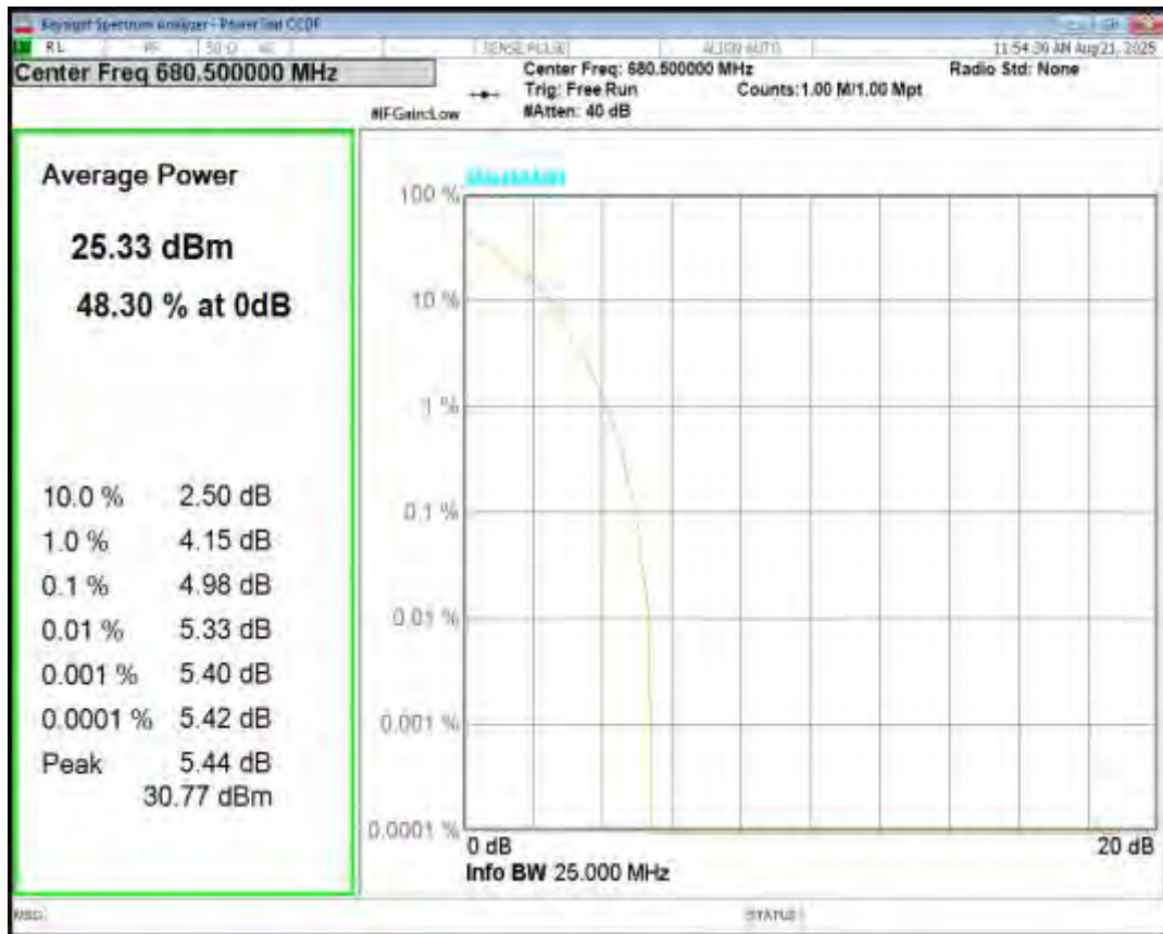
Band71 16QAM BW=15MHz Channel=133297 RB Size=1 Position=#0
