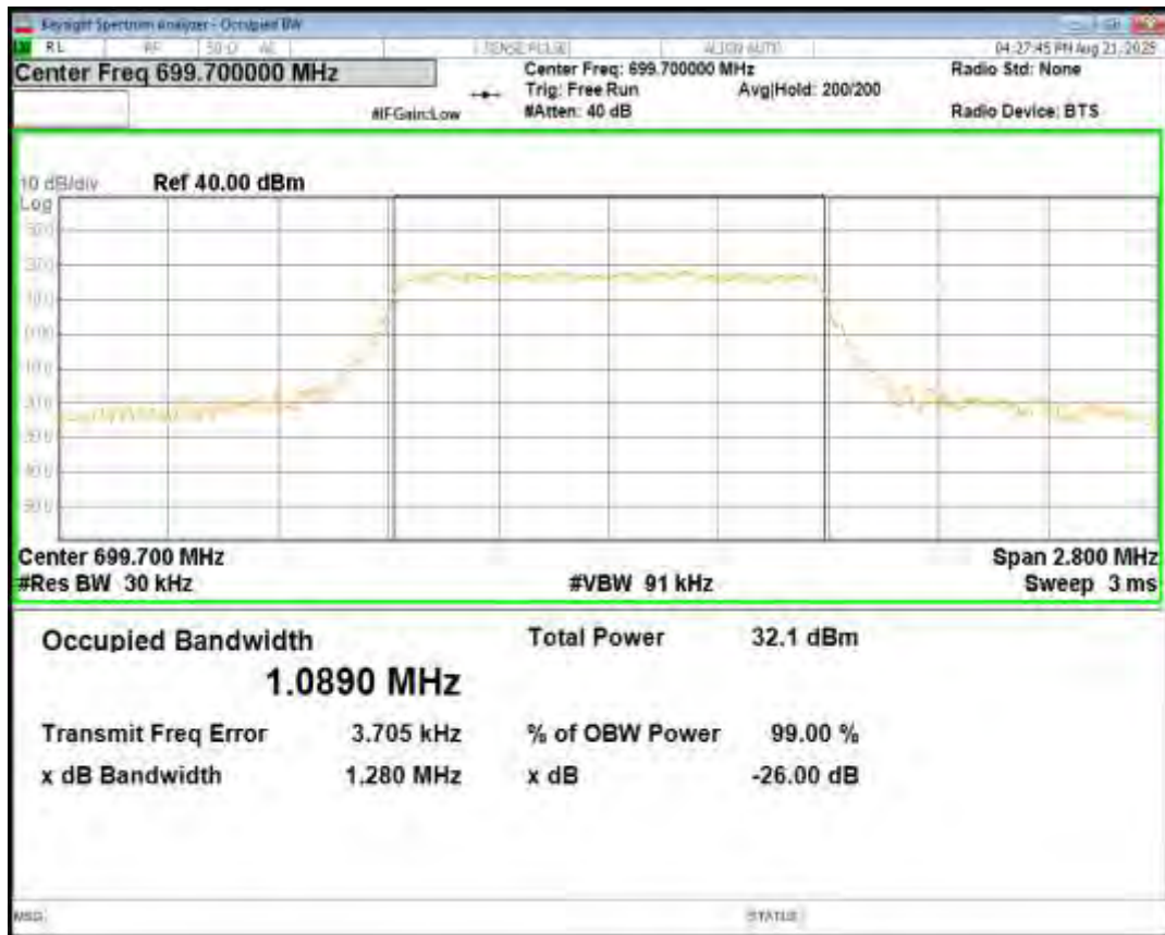
Band12 16QAM BW=1.4MHz Channel=23017 RB Size=6 Position=#0
