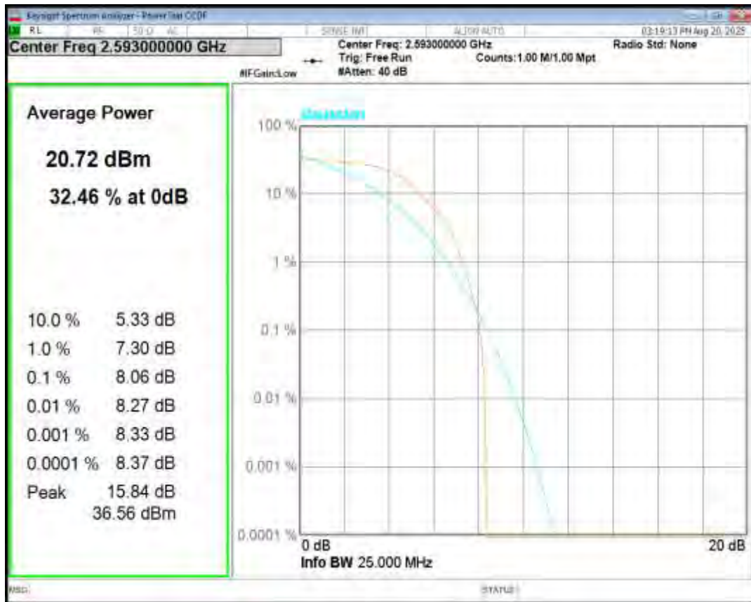
Band41 16QAM BW=10MHz Channel=40620 RB Size=1 Position=#0
