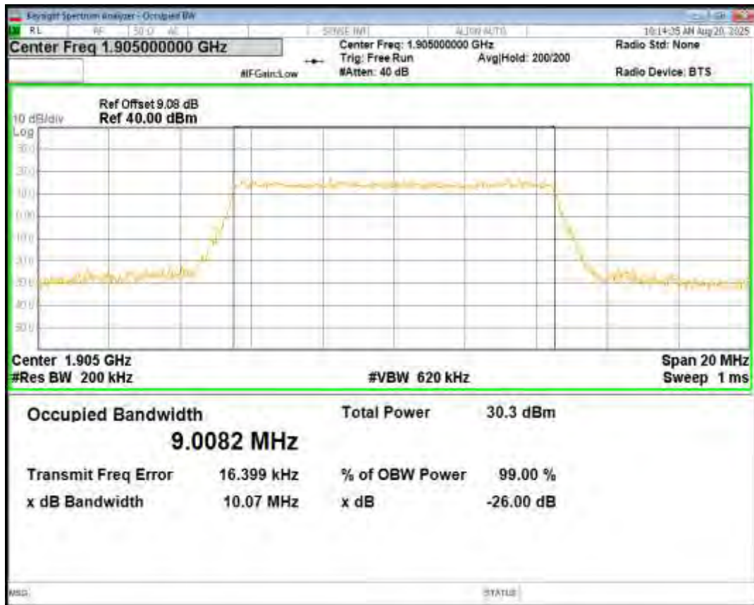
Band2 16QAM BW=10MHz Channel=19150 RB Size=50 Position=#0
