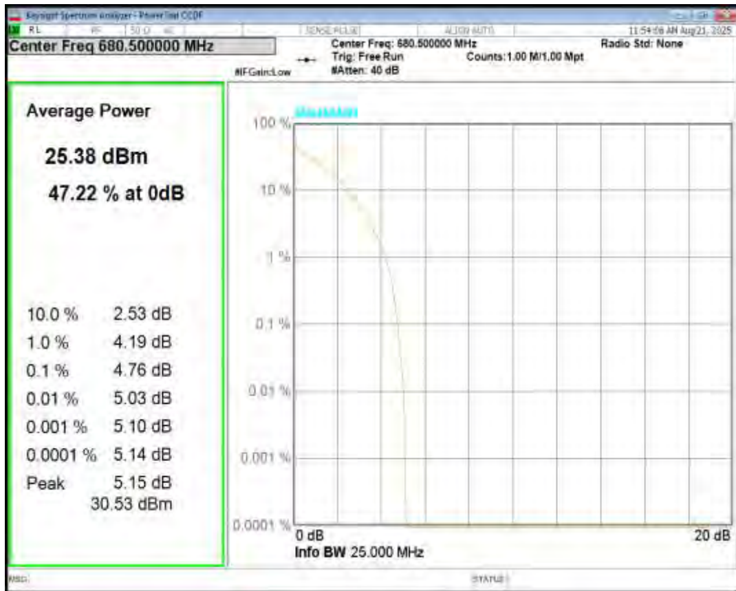
Band71 16QAM BW=10MHz Channel=133297 RB Size=1 Position=#0
