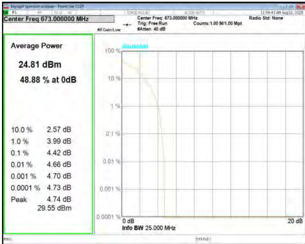
Band71 16QAM BW=20MHz Channel=133222 RB Size=1 Position=#0
