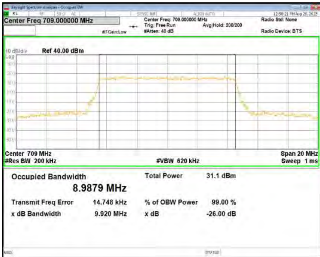
Band17 QPSK BW=10MHz Channel=23790 RB Size=50 Position=#0
