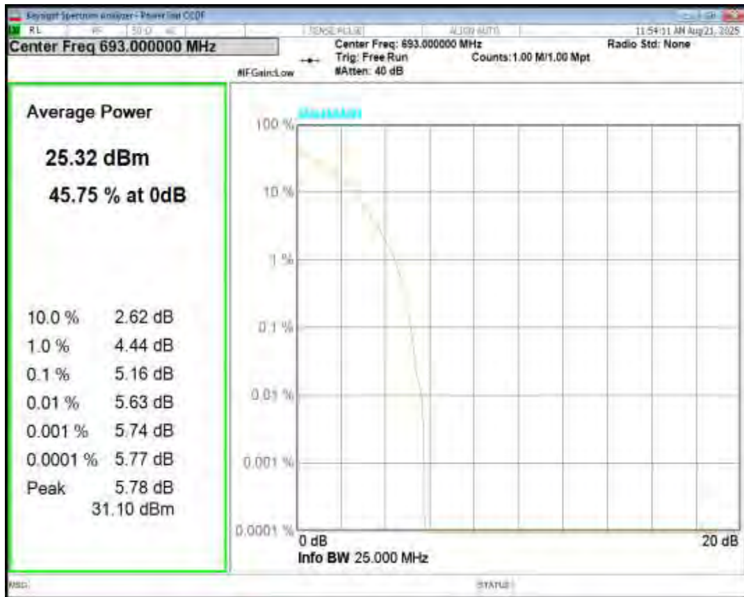
Band71 16QAM BW=10MHz Channel=133422 RB Size=1 Position=#0
