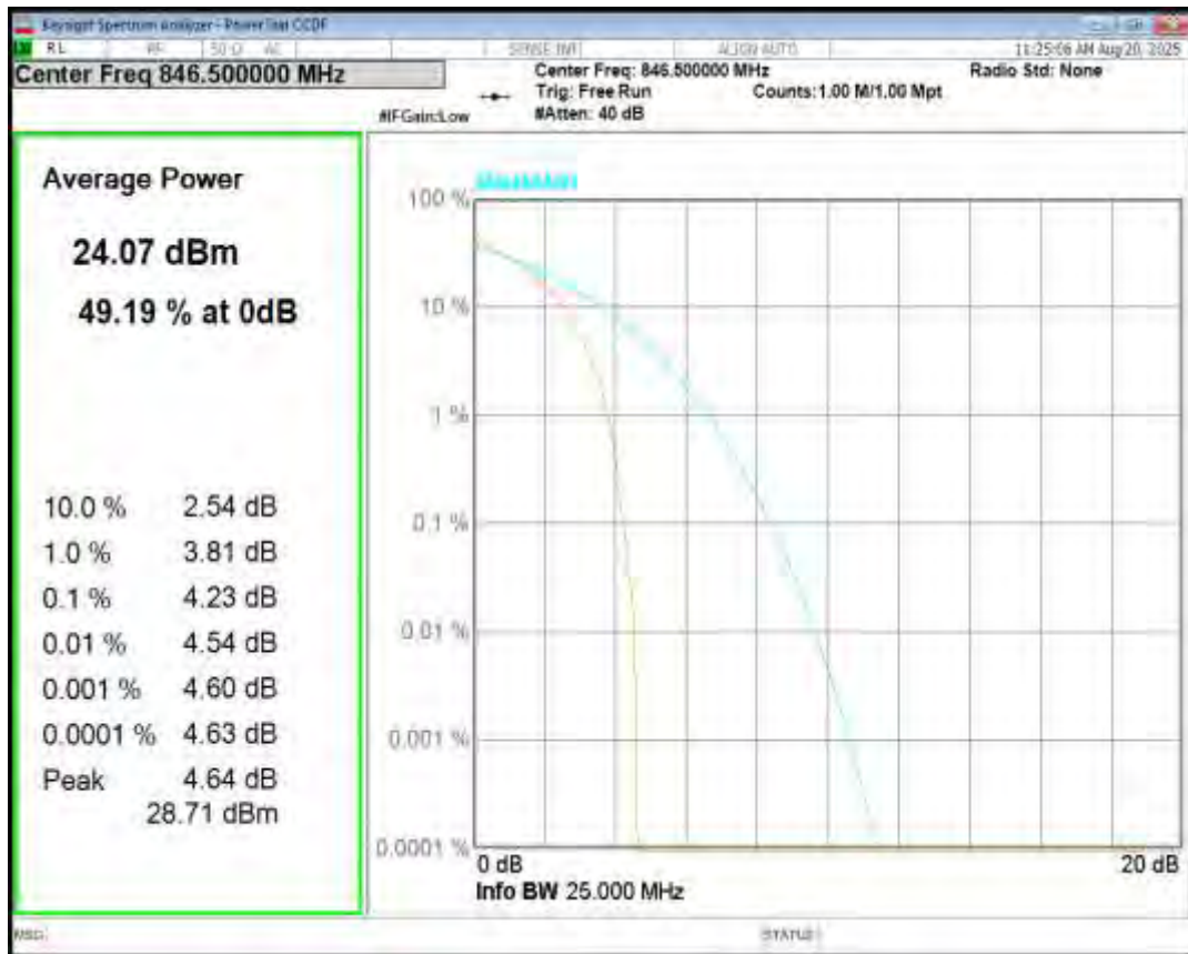
Band5 16QAM BW=5MHz Channel=20625 RB Size=1 Position=#0
