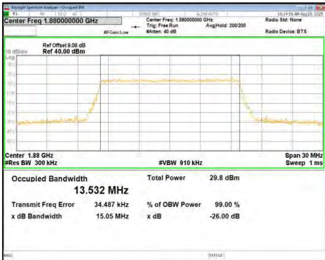
Band2 QPSK BW=15MHz Channel=19125 RB Size=75 Position=#0
