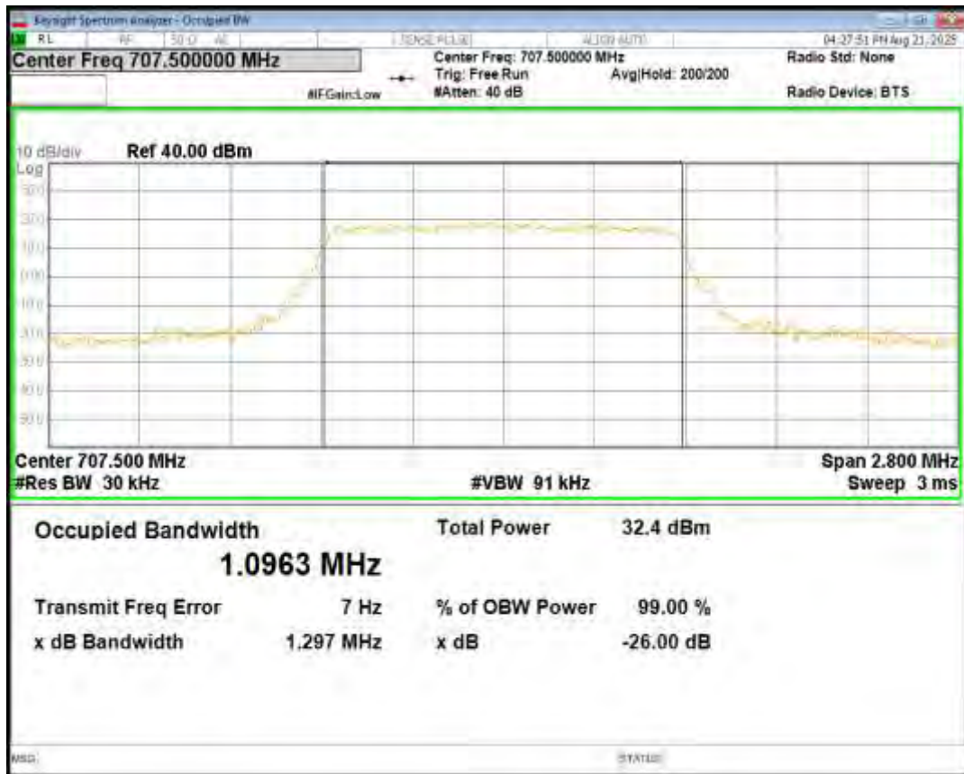
Band12 16QAM BW=1.4MHz Channel=23095 RB Size=6 Position=#0
