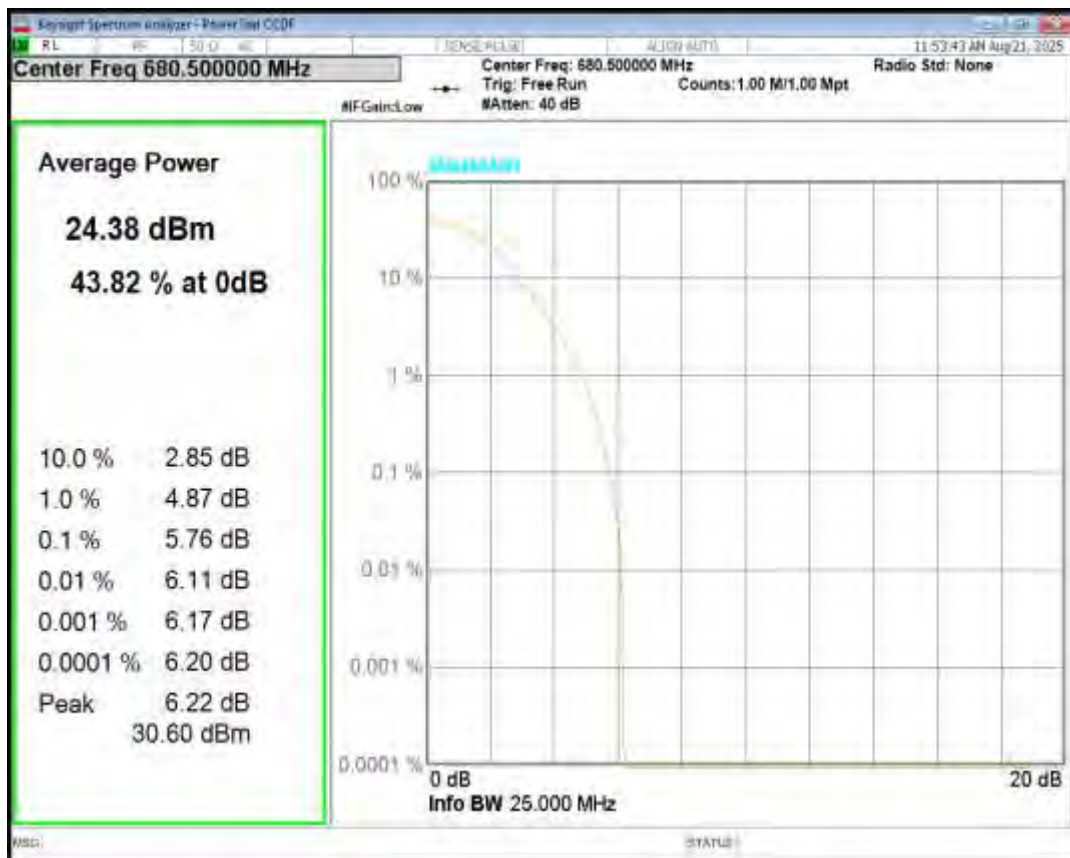
Band71 QPSK BW=5MHz Channel=133447 RB Size=1 Position=#0
