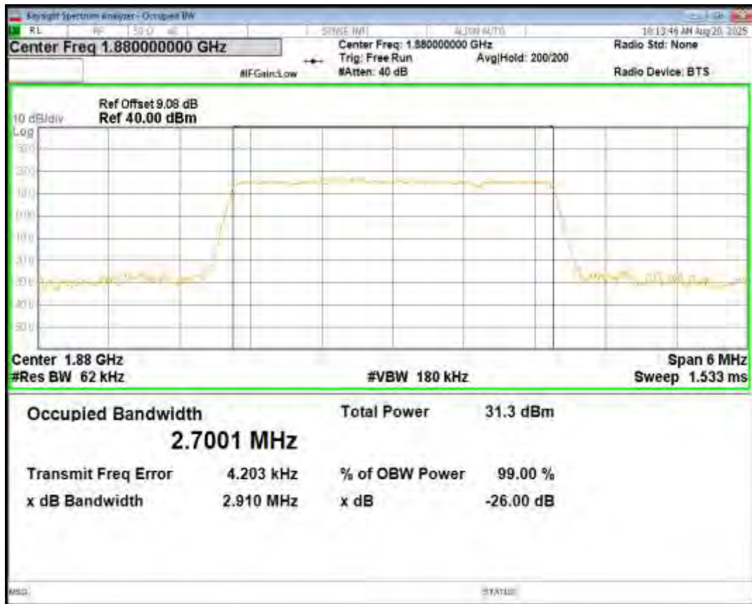
Band2 16QAM BW=3MHz Channel=18900 RB Size=15 Position=#0
