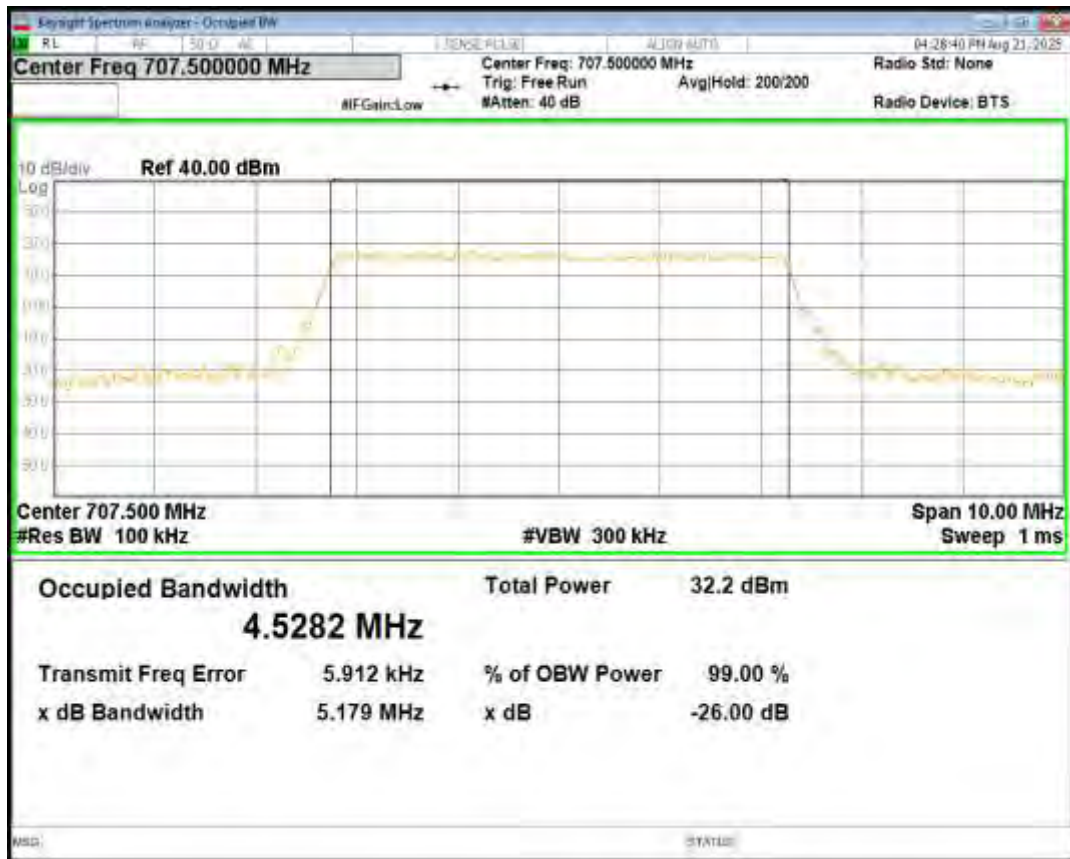
Band12 16QAM BW=5MHz Channel=23095 RB Size=25 Position=#0
