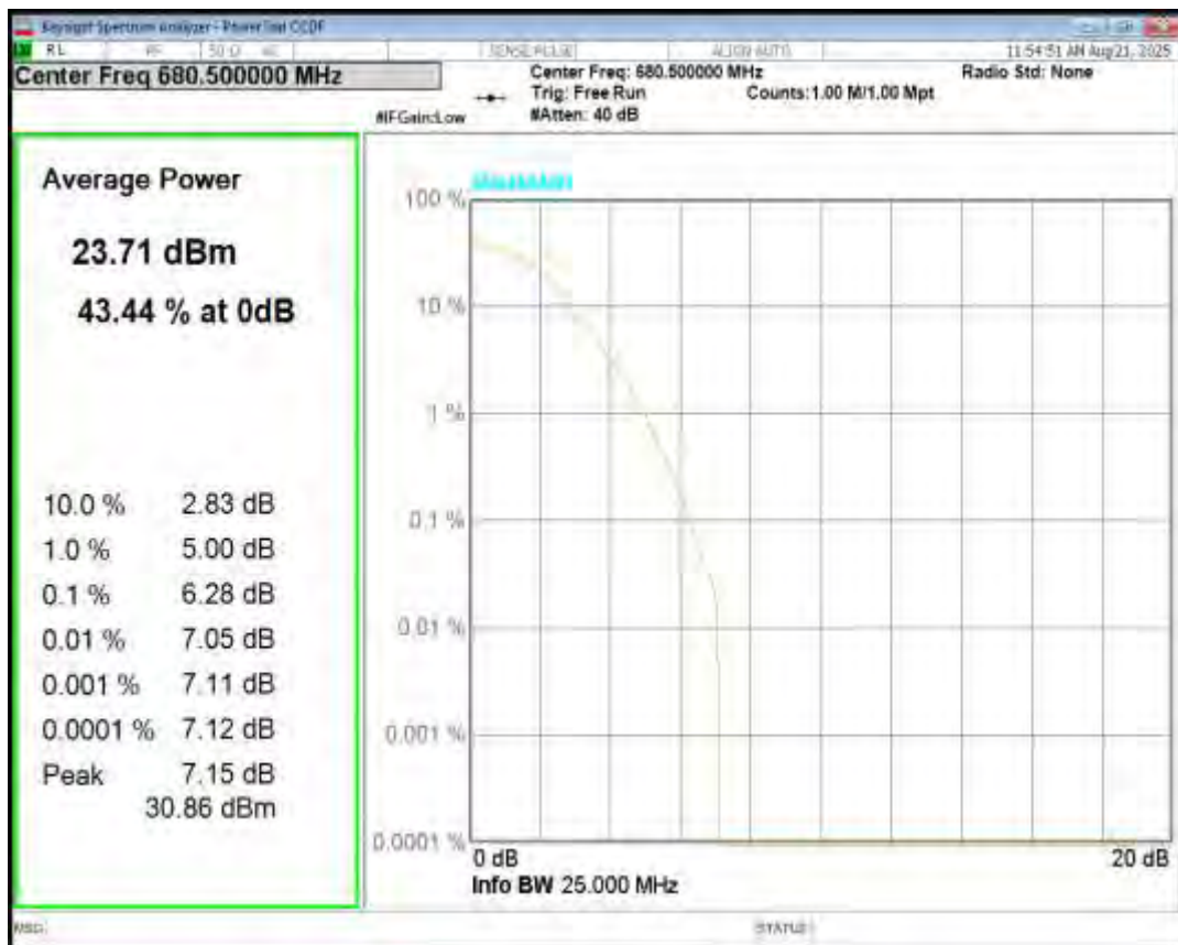
Band71 QPSK BW=20MHz Channel=133372 RB Size=1 Position=#0
