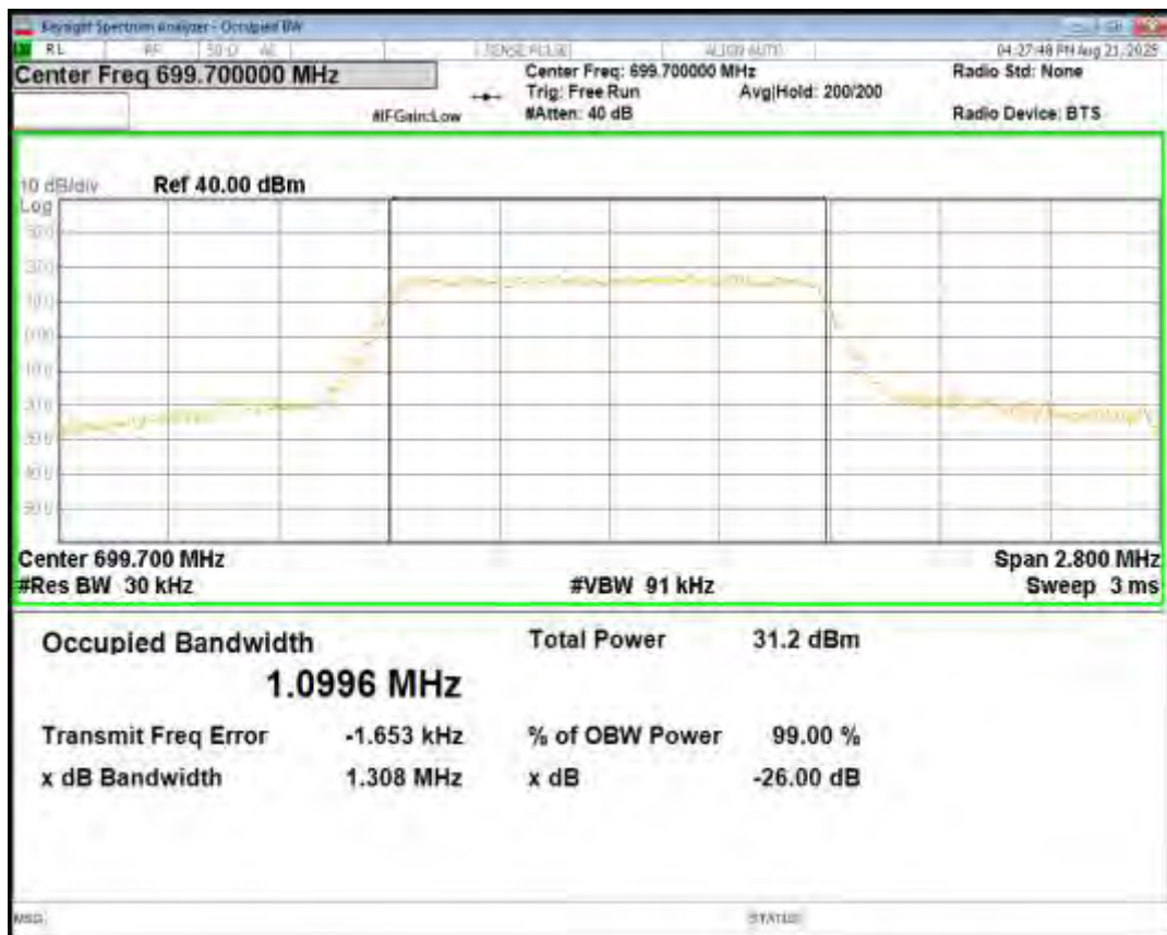
Band12 QPSK BW=1.4MHz Channel=23095 RB Size=6 Position=#0
