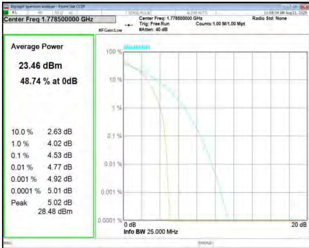
Band66 16QAM BW=3MHz Channel=132657 RB Size=1 Position=#0
