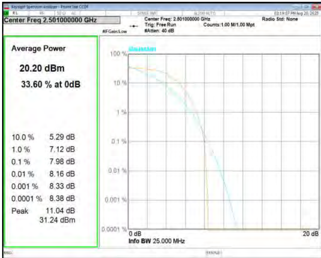
Band41 16QAM BW=10MHz Channel=39700 RB Size=1 Position=#0
