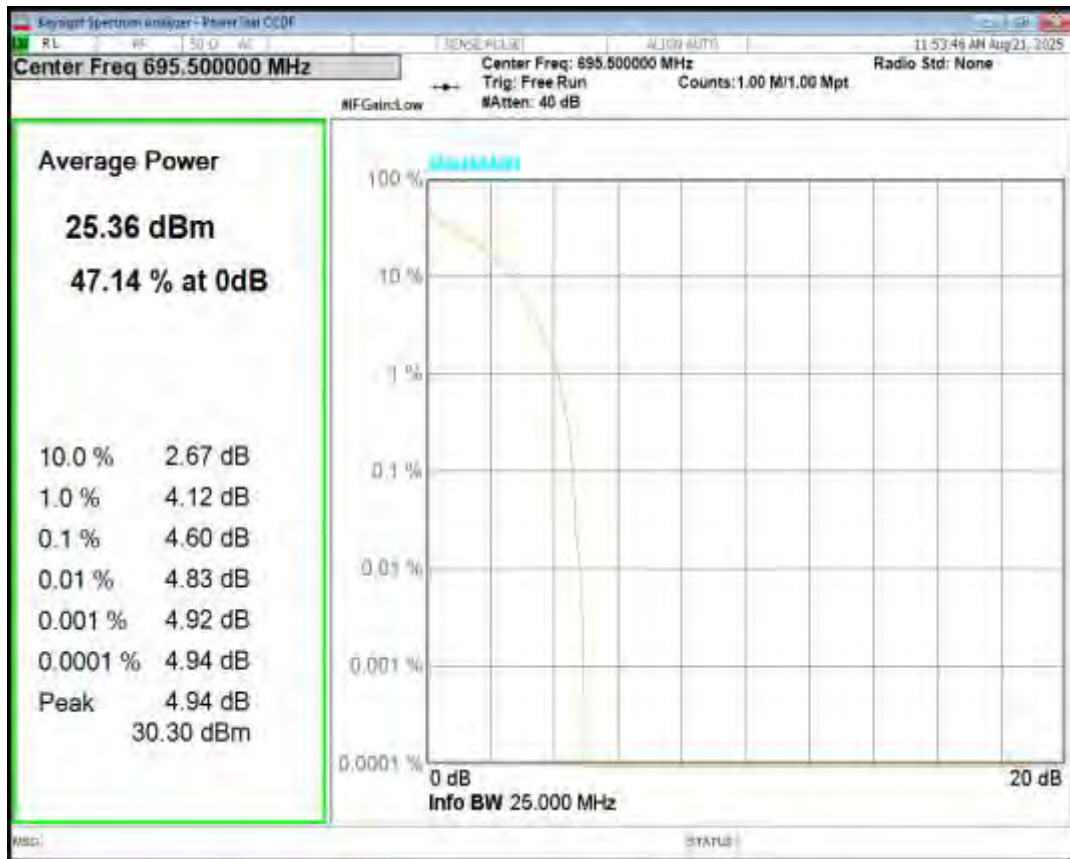
Band71 16QAM BW=5MHz Channel=133447 RB Size=1 Position=#0
