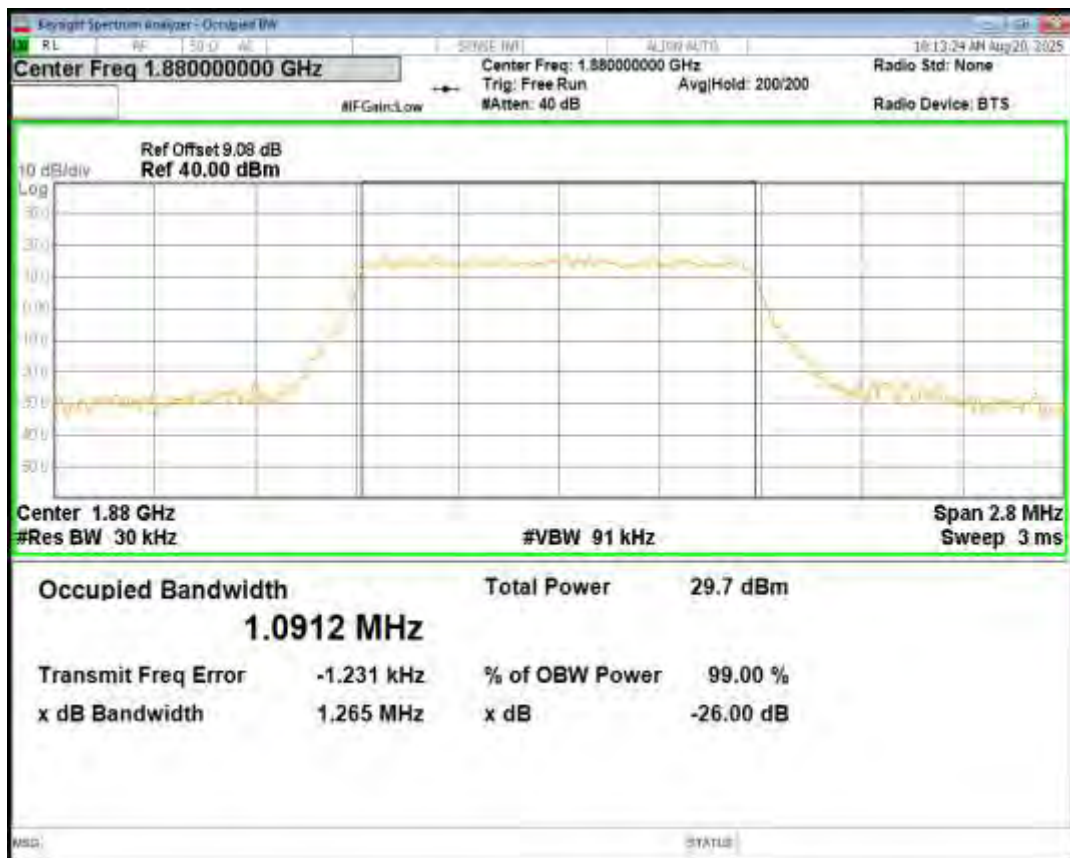
Band2 QPSK BW=1.4MHz Channel=19193 RB Size=6 Position=#0
