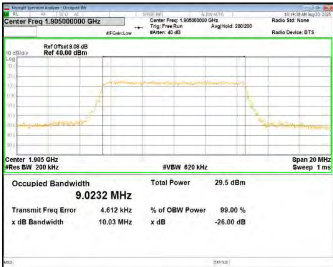
Band2 QPSK BW=15MHz Channel=18675 RB Size=75 Position=#0
