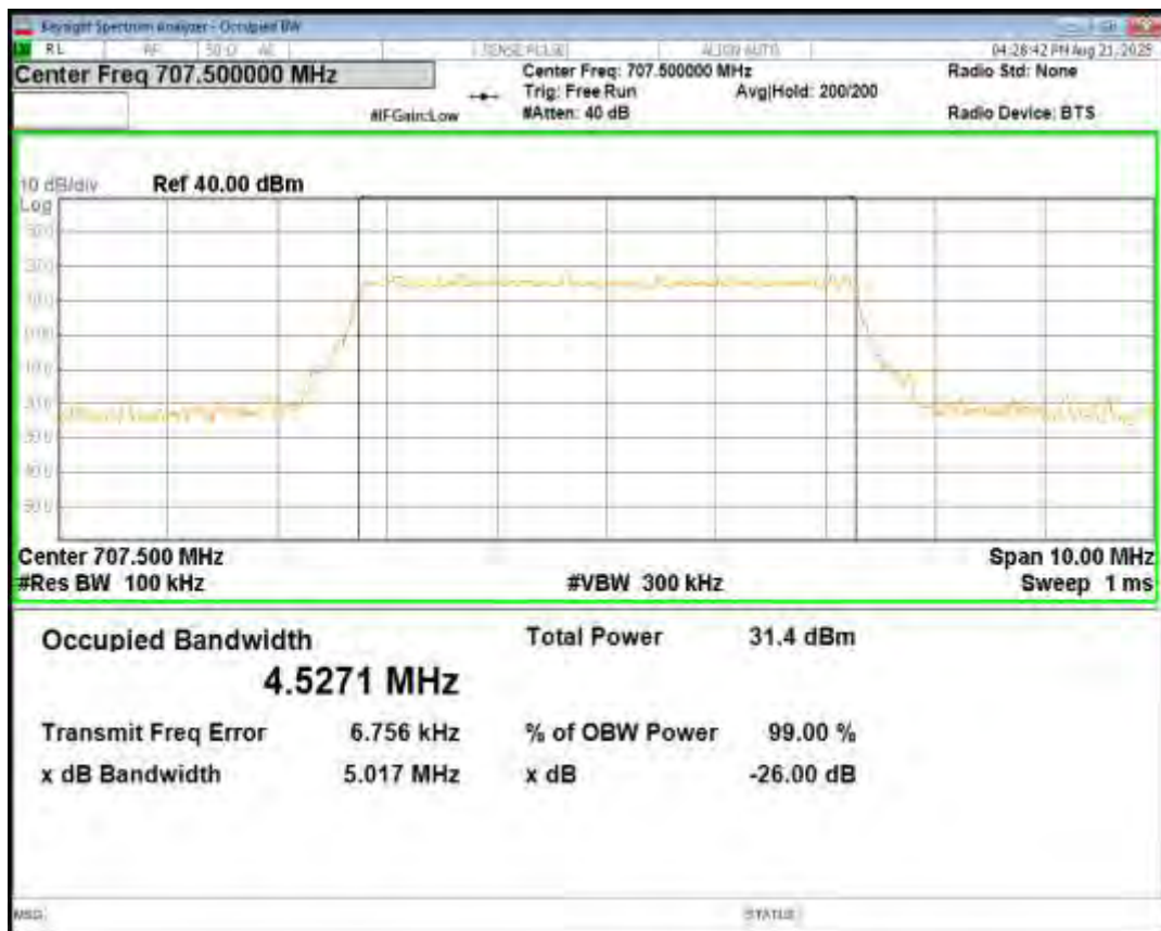
Band12 QPSK BW=5MHz Channel=23155 RB Size=25 Position=#0
