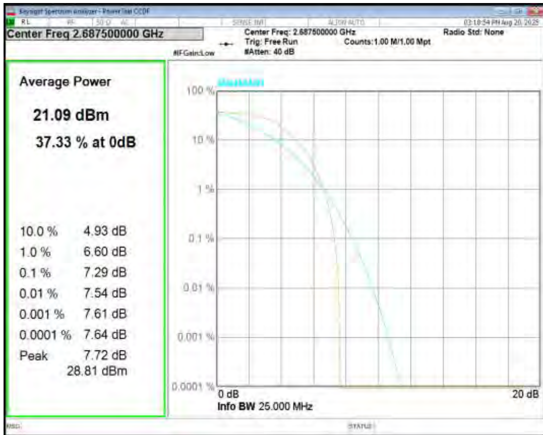
Band41 16QAM BW=5MHz Channel=41565 RB Size=1 Position=#0
