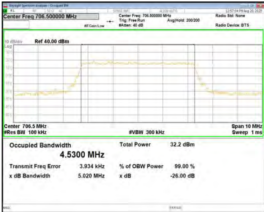
Band17 16QAM BW=5MHz Channel=23755 RB Size=25 Position=#0
