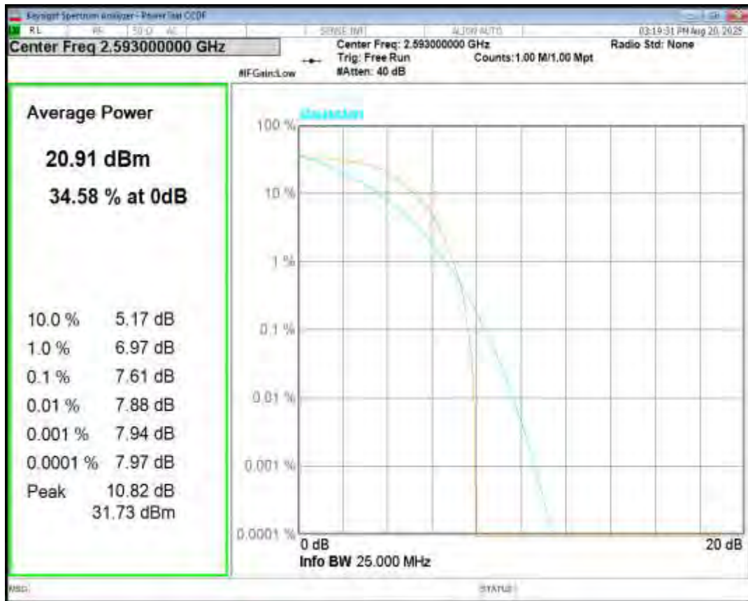
Band41 16QAM BW=15MHz Channel=40620 RB Size=1 Position=#0
