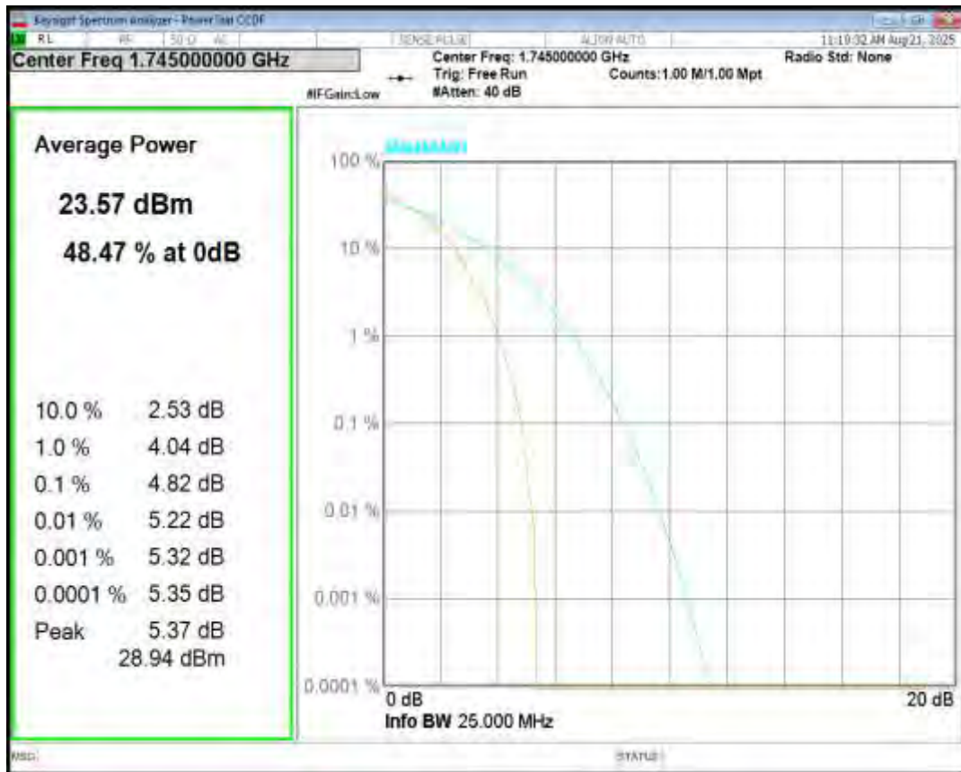
Band66 16QAM BW=15MHz Channel=132322 RB Size=1 Position=#0
