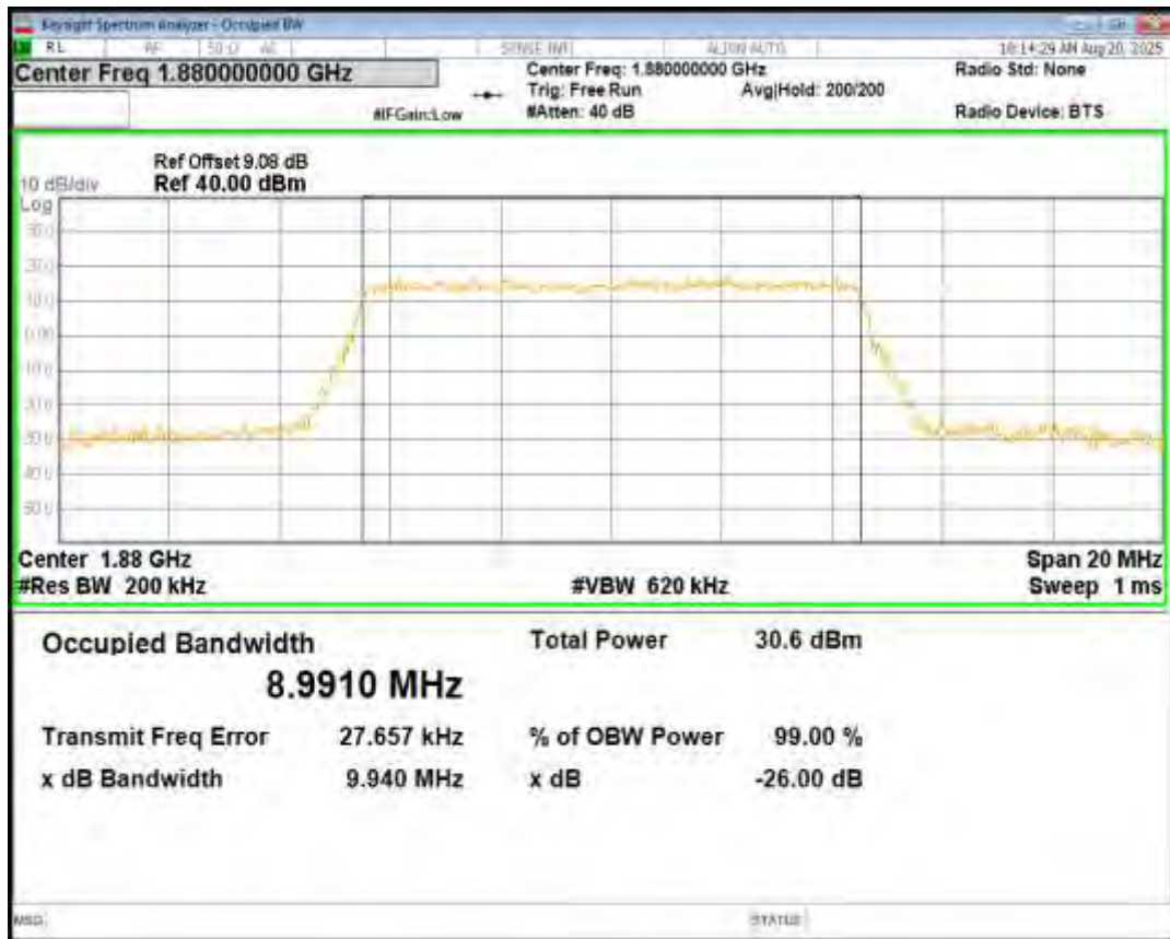
Band2 16QAM BW=10MHz Channel=18900 RB Size=50 Position=#0
