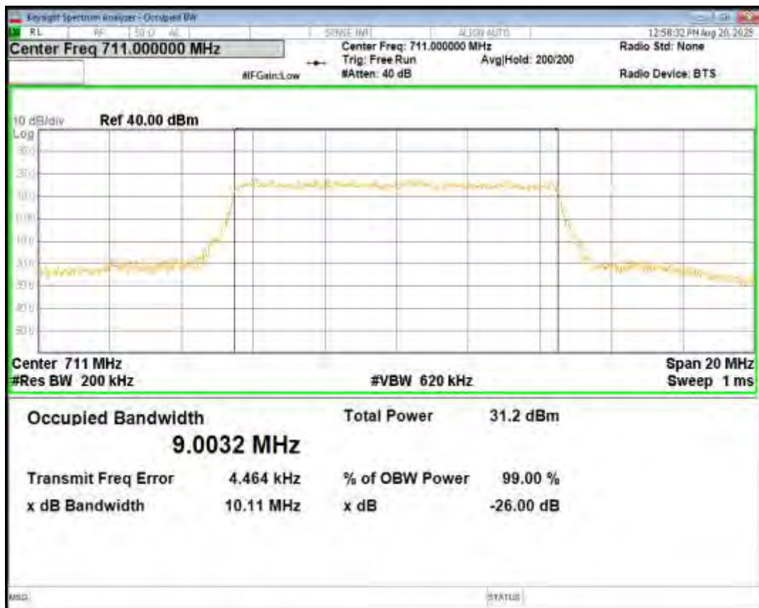
Band2 QPSK BW=1.4MHz Channel=18607 RB Size=6 Position=#0
