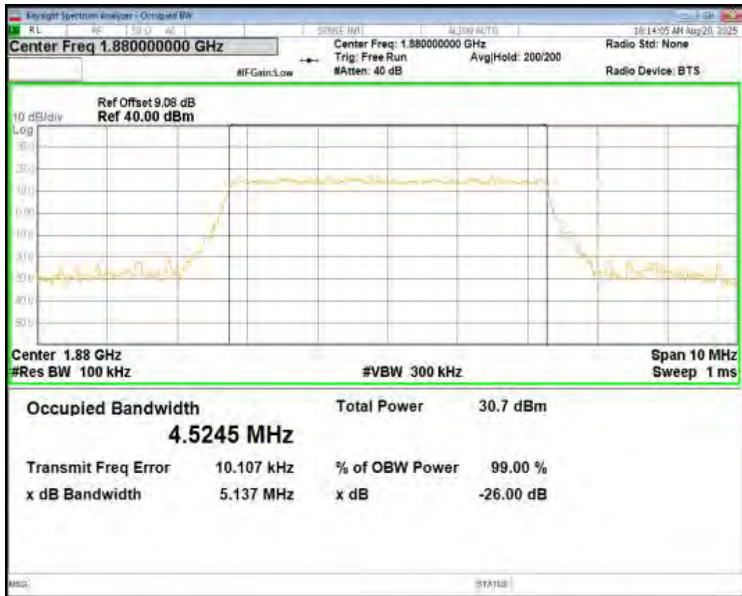
Band2 16QAM BW=5MHz Channel=18900 RB Size=25 Position=#0
