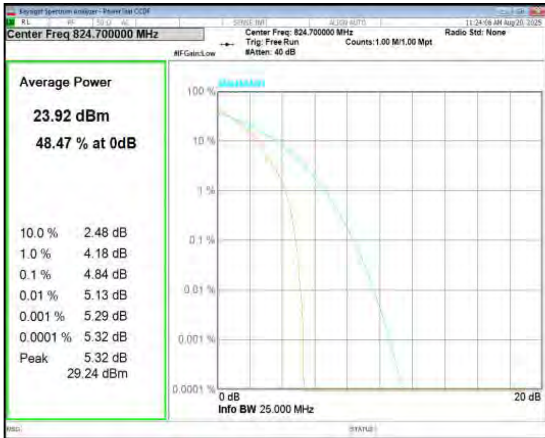
Band5 16QAM BW=1.4MHz Channel=20407 RB Size=1 Position=#0
