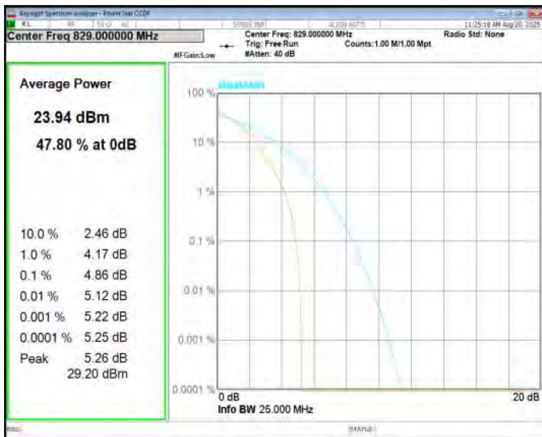
Band5 16QAM BW=10MHz Channel=20450 RB Size=1 Position=#0
