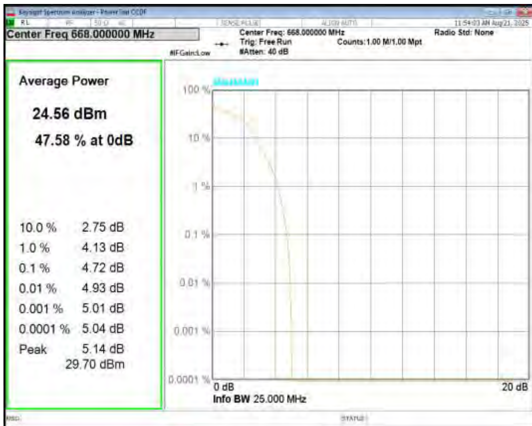
Band71 QPSK BW=10MHz Channel=133297 RB Size=1 Position=#0
