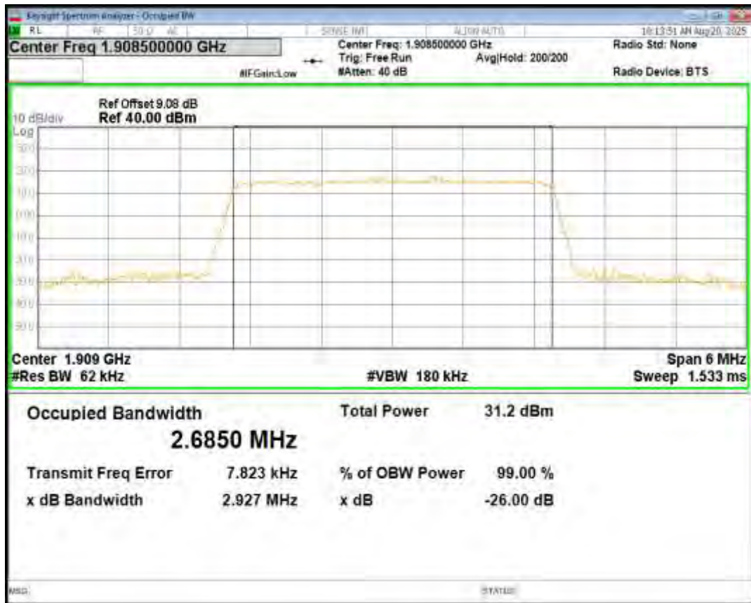
Band2 16QAM BW=3MHz Channel=19185 RB Size=15 Position=#0
