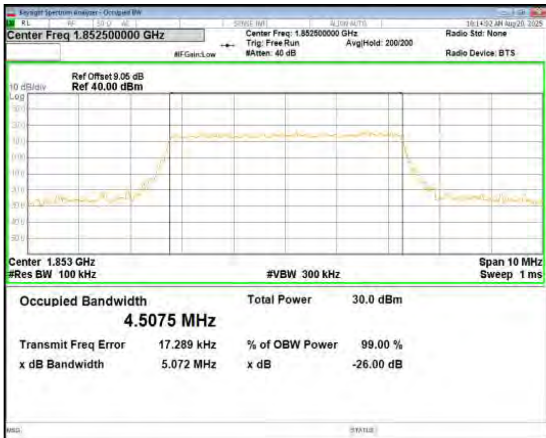
Band2 QPSK BW=5MHz Channel=18900 RB Size=25 Position=#0
