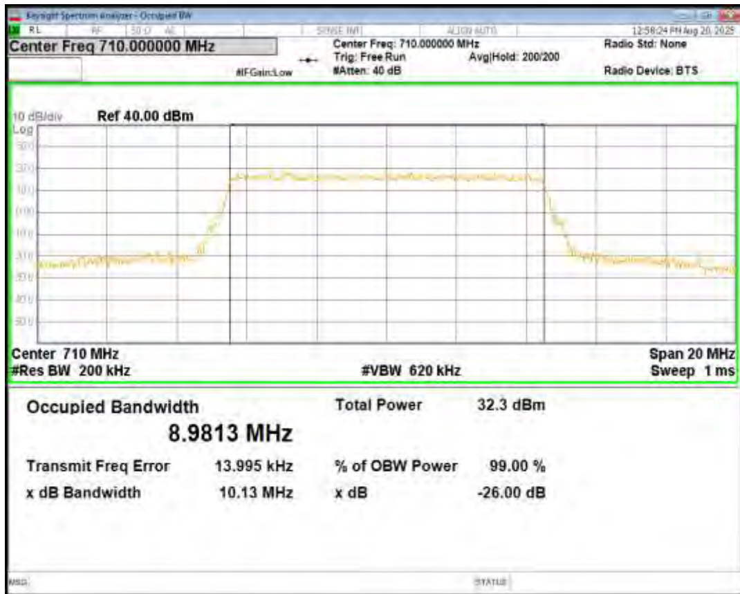
Band17 16QAM BW=10MHz Channel=23790 RB Size=50 Position=#0
