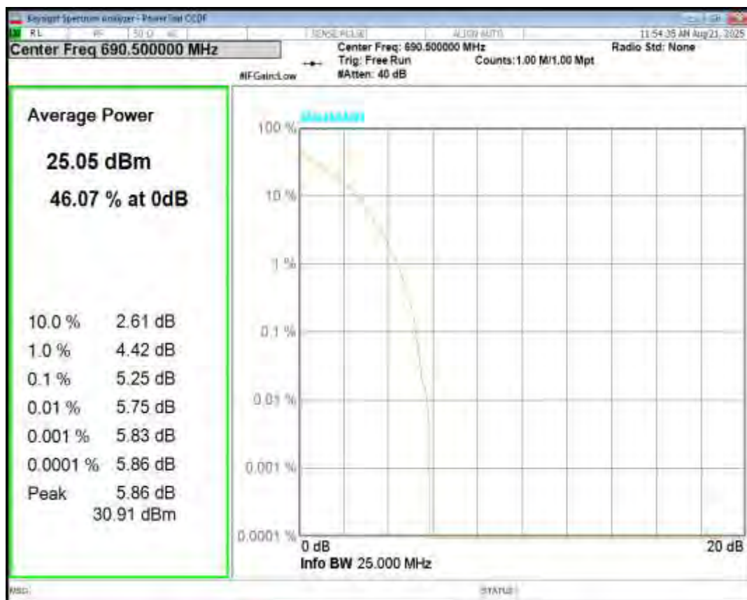
Band71 16QAM BW=15MHz Channel=133397 RB Size=1 Position=#0
