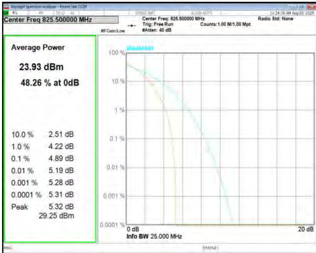
Band5 16QAM BW=3MHz Channel=20415 RB Size=1 Position=#0
