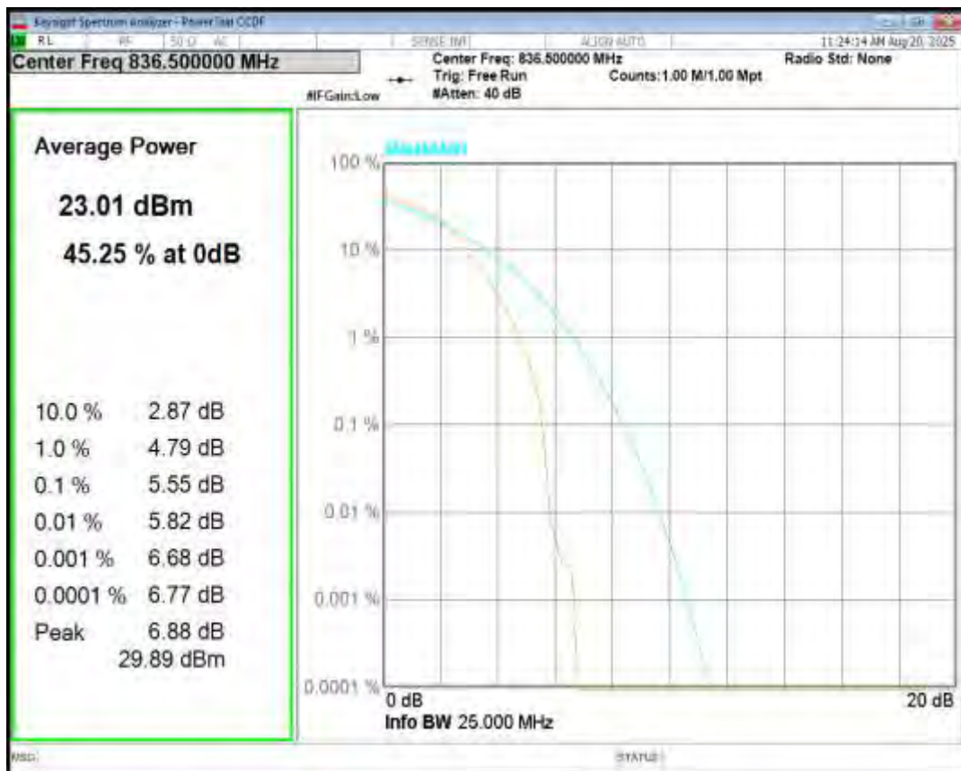
Band5 QPSK BW=1.4MHz Channel=20643 RB Size=1 Position=#0
