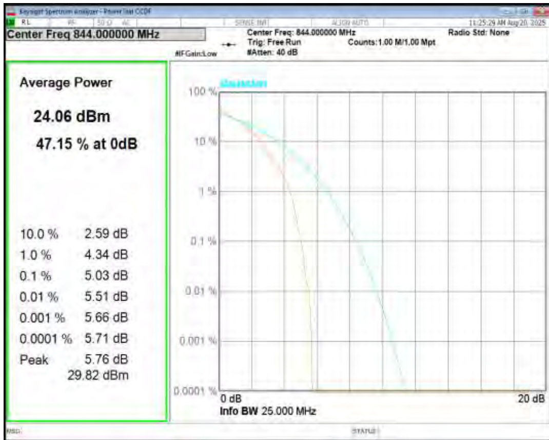
Band5 16QAM BW=10MHz Channel=20600 RB Size=1 Position=#0
