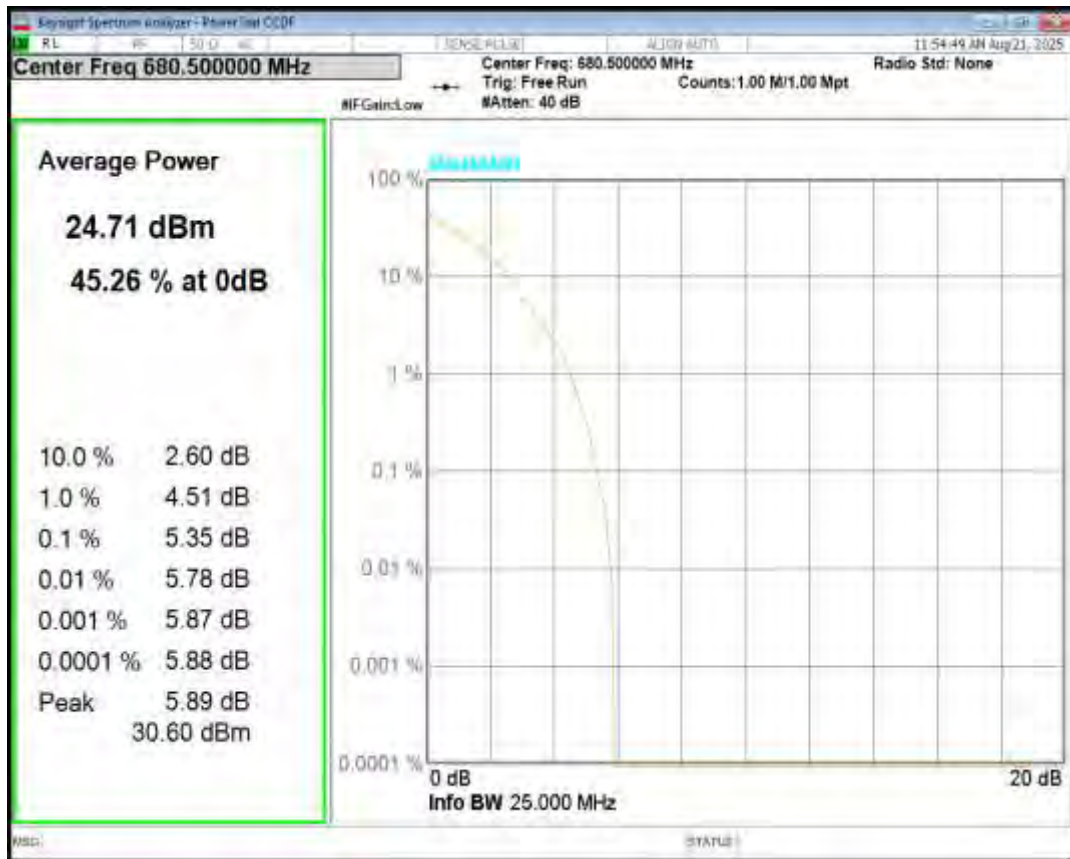
Band71 16QAM BW=20MHz Channel=133297 RB Size=1 Position=#0
