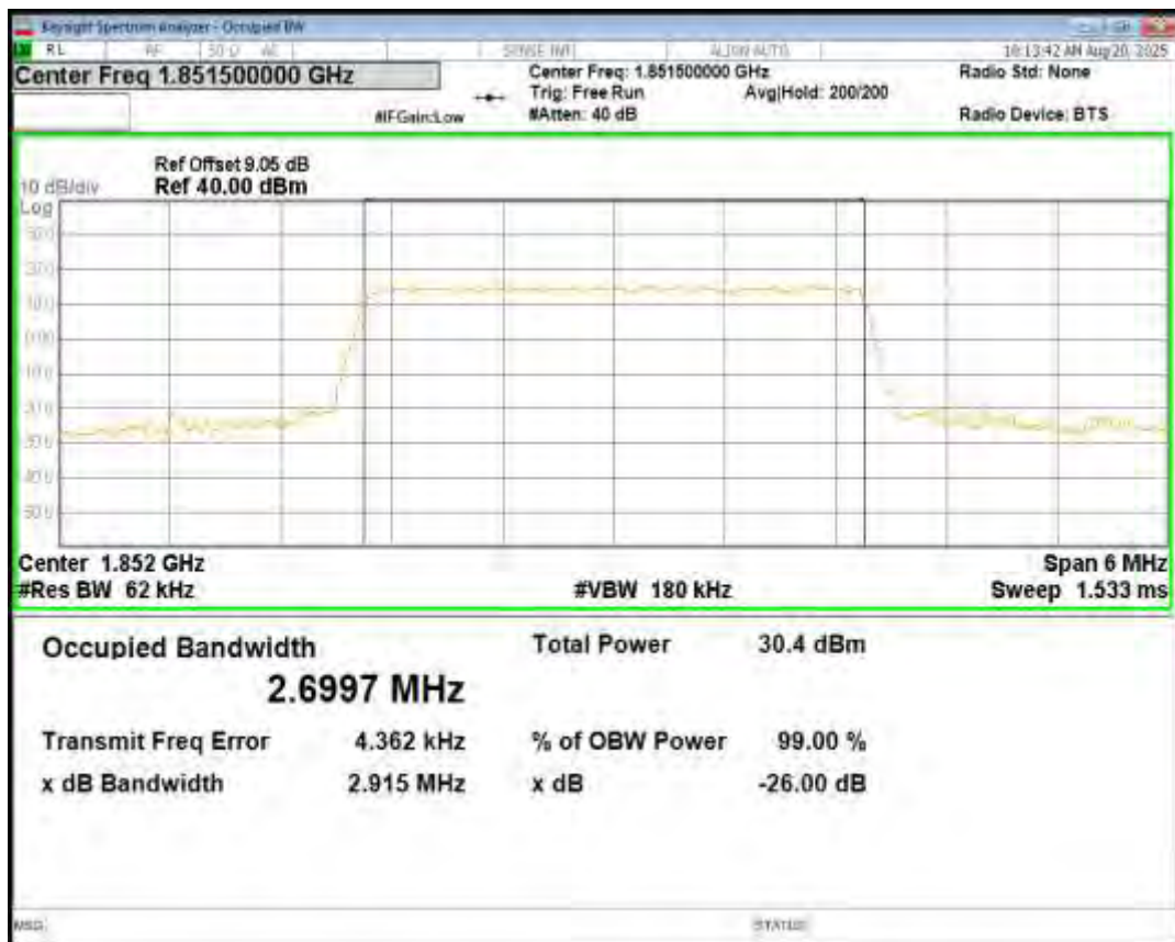
Band2 QPSK BW=3MHz Channel=18900 RB Size=15 Position=#0
