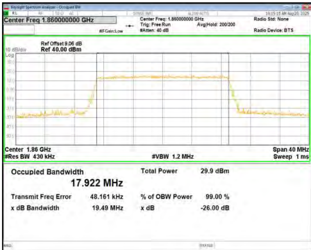
Band2 QPSK BW=20MHz Channel=18900 RB Size=100 Position=#0
