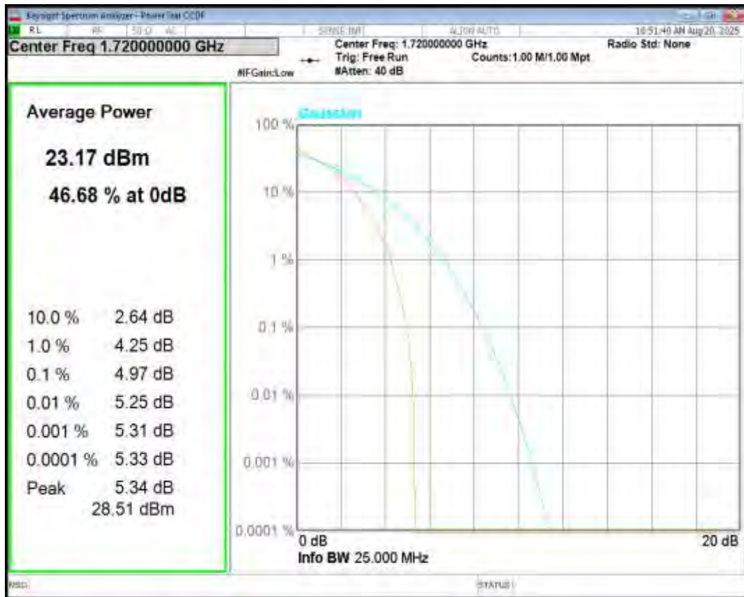
Band4 16QAM BW=20MHz Channel=20050 RB Size=1 Position=#0
