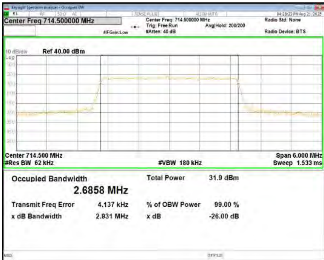
Band12 QPSK BW=5MHz Channel=23035 RB Size=25 Position=#0
