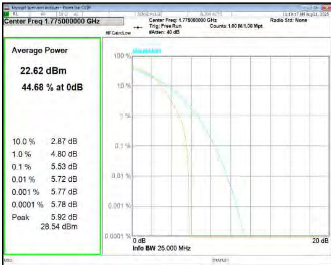
Band66 QPSK BW=15MHz Channel=132047 RB Size=1 Position=#0
