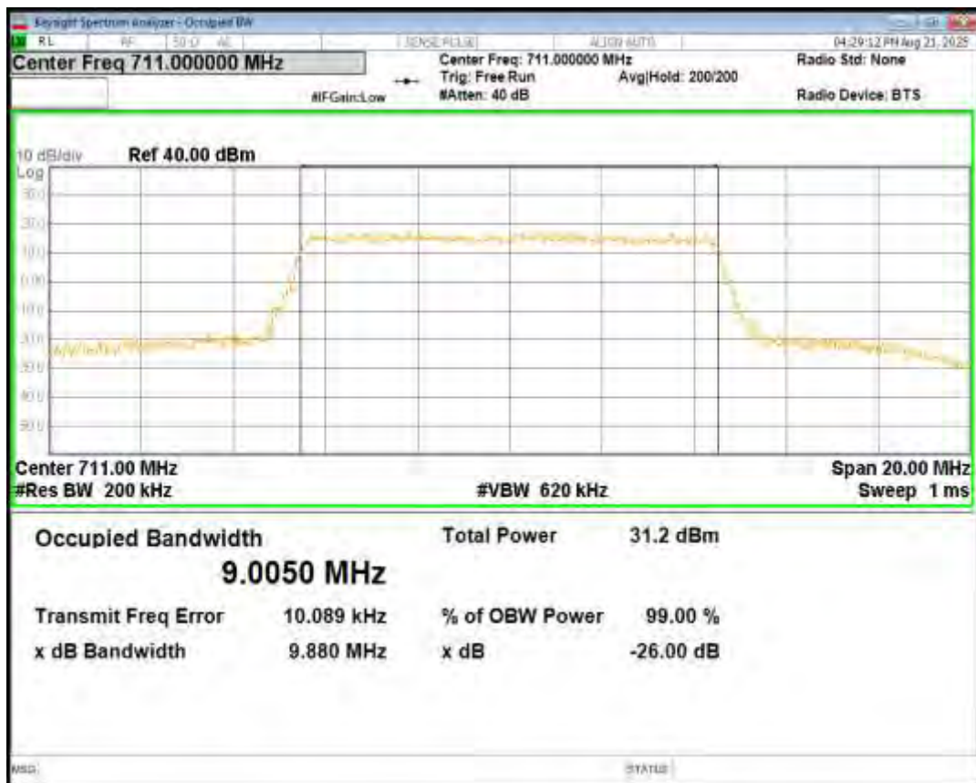
Band17 QPSK BW=5MHz Channel=23755 RB Size=25 Position=#0
