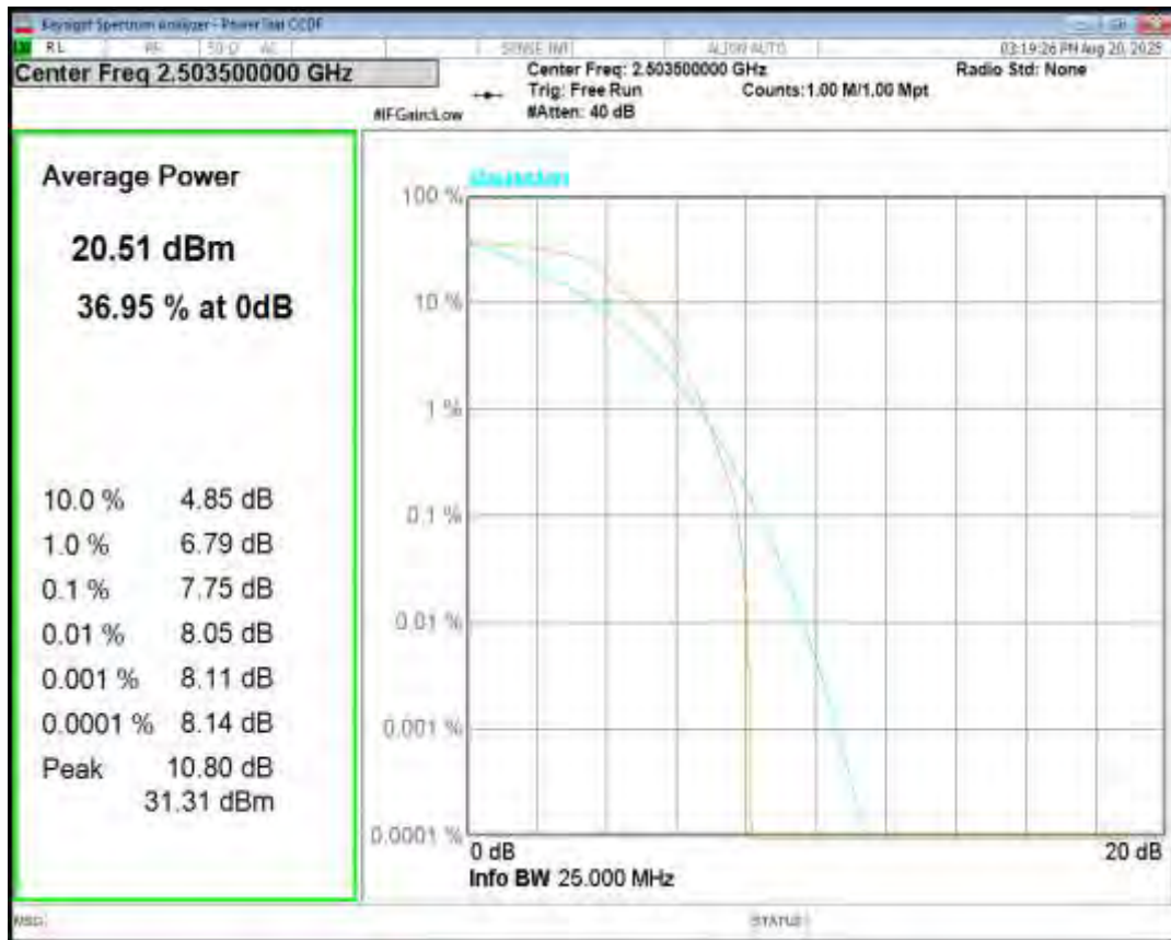
Band41 16QAM BW=15MHz Channel=39725 RB Size=1 Position=#0
