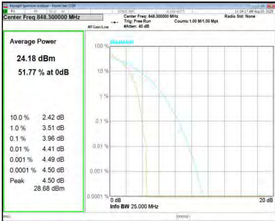
Band5 16QAM BW=1.4MHz Channel=20643 RB Size=1 Position=#0
