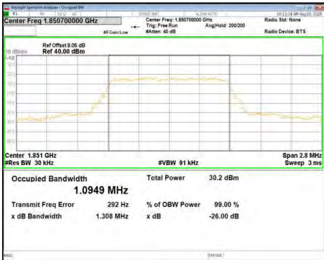
Band2 QPSK BW=1.4MHz Channel=18900 RB Size=6 Position=#0
