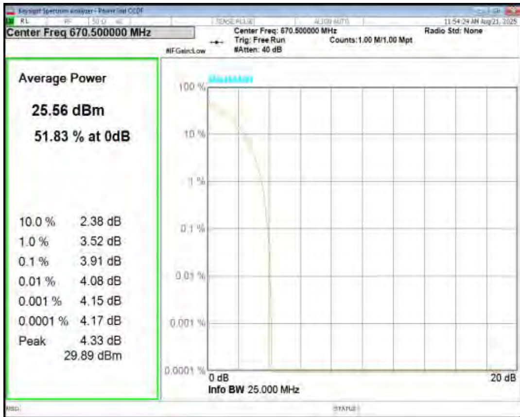
Band71 16QAM BW=15MHz Channel=133197 RB Size=1 Position=#0
