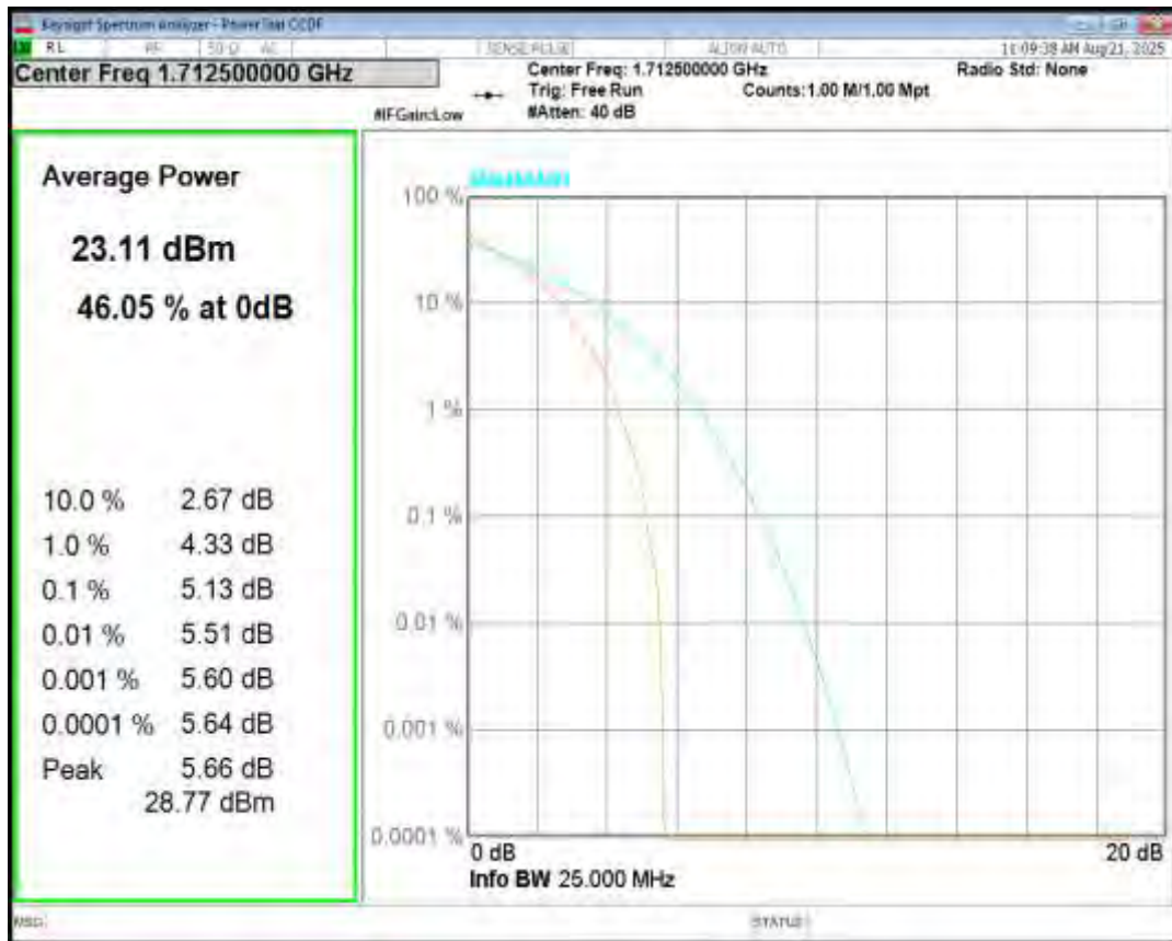
Band66 16QAM BW=5MHz Channel=131997 RB Size=1 Position=#0
