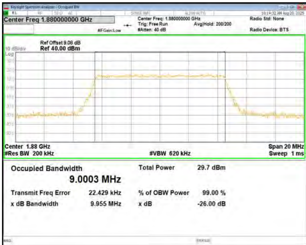
Band2 QPSK BW=10MHz Channel=19150 RB Size=50 Position=#0
