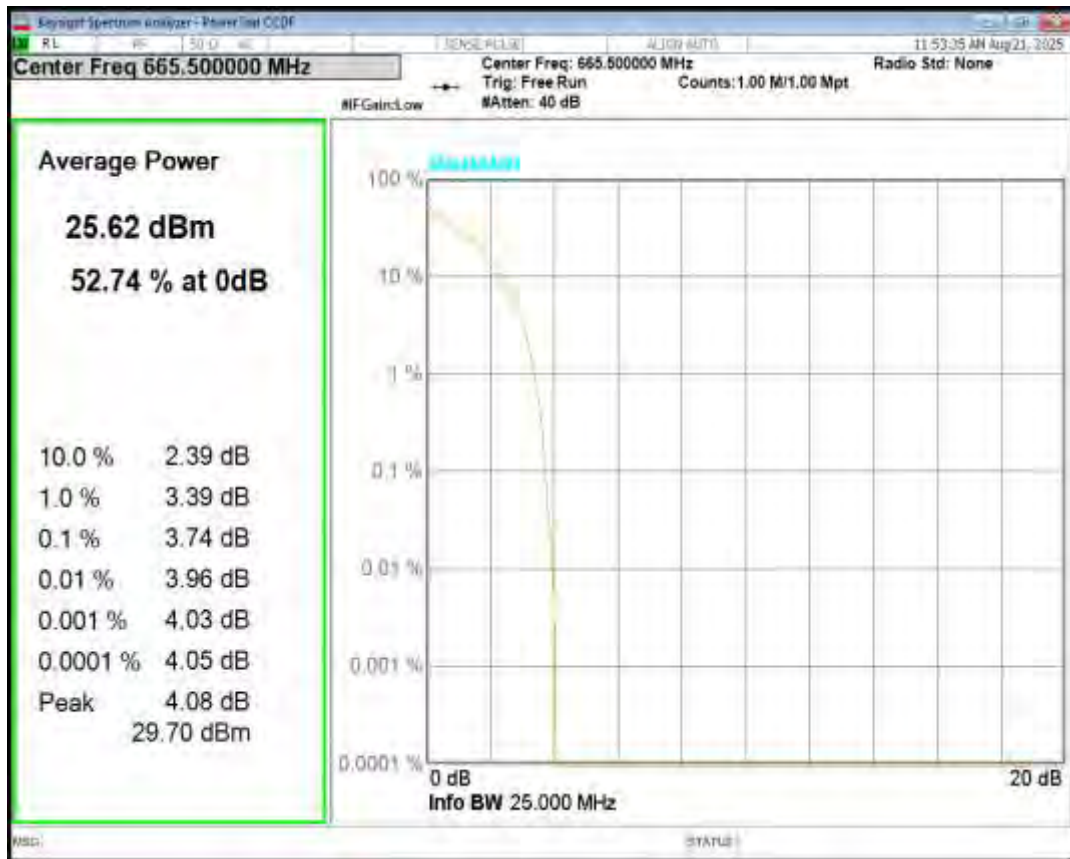
Band71 16QAM BW=5MHz Channel=133147 RB Size=1 Position=#0
