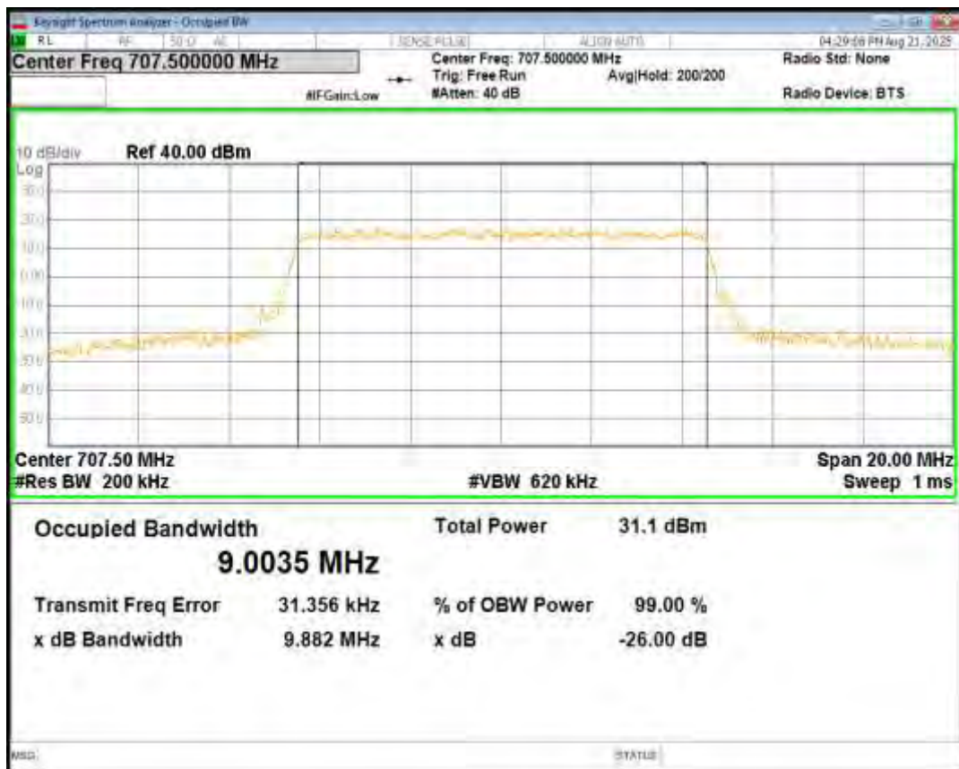
Band12 QPSK BW=10MHz Channel=23130 RB Size=50 Position=#0
