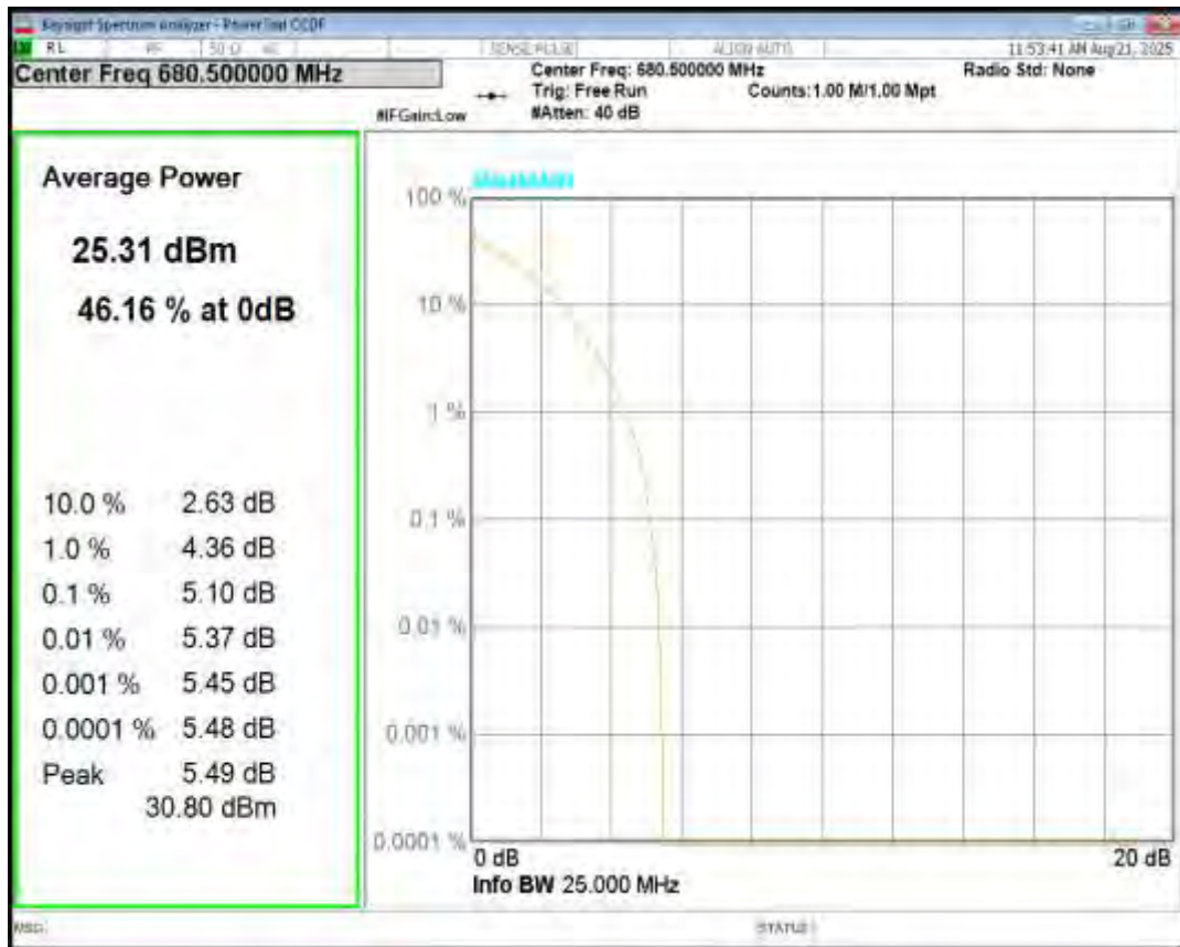
Band71 16QAM BW=5MHz Channel=133297 RB Size=1 Position=#0
