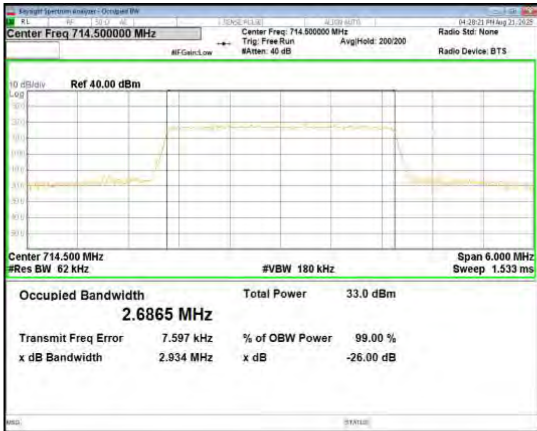
Band12 16QAM BW=3MHz Channel=23165 RB Size=15 Position=#0
