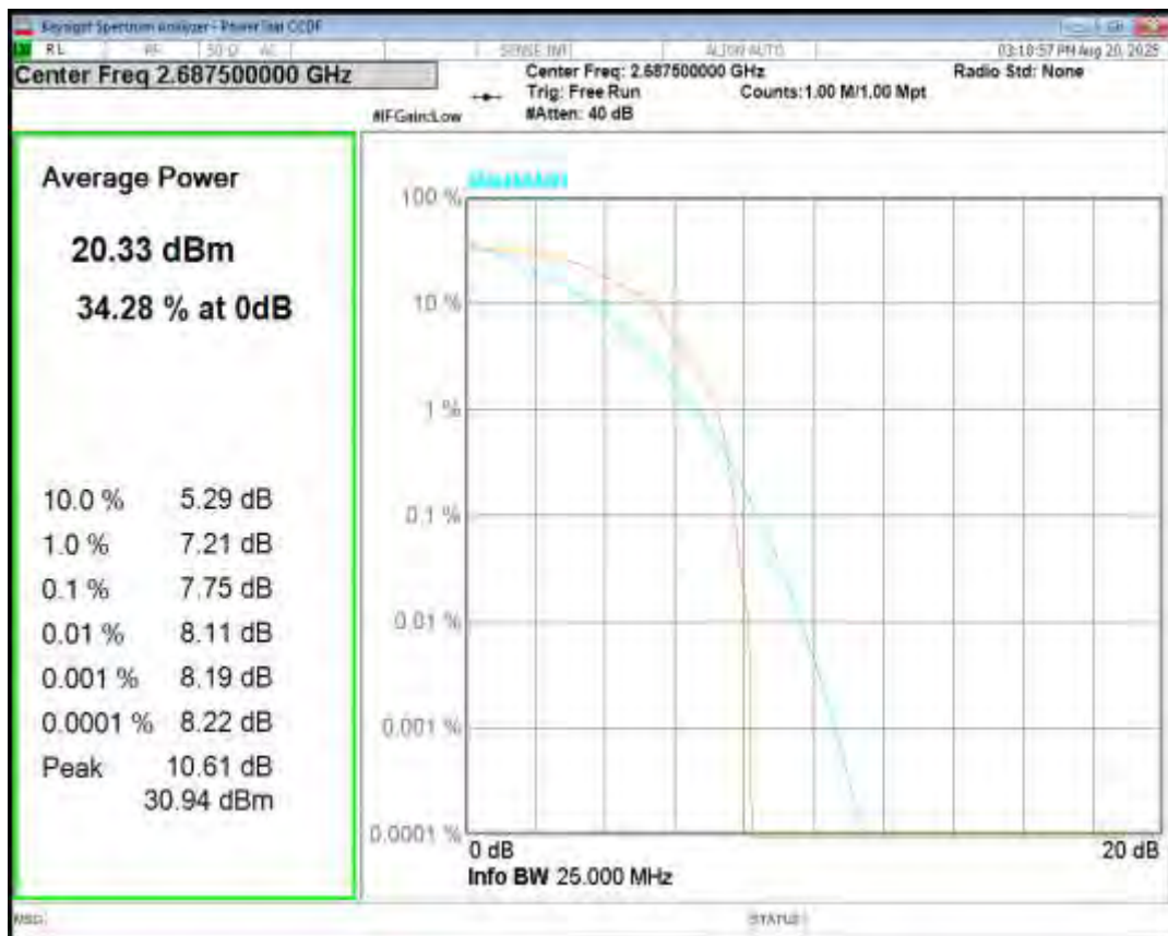
Band41 QPSK BW=10MHz Channel=39700 RB Size=1 Position=#0
