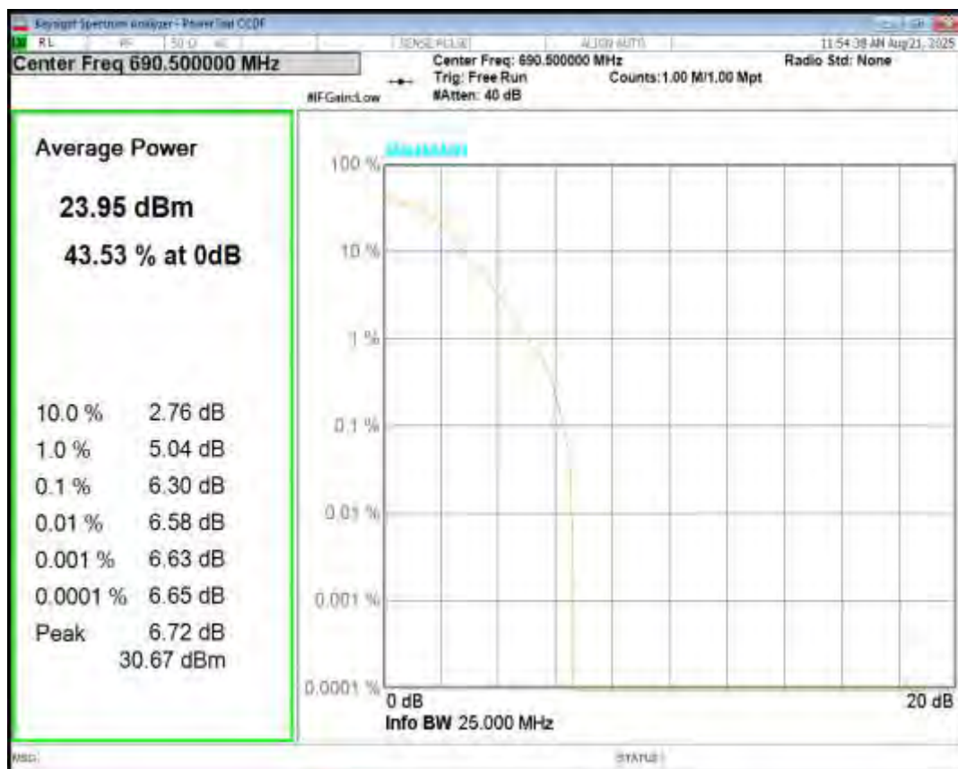
Band71 QPSK BW=20MHz Channel=133222 RB Size=1 Position=#0
