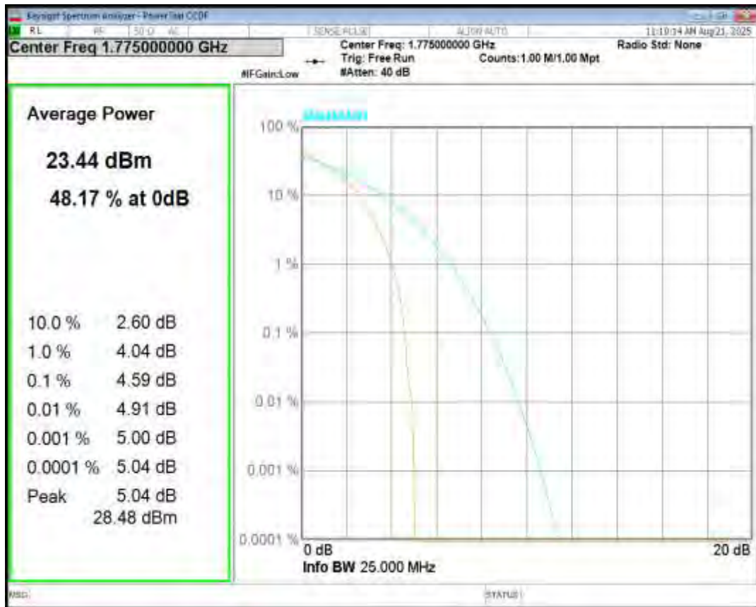
Band66 16QAM BW=10MHz Channel=132622 RB Size=1 Position=#0
