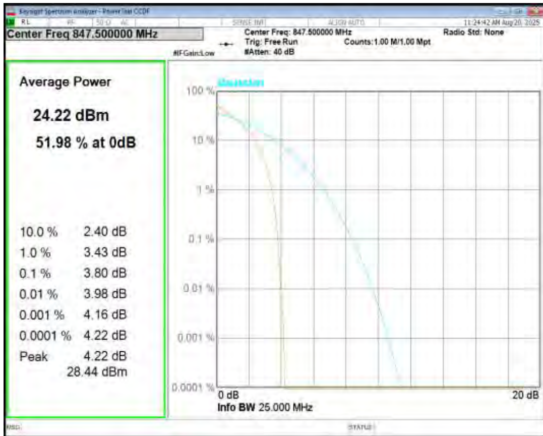
Band5 16QAM BW=3MHz Channel=20635 RB Size=1 Position=#0
