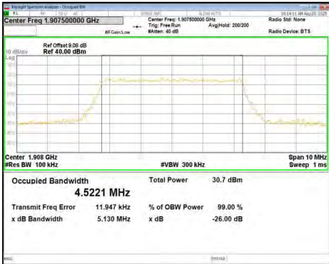
Band2 16QAM BW=5MHz Channel=19175 RB Size=25 Position=#0
