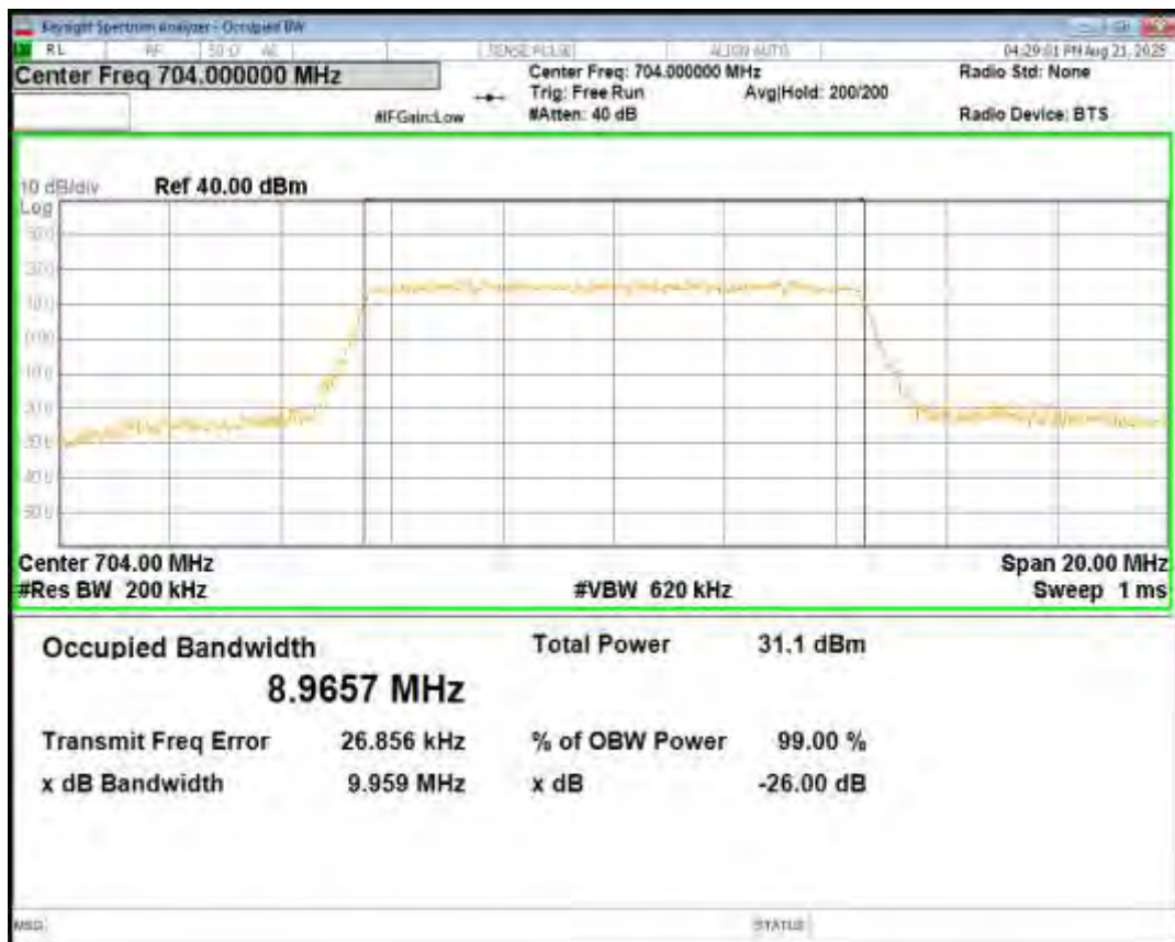
Band12 QPSK BW=10MHz Channel=23095 RB Size=50 Position=#0
