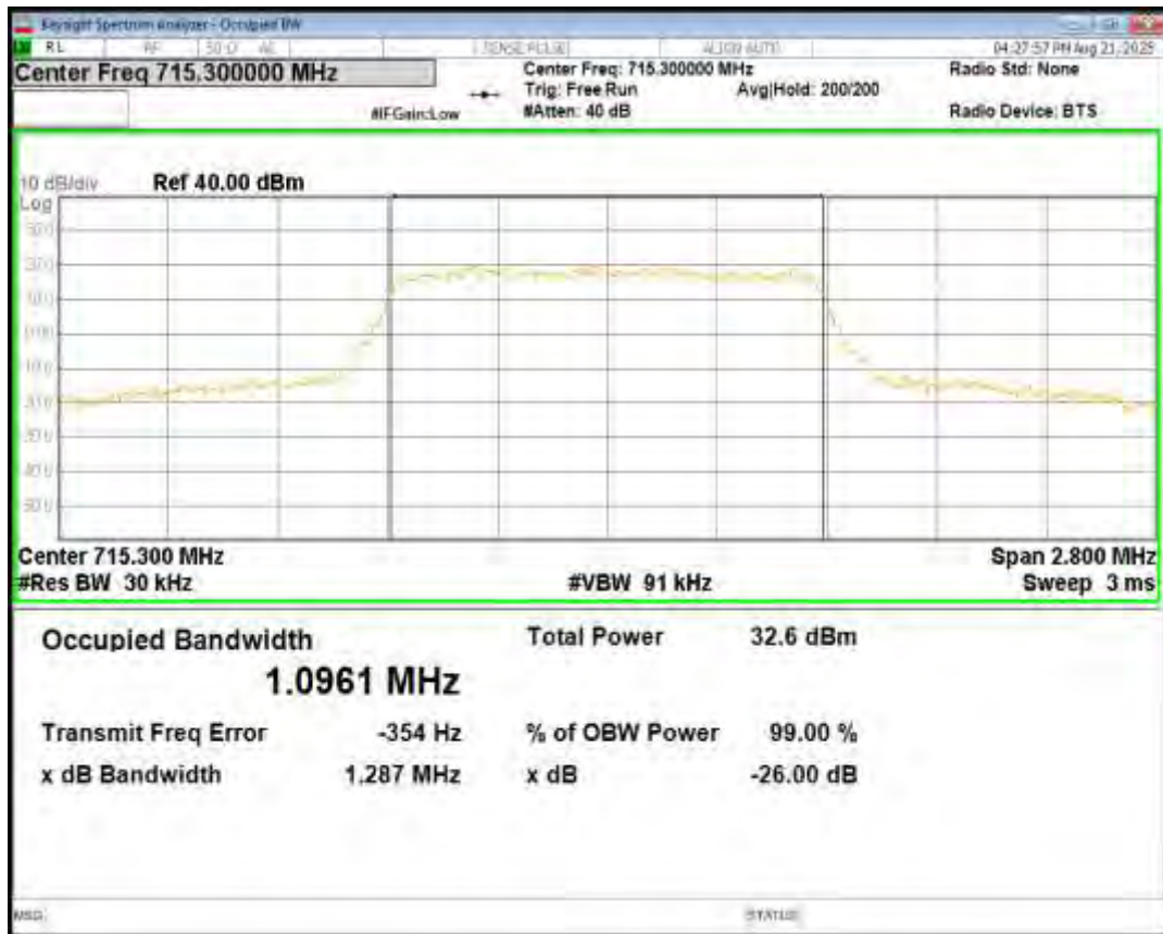
Band12 16QAM BW=1.4MHz Channel=23173 RB Size=6 Position=#0
