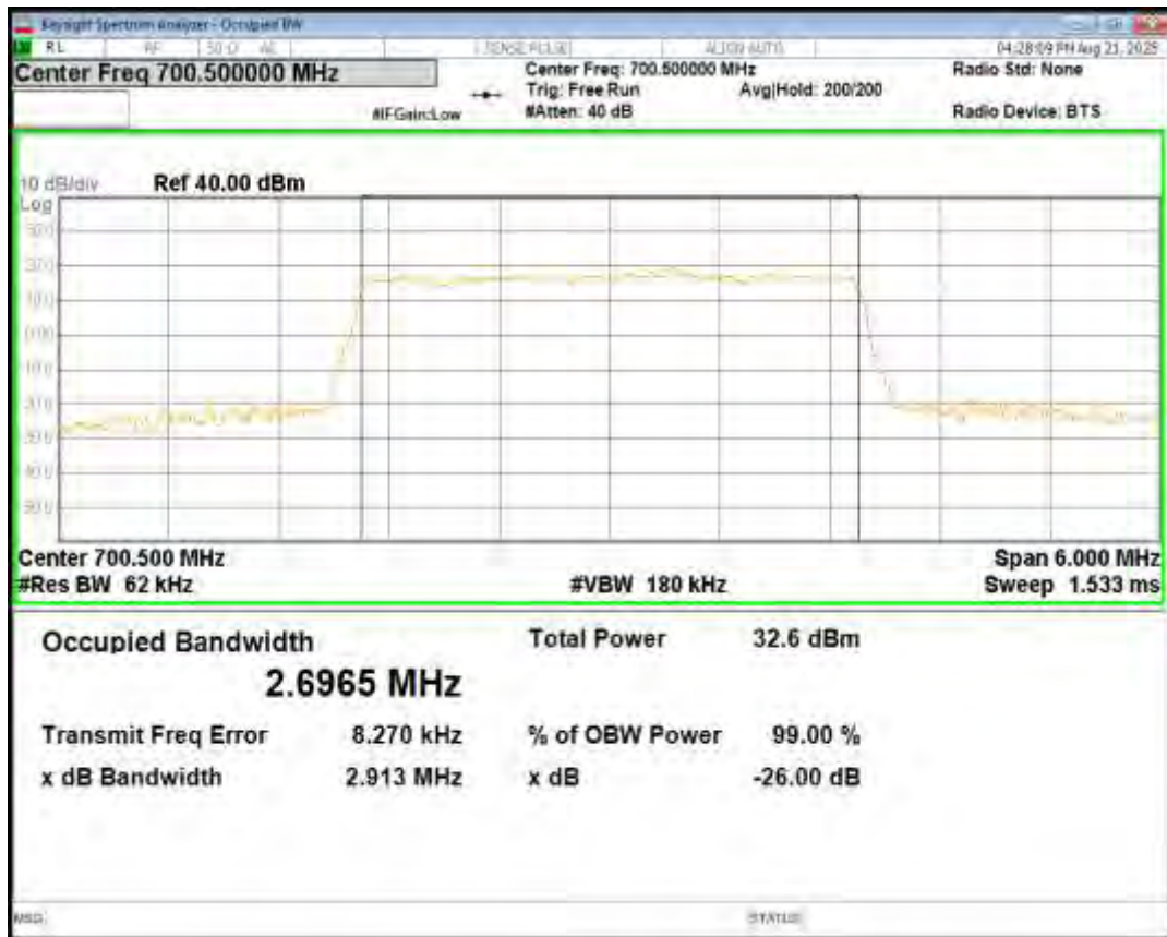
Band12 16QAM BW=3MHz Channel=23025 RB Size=15 Position=#0
