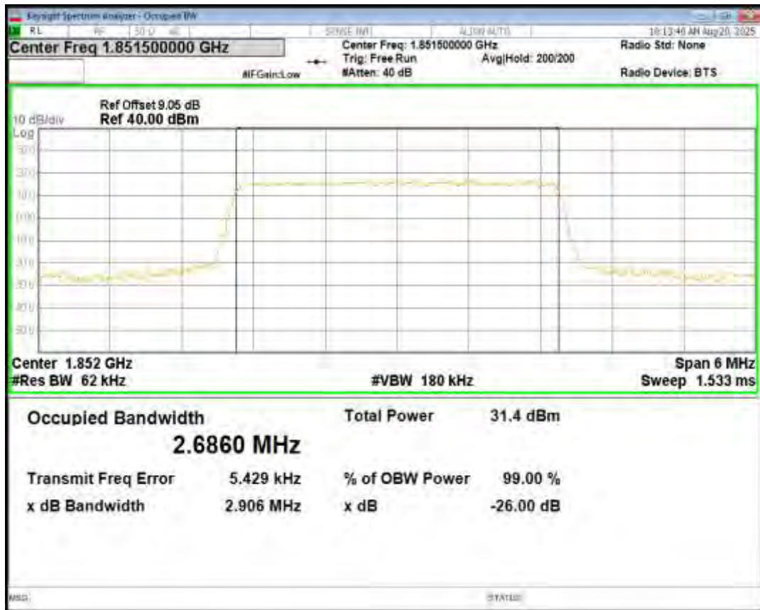
Band2 16QAM BW=3MHz Channel=18615 RB Size=15 Position=#0
