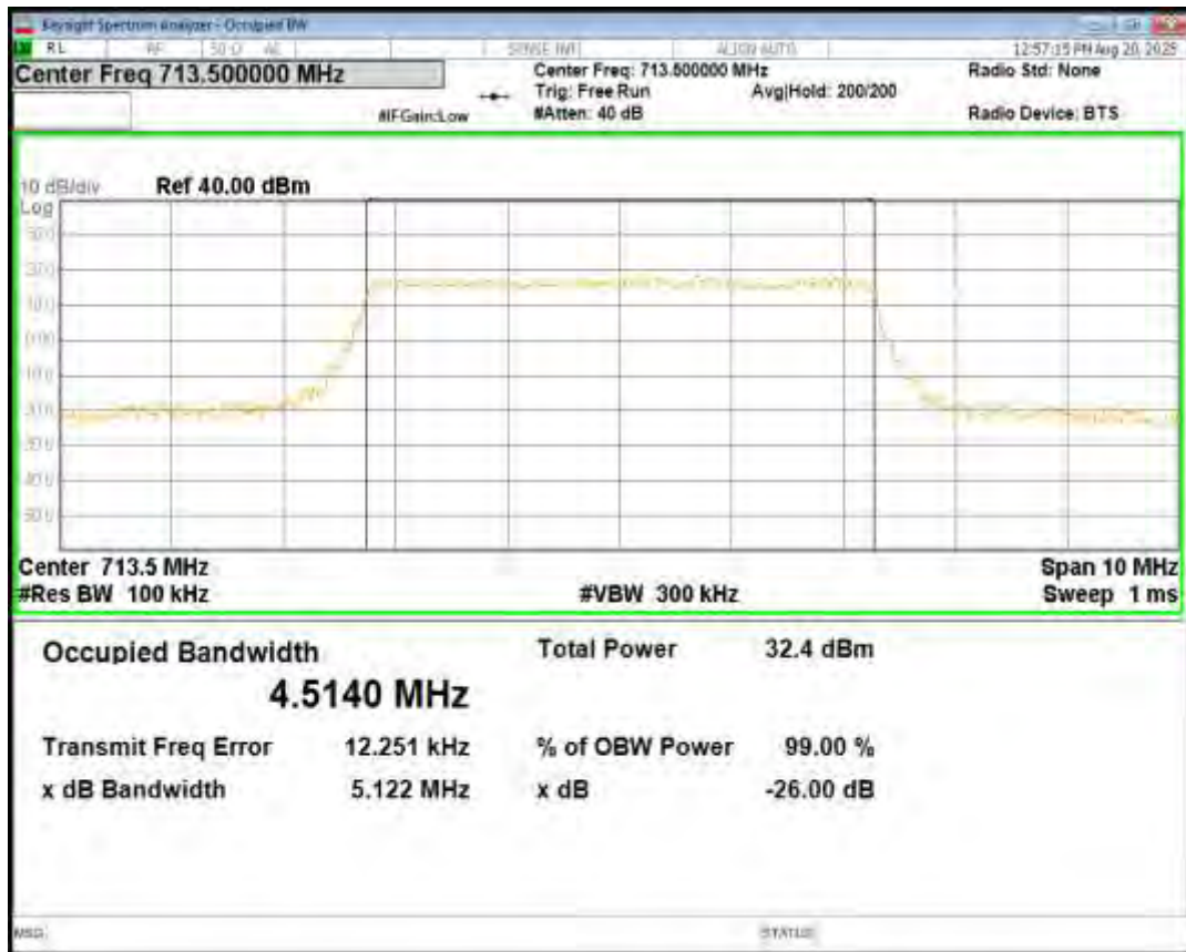
Band17 16QAM BW=5MHz Channel=23825 RB Size=25 Position=#0
