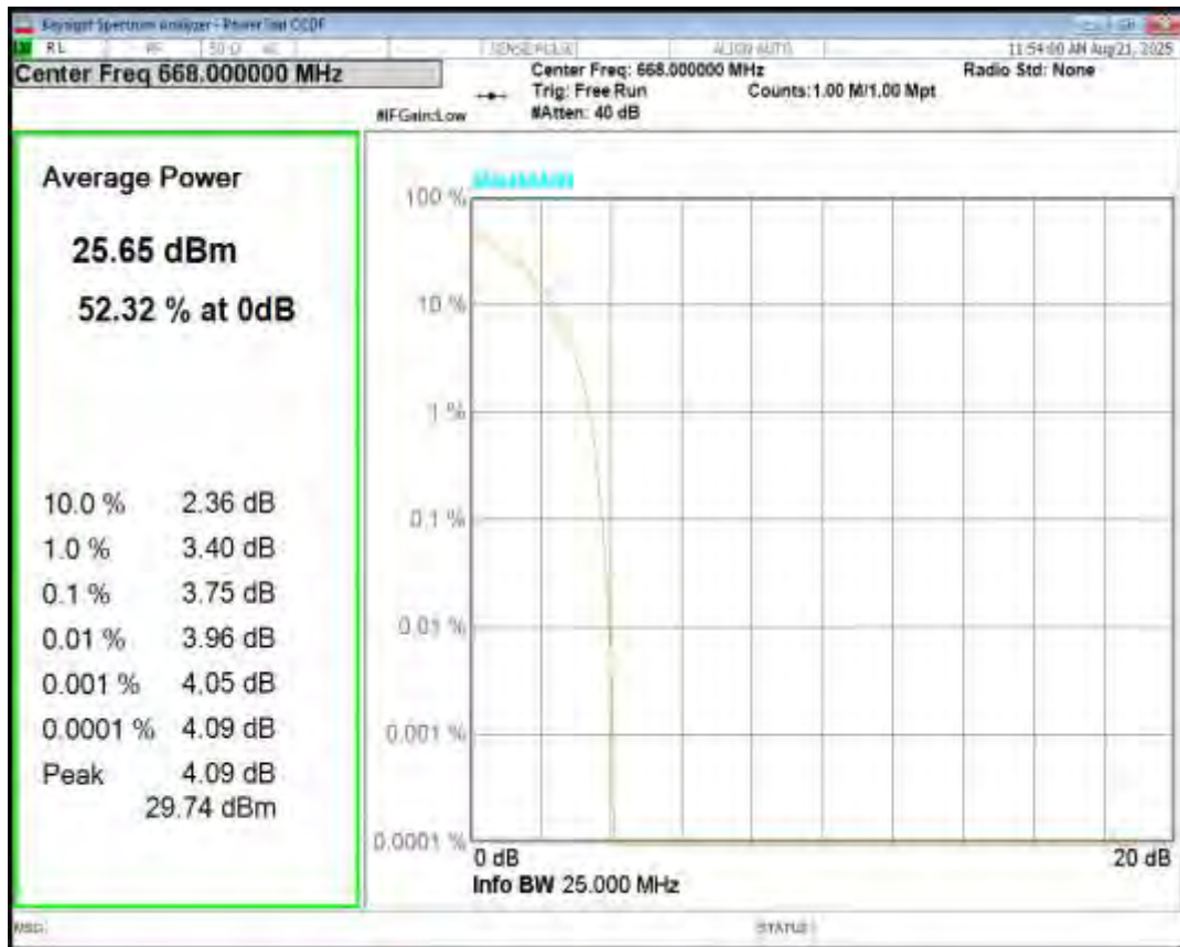
Band71 16QAM BW=10MHz Channel=133172 RB Size=1 Position=#0
