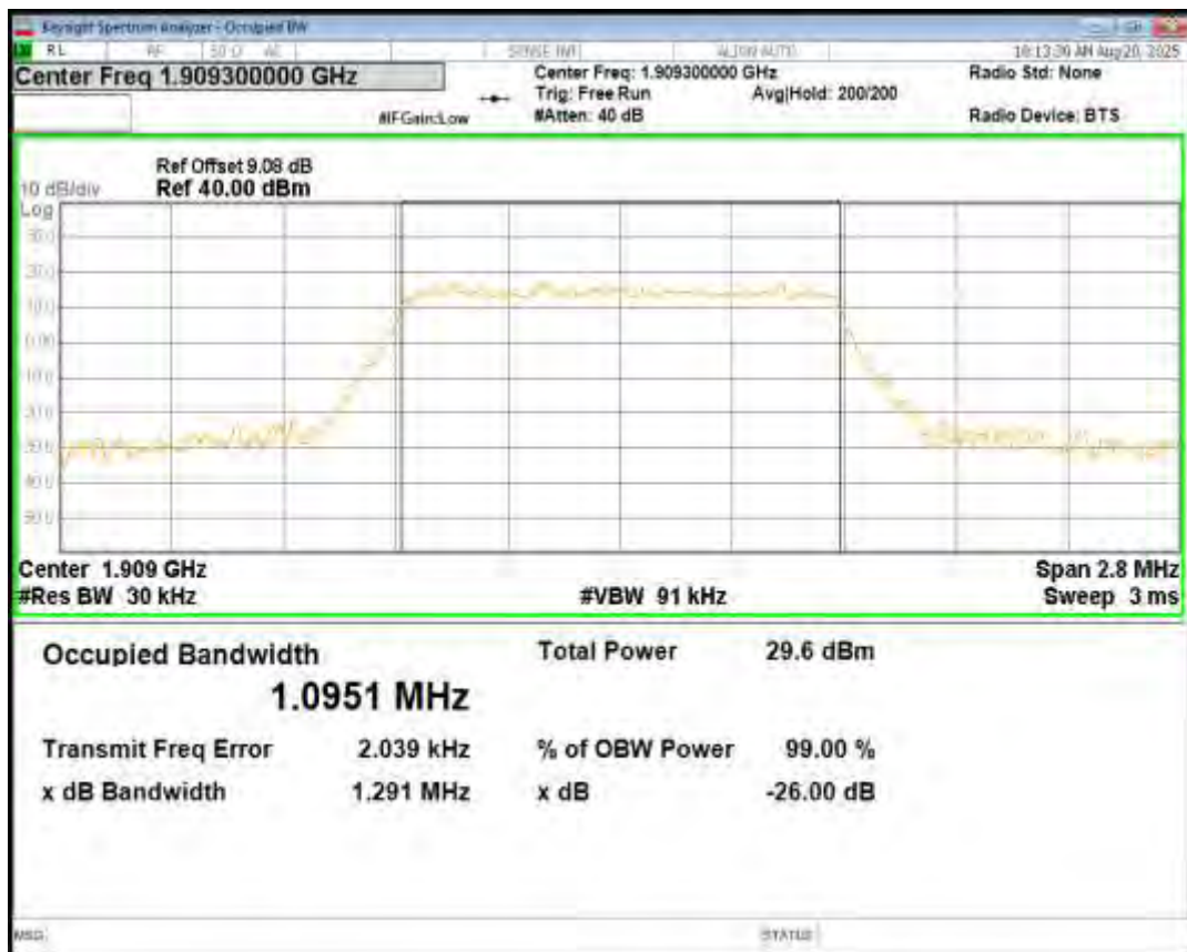
Band2 QPSK BW=3MHz Channel=18615 RB Size=15 Position=#0
