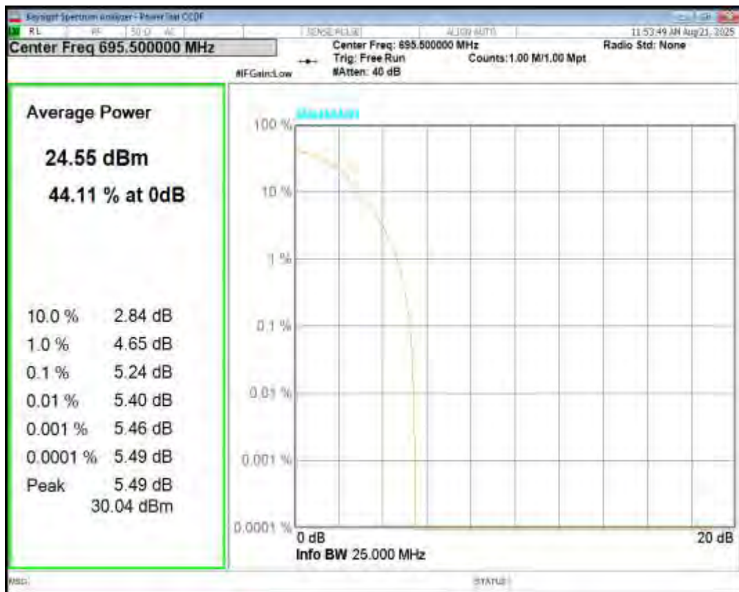
Band71 QPSK BW=10MHz Channel=133172 RB Size=1 Position=#0
