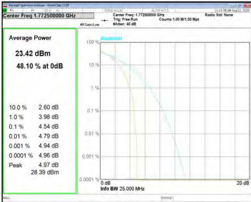
Band66 16QAM BW=15MHz Channel=132597 RB Size=1 Position=#0
