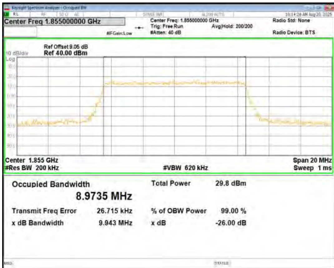
Band2 QPSK BW=10MHz Channel=18900 RB Size=50 Position=#0
