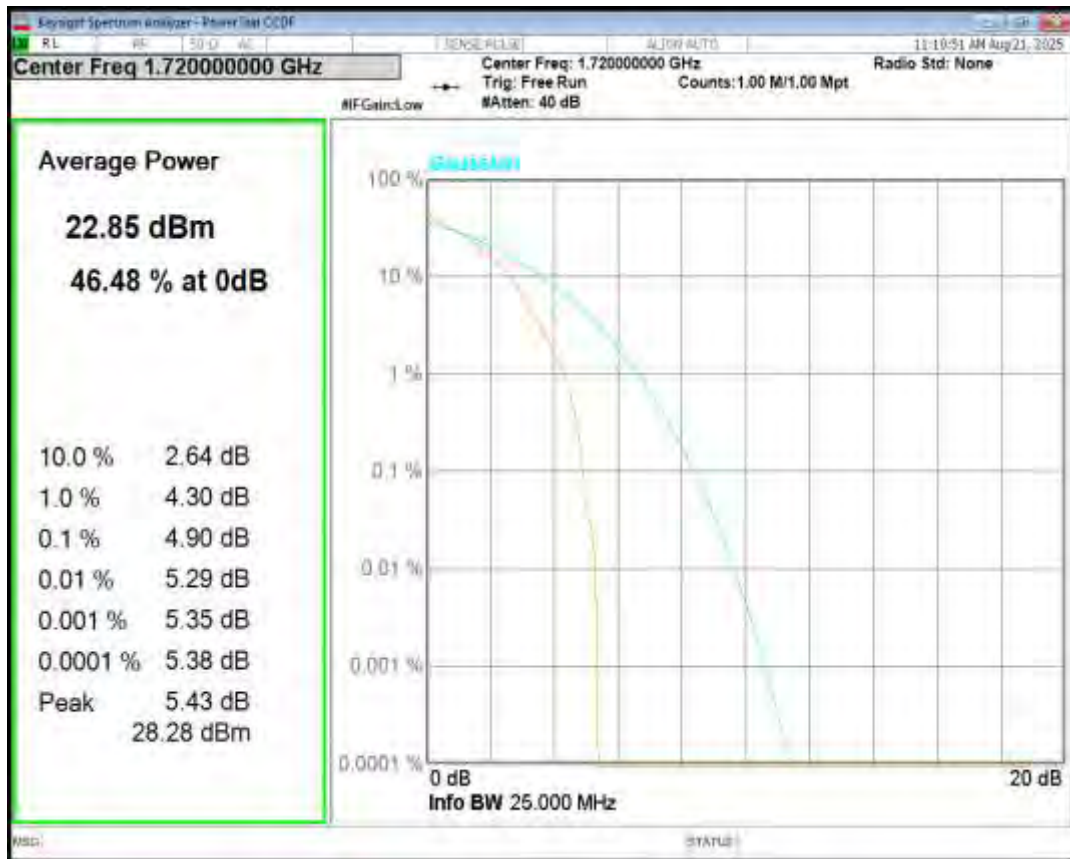
Band66 16QAM BW=20MHz Channel=132072 RB Size=1 Position=#0
