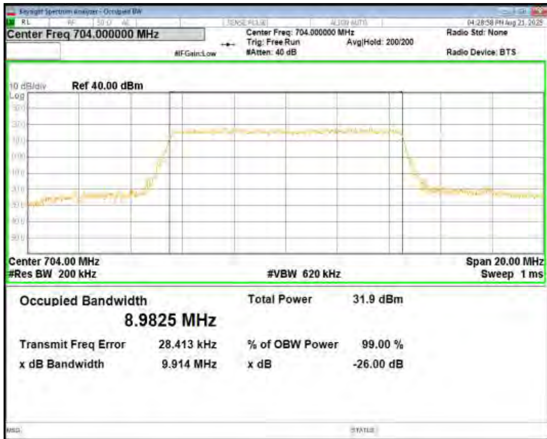
Band12 16QAM BW=10MHz Channel=23060 RB Size=50 Position=#0
