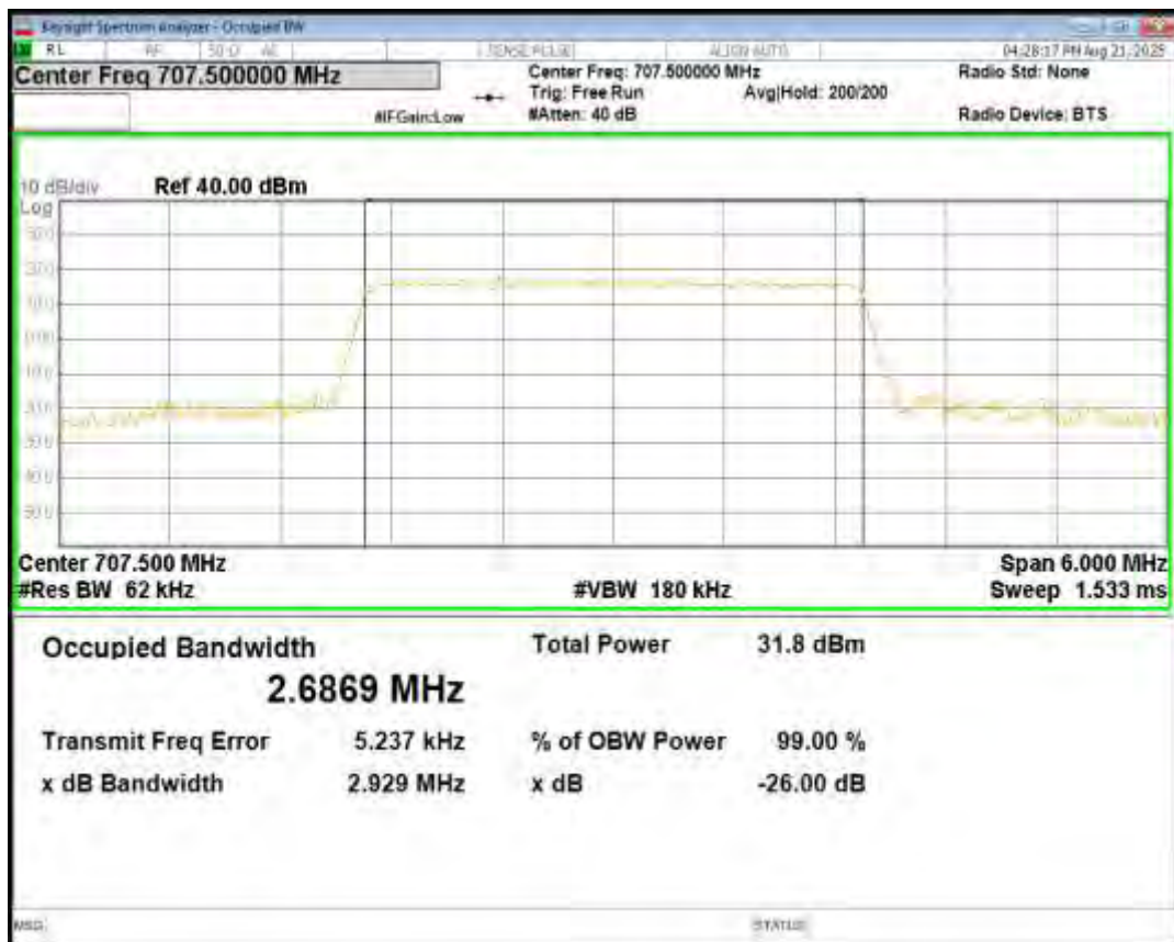
Band12 QPSK BW=3MHz Channel=23165 RB Size=15 Position=#0
