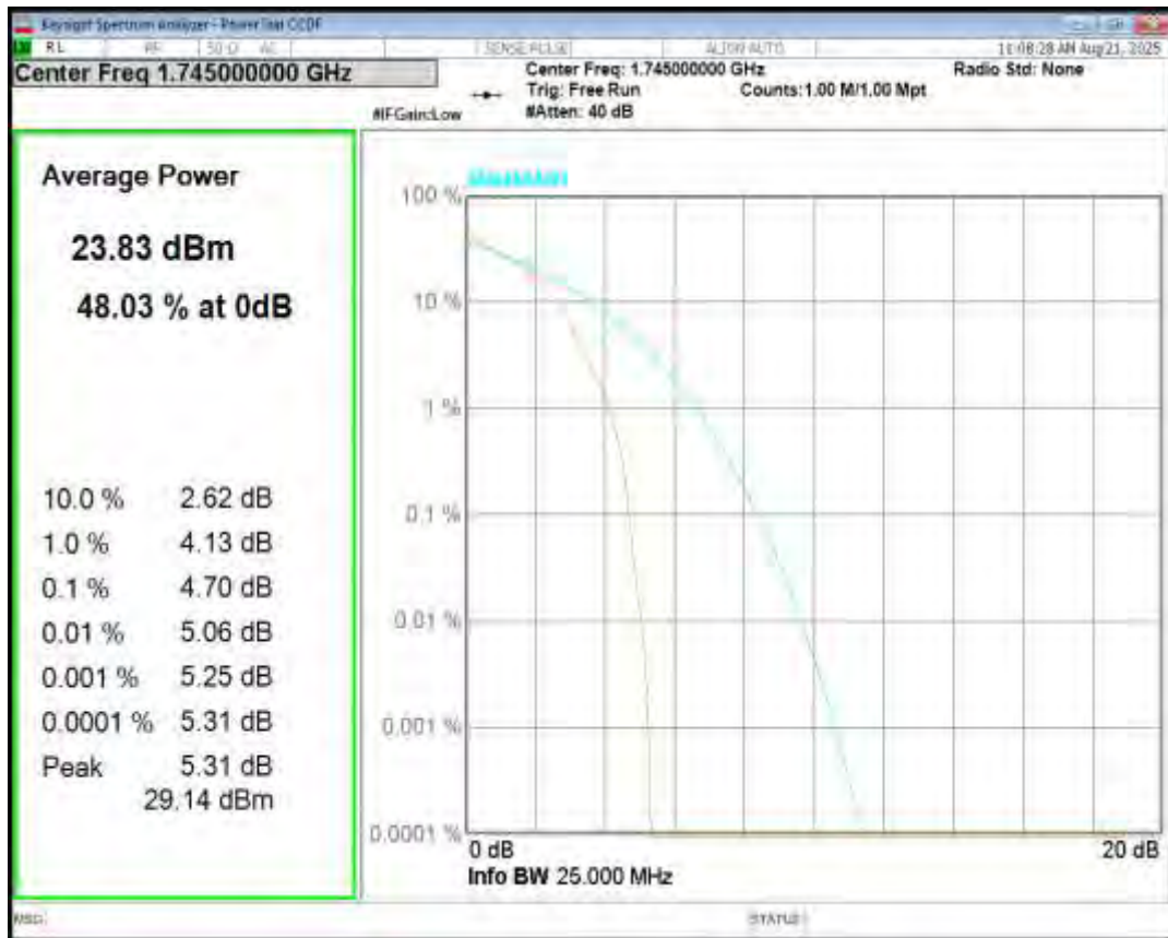
Band66 16QAM BW=3MHz Channel=132322 RB Size=1 Position=#0
