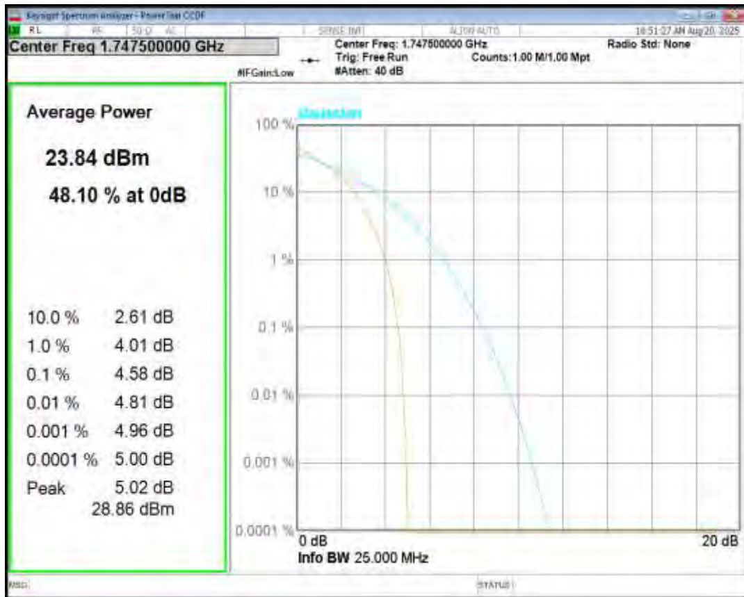
Band4 16QAM BW=15MHz Channel=20325 RB Size=1 Position=#0
