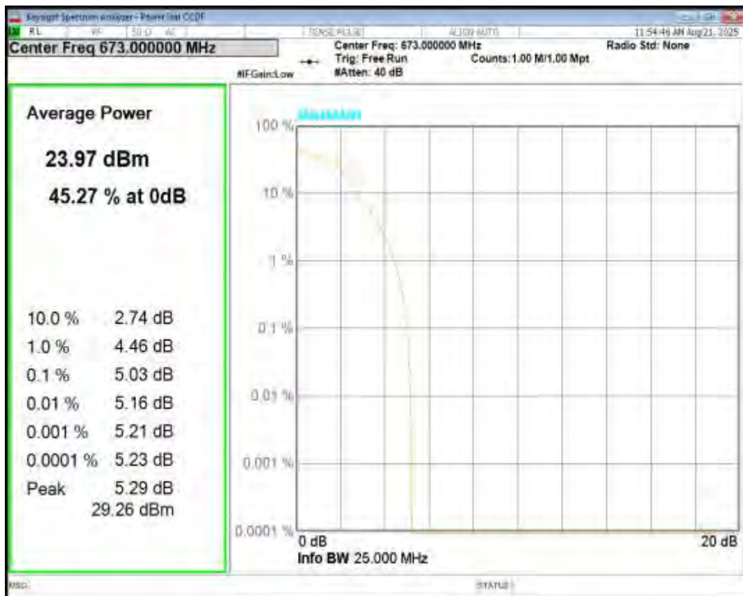
Band71 QPSK BW=20MHz Channel=133297 RB Size=1 Position=#0
