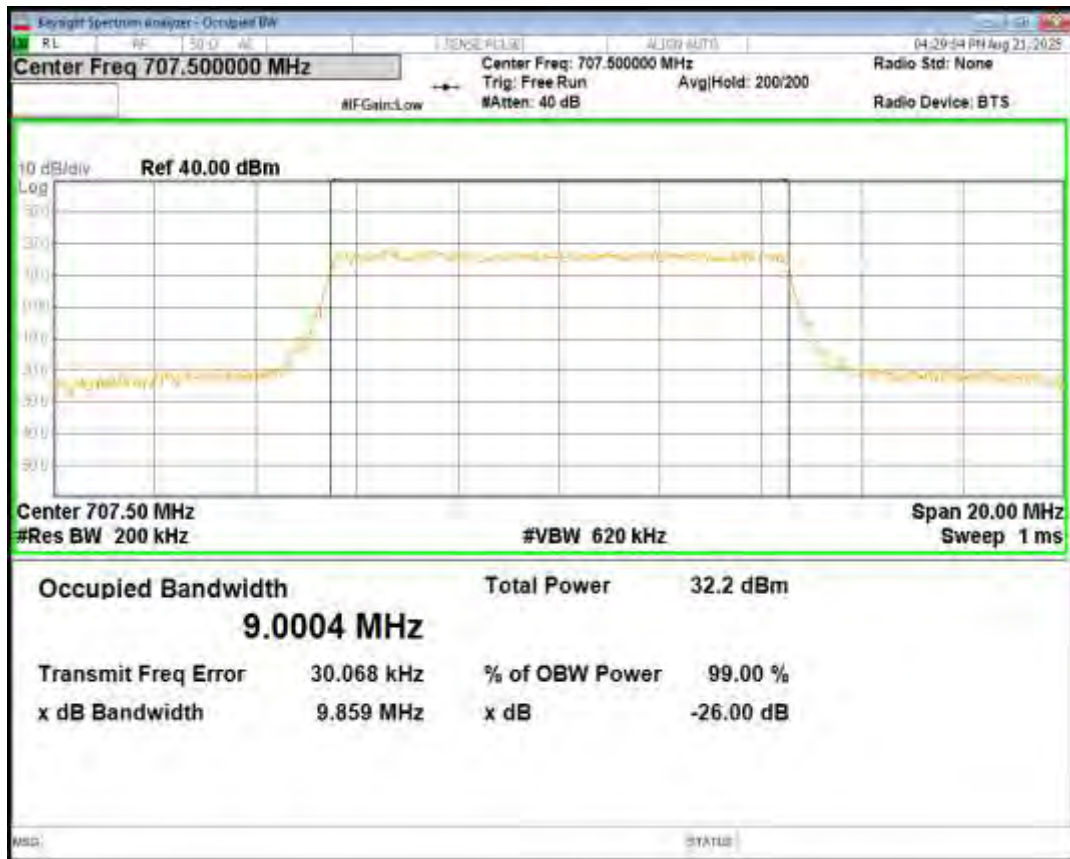
Band12 16QAM BW=10MHz Channel=23095 RB Size=50 Position=#0
