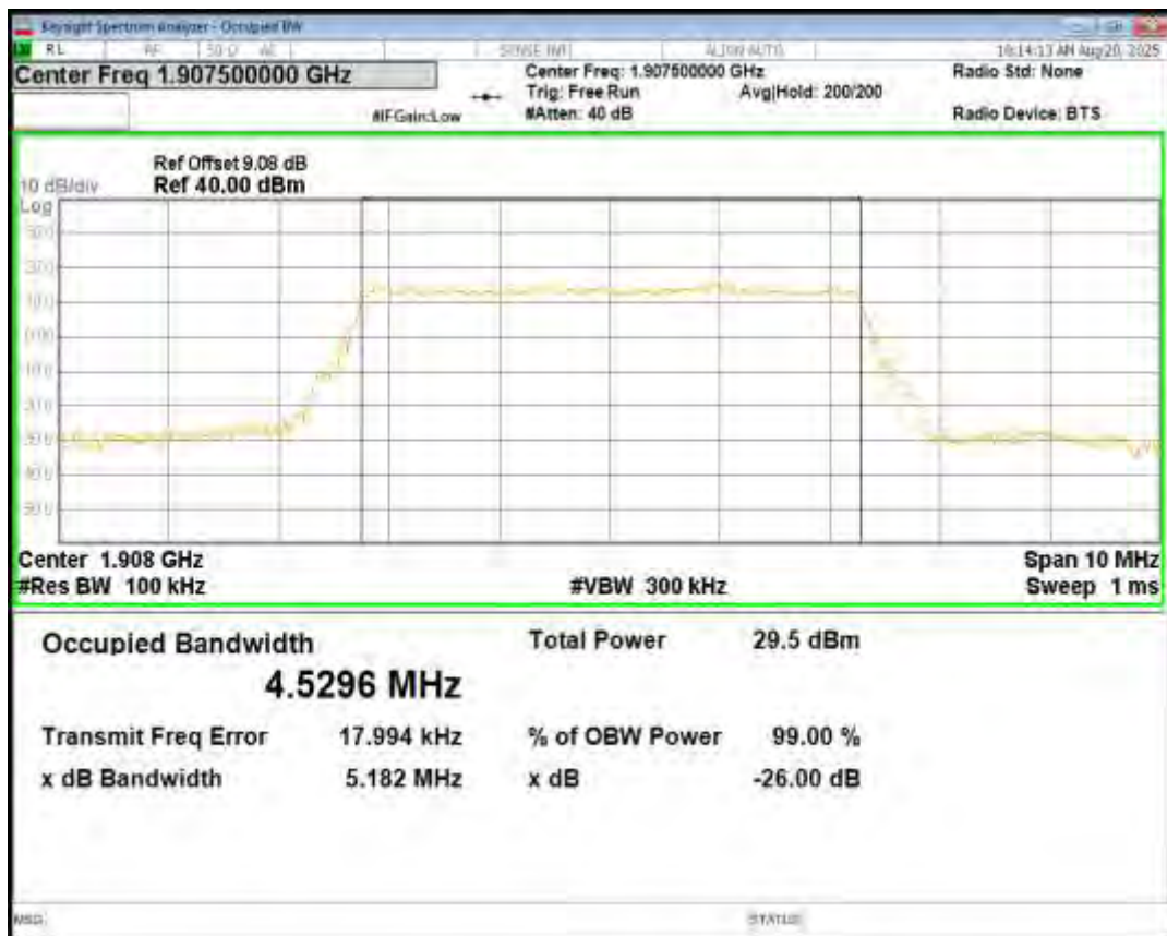
Band2 QPSK BW=10MHz Channel=18650 RB Size=50 Position=#0
