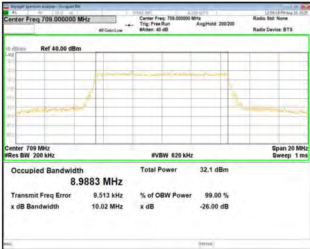
Band17 16QAM BW=10MHz Channel=23780 RB Size=50 Position=#0
