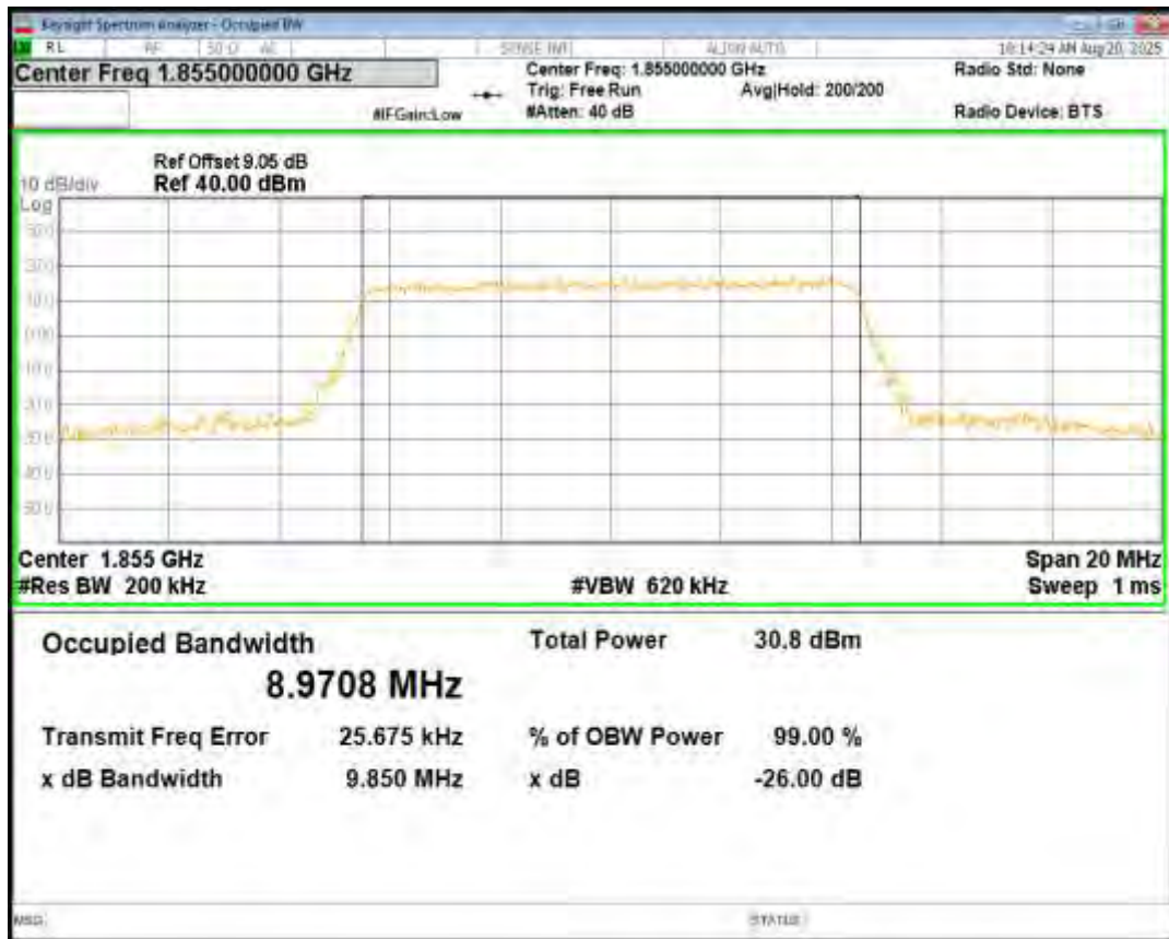
Band2 16QAM BW=10MHz Channel=18650 RB Size=50 Position=#0
