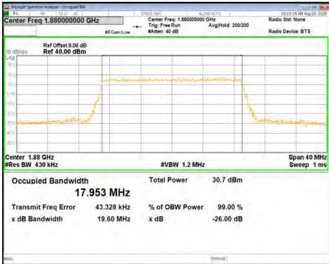
Band2 16QAM BW=20MHz Channel=18900 RB Size=100 Position=#0
