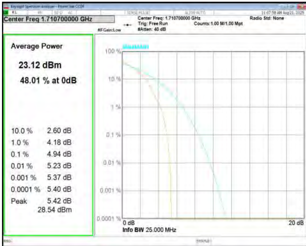
Band66 16QAM BW=1.4MHz Channel=131979 RB Size=1 Position=#0
