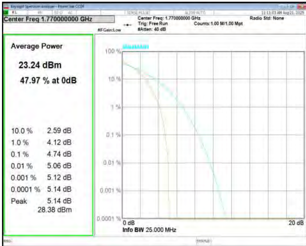
Band66 16QAM BW=20MHz Channel=132572 RB Size=1 Position=#0
