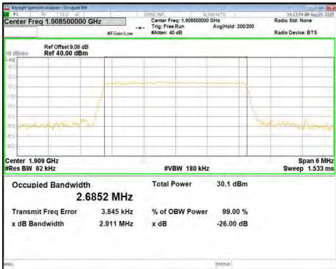
Band2 QPSK BW=5MHz Channel=18625 RB Size=25 Position=#0
