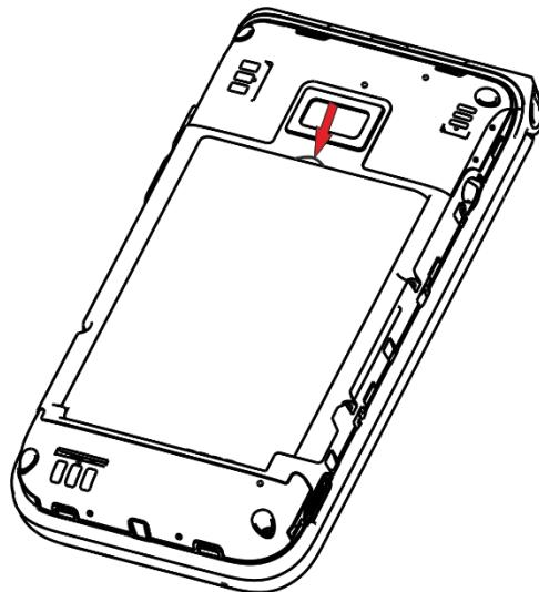
Step 3. To insert SIM card or microSD card, push the SIM card or microSD card into the card slot with the gold-colored contacts facing down.
