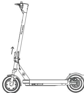
2.Rotate the folder counterclockwise while lifting the folder key.
