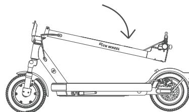
4.Open the folding clip and hang it on the rear fender buckle.
