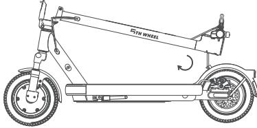
2.Pull up the body lever while opening the folding clip.
