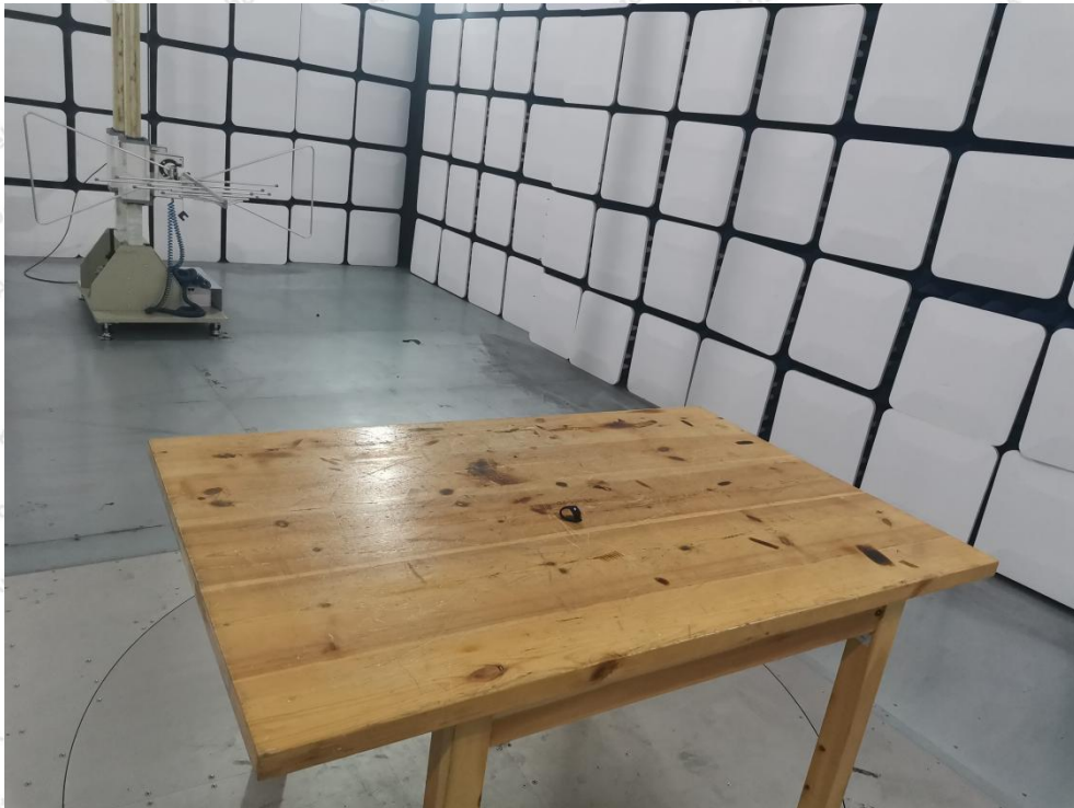
Photo of Radiation Emission Test
