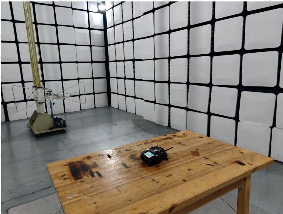
Photo of Radiation Emission Test
