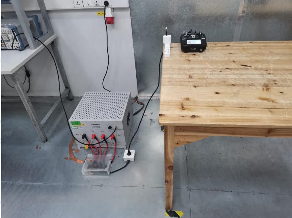
Photo of Conducted Emission Measurement
