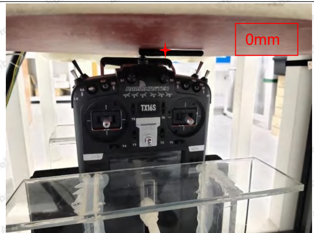
Top(0mm) Antenna bends 90 degrees
