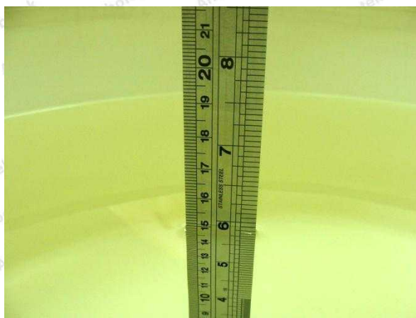
Photo of Liquid Height for Body SAR
