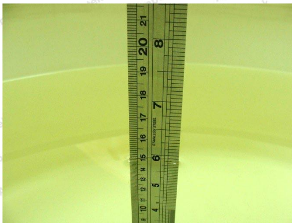
Photo of Liquid Height for Body SAR
