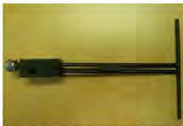
Figure 1 – MVG COMOSAR Validation Dipole
