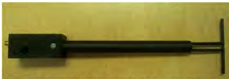
Figure 1 – MVG COMOSAR Validation Dipole
