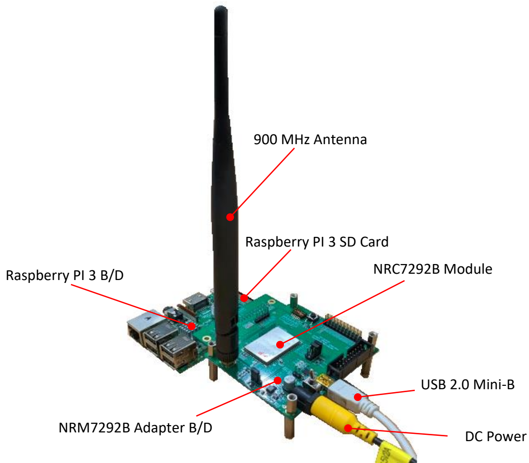
Figure 4.1 Antenna Connection on EVK
