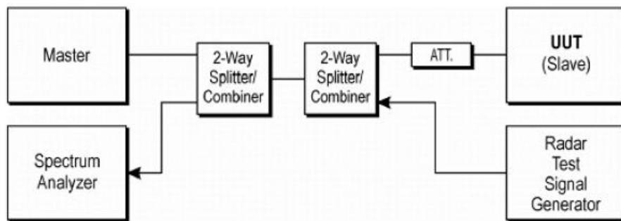
Figure 3-1. Conducted Test Setup for DFS
