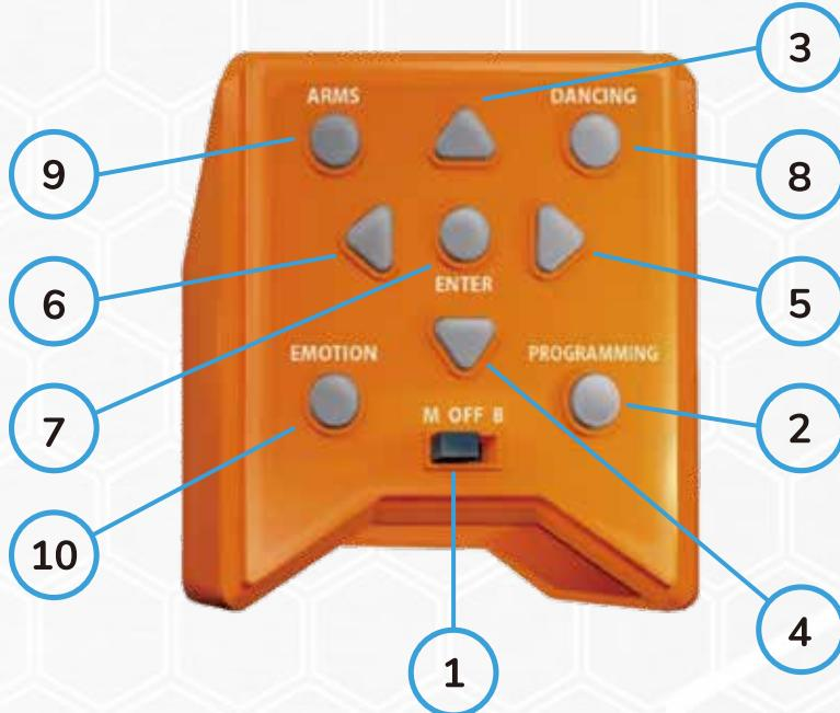
The MANUAL PROGRAMMING uses the unit control at the robot's back. It is not required the use of Smartphone or Tablet.
