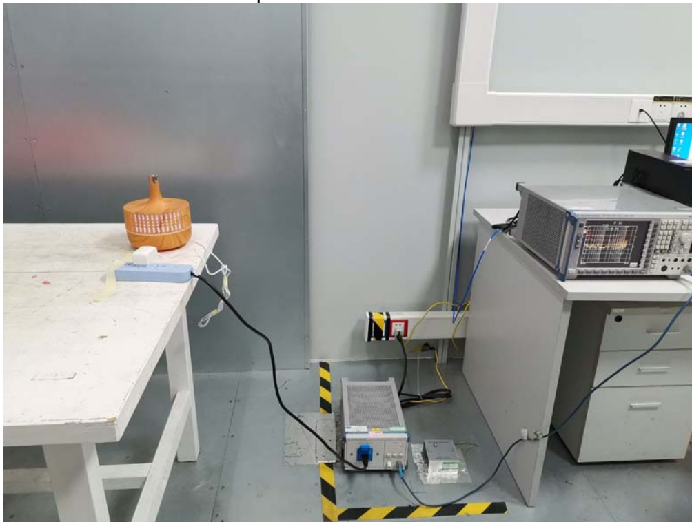
Photos of radiated emission test 30MHz – 1GHz
