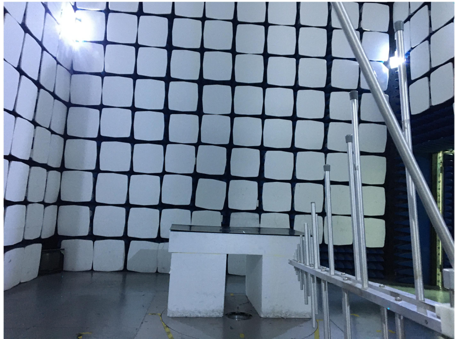
Radiation Emission Test Setup (30MHz to 1GHz)
