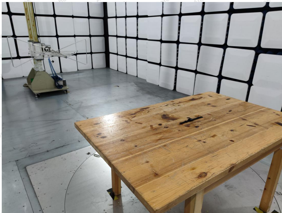
Photo of Radiation Emission Test
