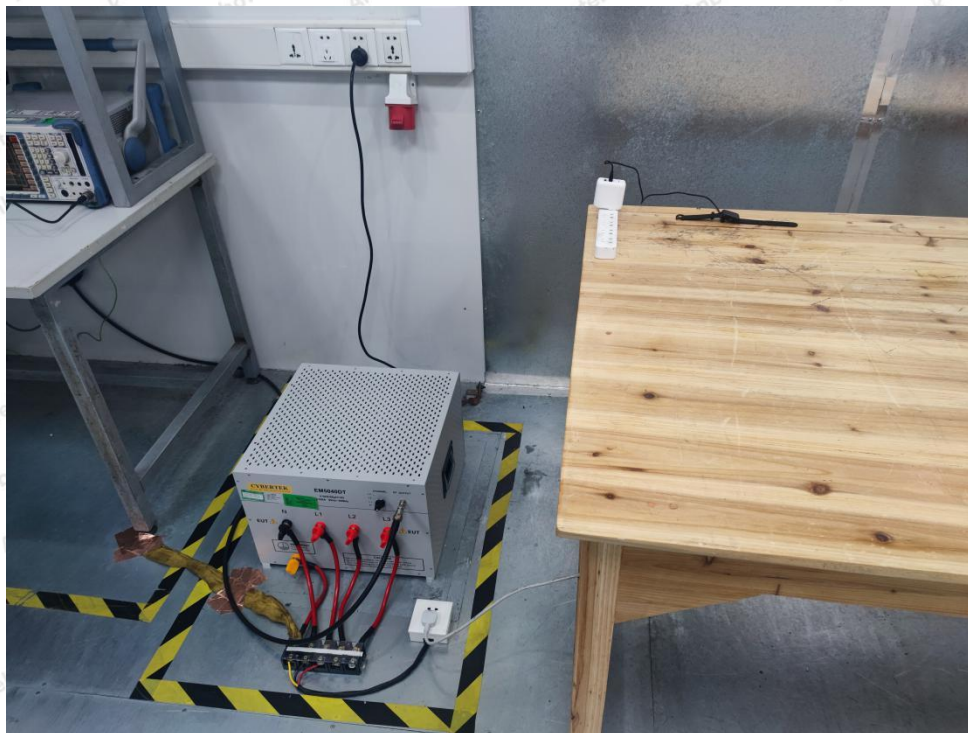
Photo of Conducted Emission Measurement
