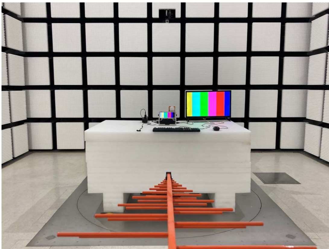
Radiated Emission Above 1GHz View
