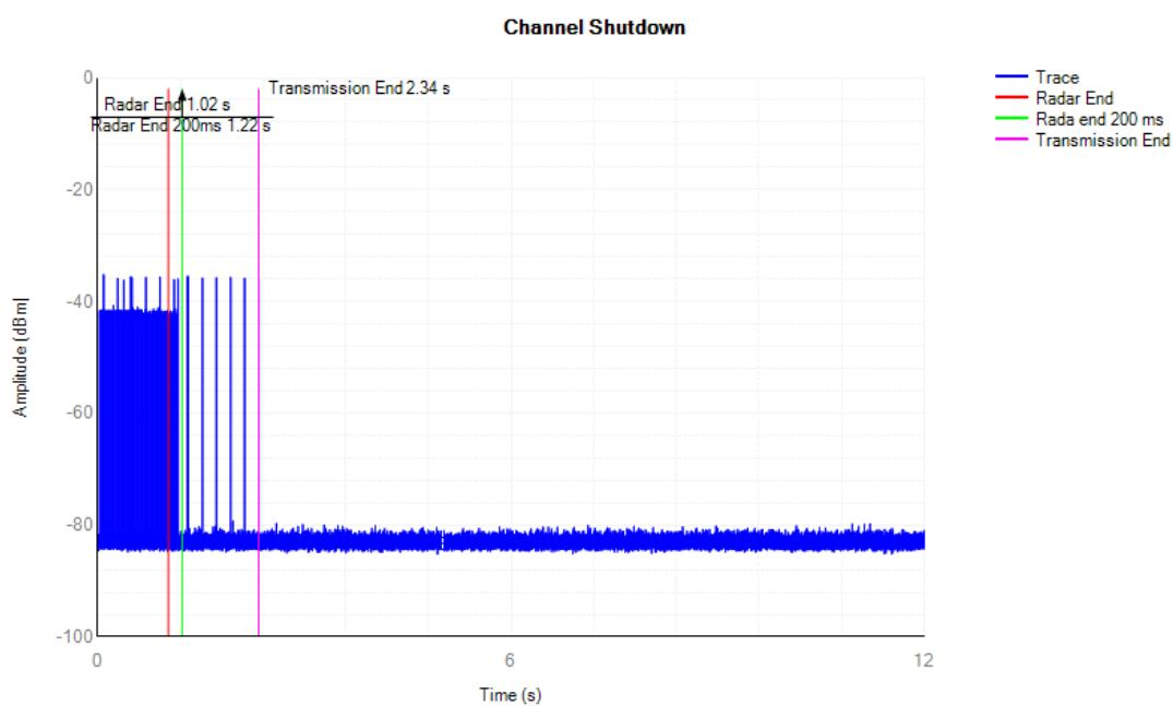
**Radar Type 0 Channel Closing Transmission**
