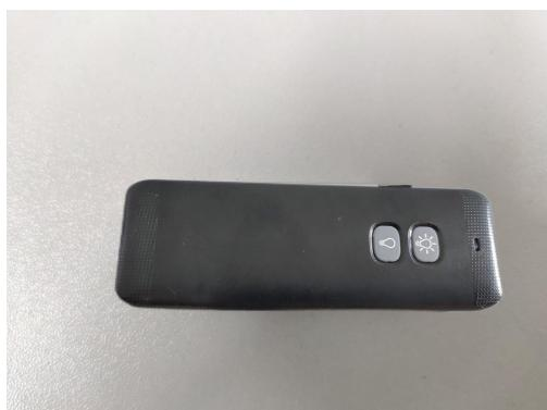
1. Press the button
