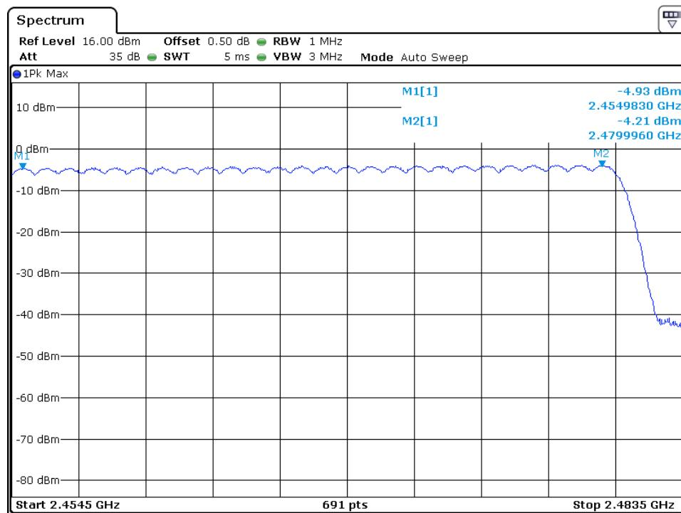
**4.6 Channel Separation (Carrier Frequency Separation)**
