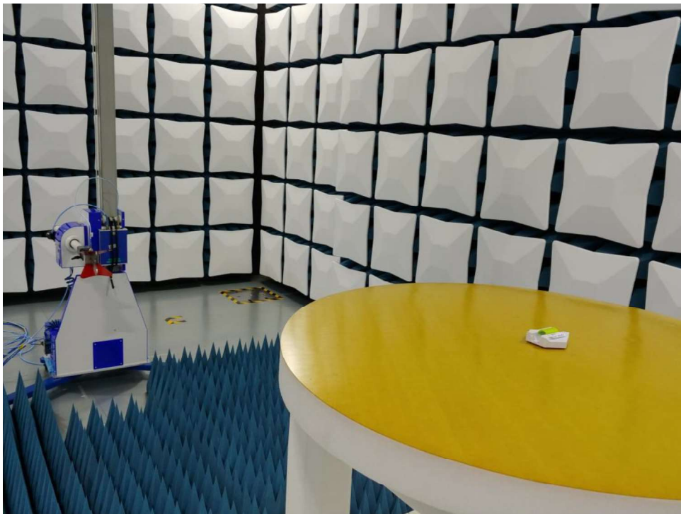
Set-up for Radiated Emission (1GHz above)
