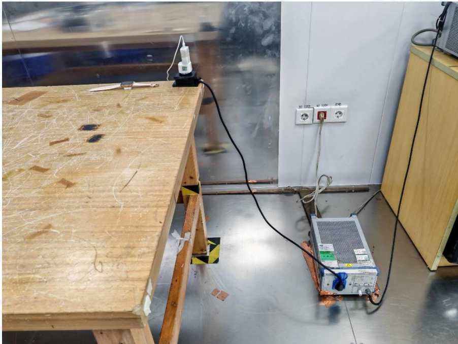
Photo of Setup for Radiated Emission (30MHz~1GHz)
