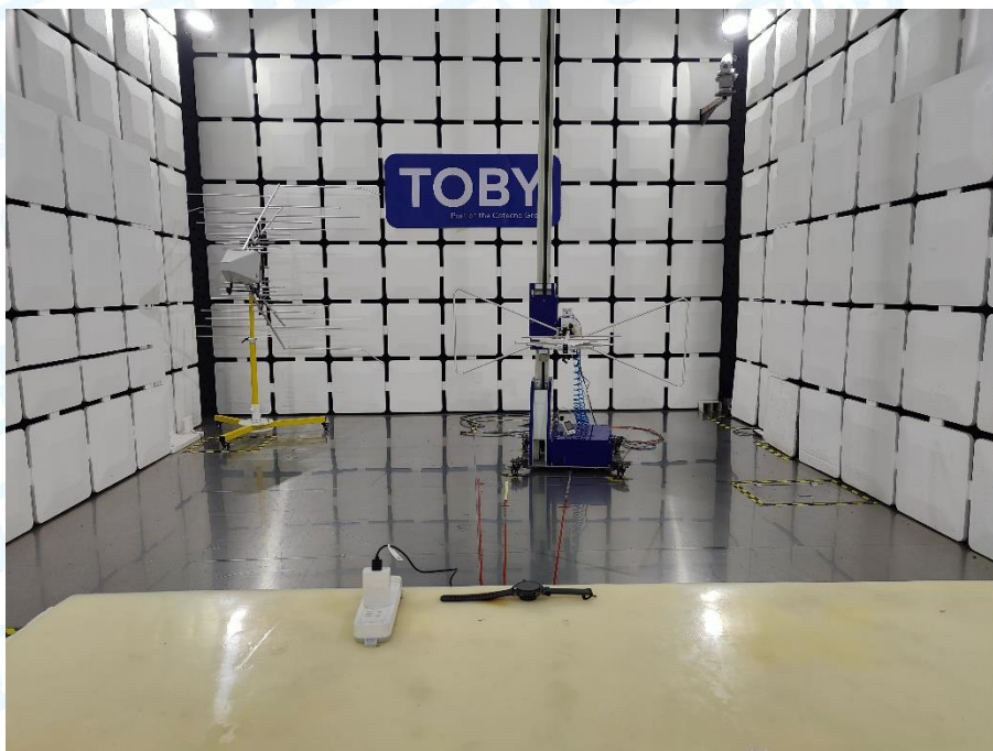
Photo of Setup for Radiated Emission (30MHz~1GHz)
