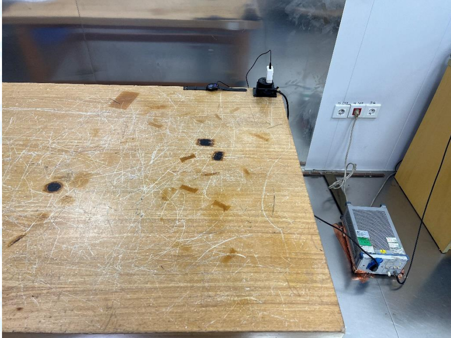
Photo of Setup for Radiated Emission (30MHz~1GHz)
