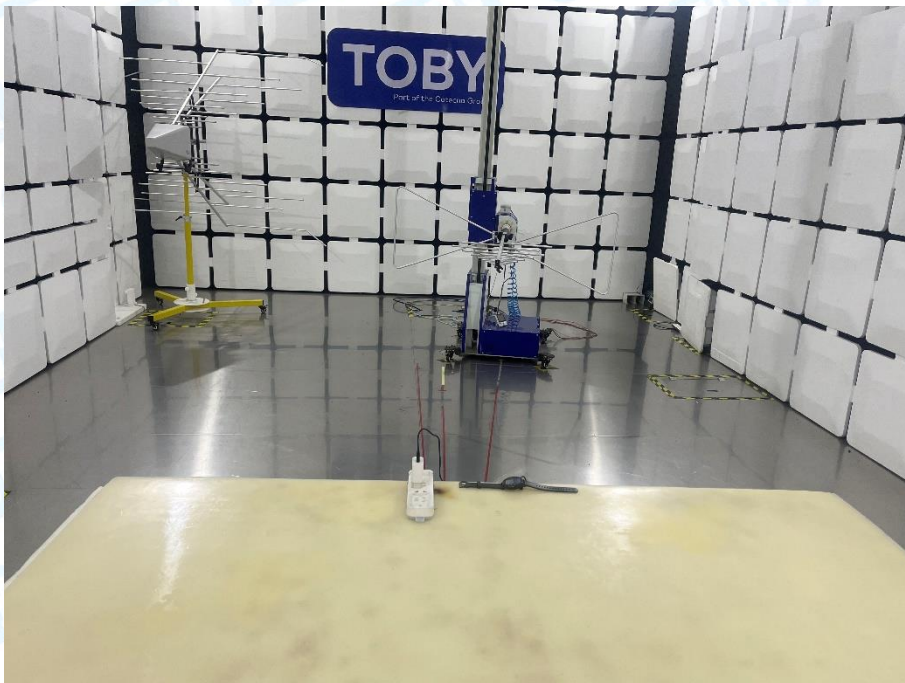
Photo of Setup for Radiated Emission (30MHz~1GHz)
