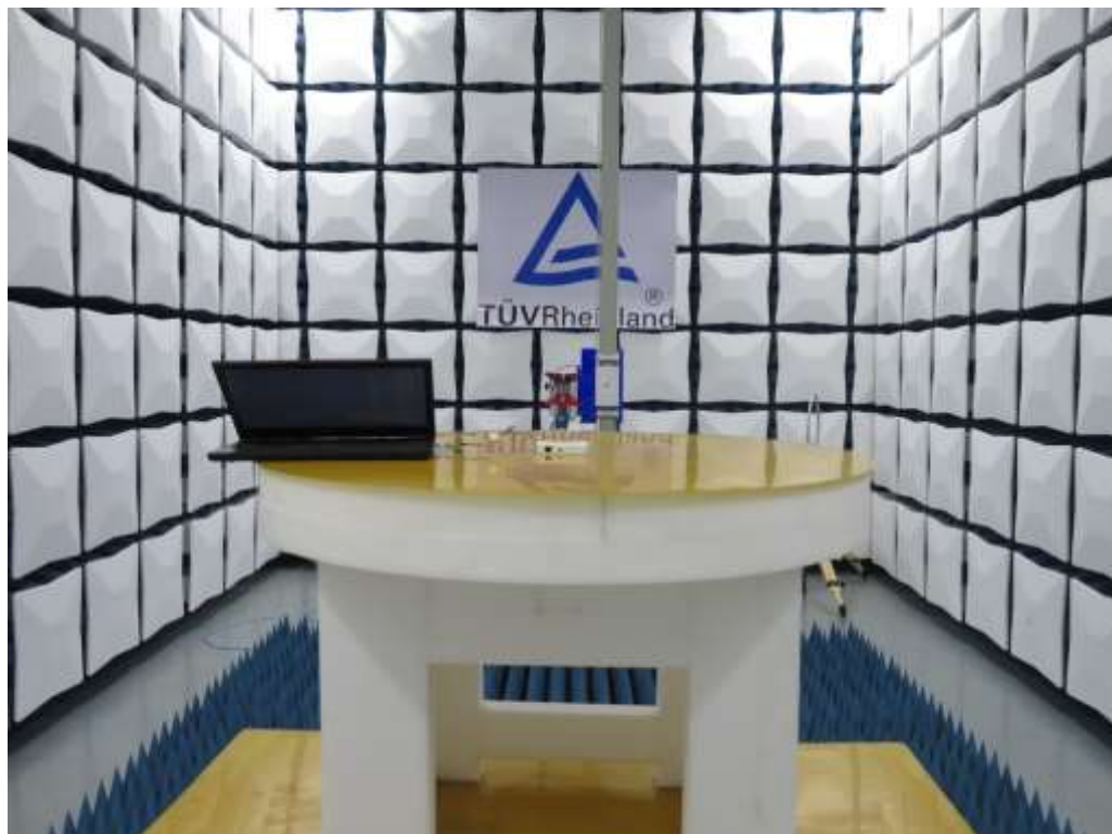
Photograph 2: Set-up for Radiated Spurious Emission, Above 1GHz
