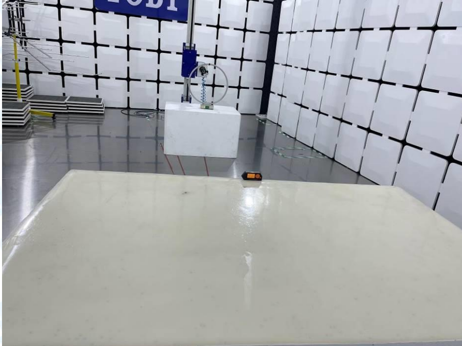
Photo of Setup for Radiated Emission (30MHz-1GHz)
