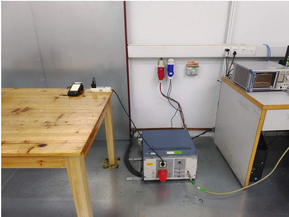
RADIATED EMISSION TEST SETUP BELOW 1GHZ
