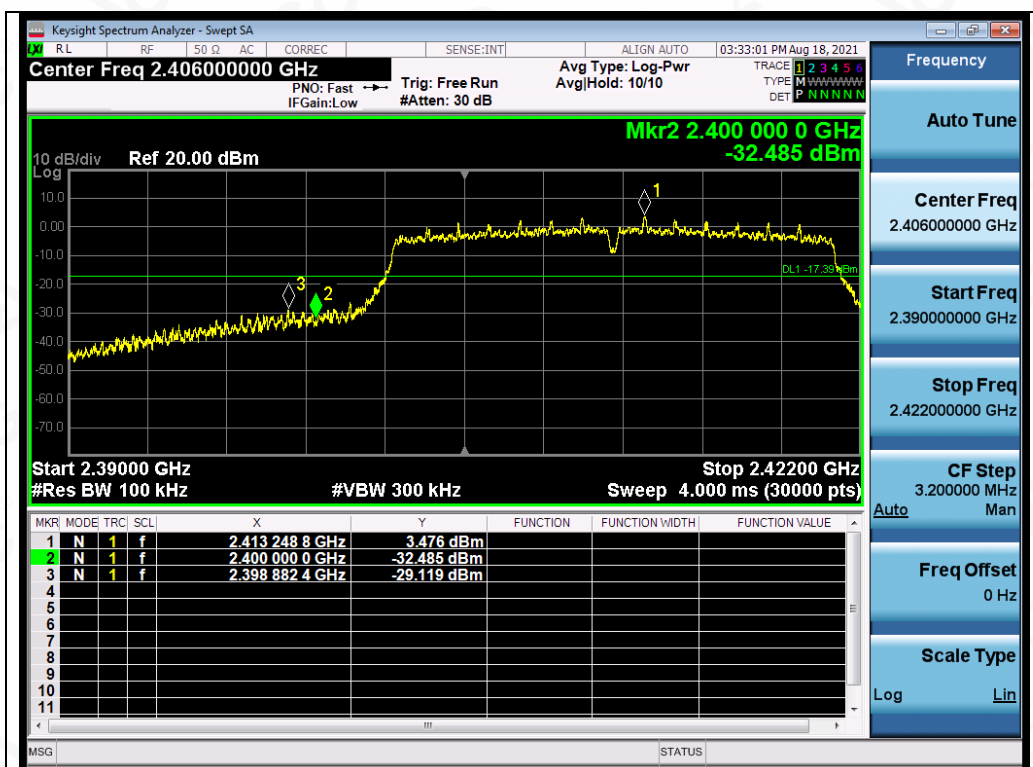
Test_Graph_802.11n20_ANT1_2412_MCS0_Lower Band Edge Emissions
