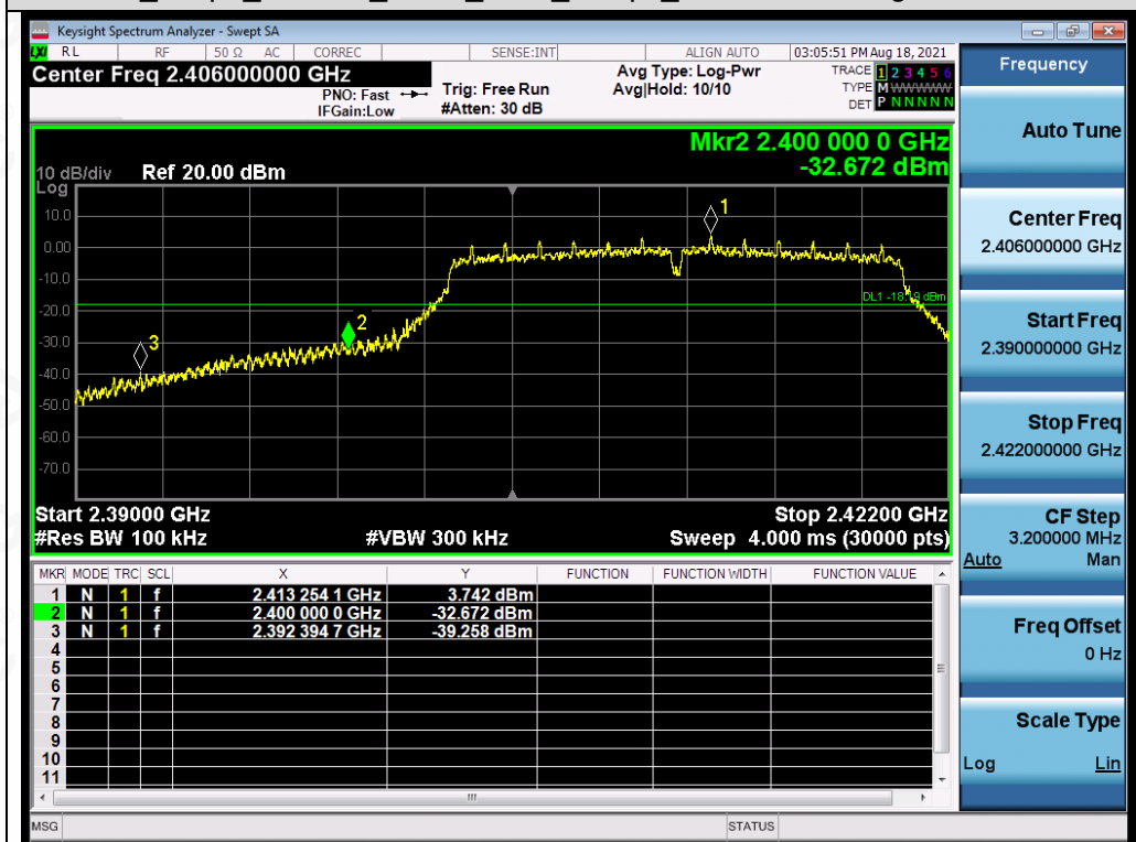
Test_Graph_802.11g_ANT1_2412_6Mbps_Lower Band Edge Emissions
