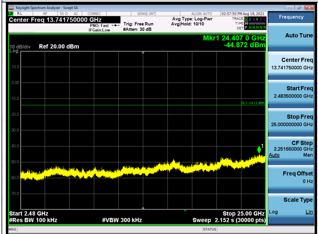
Test_Graph_802.11b_ANT1_2437_1Mbps_Higher Band Emissions
