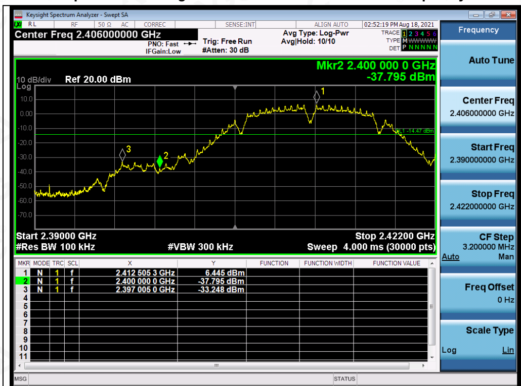
Test_Graph_802.11b_ANT1_2412_1Mbps_Lower Band Edge Emissions
