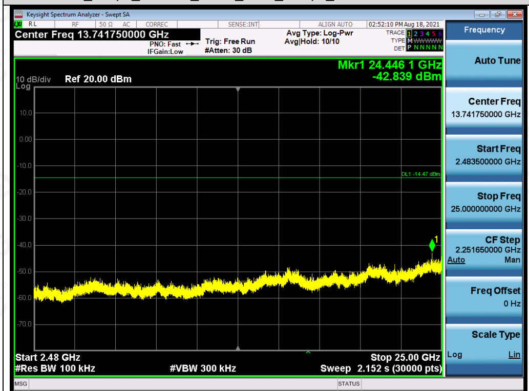
Test_Graph_802.11b_ANT1_2412_1Mbps_Higher Band Emissions
