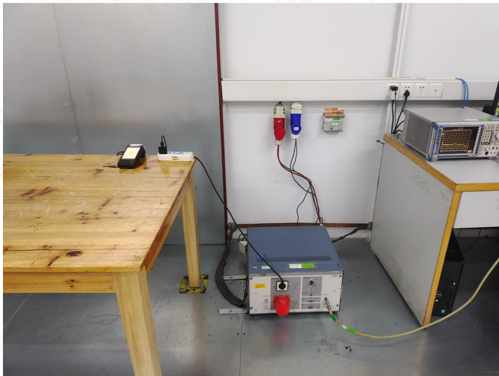
RADIATED EMISSION TEST SETUP BELOW 30MHz
