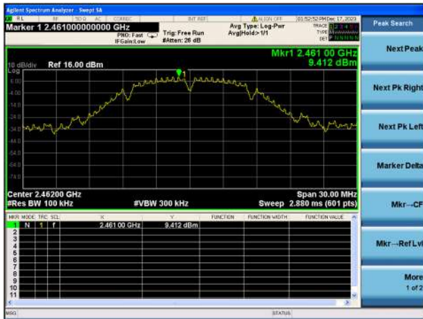
802.11b HIGH CHANNEL, CARRIER LEVEL
