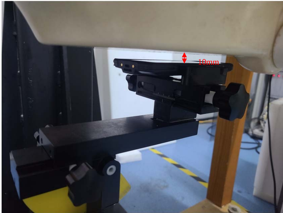
Body (Wron)Back Setup Photo (10mm)
