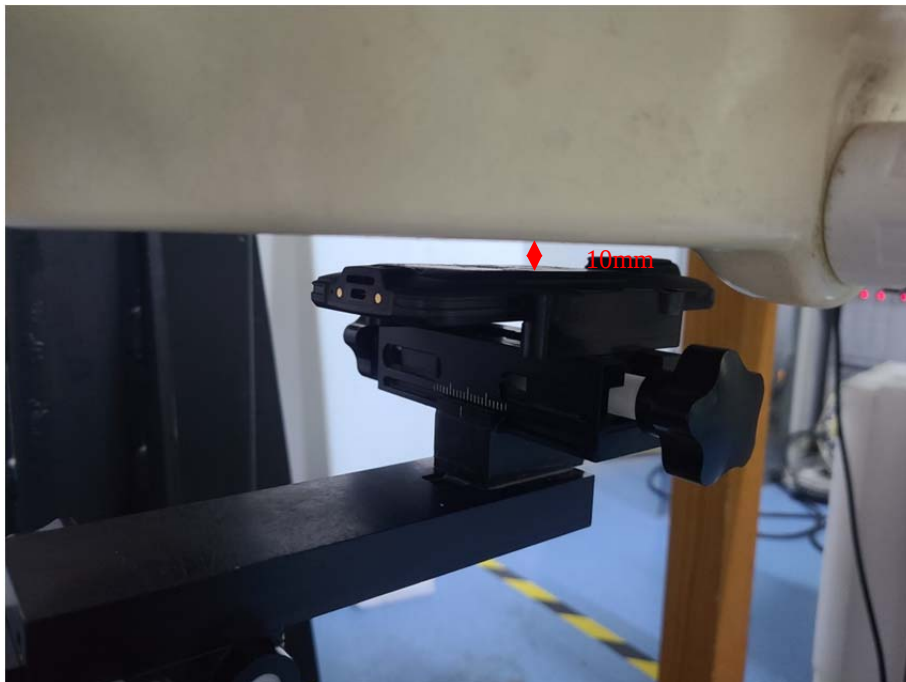
Body (Wron)Back Setup Photo (10mm)
