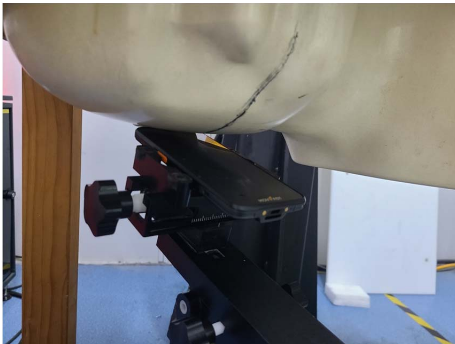
Head Right Tilt Setup Photo (0mm)
