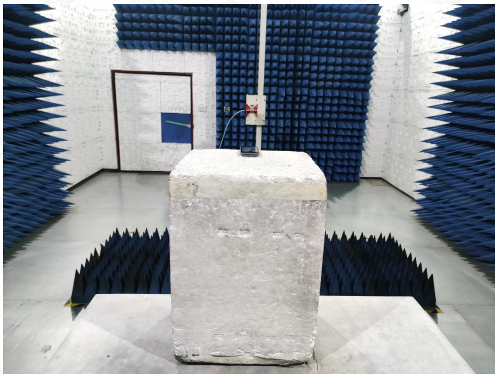
RADIATED EMISSION TEST SETUP BELOW 1GHZ
