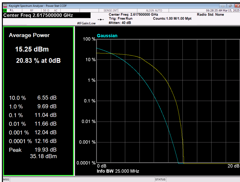
Band38 QPSK BW=5MHz Channel=38225 RB Size=25 Position=#0
