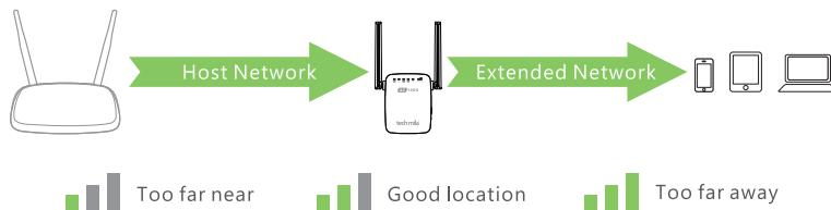
2. Wait until the signal LED is display two or three lattice signals. If not, relocate it closer to the router to achieve better signal quality.
