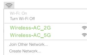
Disconnect the Ethernet (wired) connection from your computer (if any). Click the Wi-Fi icon in the top right corner of the screen, and connect to the Repeater's network (e.g. **Wireless-AC\_2G/5G**).
