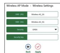
**SSID(2G)/SSID(5G)** - Enter a value of up to 32 characters. The same name of SSID (Service Set Identification) must be assigned to all wireless devices in your network. The default SSID is set to be **Wireless-AC\_2G** and **Wireless-AC\_5G**.
