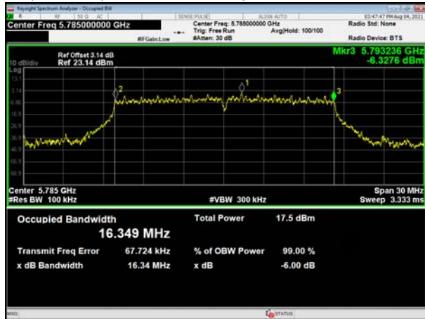
(802.11a) 99%Bandwidth plot on channel 157
