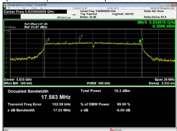
(802.11 n20) 99%Bandwidth plot on channel 165
