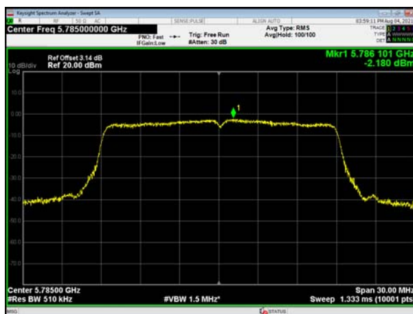
(802.11n20) PSD plot on channel 157
