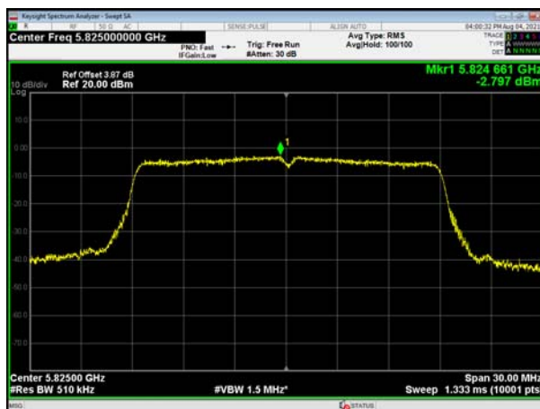
(802.11n20) PSD plot on channel 165
