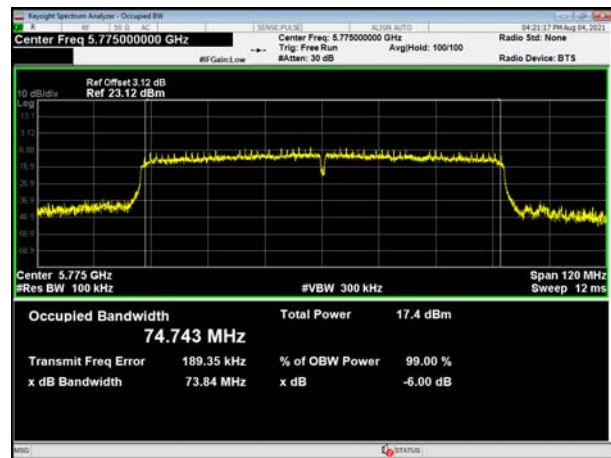
(802.11 ac80) 99%Bandwidth plot on channel 155
