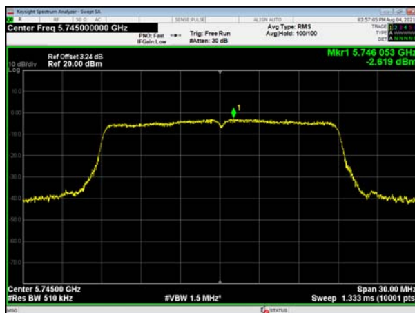
(802.11n20) PSD plot on channel 157
