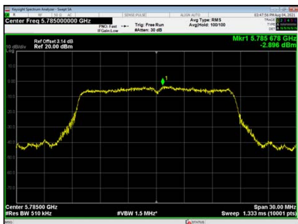
(802.11a) PSD plot on channel 157
