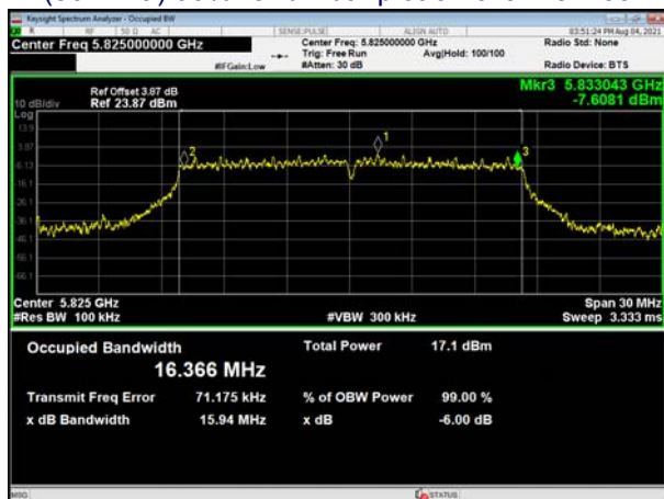
(802.11a) 99%Bandwidth plot on channel 165
