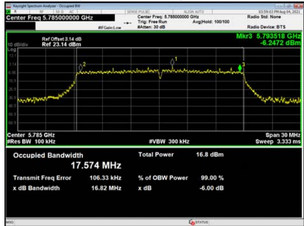
(802.11 n20) 99%Bandwidth plot on channel 157
