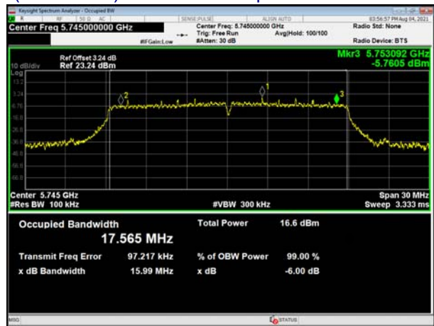
(802.11 n20) 99%Bandwidth plot on channel 149
