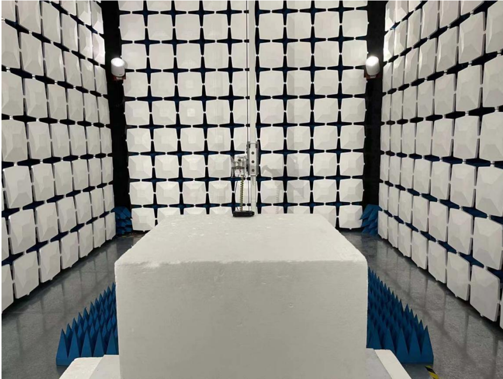
Above 1GHz for radiated emission test setup
