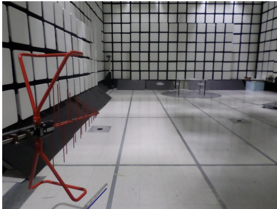
Figure 35: Radiated Emissions - 30-1000 MHz- Setup Antenna View
