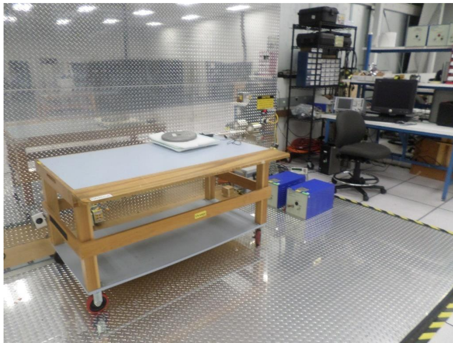
Figure 4. Conducted Emissions, 15.207(a), Test Setup, Front View
